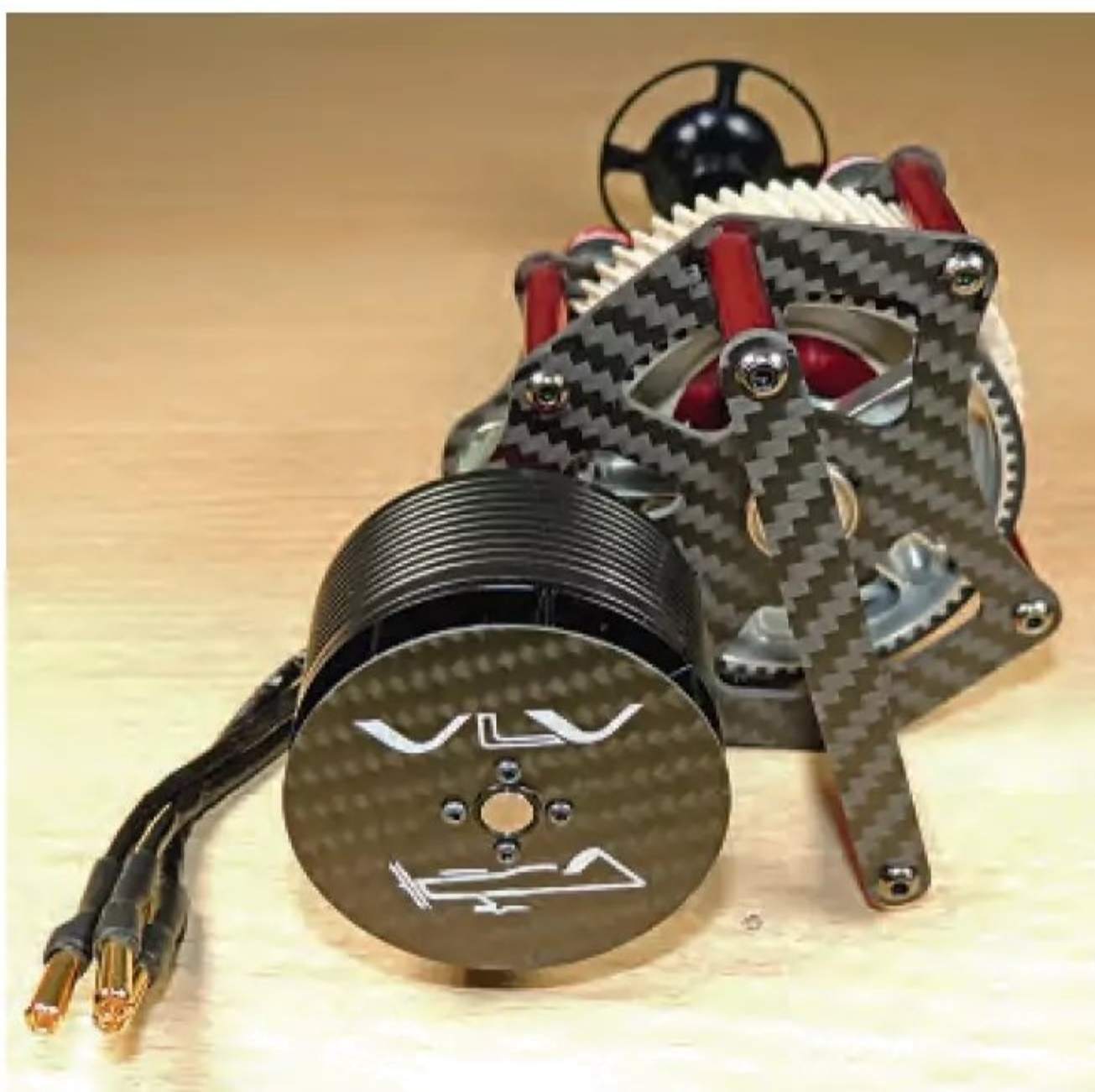
The rear motor disk is from 0.25mm carbon fibre plate and serves to form a cooling fan arrangement.
