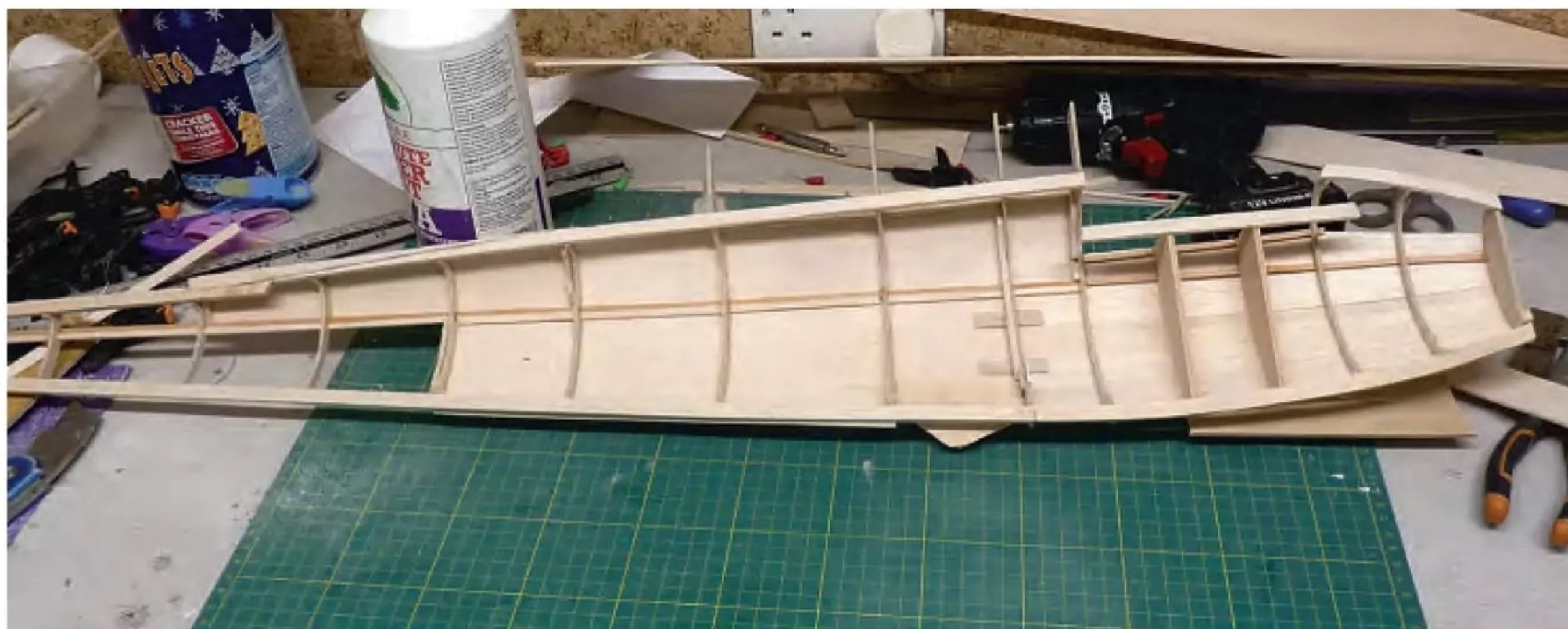
Half-shell removed from the board and ready for the other side.
