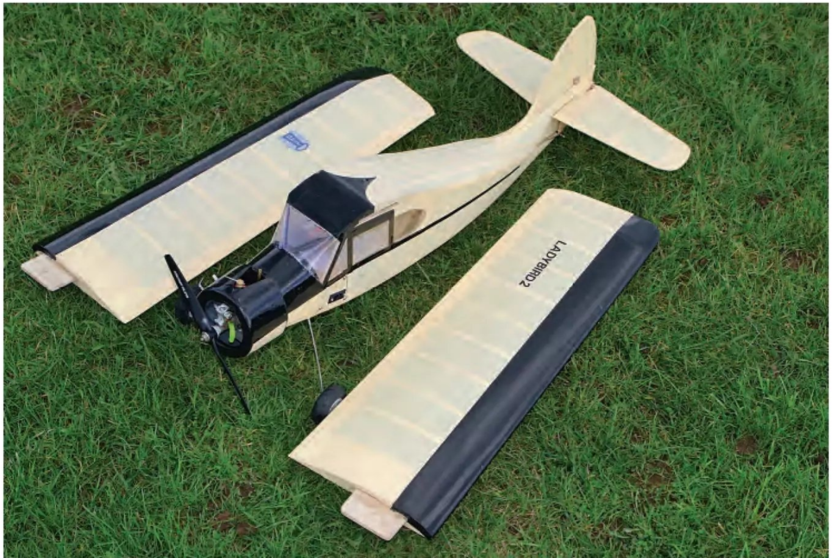
Ladybird shows its free flight origins in the use of plug-in wing panels which are designed to allow the wings to harmlessly part company with the fuselage in the event of a heavy landing. Gentle R/C guidance should forestall that - hopefully!
