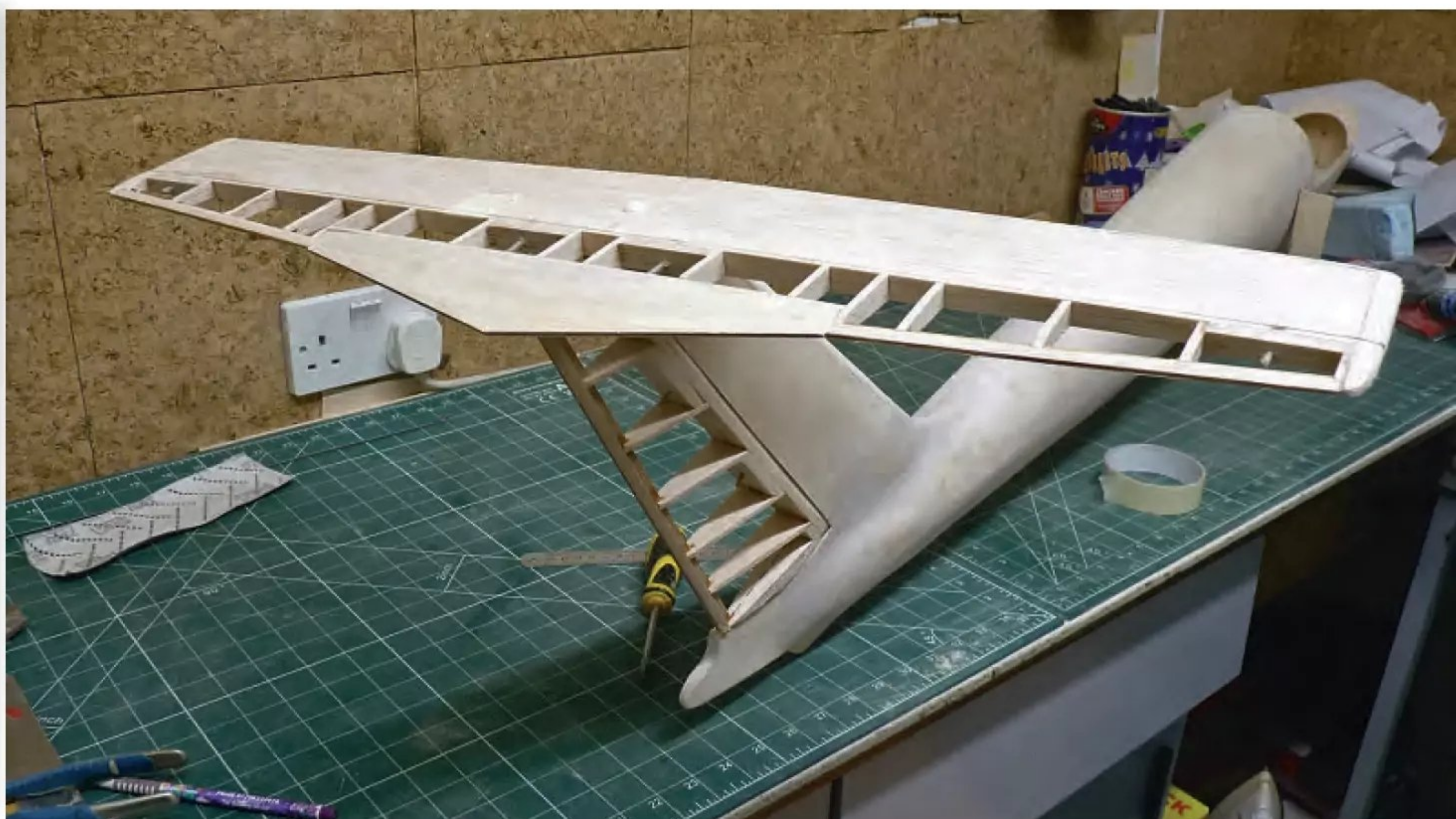
Nearly completed tail end.
