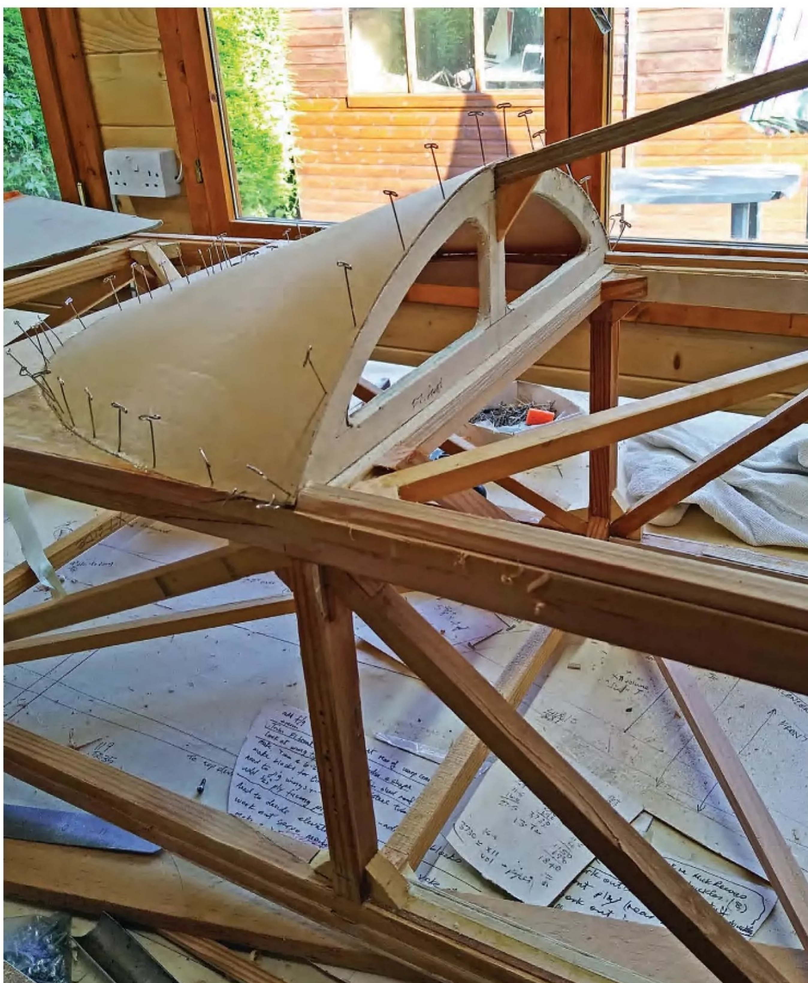
Whilst the fuselage was inverted new half round lite ply formers were added for the lower front fuselage fairing, followed by 0.8 mm scarf jointed ply panels.
