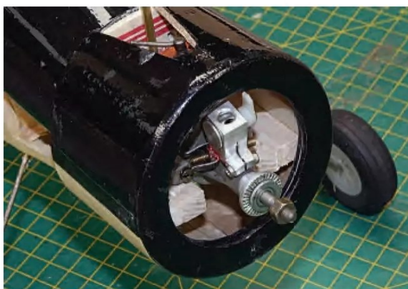
With the cowl slipped into place it became obvious that both the compression screw and needle would need extending to allow easy adjustment.
