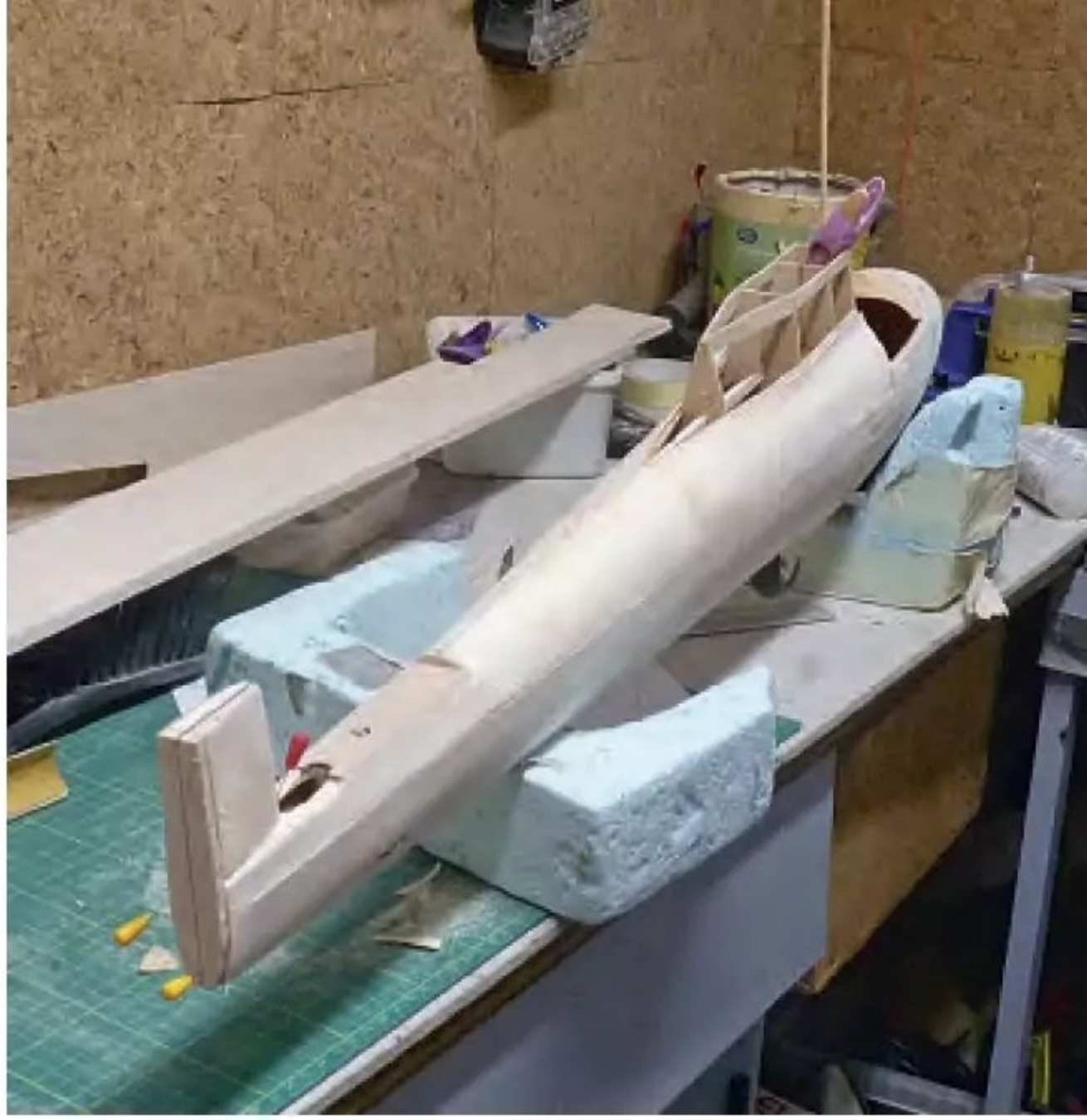
Using a vertical marker to line up the fin post before gluing.
