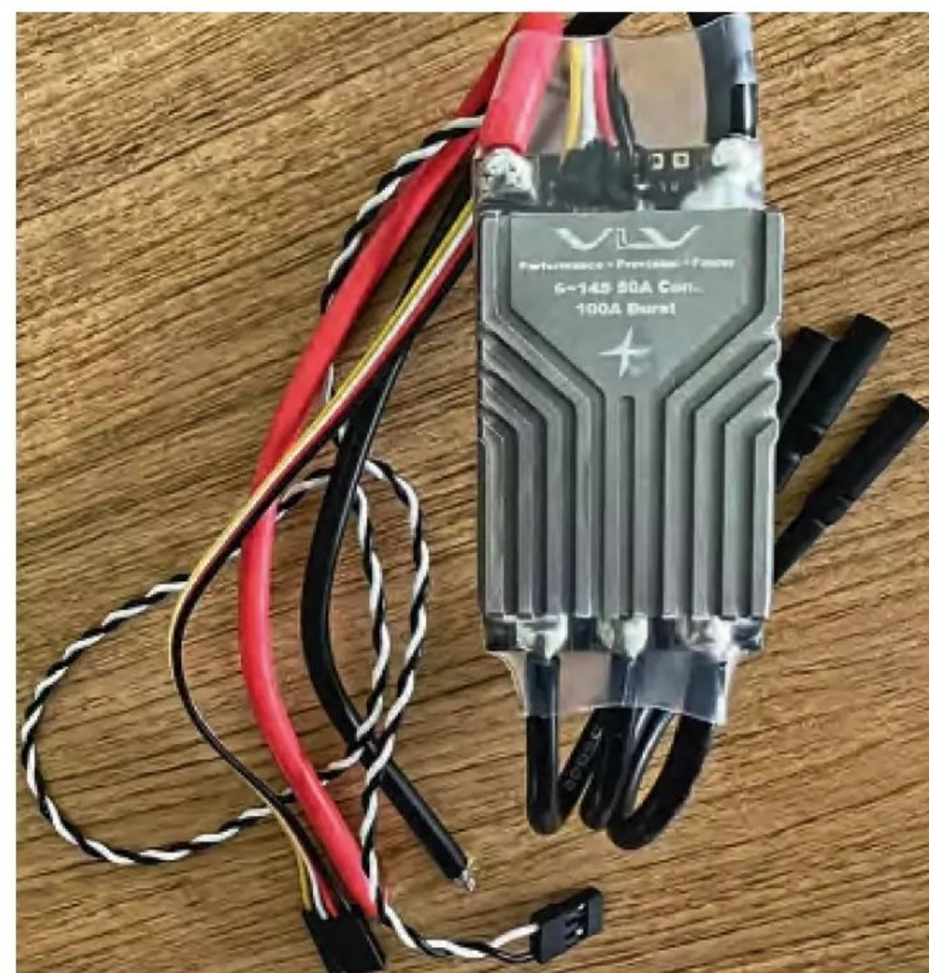
VLV ESC rated to 80A continuous current.
