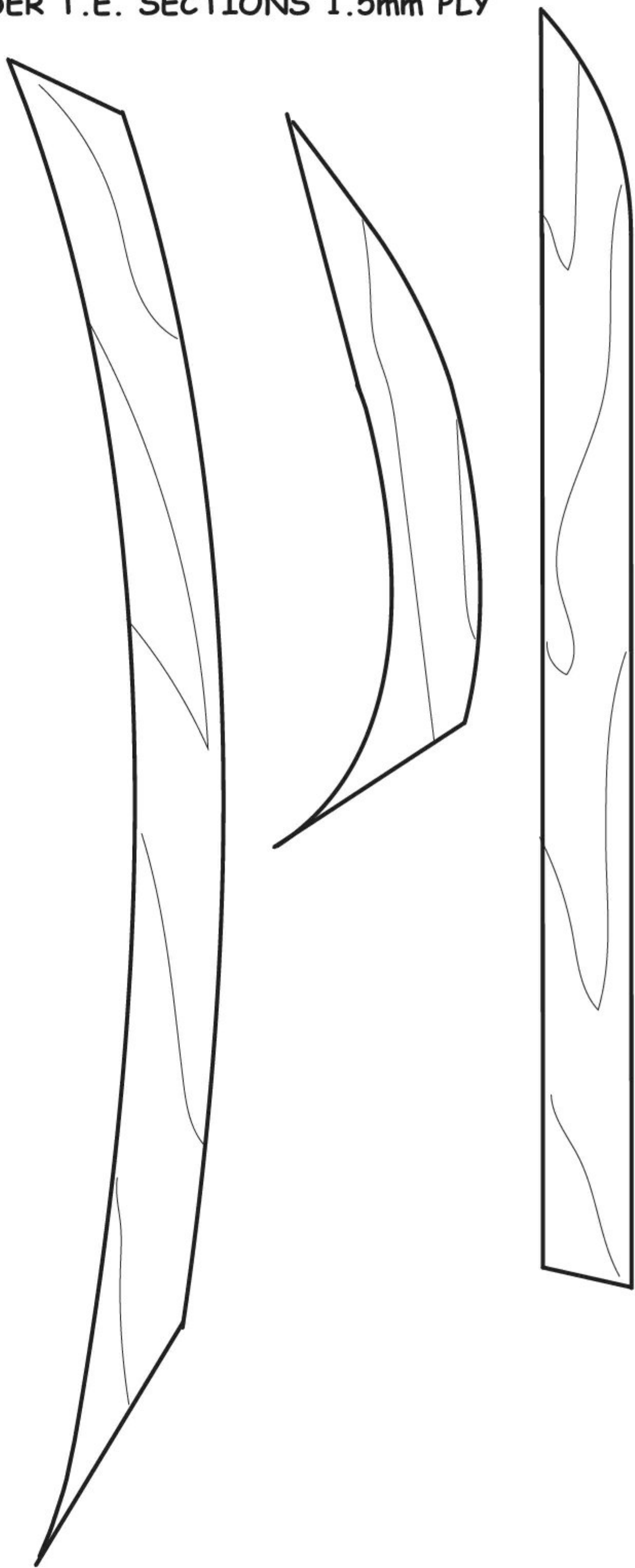
RUDDER T.E. SECTIONS 1.5mm PLY
