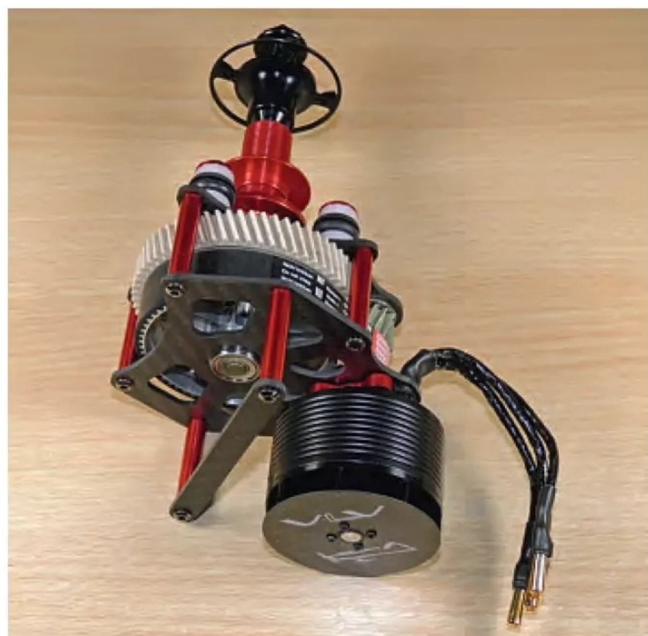
Rear view of the VLV contra drive.
