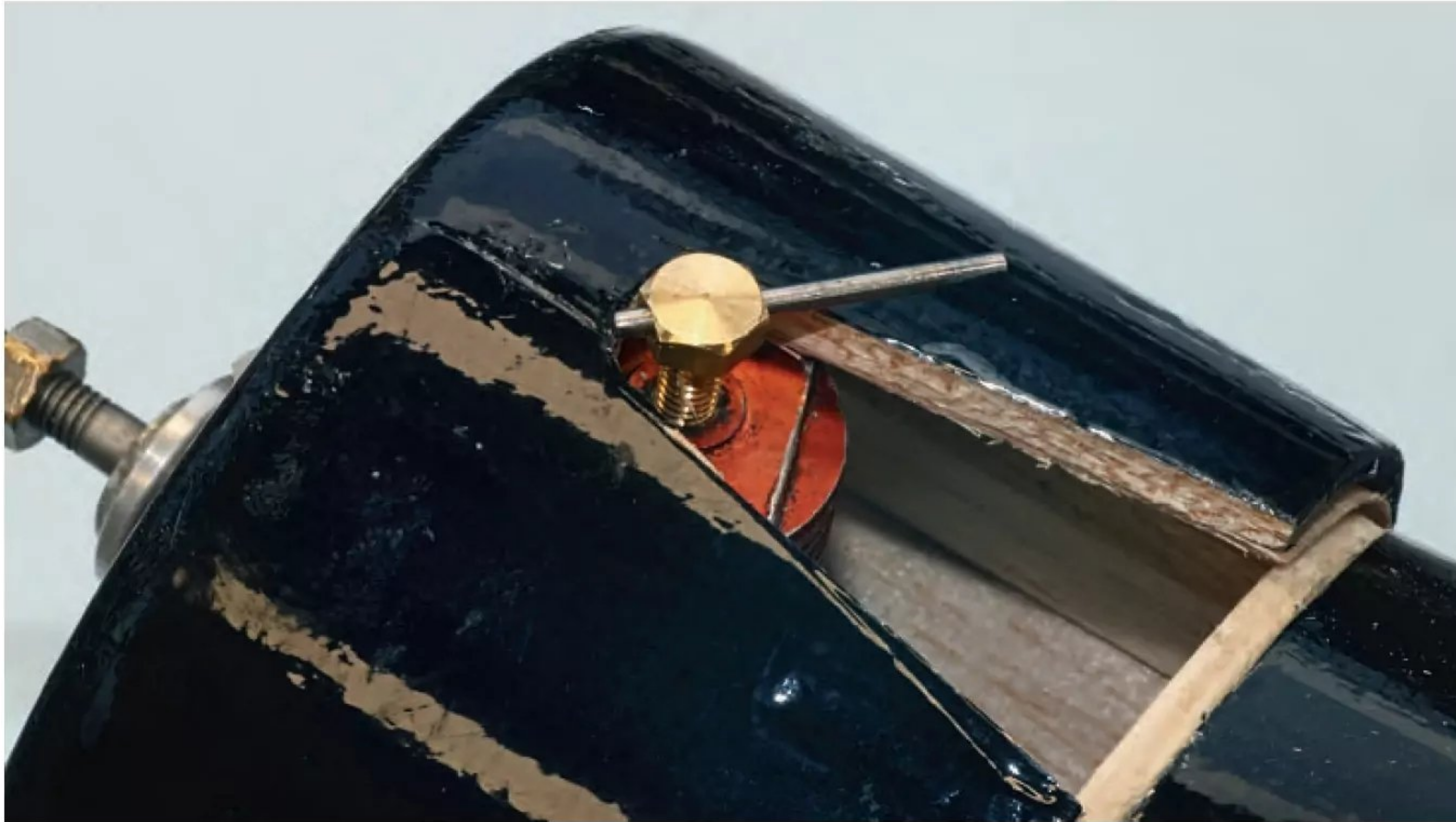
The head of the brass comp screw was cross-drilled and a piano wire tommy bar pressed into place.
