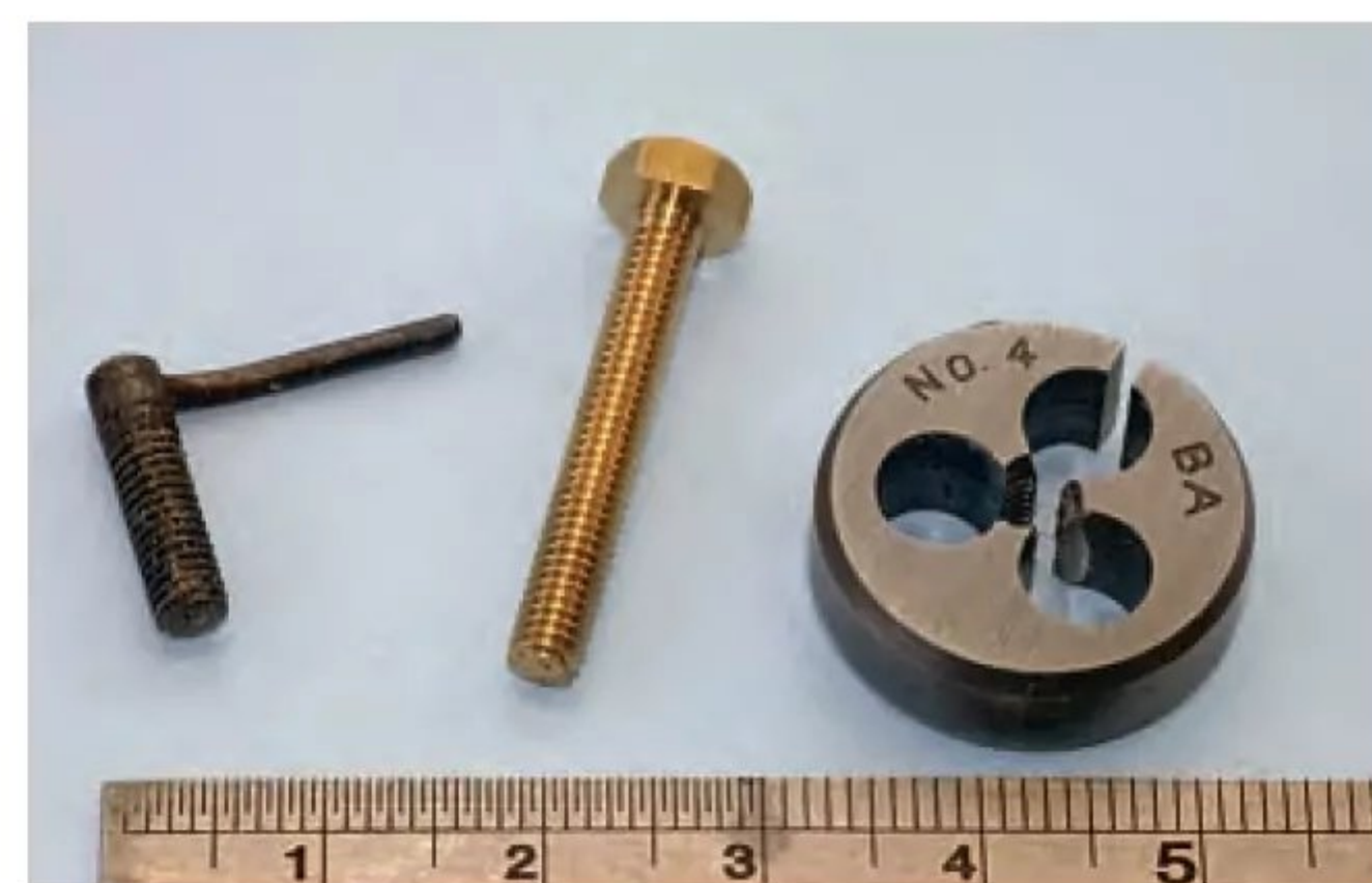
The 4 BA comp screw was stood down in favour of a similarly threaded brass bolt which was cut to a suitable length. The threading tap wasn't needed in the end.
