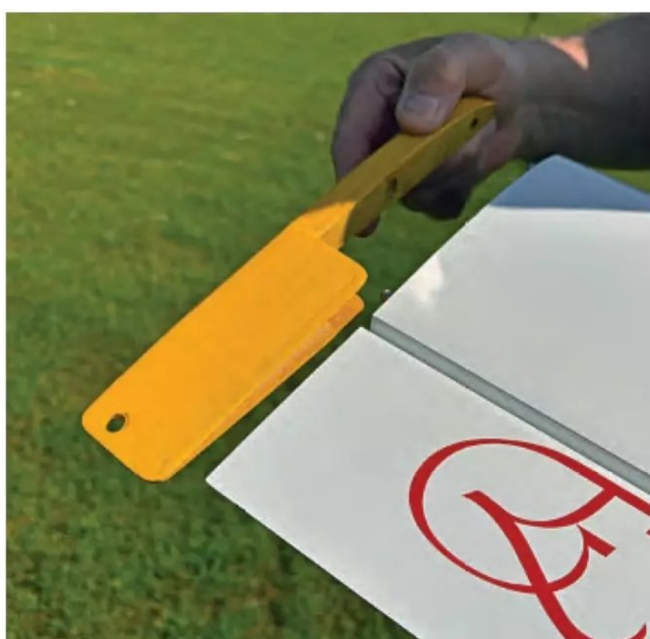
I liked Bob Ryan's neat homemade wing tip protectors that also protect control surfaces and servos from knocks.
