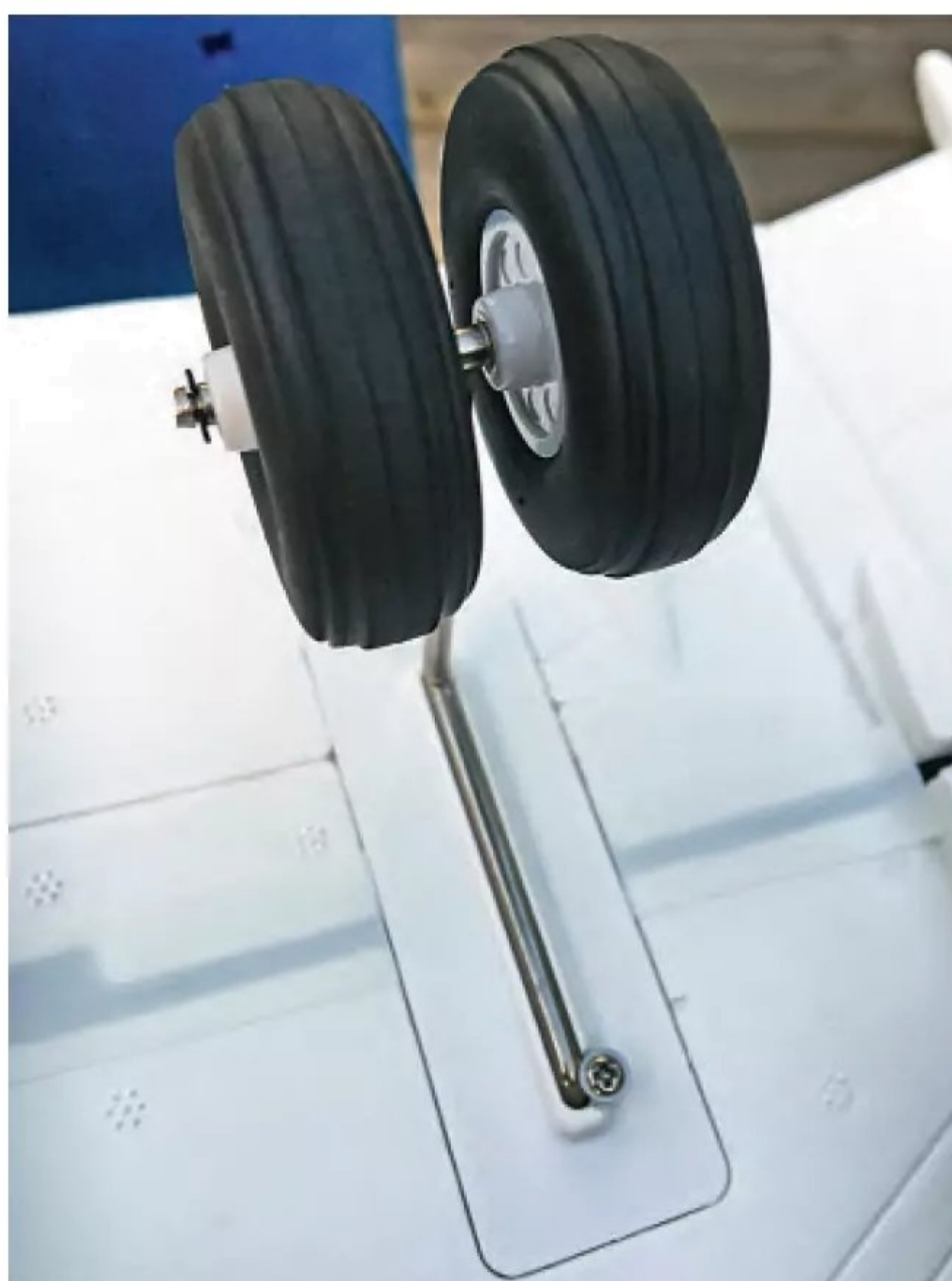
Torque slots for the main undercarriage legs run chordwise. Each leg is secured with just one screwhead. Absolutely minimalist but has worked well so far.
