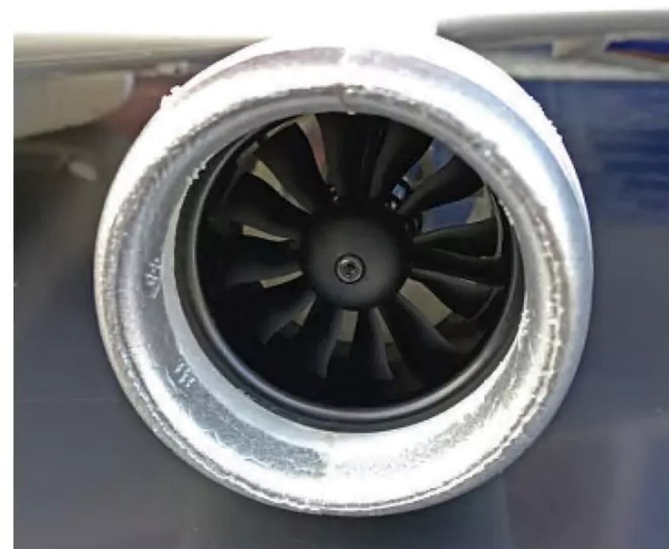
Each 40 mm, 12 blade fan unit sits in a realistic dummy turbofan nacelle. Quiet and efficient.
