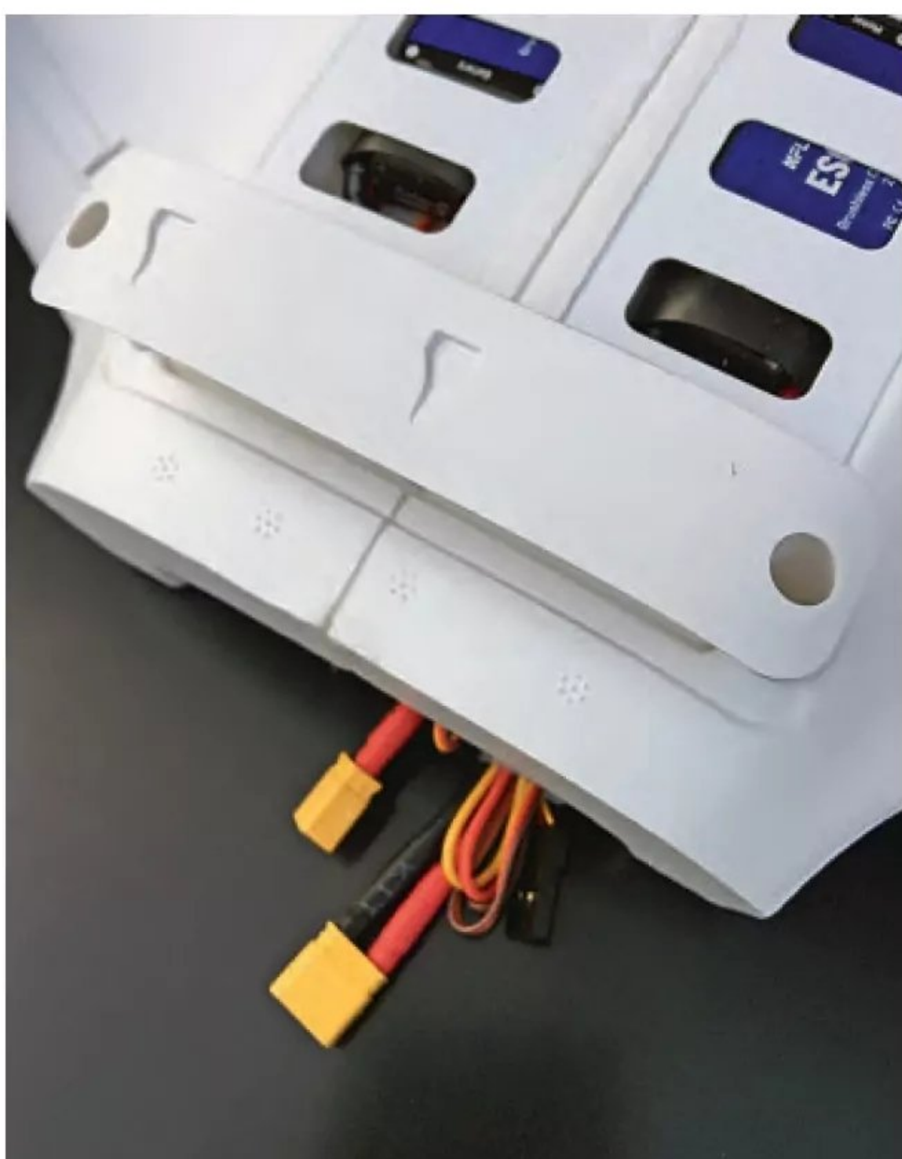
Two braces, fore and aft, keep the wings together and through screws join the panels to the fuselage.
