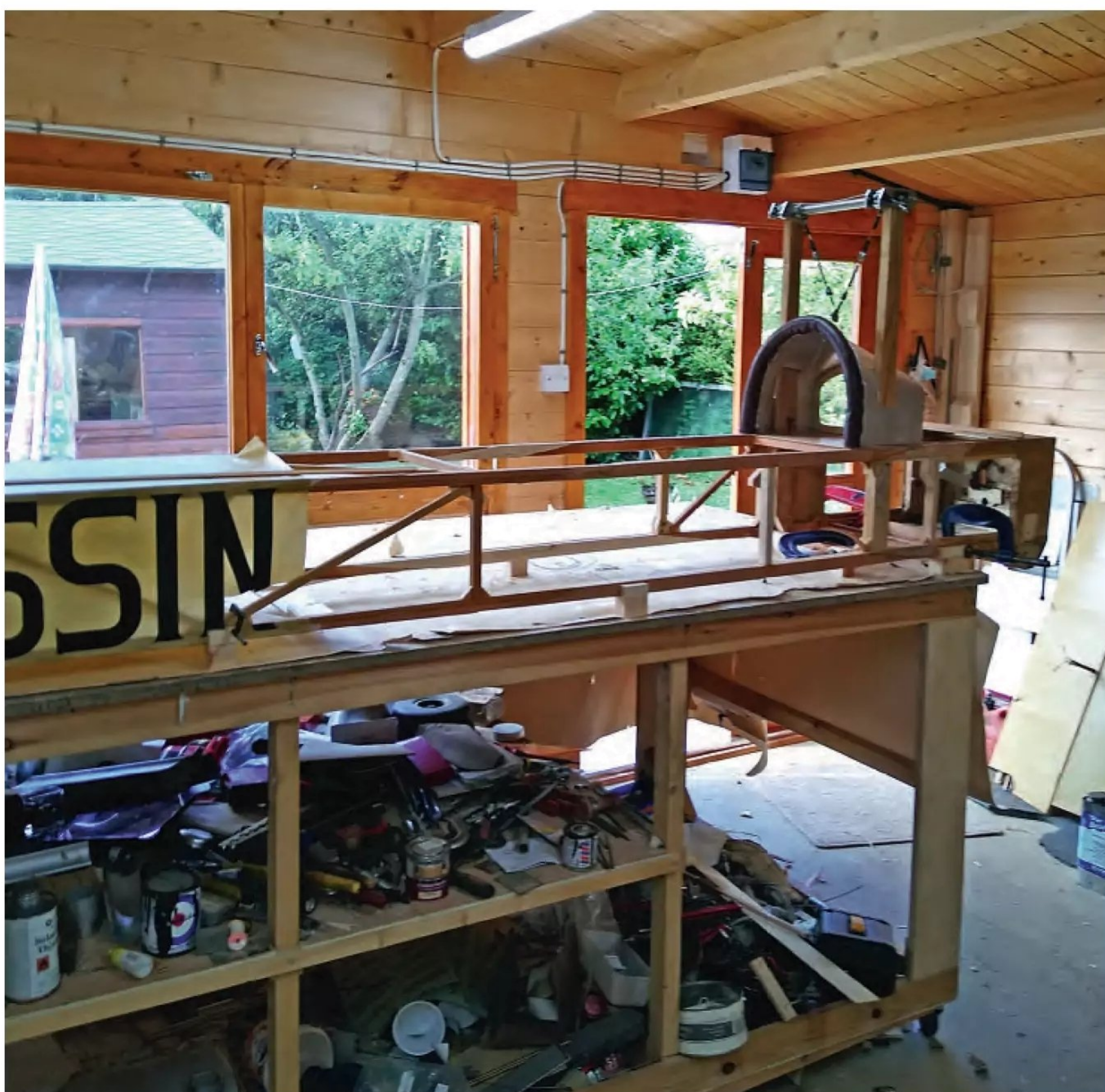
The front and rear parts of the fuselage were clamped to fourteen blocks mounted on Ian's workbench to hold them in the correct position.
