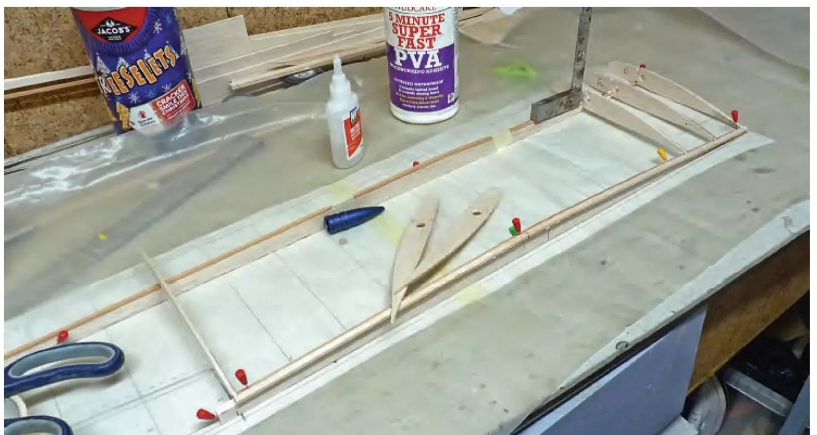
First stage of wing construction with lower spar and trailing edge set up on gull jigs.
