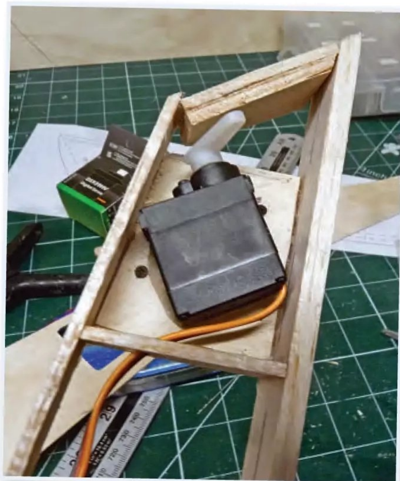
Squeezing a servo into the top of the Foka 5 fin.
