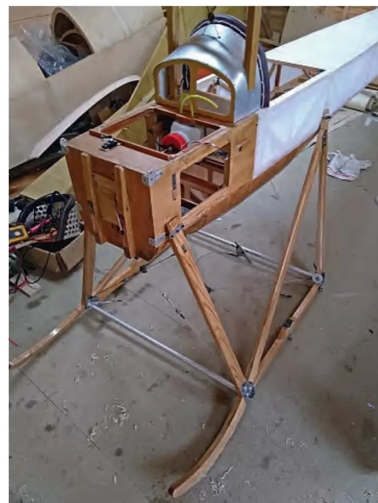
Metal plates were salvaged from the original undercarriage but new Allen bolts and bracing cables were fitted to hold it all together.
