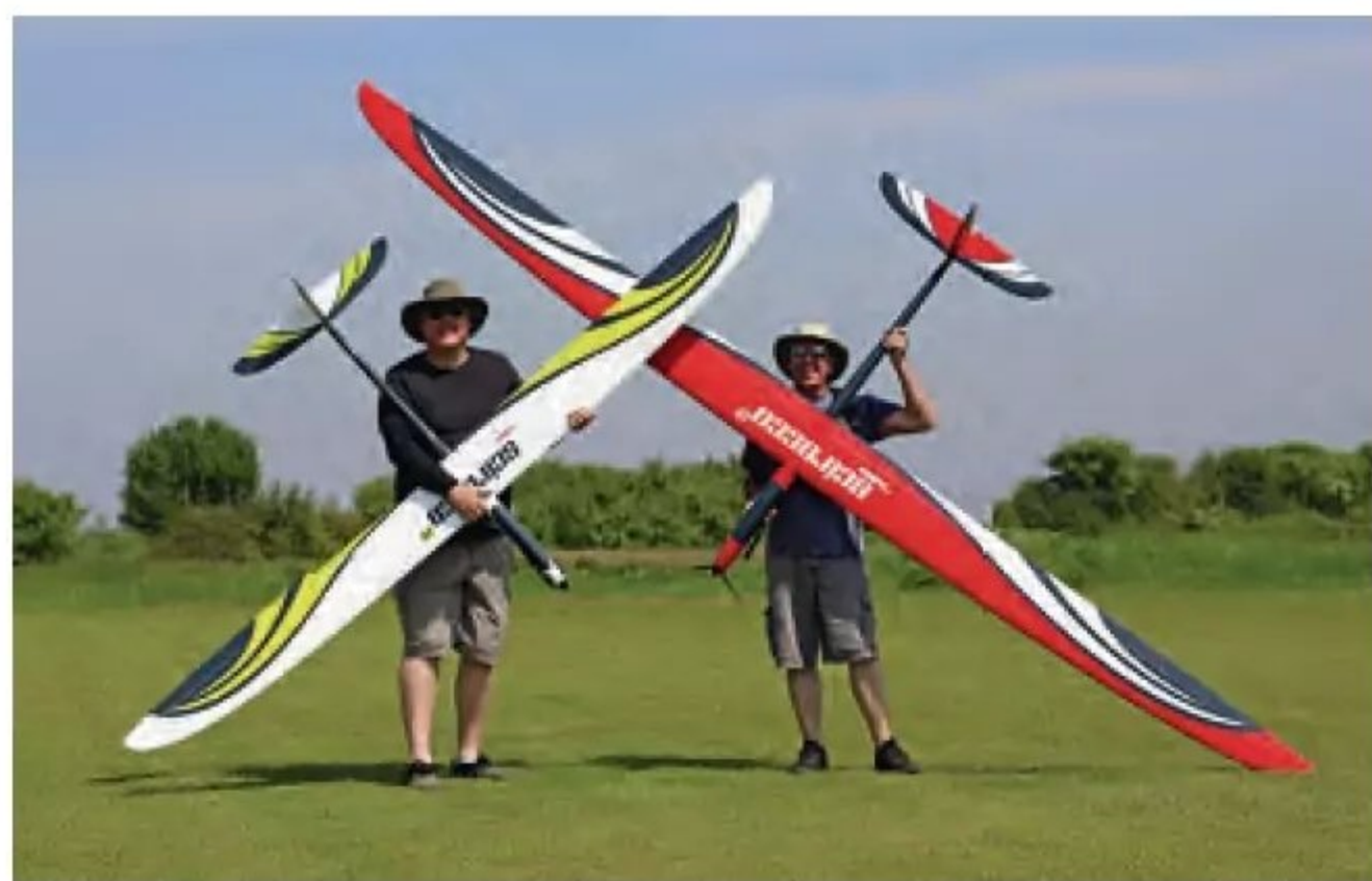
Scirocco fans, Dave Wray (left) with the 3.75 m span XS version and Dean Tilley with his 4.5 m XL version. At the flat field or hill, these fully moulded machines are great all-round performers.
