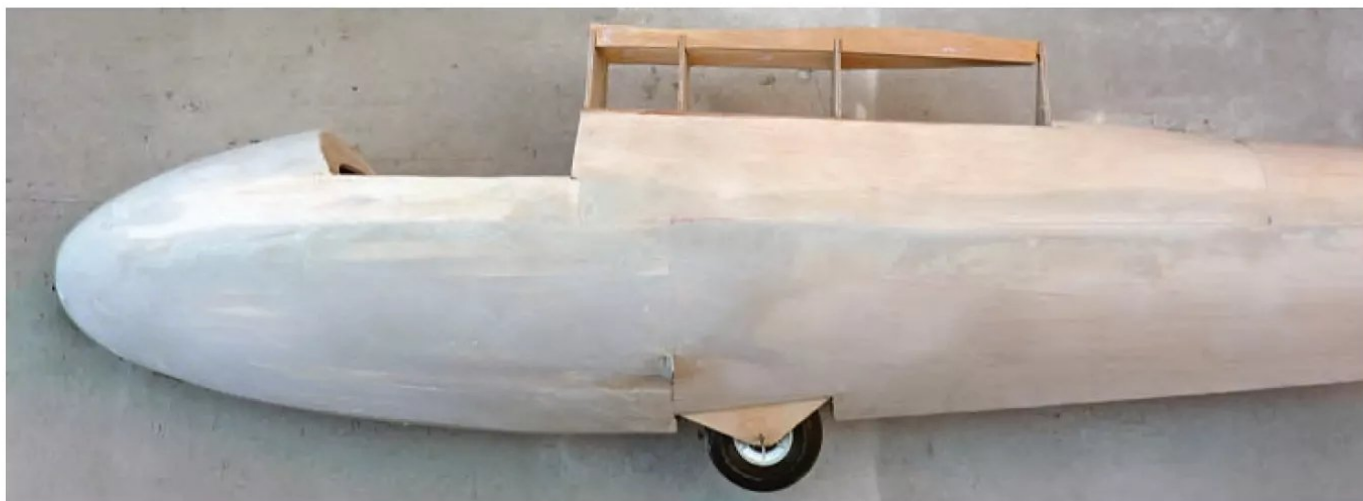
Car body filler finishes off the shape of the fuselage.
