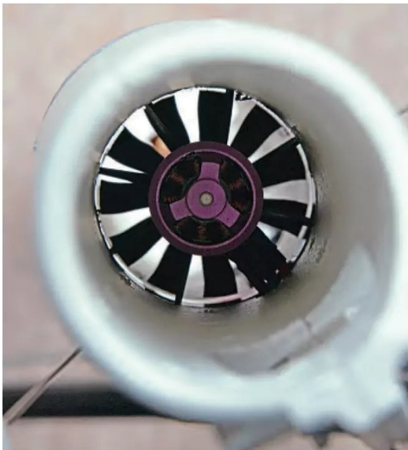
Inside the thrust tube showing the close fitting 50mm, 11 blade fan. Quiet and efficient.
