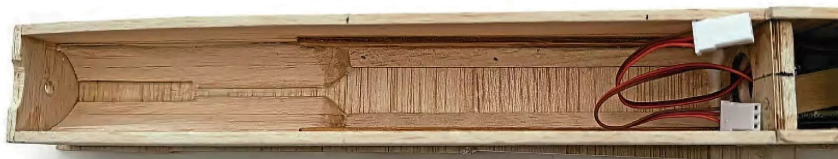
Left: Holes in the ply/balsa sandwich formers were cut so that the boom would slide into the fuselage and be well aligned down its length.
