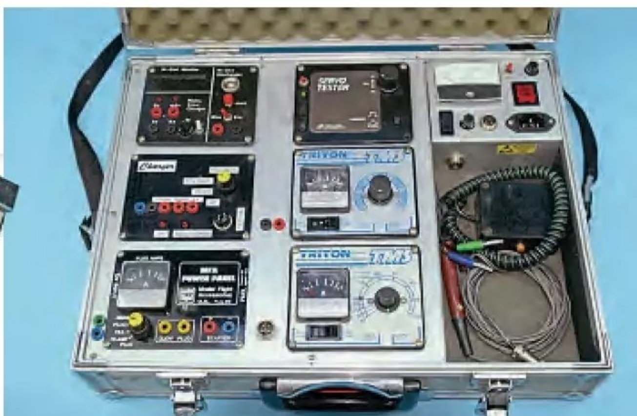
My early attempt at an all-in-one field starting / charging station. It included a 12-volt gel-cell but could also be mains powered for shed use. A great idea - until you tried carrying it!
