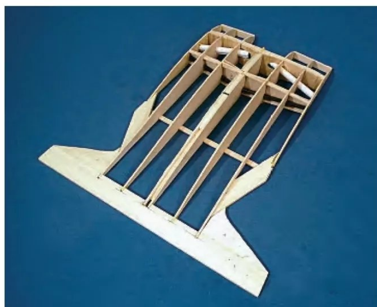
Basic centre section construction.
