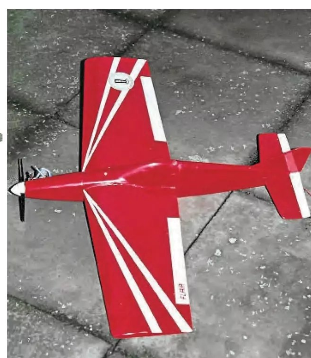
Stephen Farmer's Dara 20 was powered by an Enya 19BB and although not the most powerful .20 size motor the model was still pretty fast.
