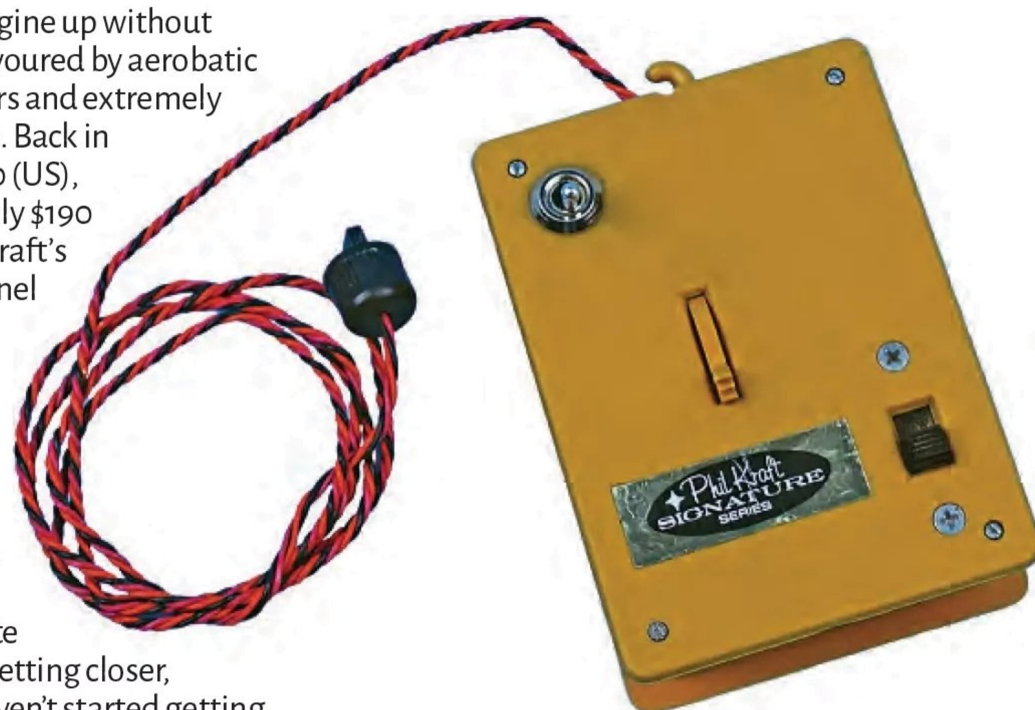
Last column's mystery item was the Kraft DSC unit. It allowed Direct Servo Control of a model's throttle and retracts without switching your transmitter on. Perfect for busy flying sites.
