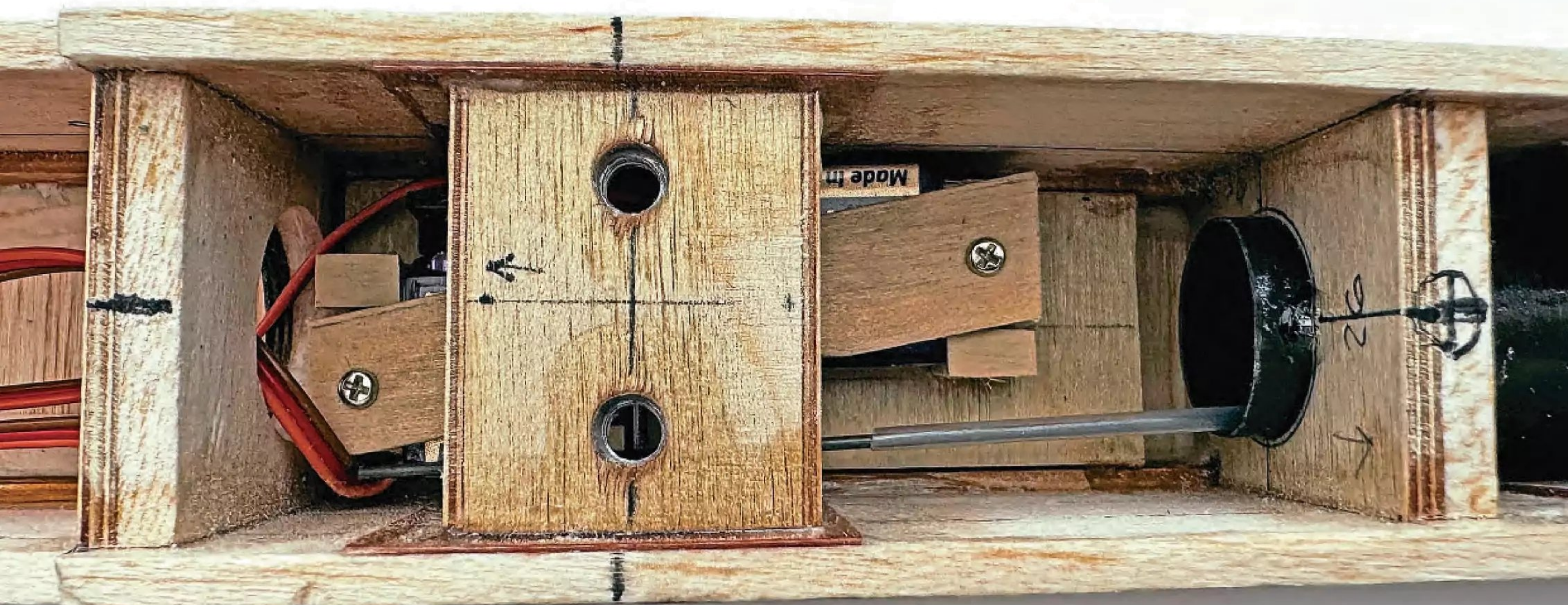
The wings attach to the fuselage using nylon bolts that thread into custom made aluminium plates. The servo mount is situated below.
