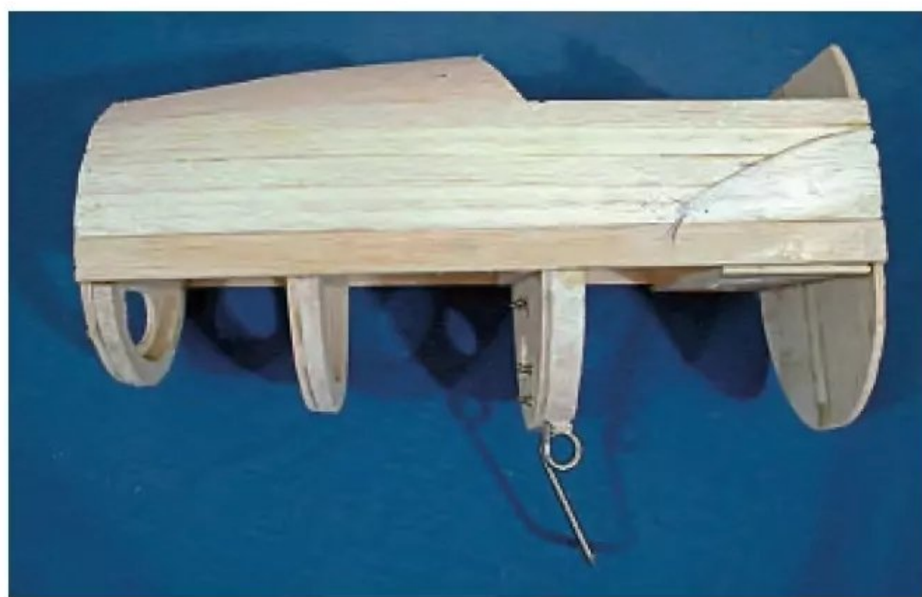
Fuselage with top planking fitted. Note the marked wing location.
