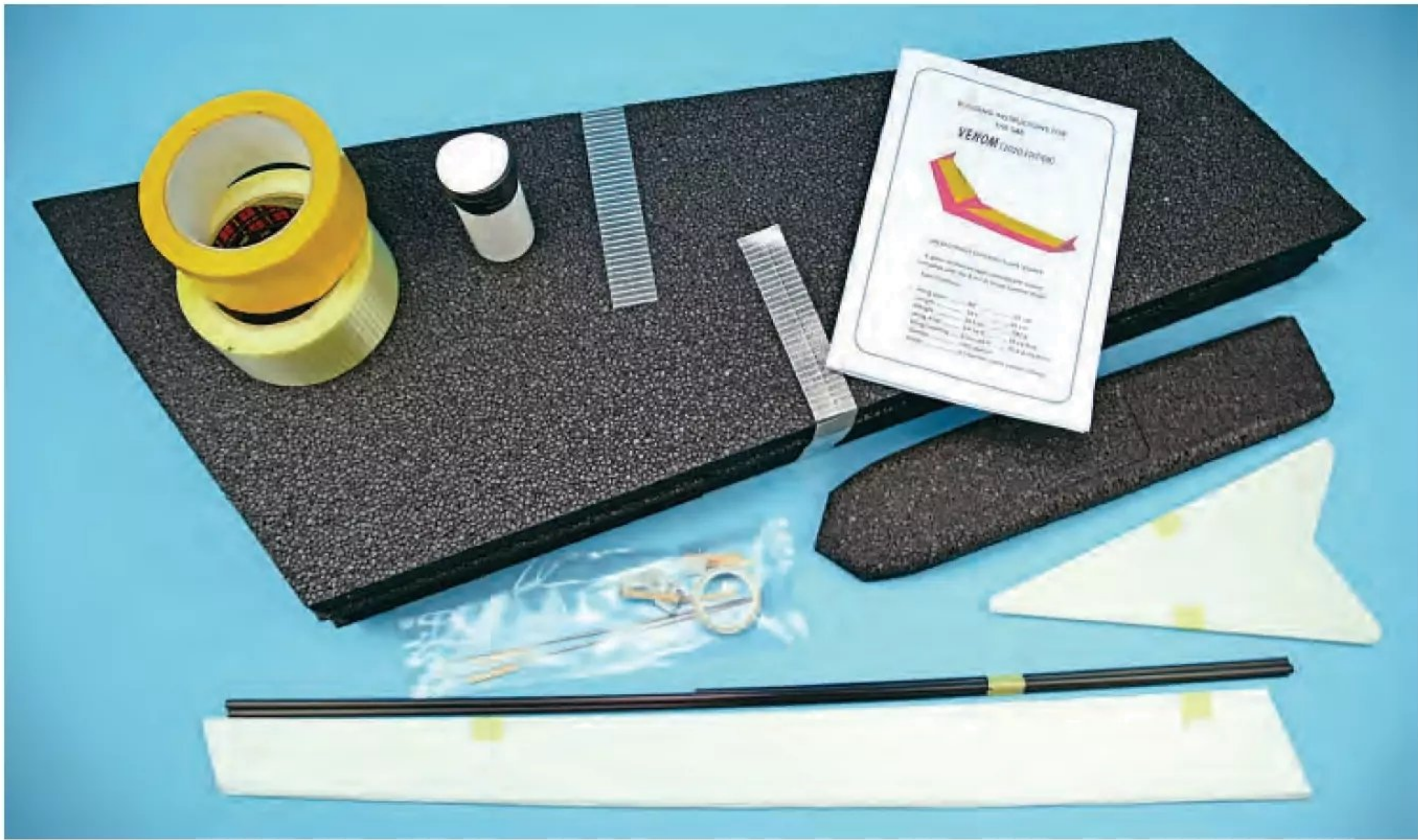
Left: Unboxed Venom waiting to be assembled. Again, not many parts but quality components with excellently cut cores. I believe a CNC hot wire machine is used to ensure accuracy.
