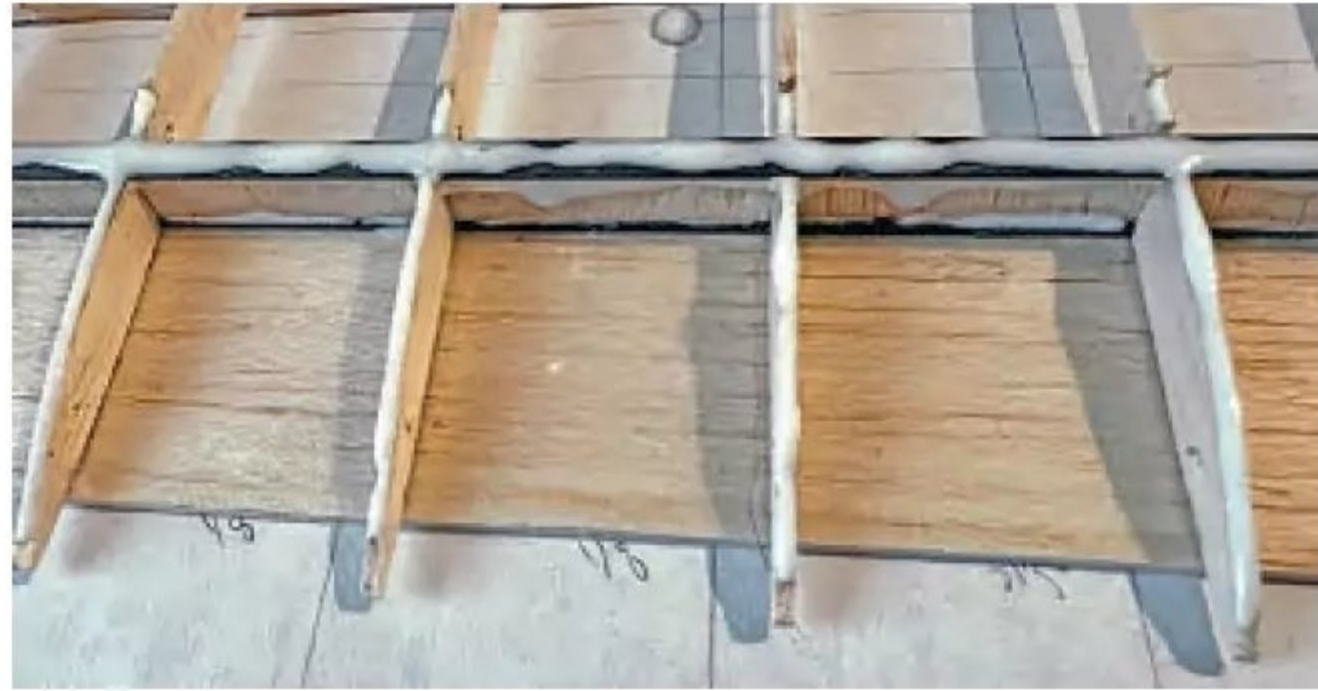
Wingspars are made from carbon fibre pultruded strips and use a full D-box leading edge, helping to provide good torsional stiffness.
