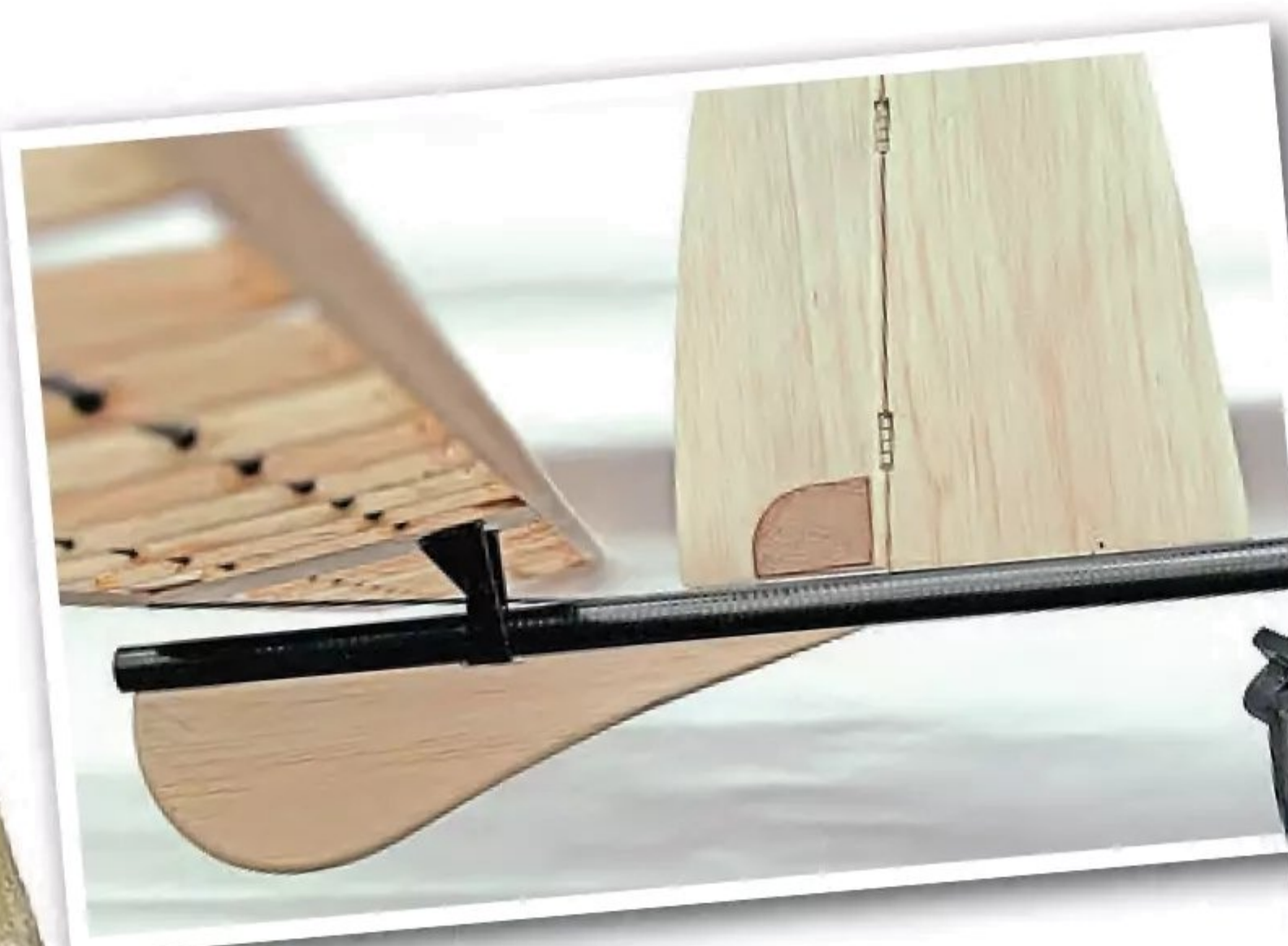
The 'all moving tail' mount is a carbon fibre assembly that slides onto the back of the circular tail boom.
