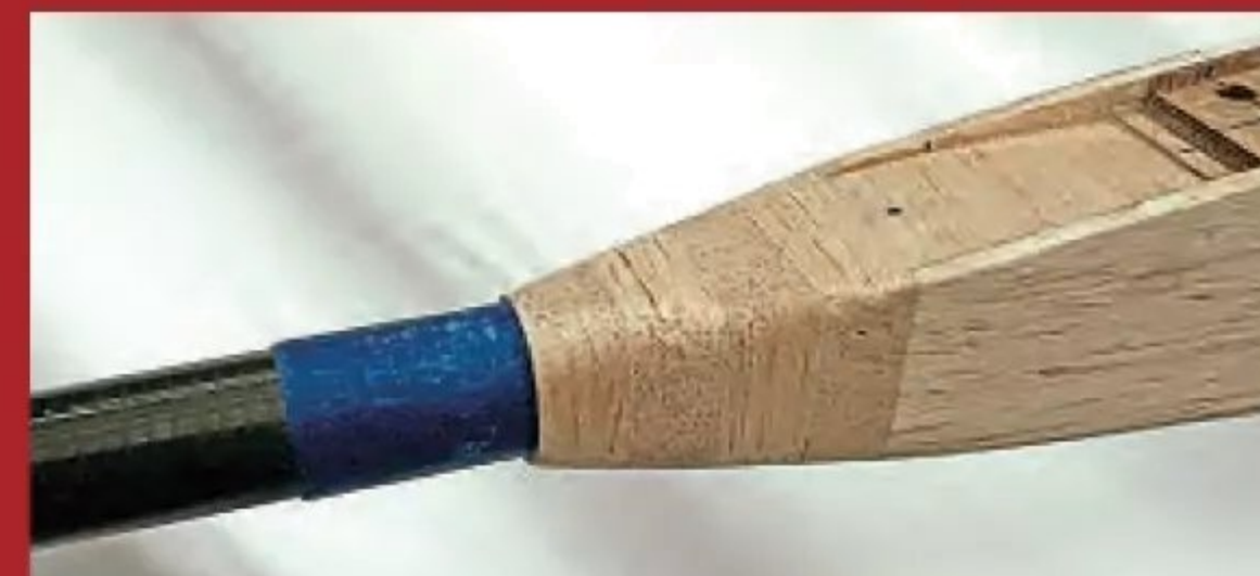
Fabricating the boom support from alternating squares of balsa.
