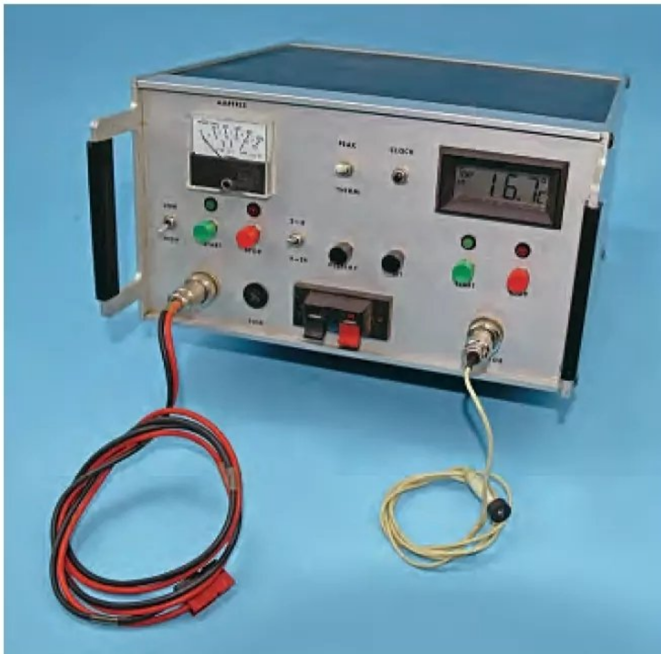
Above: This was my pride and joy, the kit-built Ampere Flyer NiCad charger. 2–24 cell capable, with peak or thermal cut off. Sold in the UK by Gordon Tarling, it was designed by members of the 1982 Benelux Electro Team.
