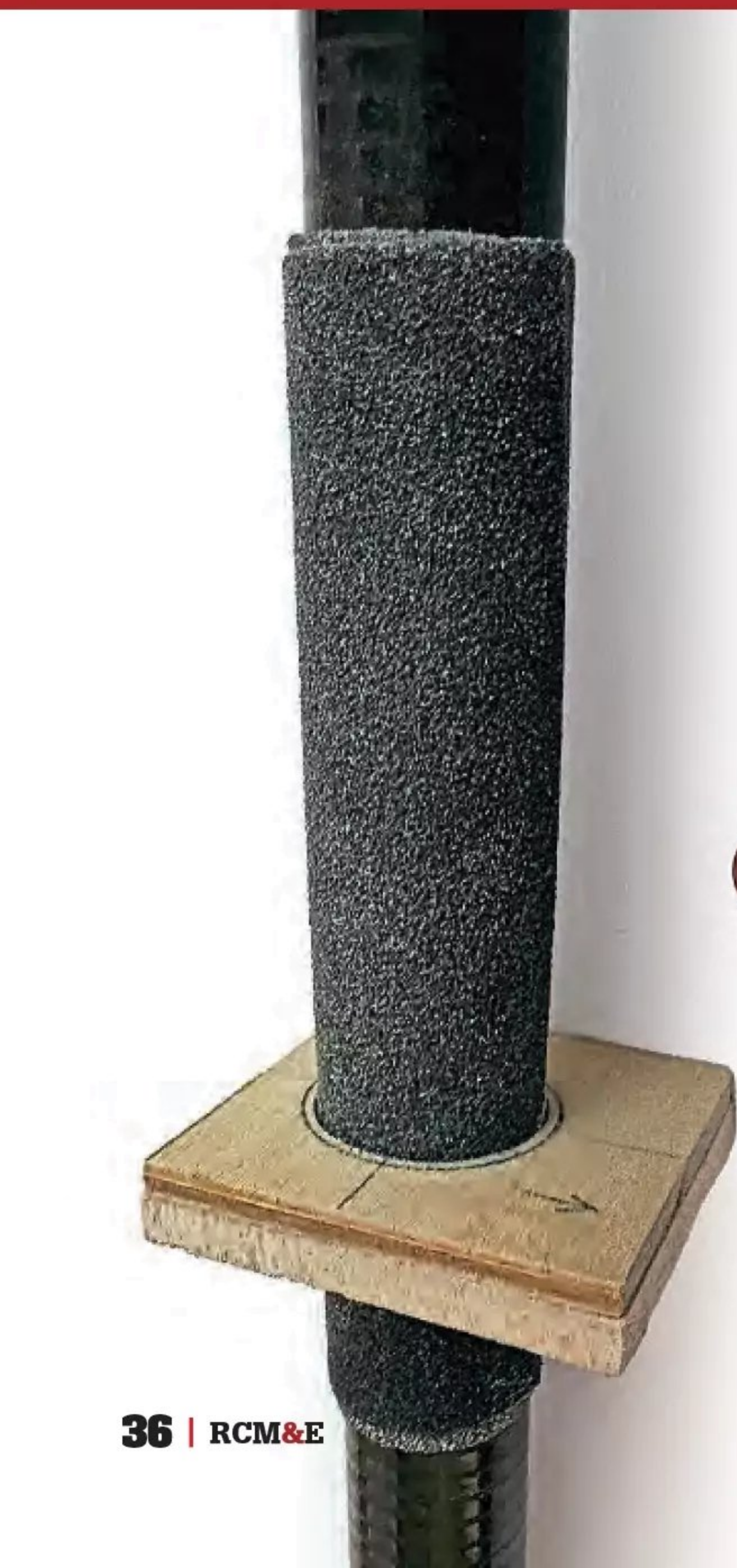
Left: Sizing the hole in a former using sandpaper wrapped around the carbon boom.
