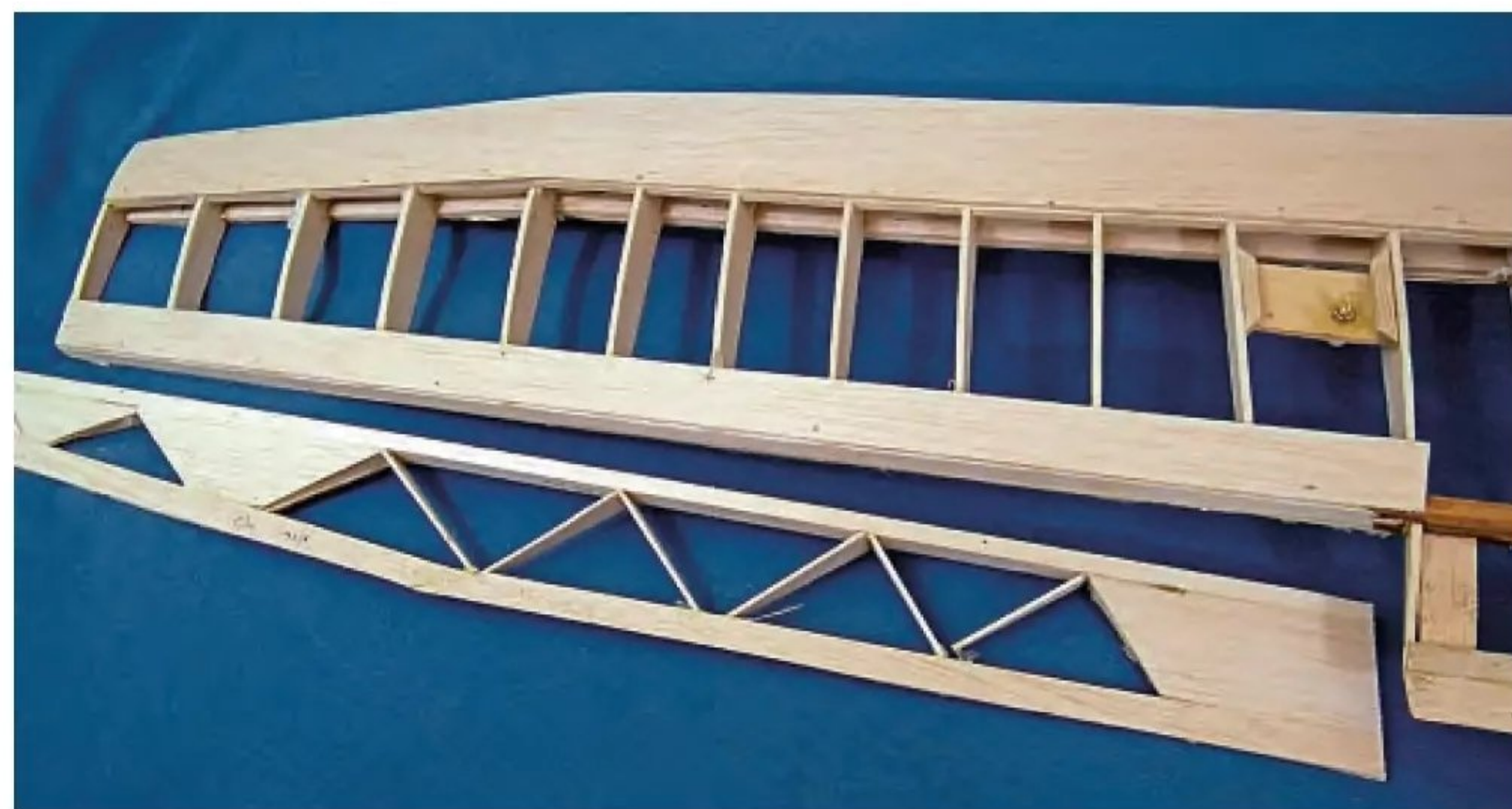
Aileron construction shown next to the wing and getting ready for hinging.
