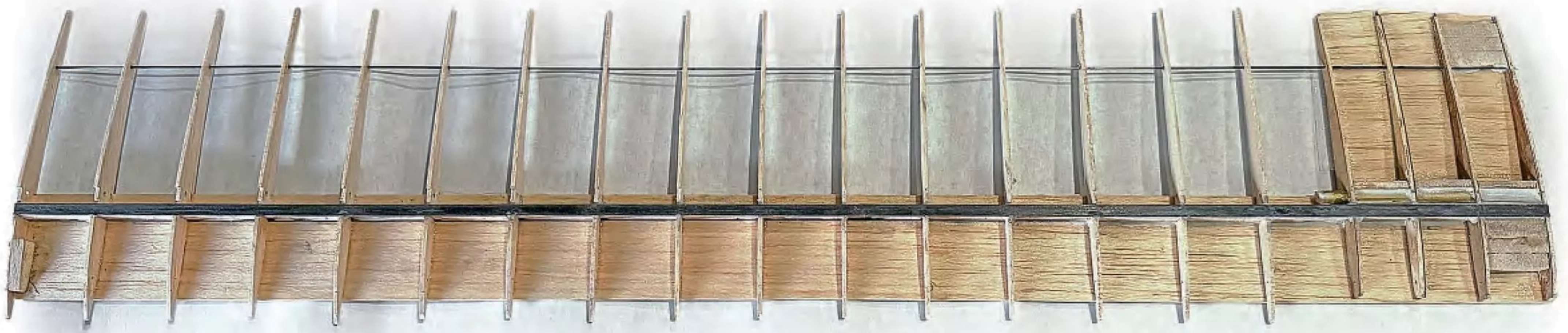
Wingspars are made from carbon fibre pultruded strips and use a full D-box leading edge, helping to provide good torsional stiffness.
