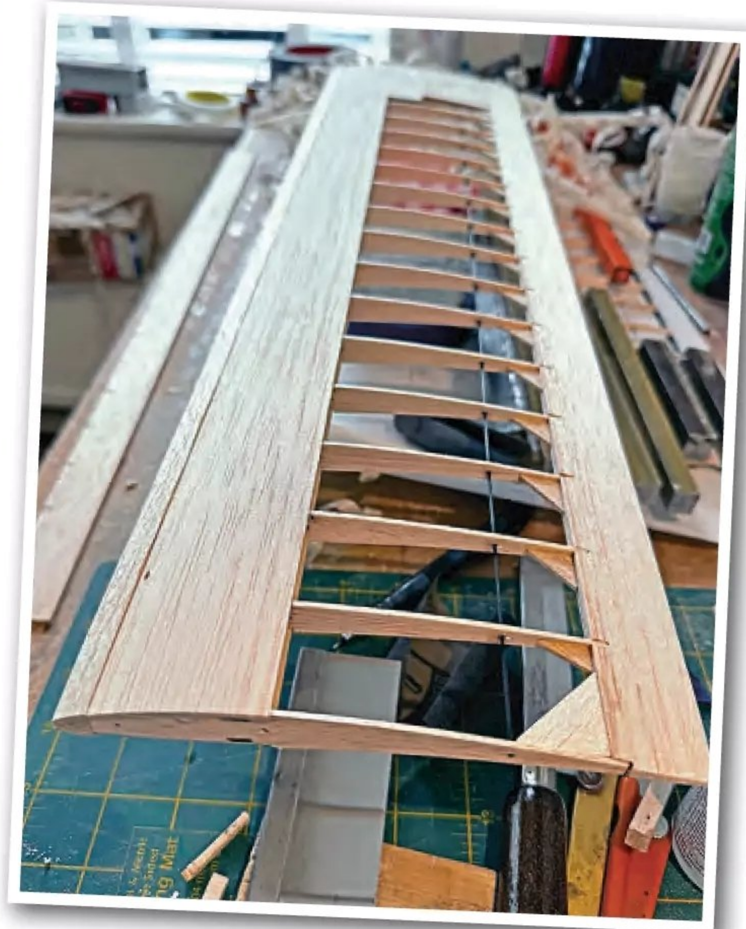
Wingspars are made from carbon fibre pultruded strips and use a full D-box leading edge, helping to provide good torsional stiffness.
