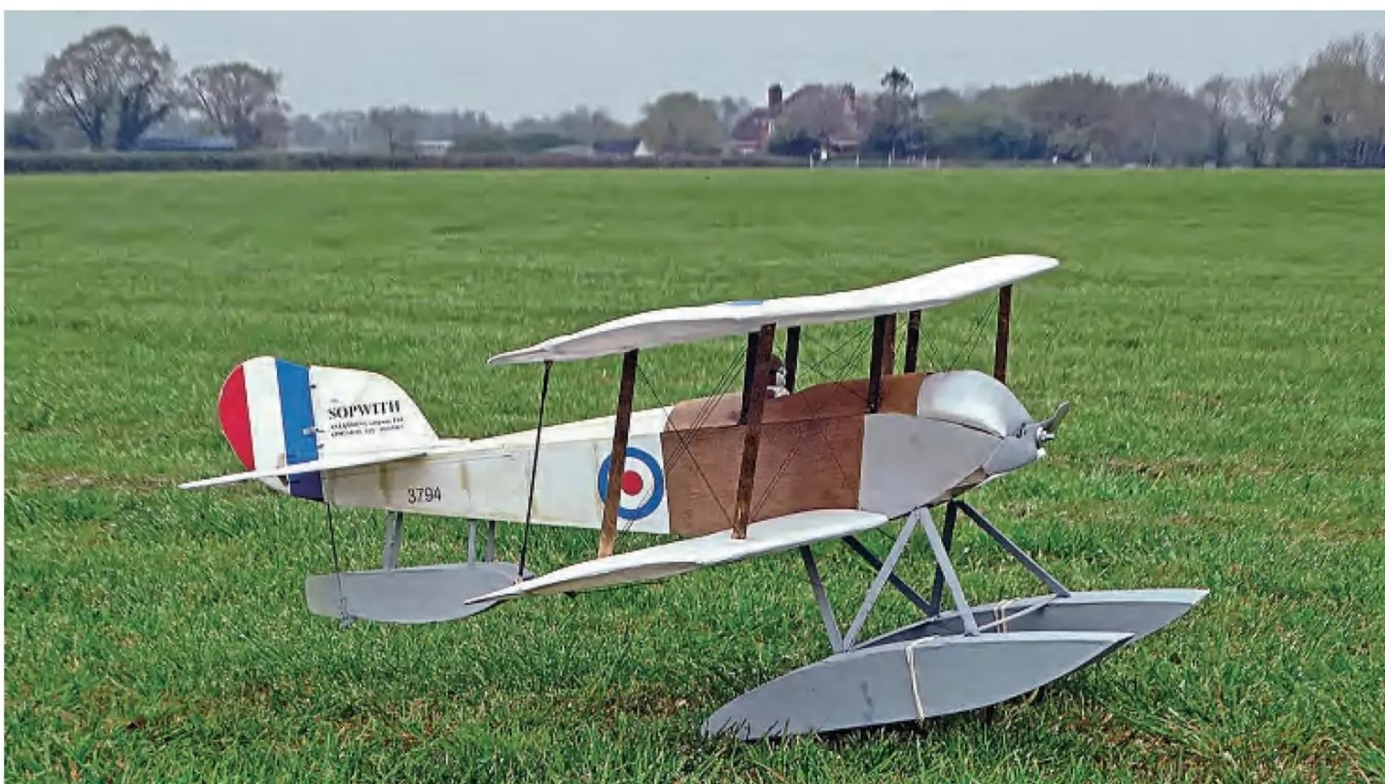
A Sopwith Schneider from the author's plan. Most floatplanes can be flown off grass with some discreet wheels added just before the CG.
