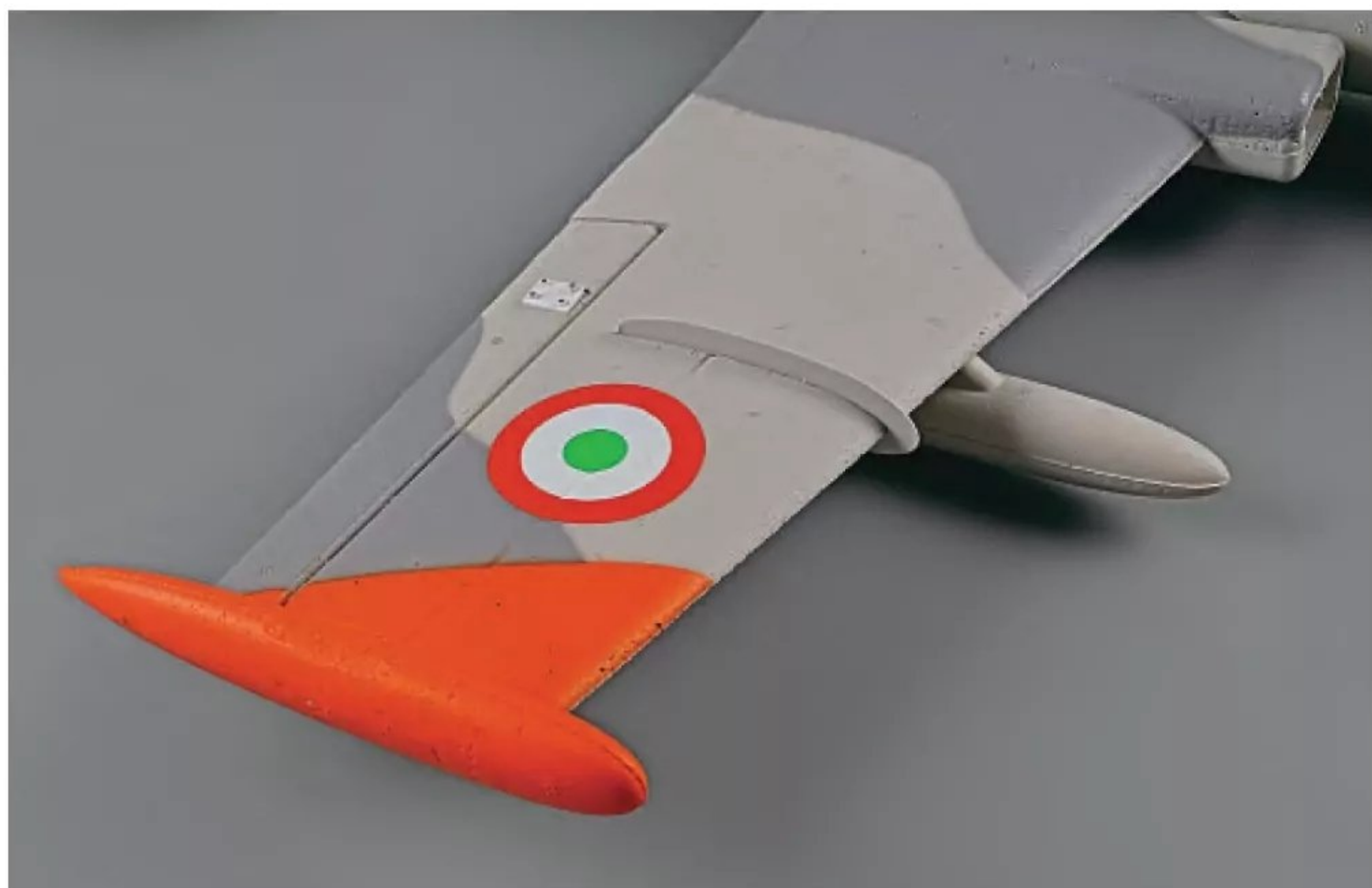
Wing tip and drop tanks are meant to be glued on early in construction but I left mine off until near the end to save them from hangar rash.
