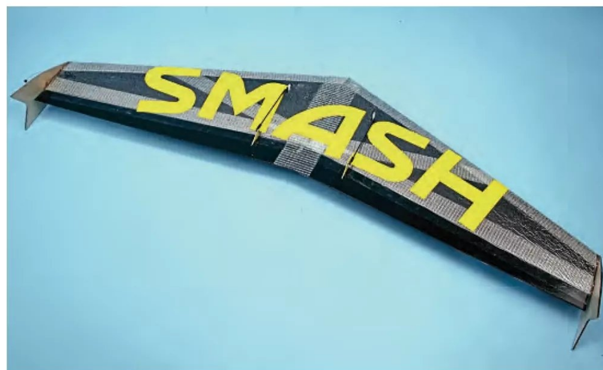
Finished and ready to go. You can see the cross weave tape (as used on the Wildthing) under the Doculam covering. Again, a bespoke decal was used to jazz it up.
