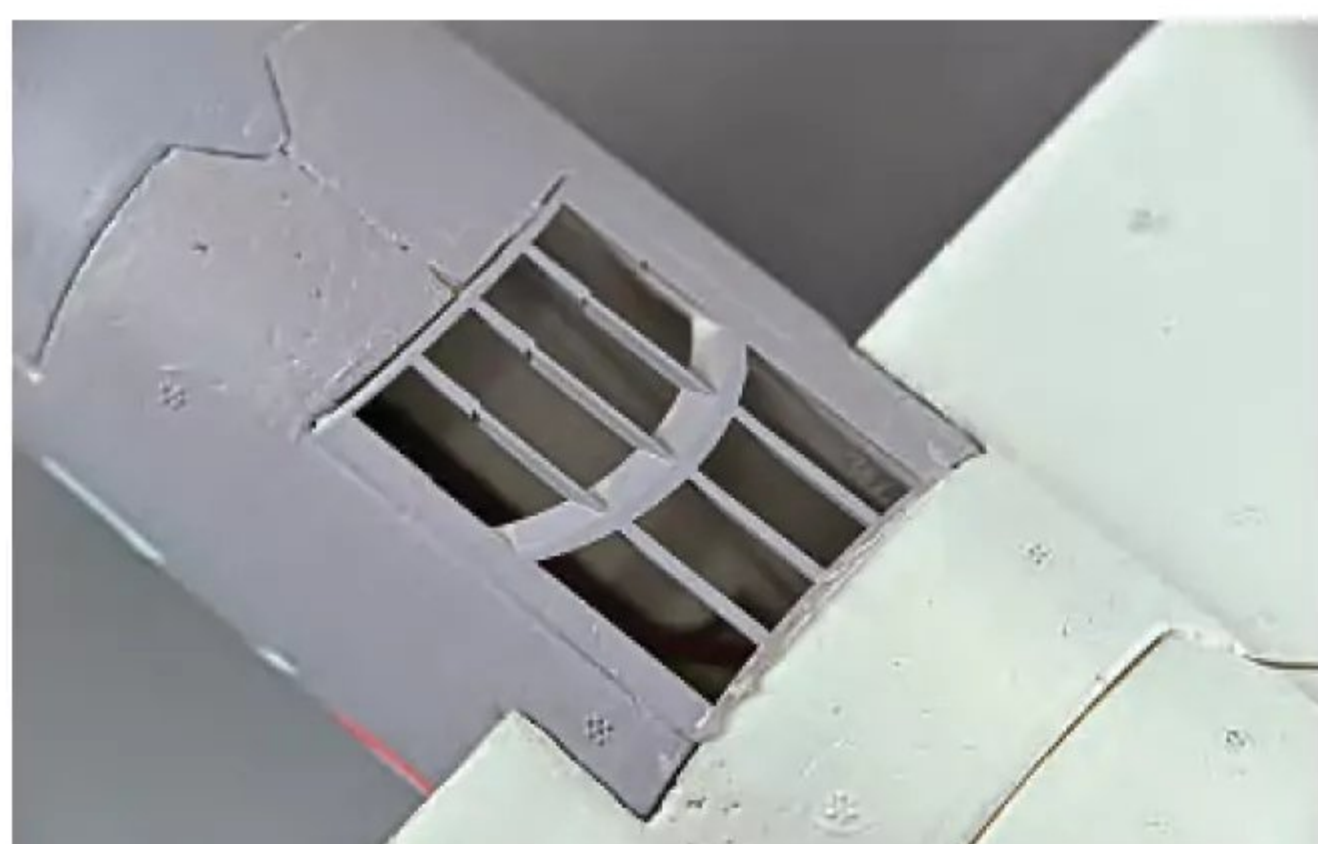
A generous air inlet is fitted to the underside just before the fan unit.
