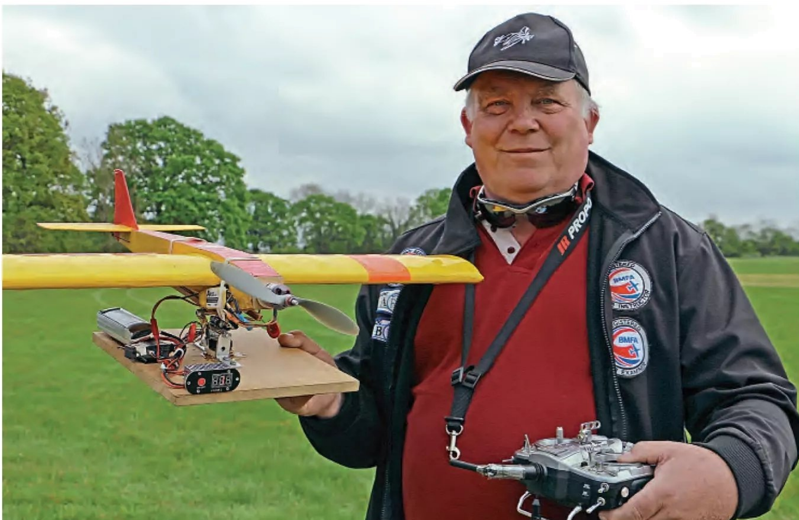
Bert Baker is one of the many experienced instructors whose services Bootcamp calls upon. Bert developed this neat training aid that replicates a model's response to any given stick input. Simple, but cunning.
