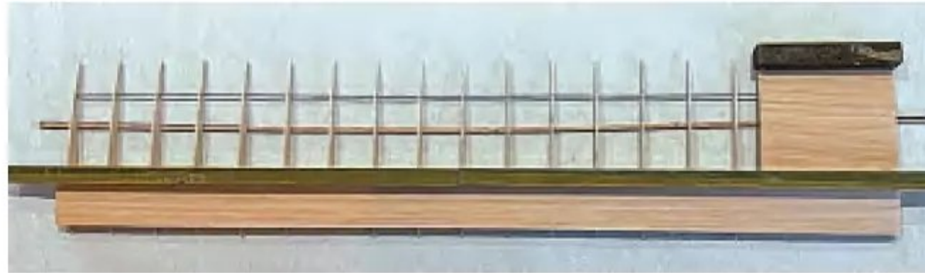
Left: Webs and top sheeting were glued on using thin epoxy resin mixed with a small amount of micro balloon filler.
