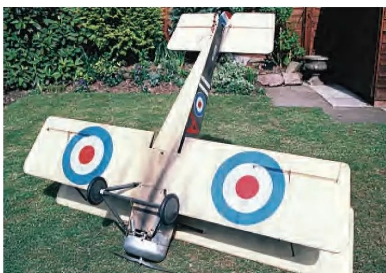
Flair Scouts were widely copied. Dudley says, 'The number of times that someone had had an 'accident' and needed a cowl, undercarriage set and cabane struts were legion.' Here's an underside view of Bob Shuttleworth's Puppeteer showing some of the difficult to copy parts.
