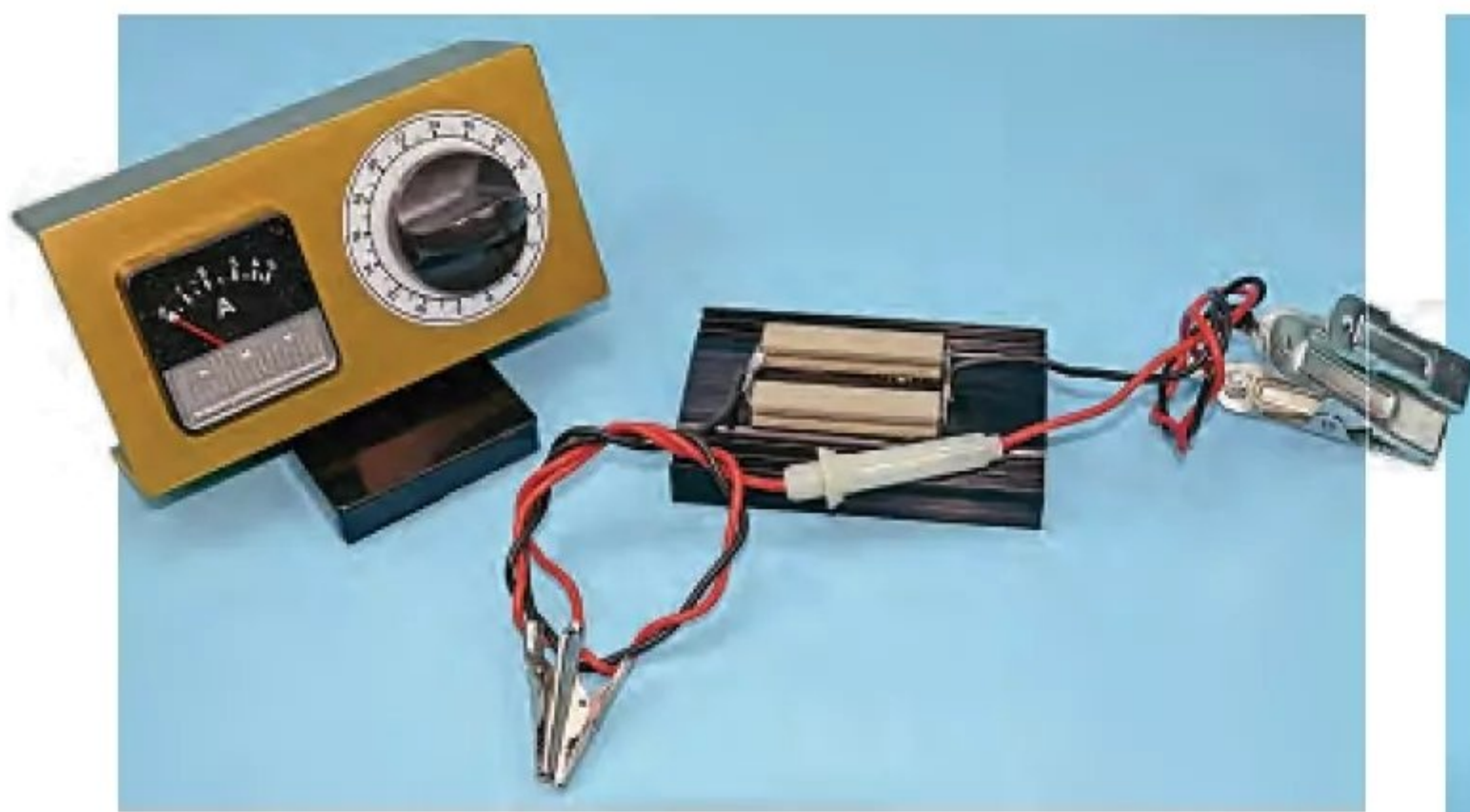
Early NiCad chargers were simply a bunch of resistors fixed to a heat sink. Slightly more sophisticated ones used a clockwork timer. Both could be dangerous in the wrong hands.
