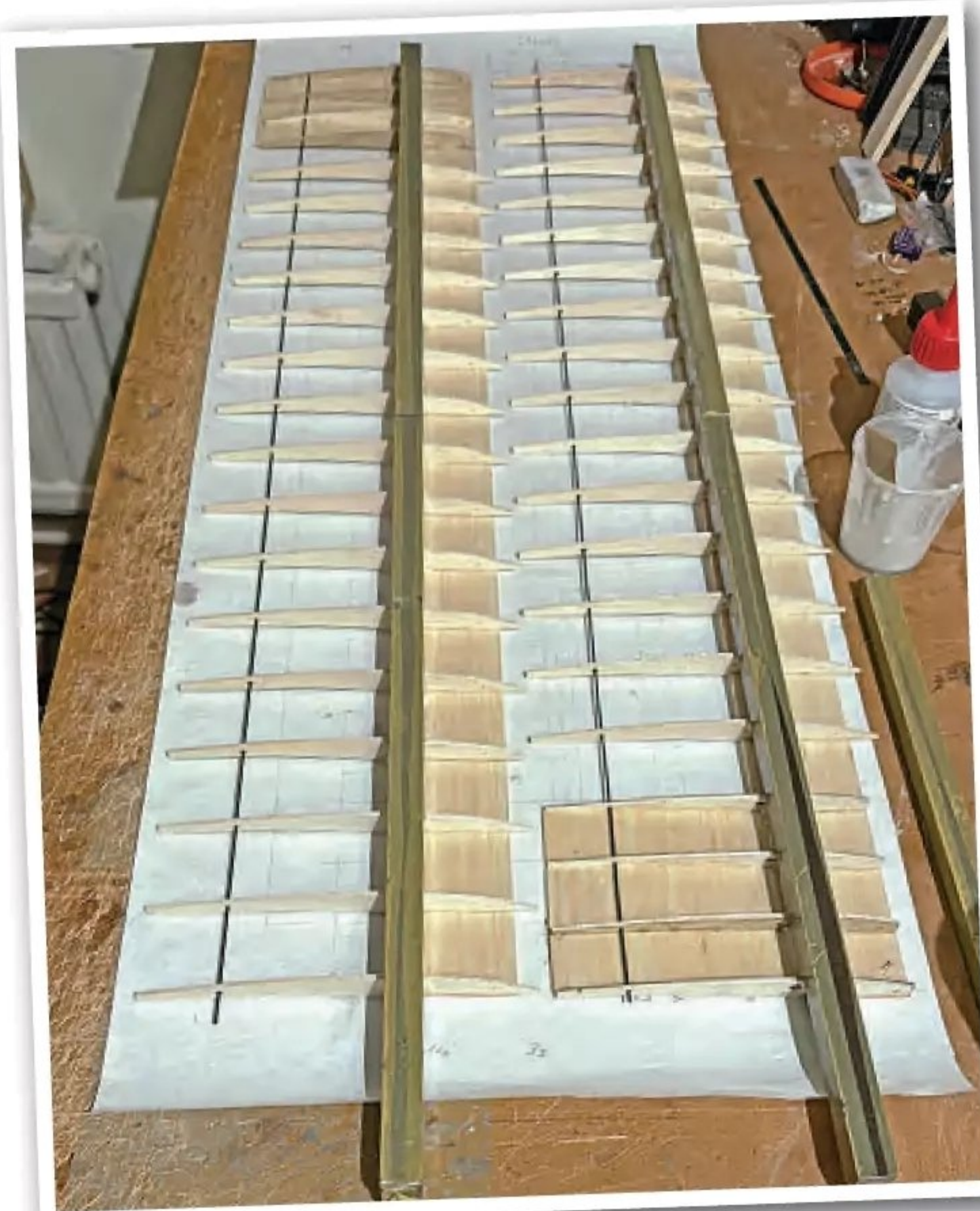
Inner panel construction started by gluing carbon spars to the bottom sheeting, followed by the ribs.
