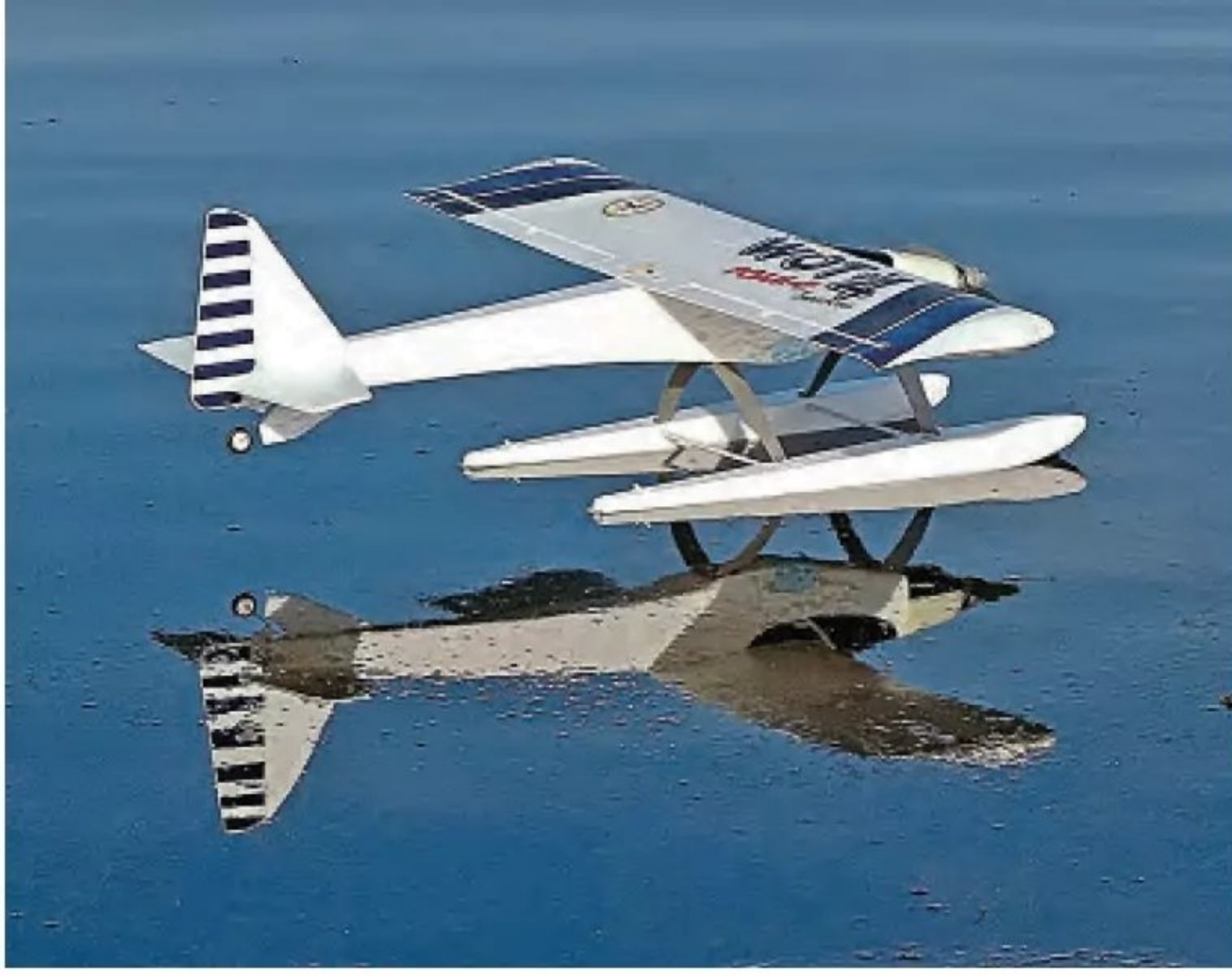
The WOT4 makes an excellent sport model on floats but needs an additional alloy U/C and reinforcement for the rear mount. The floats are from an ST Models Beaver.
