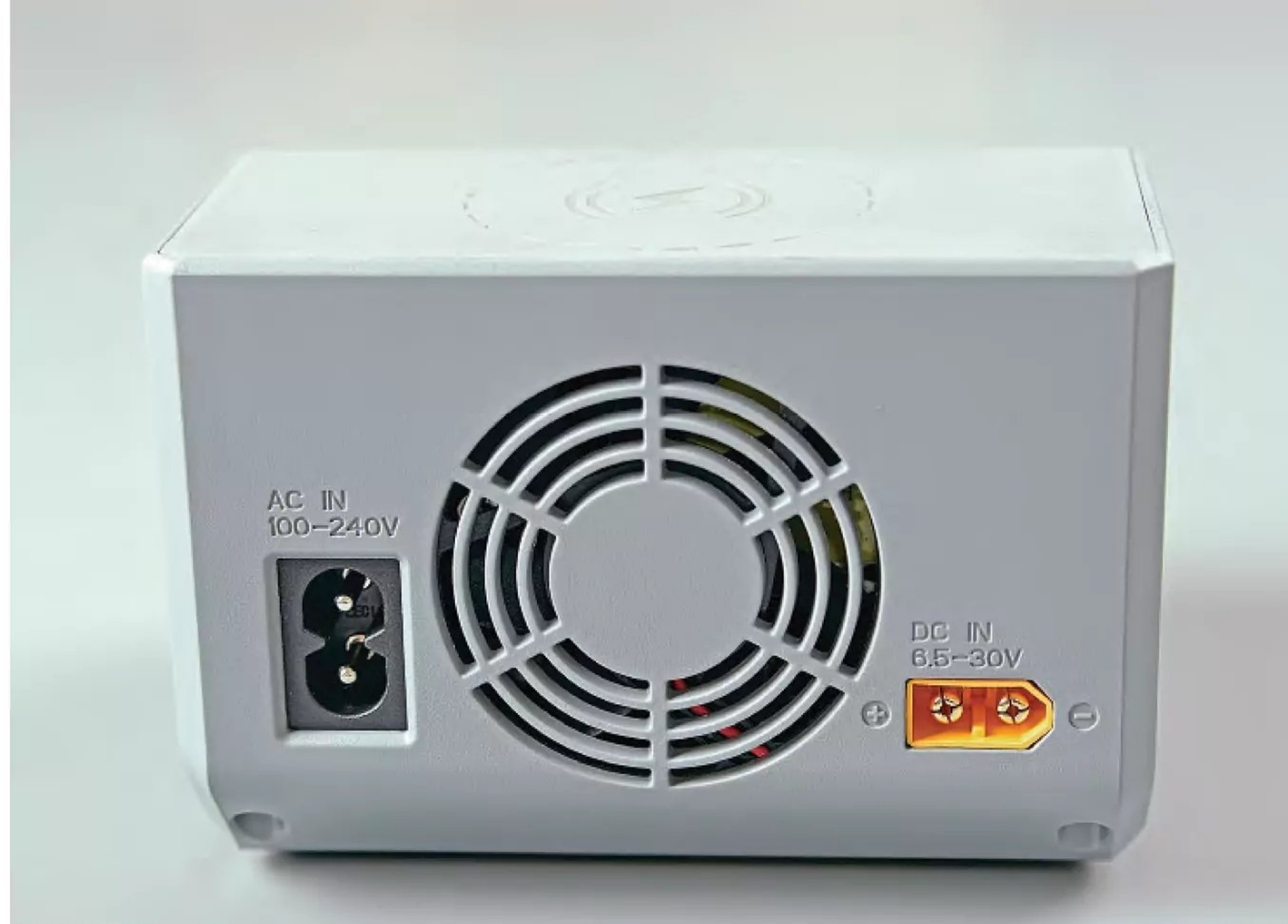
Back panel showing the AC and DC inputs as well as the efficient cooling fan.
