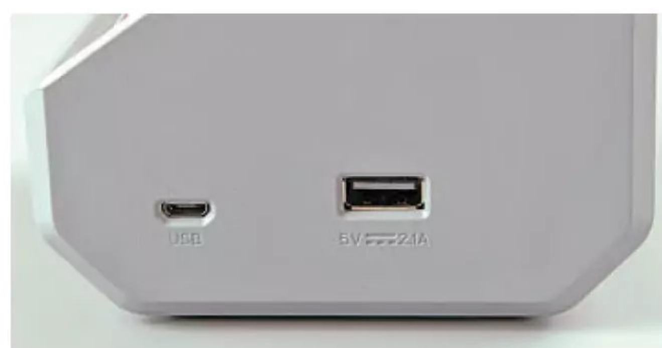
Side panel showing the two USB ports. The small one is used for updates whilst the larger one provides a conventional USB output.
