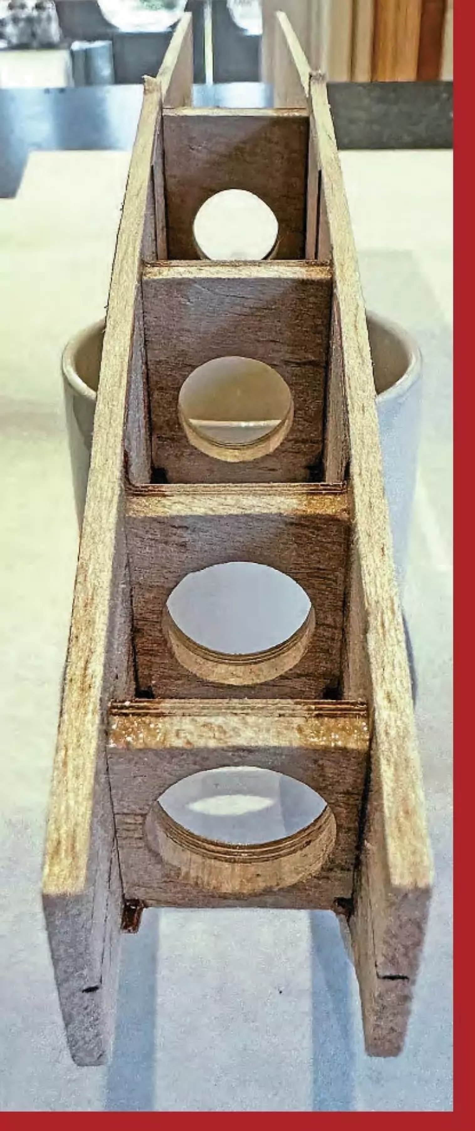
Left: Holes in the ply/balsa sandwich formers were cut so that the boom would slide into the fuselage and be well aligned down its length.
