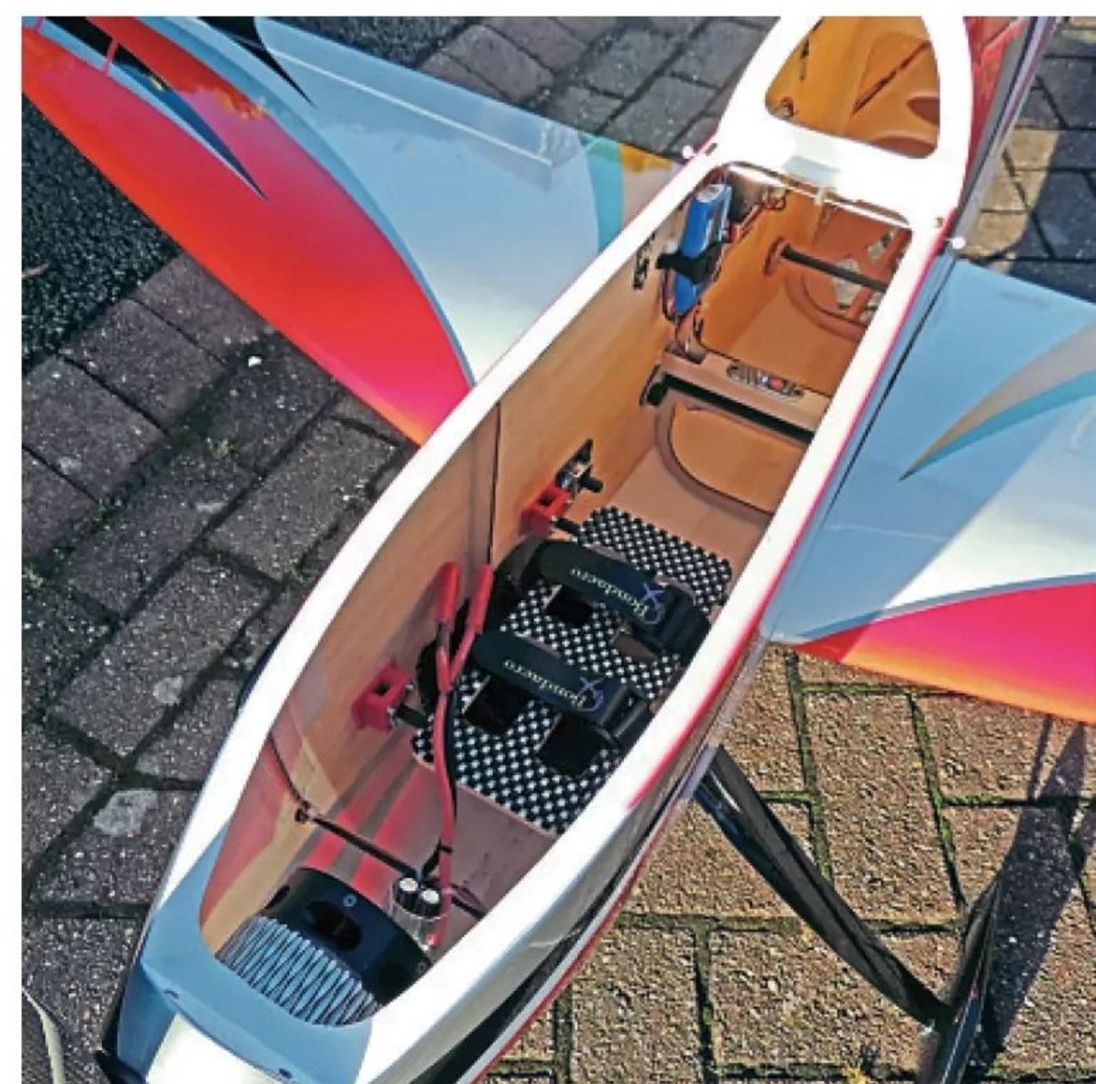
Anthem radio installation.
