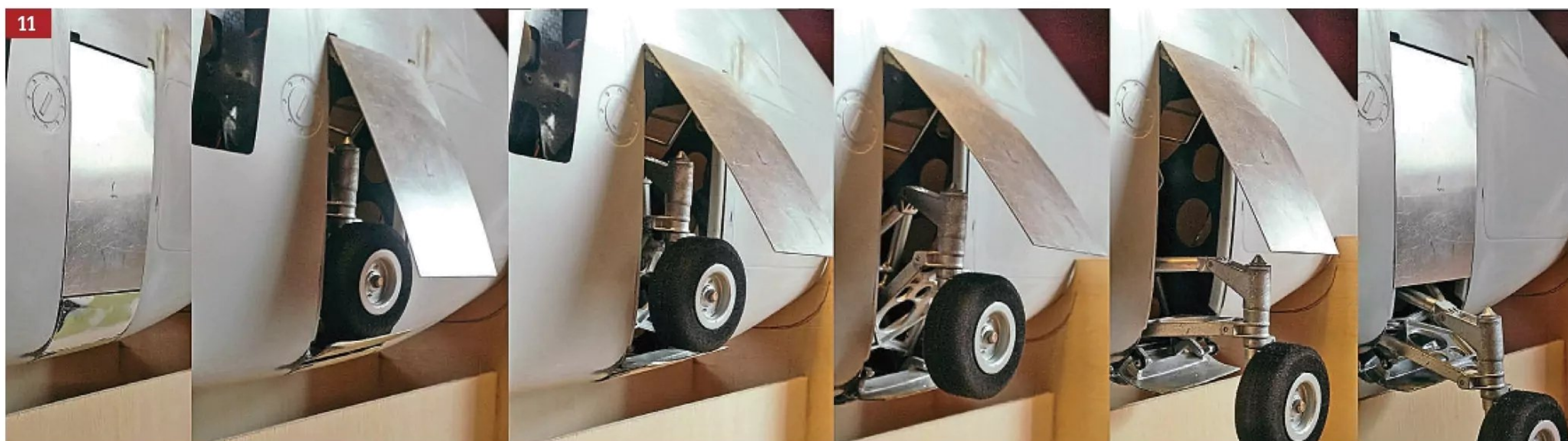
11/12: Upper and lower bay door opening sequences.
