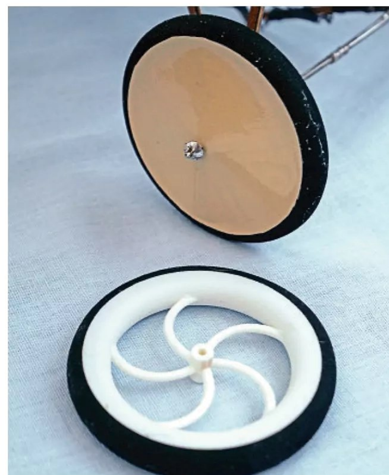
An ‘indoor’ lightweight 50 mm dia. wheel has film covered thin card discs added to emulate ‘Golden Age’ wheels. Simple and cheap.
