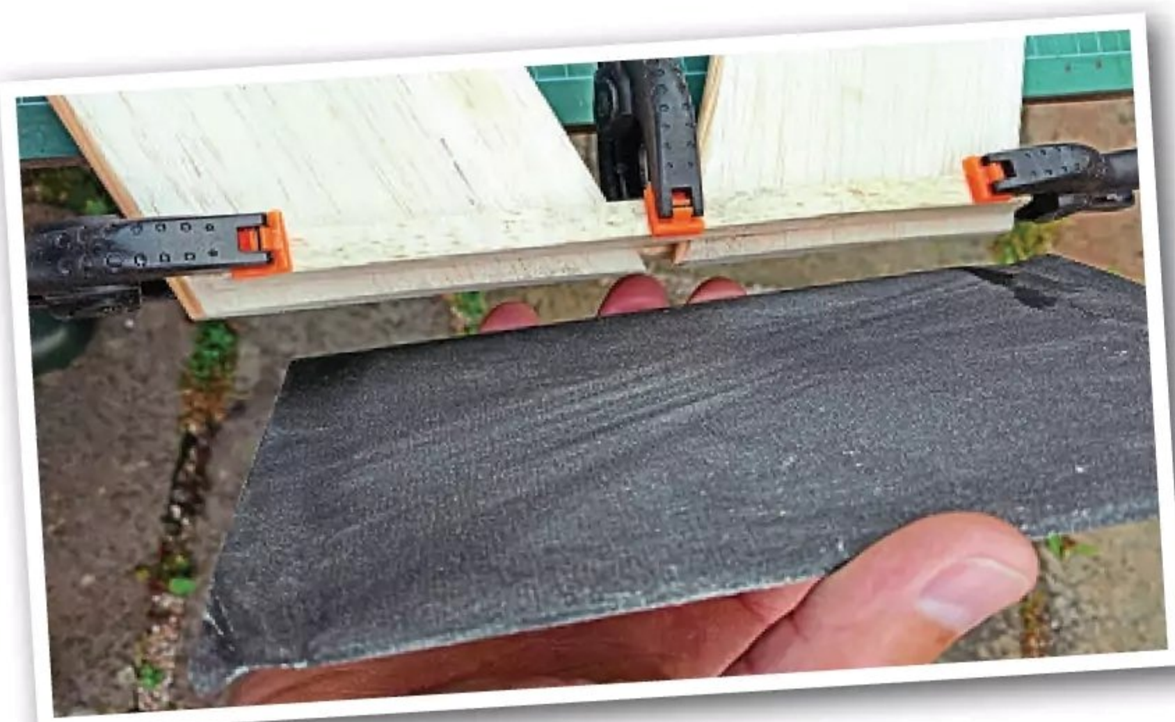
Above: Gently clamp the front and rear wing tips in alignment. Sand straight and level before fitting the carbon joiner tubes.
