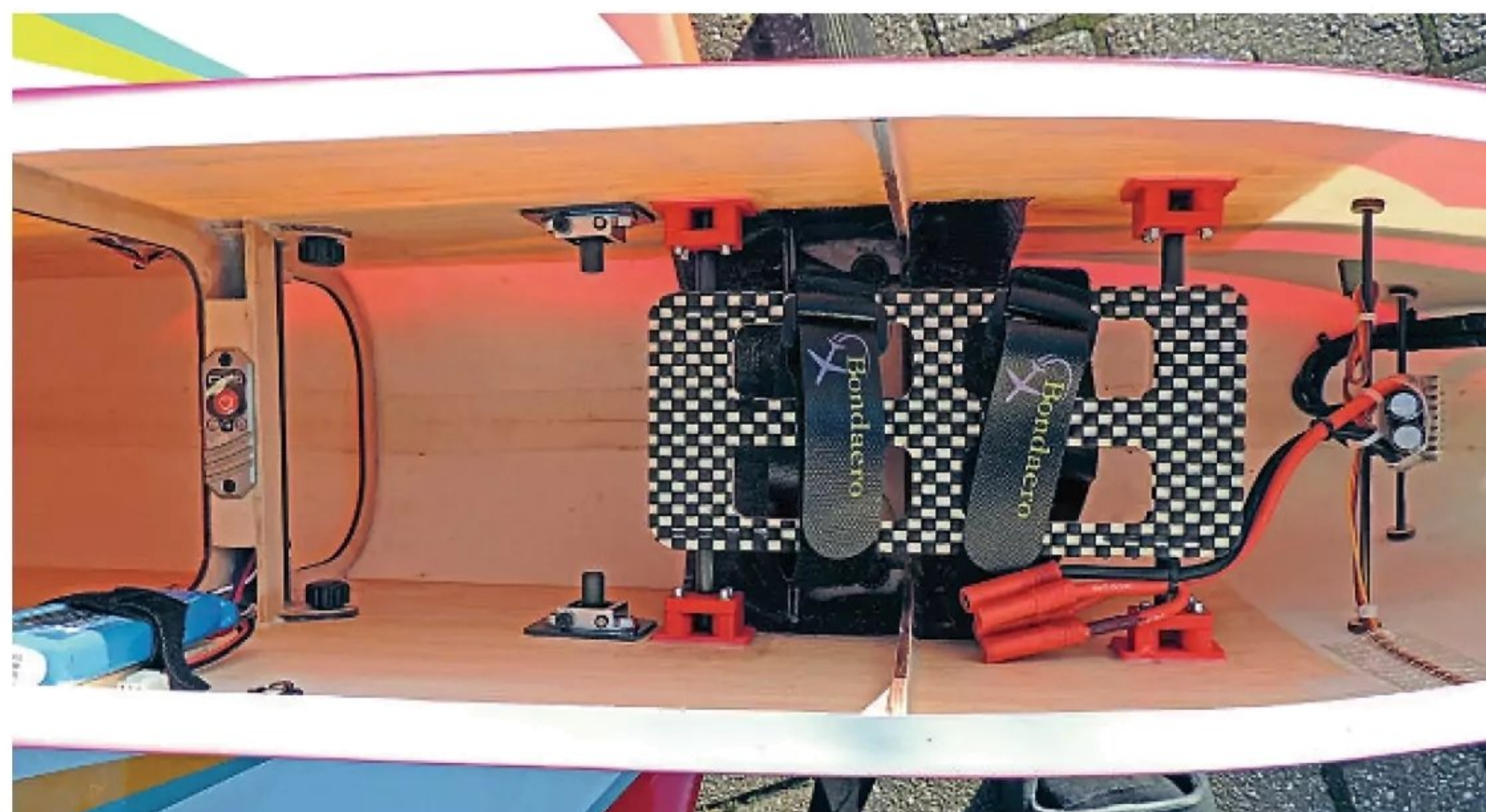
Left: Anthem nose showing R220 and D3 ESC locations.
