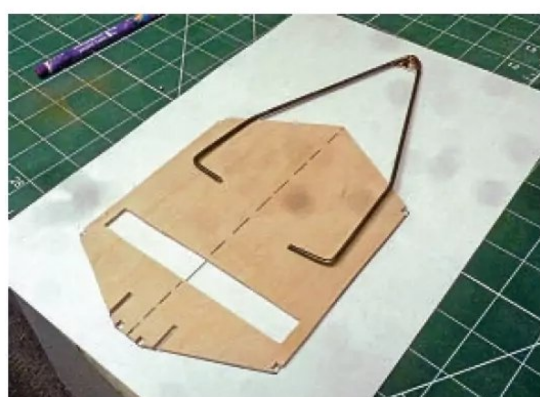
Setting up the front wing strut for the T31 with direct reference to the drawing.
