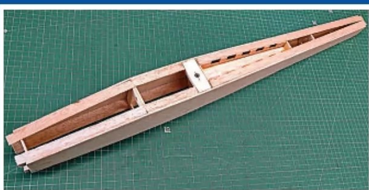
Fuselage stage 1 completed, ready for trial fitting the wings. F1 is glued in with zero side thrust and down thrust.
