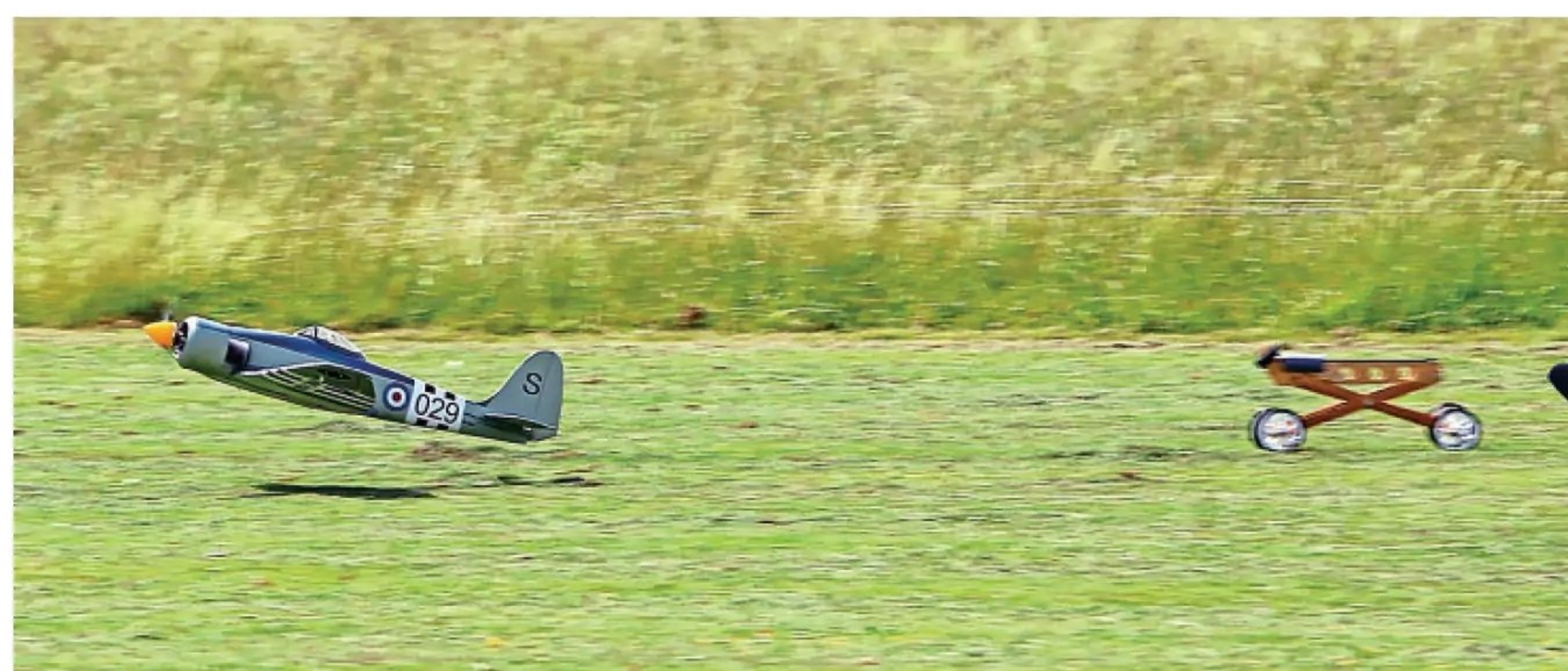
Off too soon! This contra-coax Sea Fury lifted off the dolly before proper flying speed was reached but very fortunately it survived.
