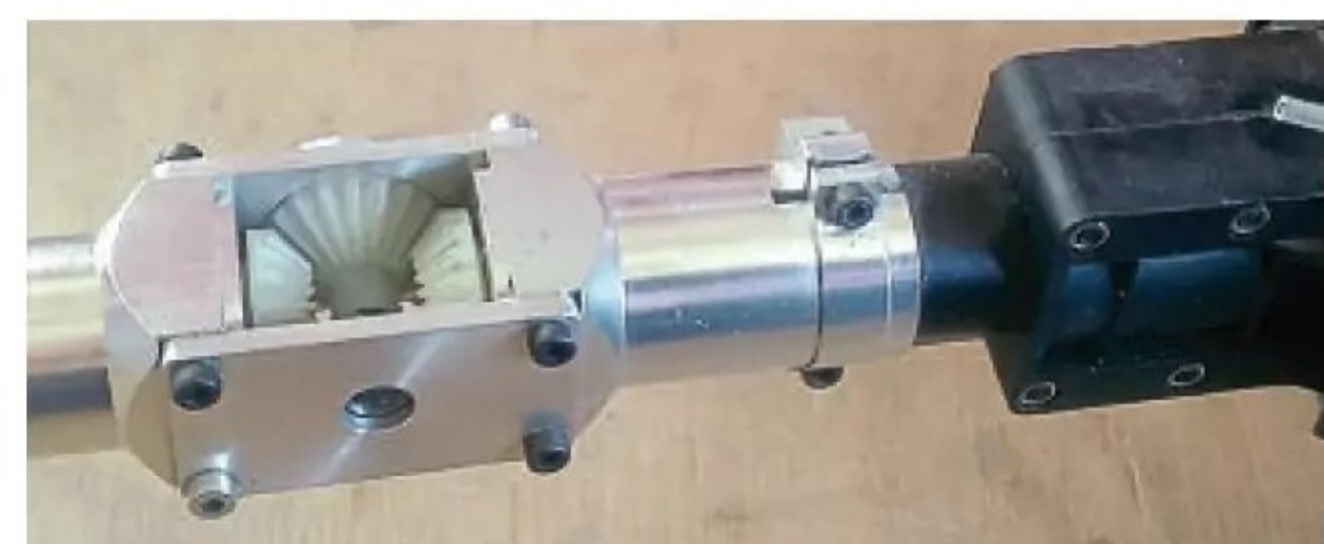
Tail rotor rotation was reversed using a homemade gearbox fitted with bevel gears.
