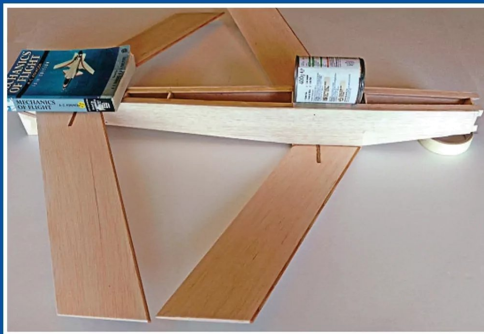
With the front wings already bolted in position and the fuselage inverted, fine tune the position of the rear wings before drilling for the wing bolt.
