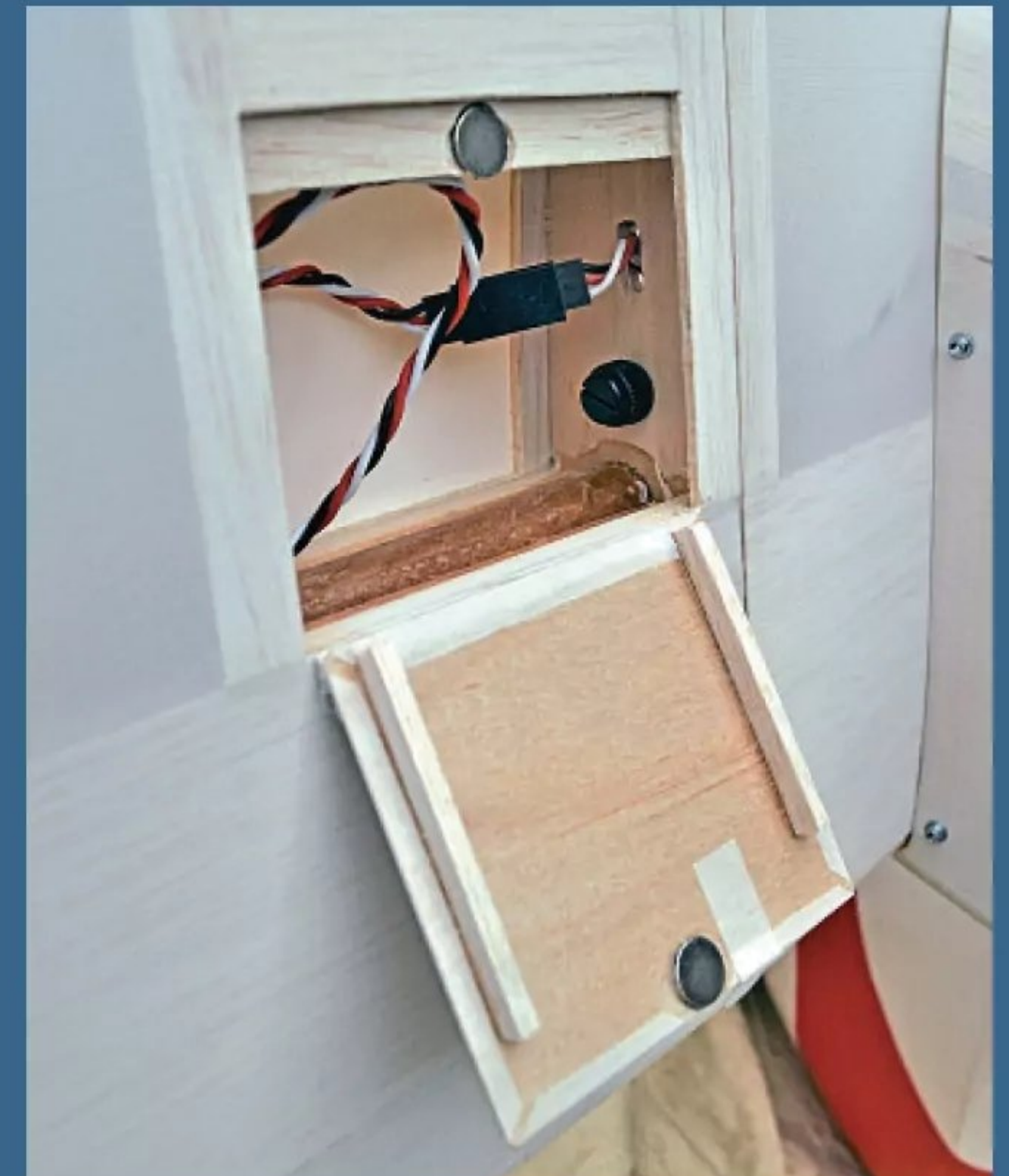
With the hatch open the Buzzard's wing bolt is easy to access, while the magnets and Solartex hinge ensure that the hatch doesn't blow open in flight.
