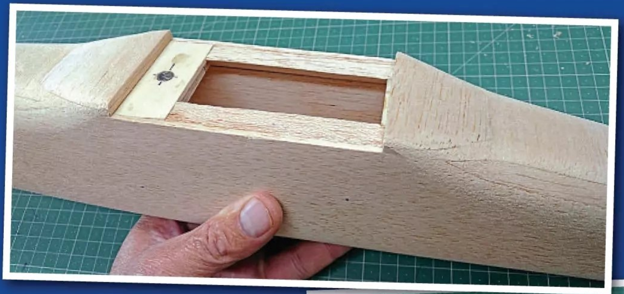
Above: Carve, plane and sand the fuselage to a curvaceous shape. Be brave and take full advantage of those corner triangular strips.
