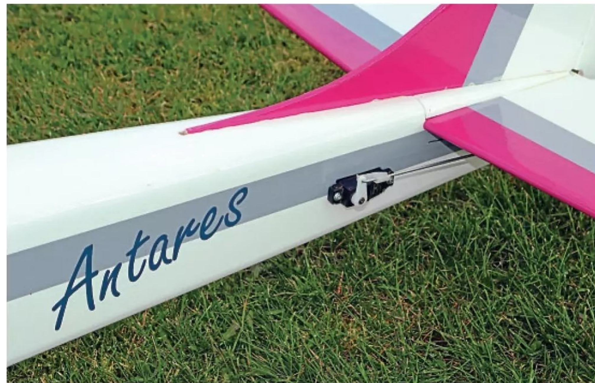
Exposed servos tend to garner detractors but are supremely practical in a non-scale model.
