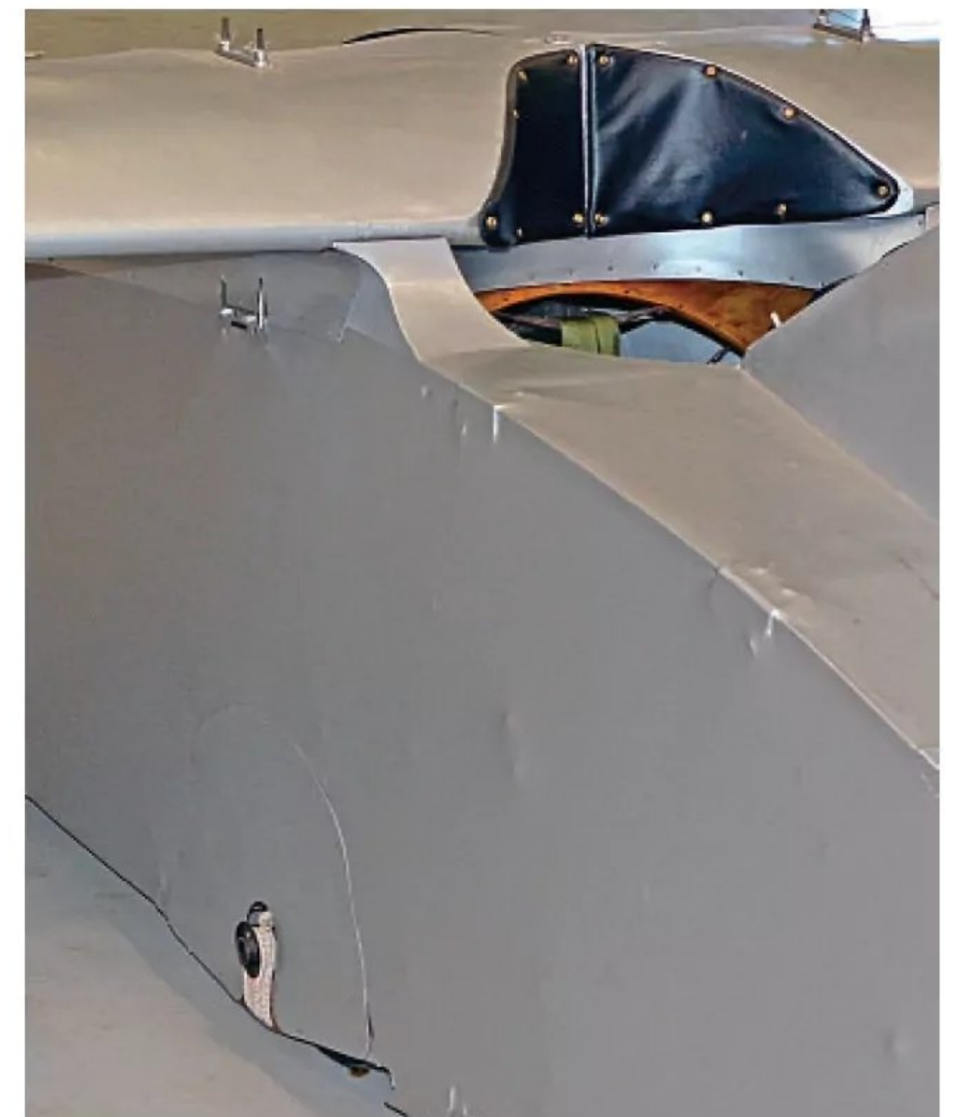
The 1923 EE 'Wren' at the Shuttleworth Collection shows its 'axle-in-slot' and bungee cord suspension.
