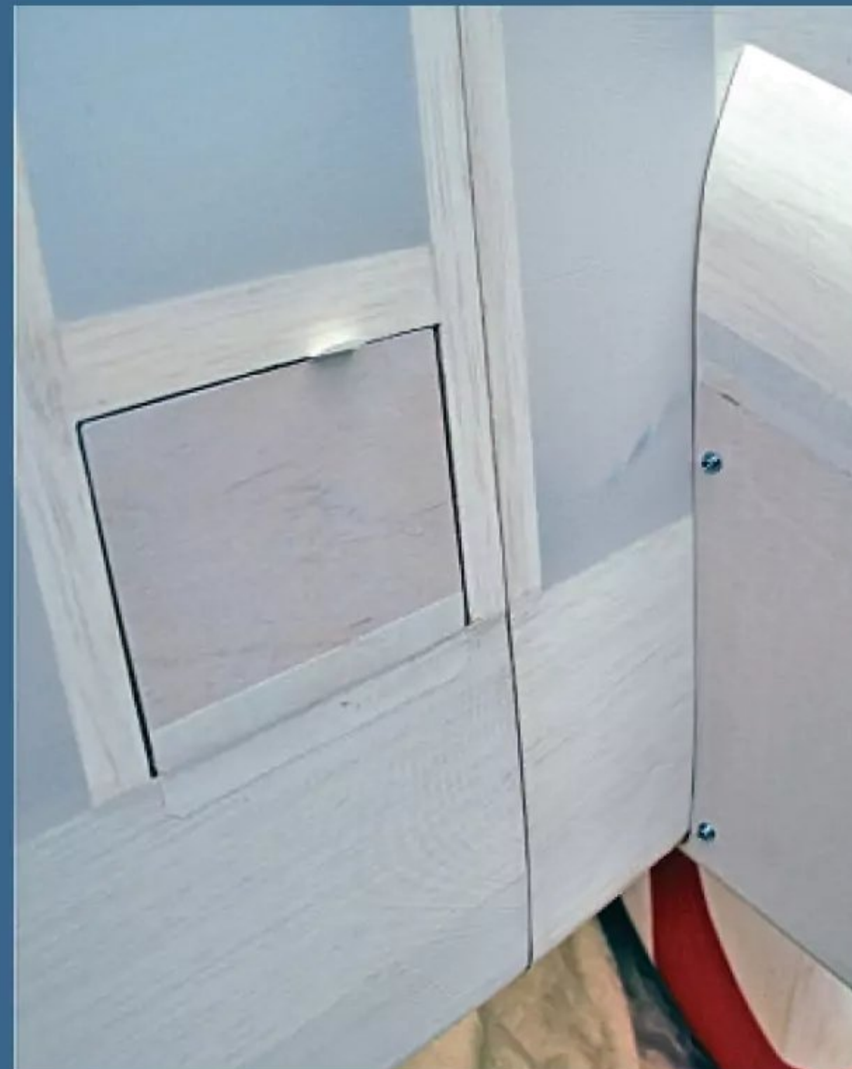
Luton Buzzard under wing hatch with its Solartex hinge (bottom) and pull tag (top). It's a simple but effective way of disguising wing bolt access.
