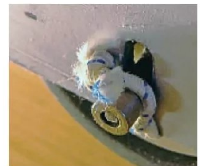
The 1923 EE 'Wren' at the Shuttleworth Collection shows its 'axle-in-slot' and bungee cord suspension.
