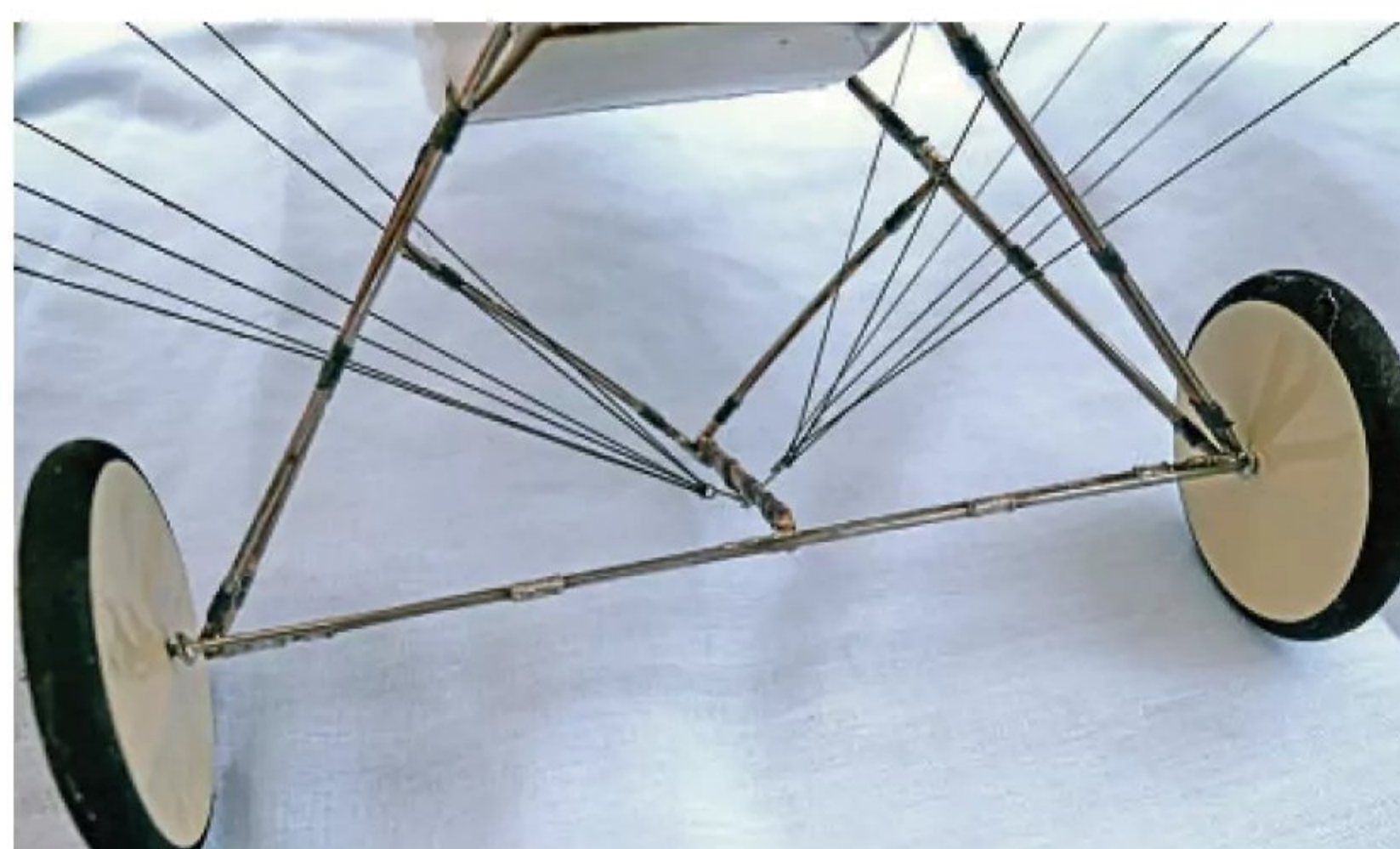
Left: The little Caudron 11 used to have a solid axle that imparted fuselage damage in less than perfect landings.
