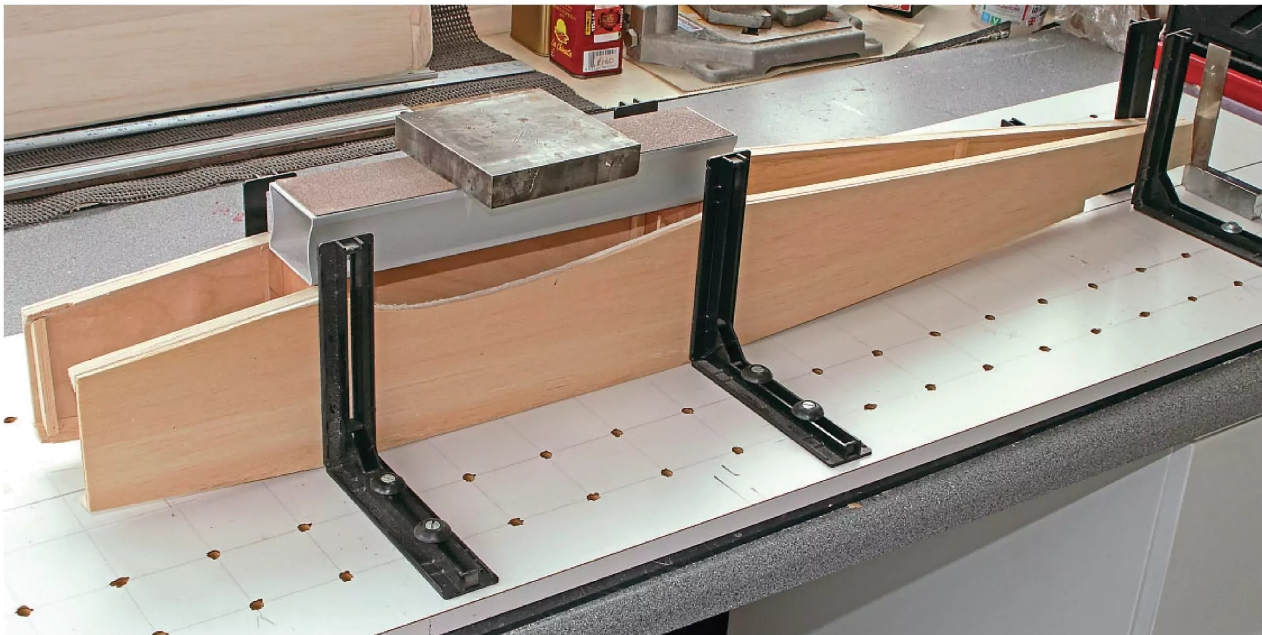
Fuselage sides are inverted and joined together within my SLEC based jig. The rear end is centred to avoid the dreaded banana syndrome.
