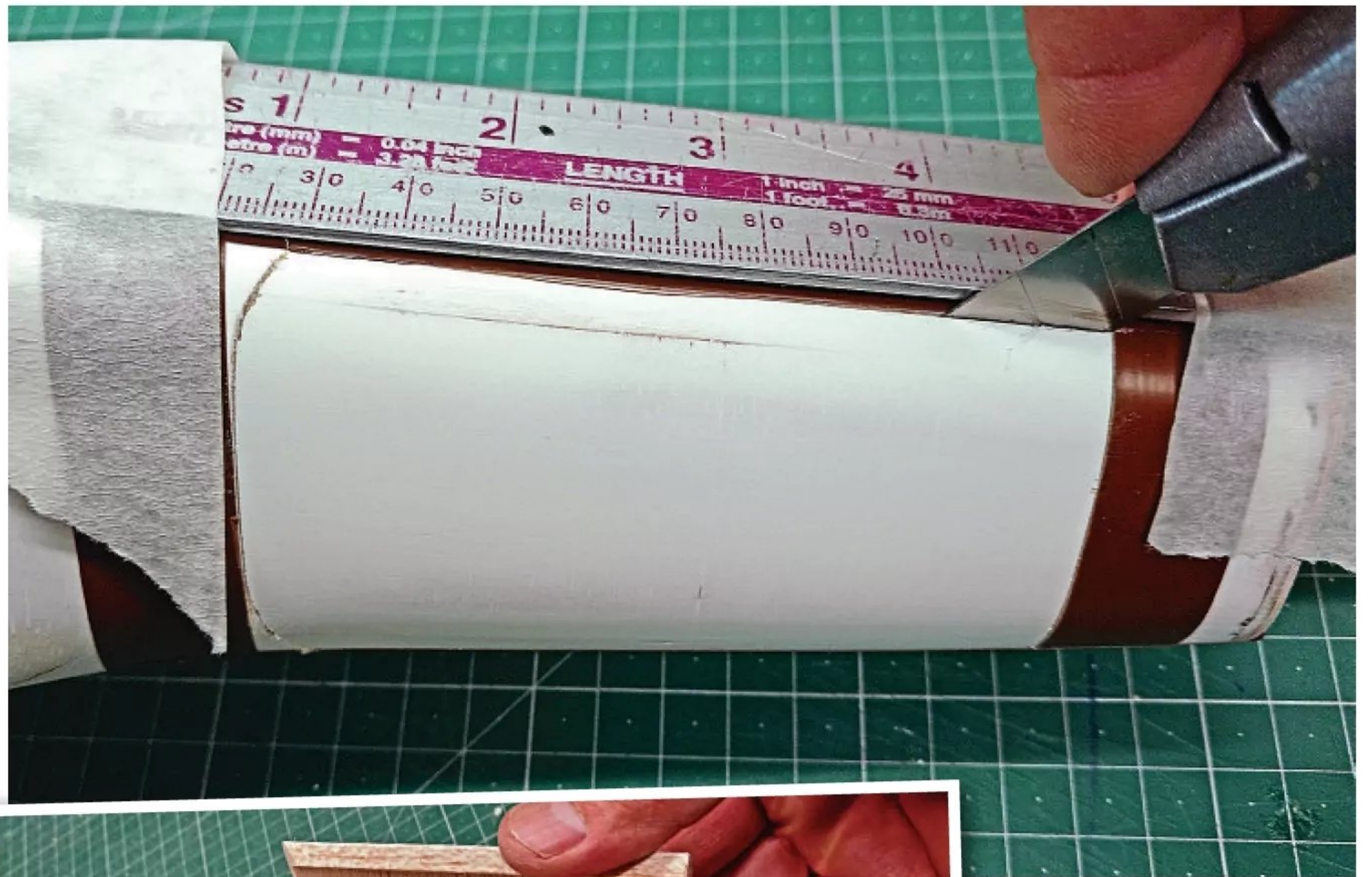
Above: Cut the ends of the hatch at an angle using a razor saw, then cut the hatch sides at an angle using a knife. This creates a bevelled seating.
