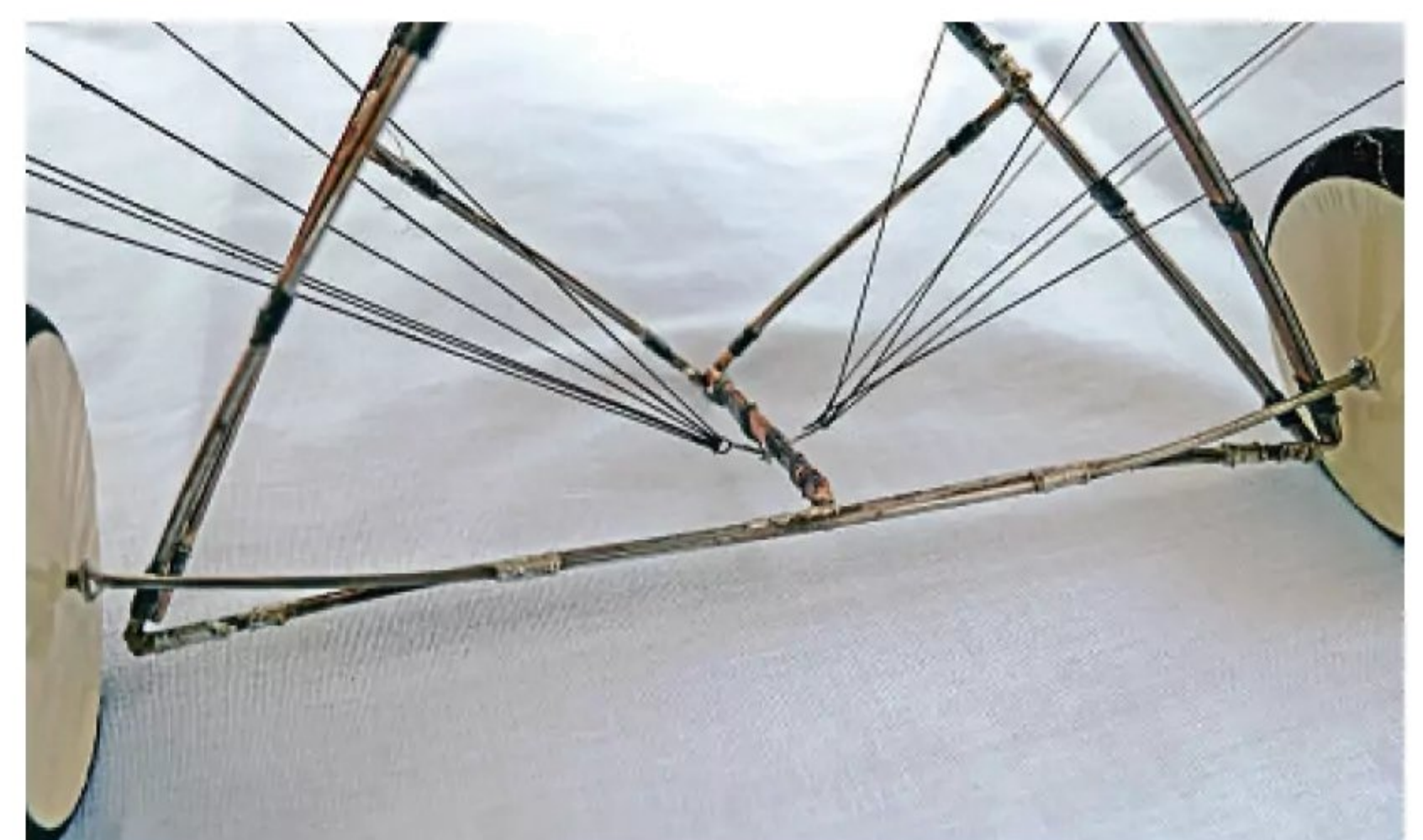
Left: The little Caudron 11 used to have a solid axle that imparted fuselage damage in less than perfect landings.
