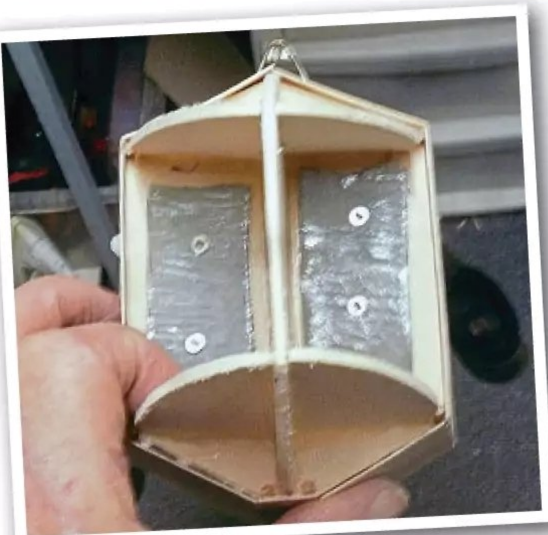
A big mistake. Embedded T31 ballast proved entirely unnecessary.
