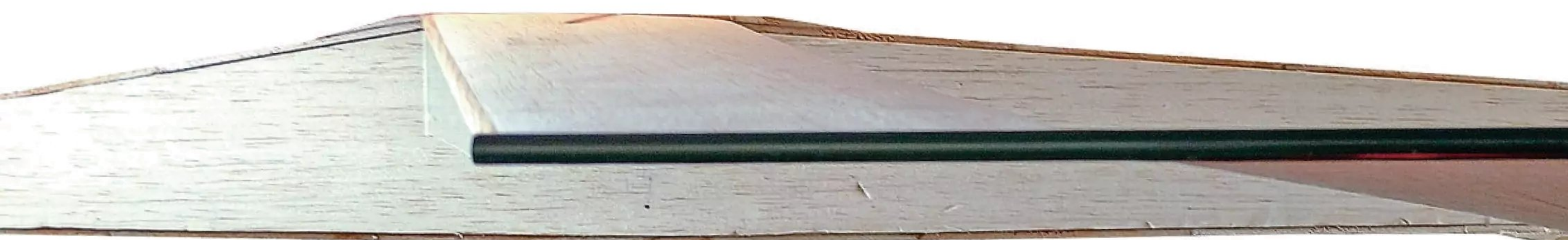
Above: Gently clamp the front and rear wing tips in alignment. Sand straight and level before fitting the carbon joiner tubes.
