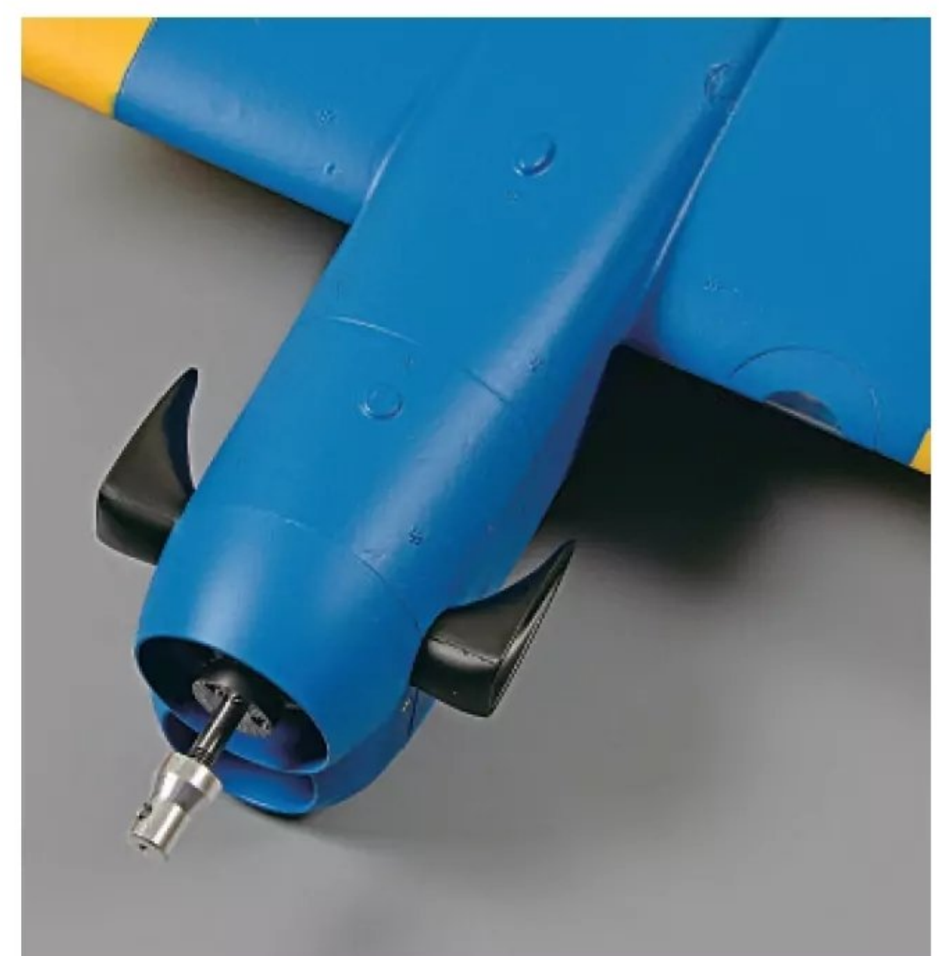
The 3-blade props are nipped up using a tommy bar through the prop nuts. A suitably sized screwdriver shaft does the job nicely.
