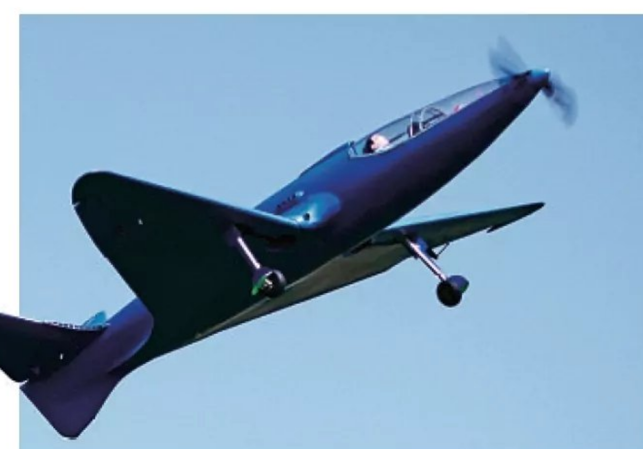
Bugatti maiden flight. The coaxial propellor was lacking a front bearing, which caused severe vibration, leading the model to crash.
