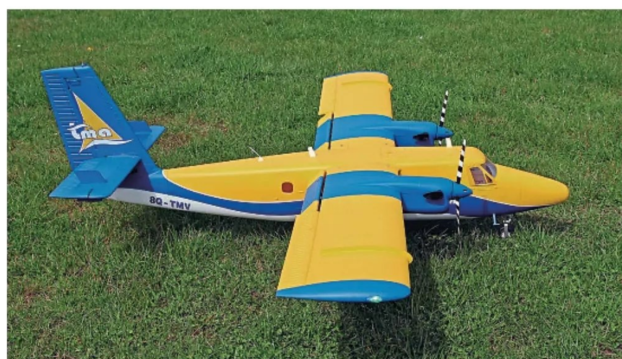
All move forwards, please! My 5000 mAh LiPo needed to be placed at the front of the battery bay to balance the model.
