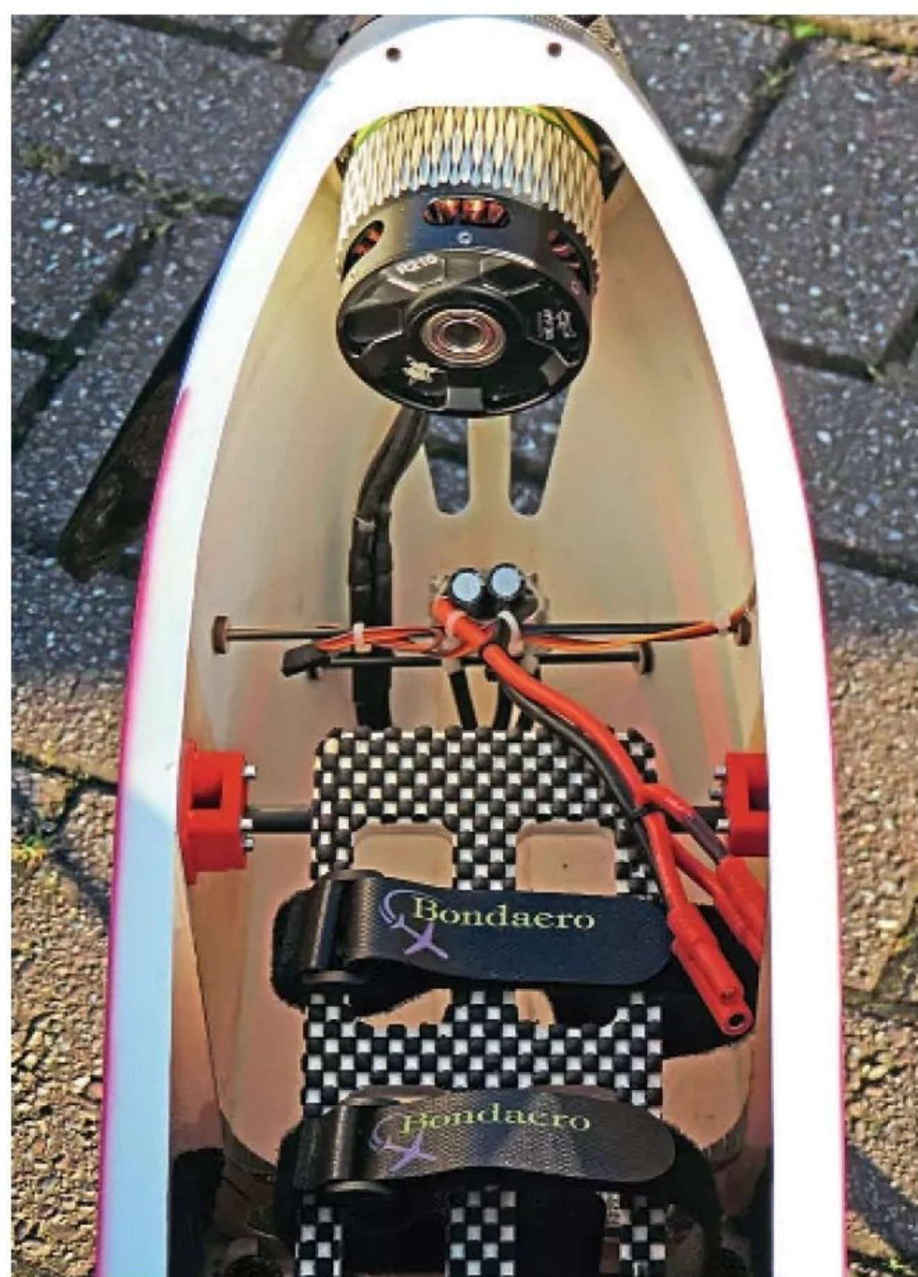
Left: Anthem nose showing R220 and D3 ESC locations.
