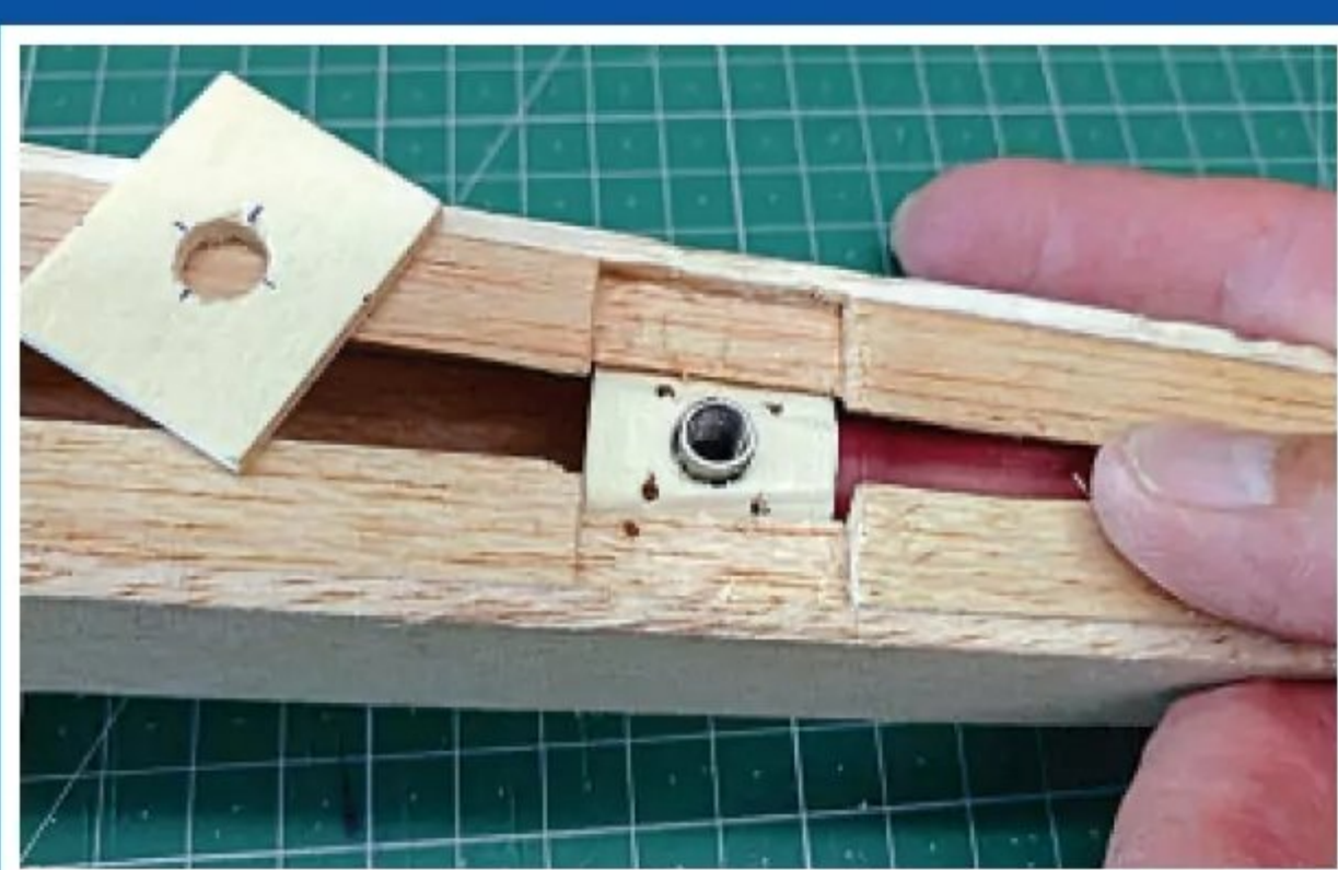
Fit the rear wing mitred support pieces in through the open rear of the fuselage.
