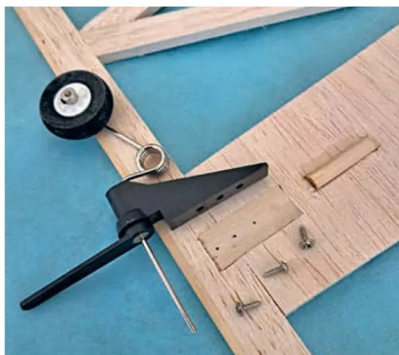
The Bigger Ship tailplane shows the ply tailwheel mount inset and one of the rounded location 'keys'.
