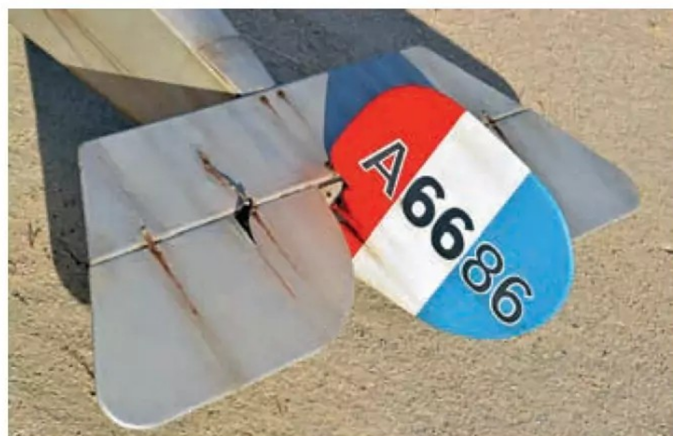
Tail surfaces are built entirely from balsa strip, which is light but prone to warping. The elevator and rudder are actuated through pull-pull wires.
