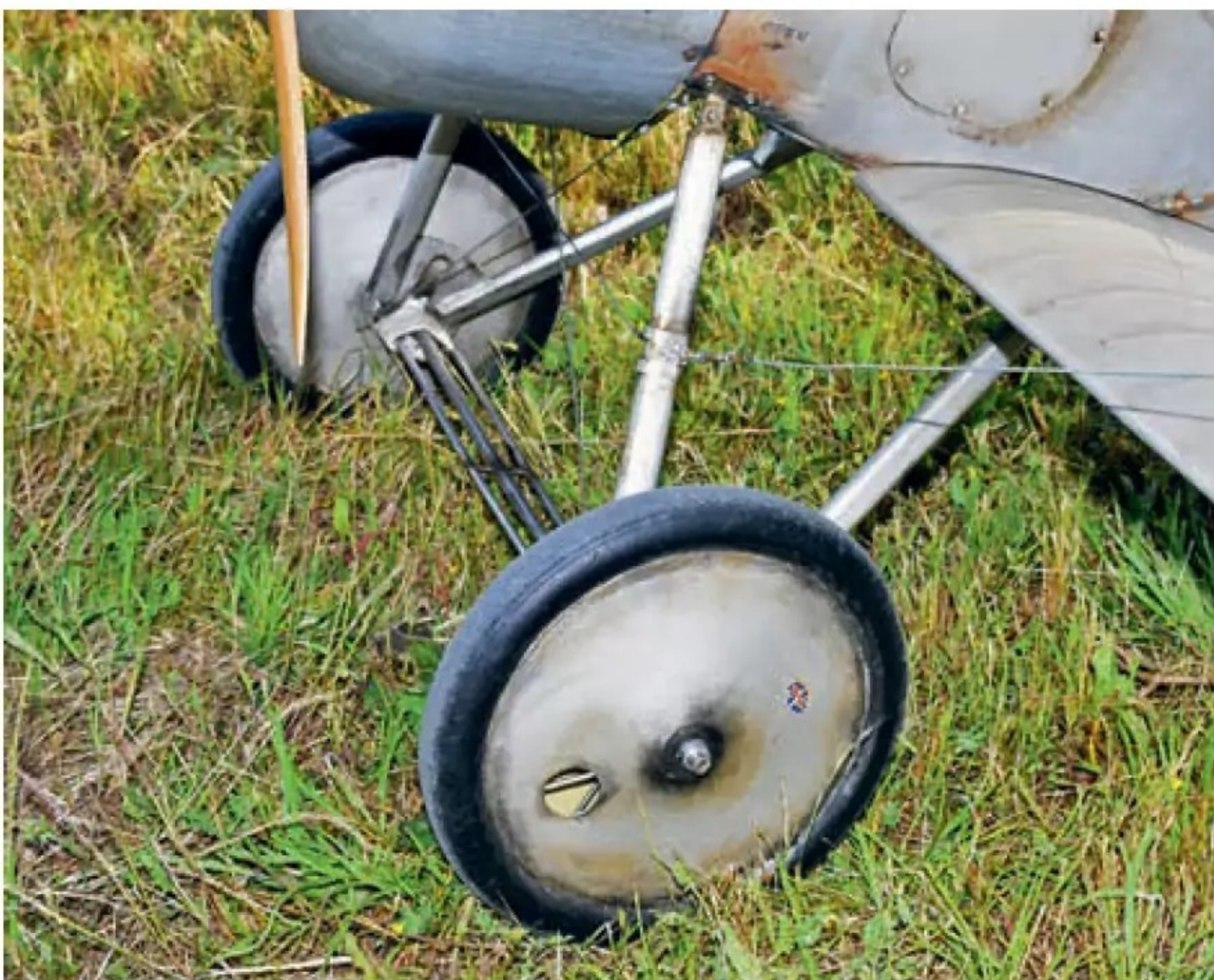
Landing gear is made from beech with embedded steel plates at the ends. Suspension is by bungee cord as per the prototype.
