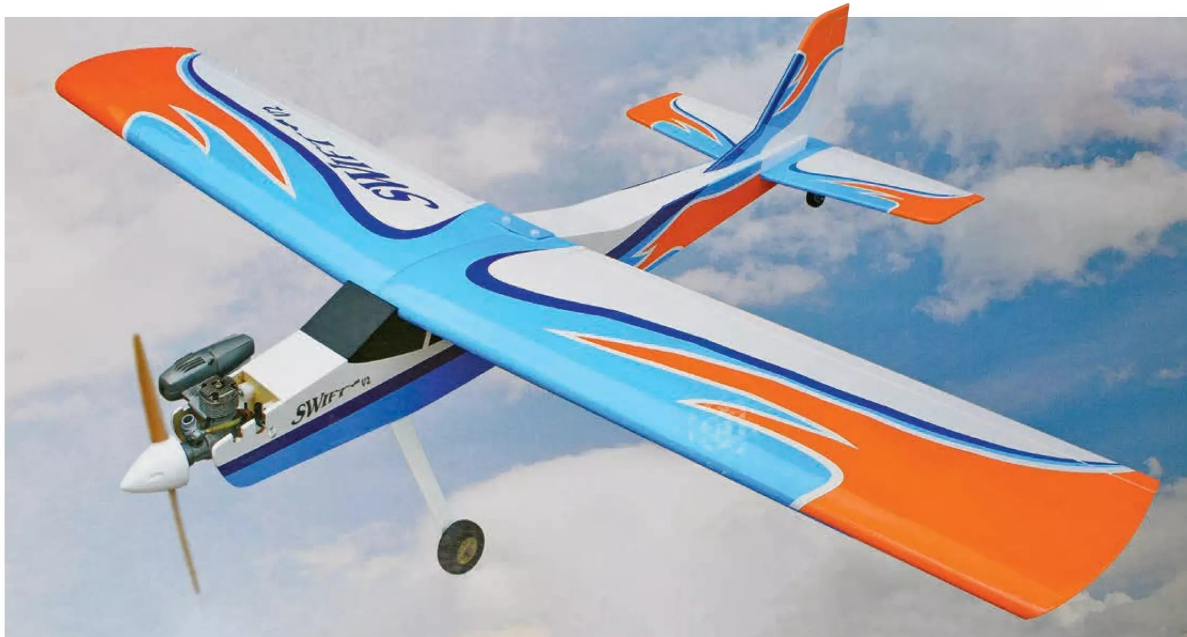
An upright engine installation in a model such as Seagull's Swift trainer is ideal for getting one's hand back in when operating an IC engine for the first time after a long lay-off.
