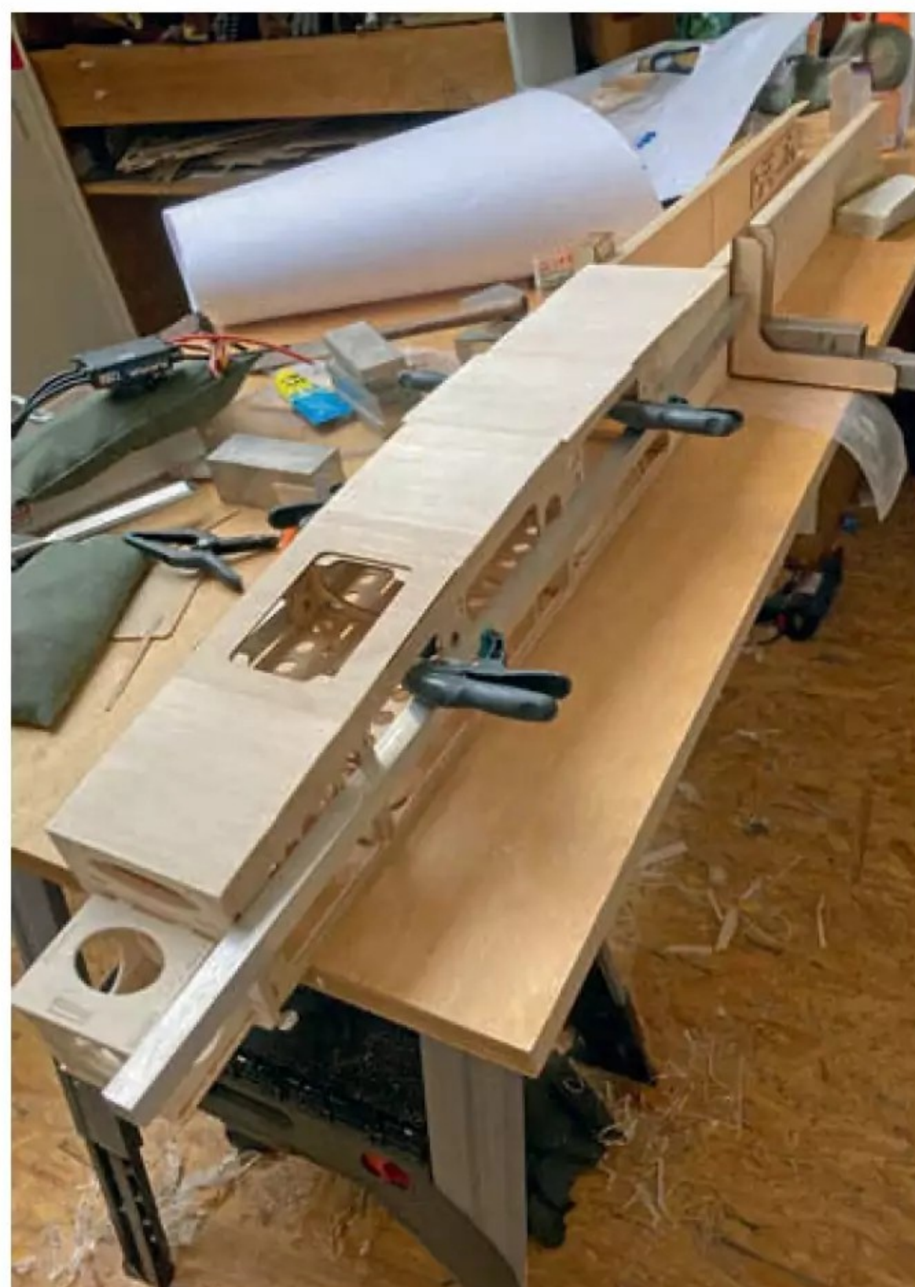
The front half of the fuselage is basically a square box. It is clamped tightly to the workbench and multiple aluminium sections are temporarily attached to ensure it remains straight during initial sheeting. Once the glue has dried the fuselage becomes so stiff that it is nearly impossible for it to go banana shaped.
