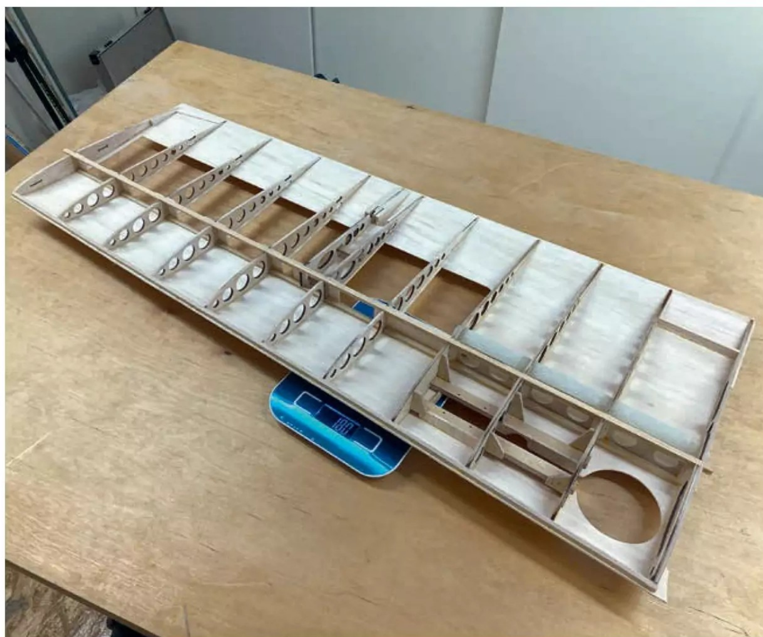
First half of a wing panel completed, as it comes out of the jig. Lower sheeting, wing tips and LE still need to be added. Weight at this stage is a mere 180 grammes.
