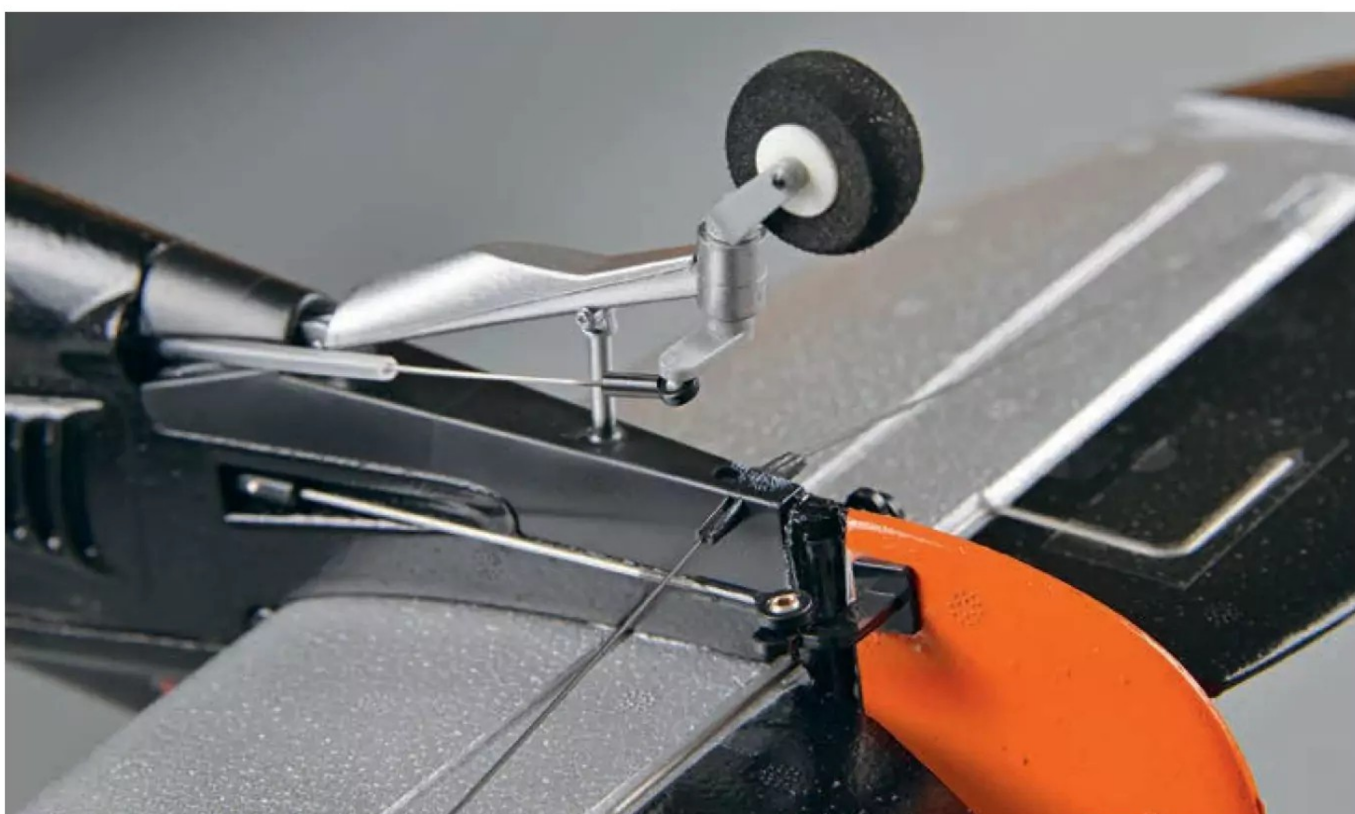
The steerable tail wheel closely resembles the full-size affair and is operated by a separate, thinner pushrod. Note the sturdier gauge wire used to operate the tail surfaces.
