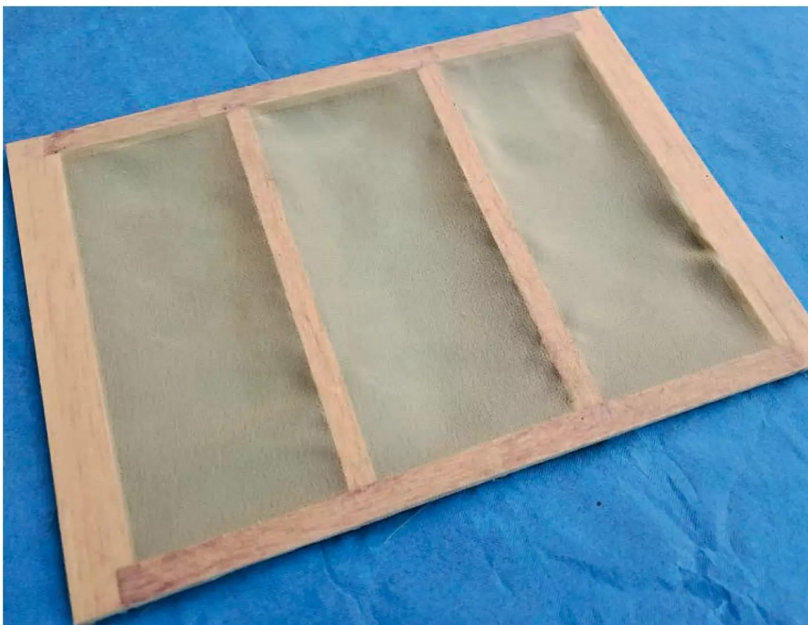
The test frame I made to check out polyester cloth as a covering material.
