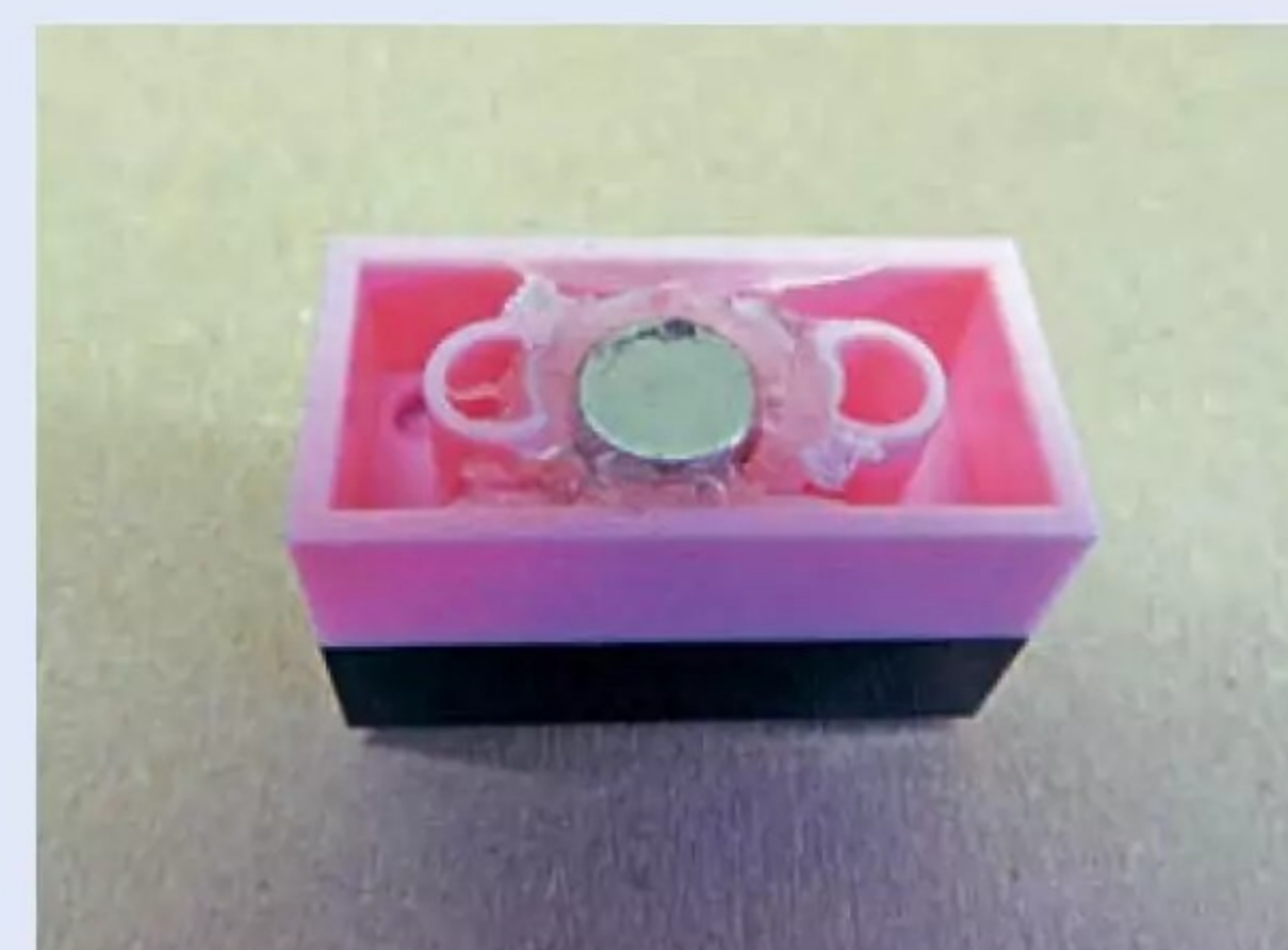
Standard square and rectangular bricks with magnets epoxied in place.
