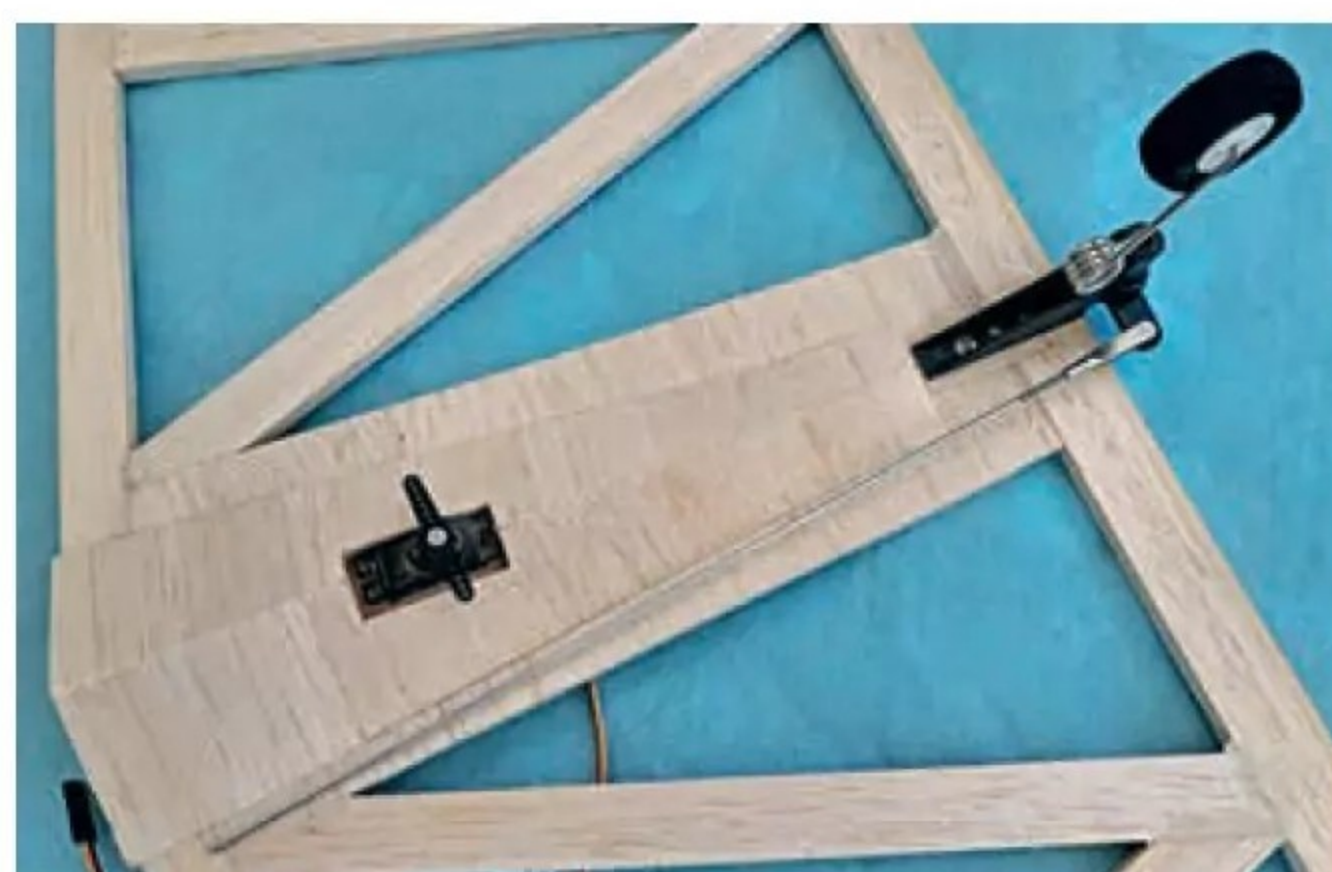
Under 'The Bigger Ship' tailplane showing the steerable tailwheel option. If the tailwheel turns in opposition to the rudder, I'll simply swap the pushrod from one servo arm to the other.
