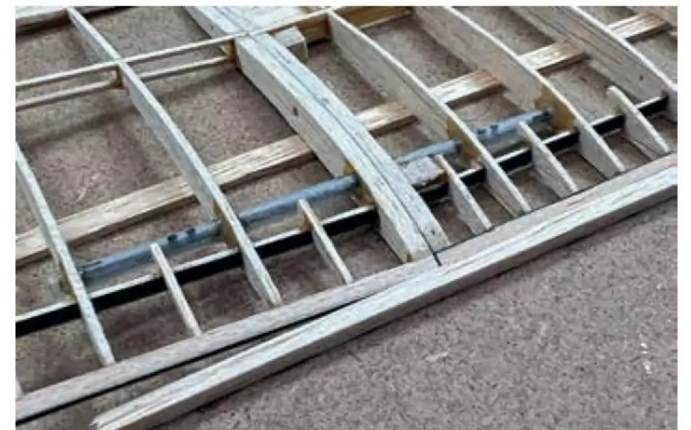
Dihedral joints are made using thin plastic tubes and one and two millimetre carbon fibre tubes.
