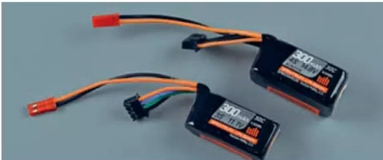
Micro Scrappy flies well on either a 3S or 4S 300 mAh LiPo but needs to be fitted with a red JST-RCY connector to match the power lead inside the battery bay.
