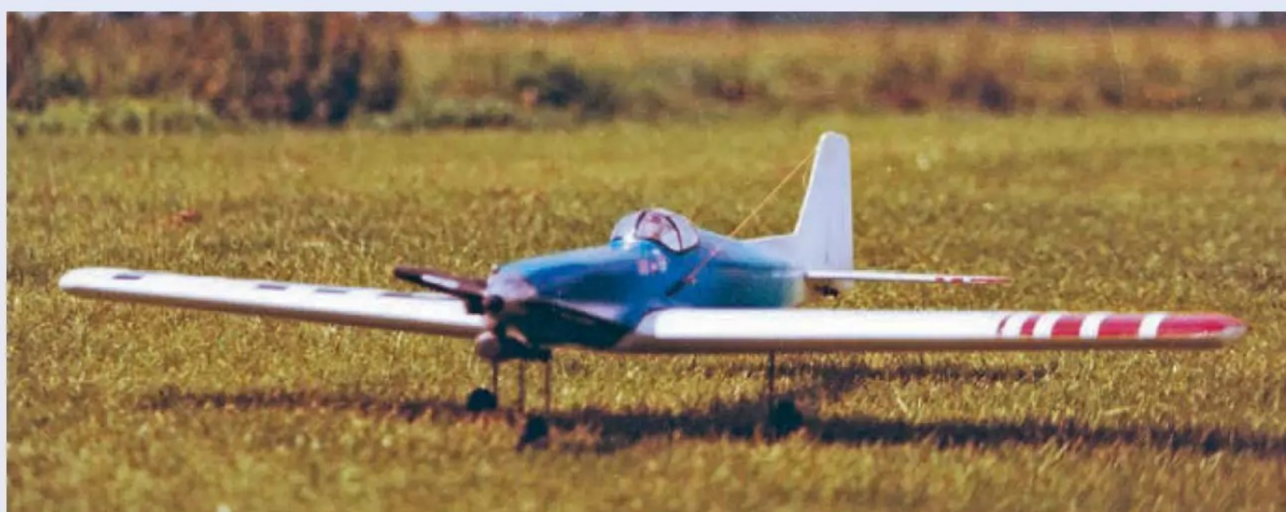
The author's Mäxi, built during the mid-eighties. Covered in nylon, with the front of the fuselage sprayed in an attractive translucent blue, gradually fading into the white base colour. Note the enlarged Mäxi logo on the starboard upper wing.
