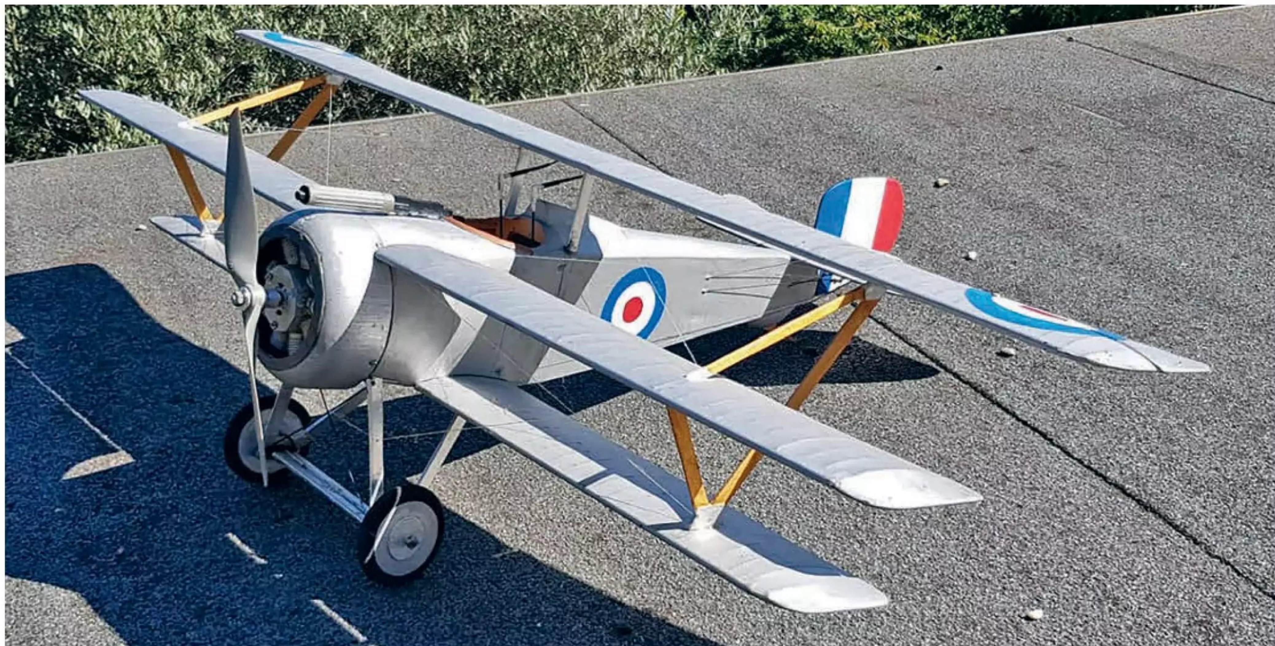
To test the calculated CG position António built this 3S LiPo powered eighth scale model. Not too shabby, especially for a guinea pig! (Photo: Mário Vilaça)
