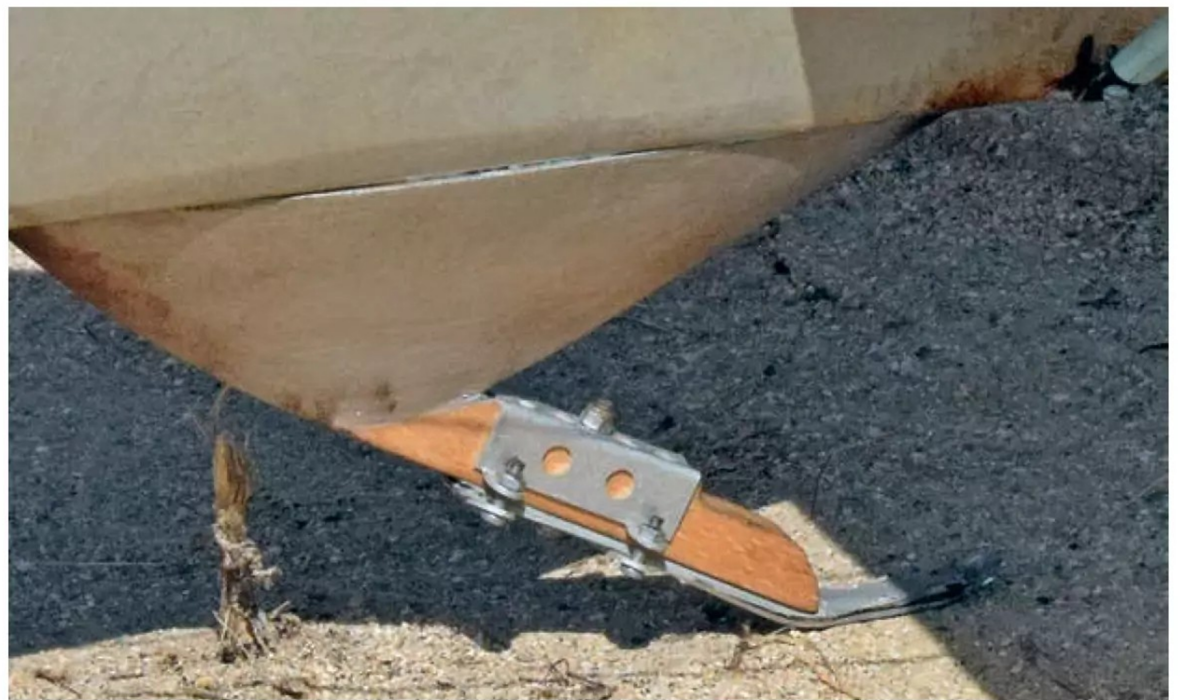
Tail skid is made from Marupa and steel plates, glued to a ply former and faired with balsa wood.
