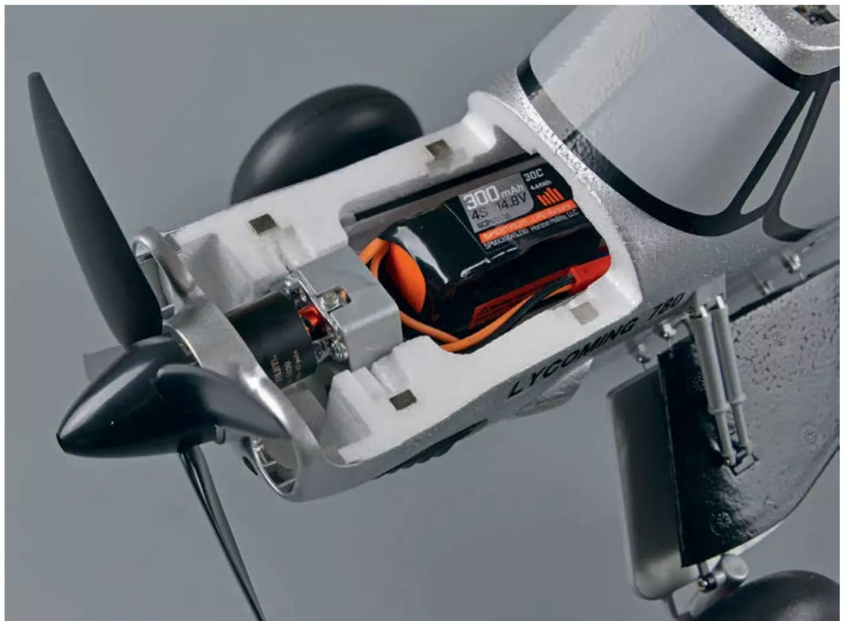
Cowl hatch pops off to reveal the motor mount and battery bay. Plenty of room inside for either a 3S or 4S Lipo.
