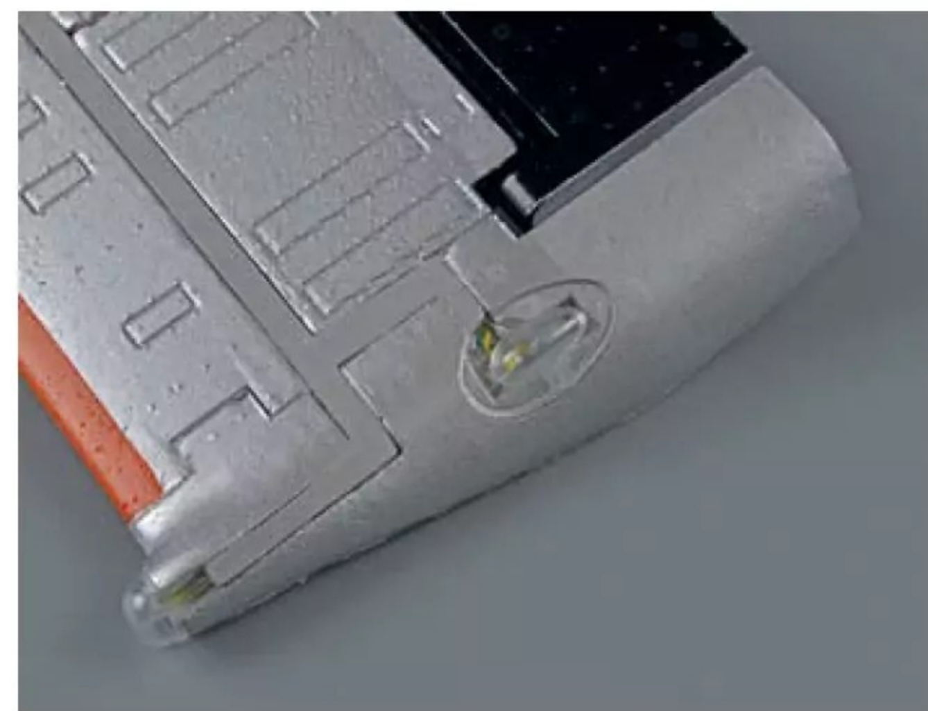
Each wingtip houses two lights with the wiring covered by neat full-span plastic covers. These covers are handy placed at the CG point, giving an easy reference for balancing.
