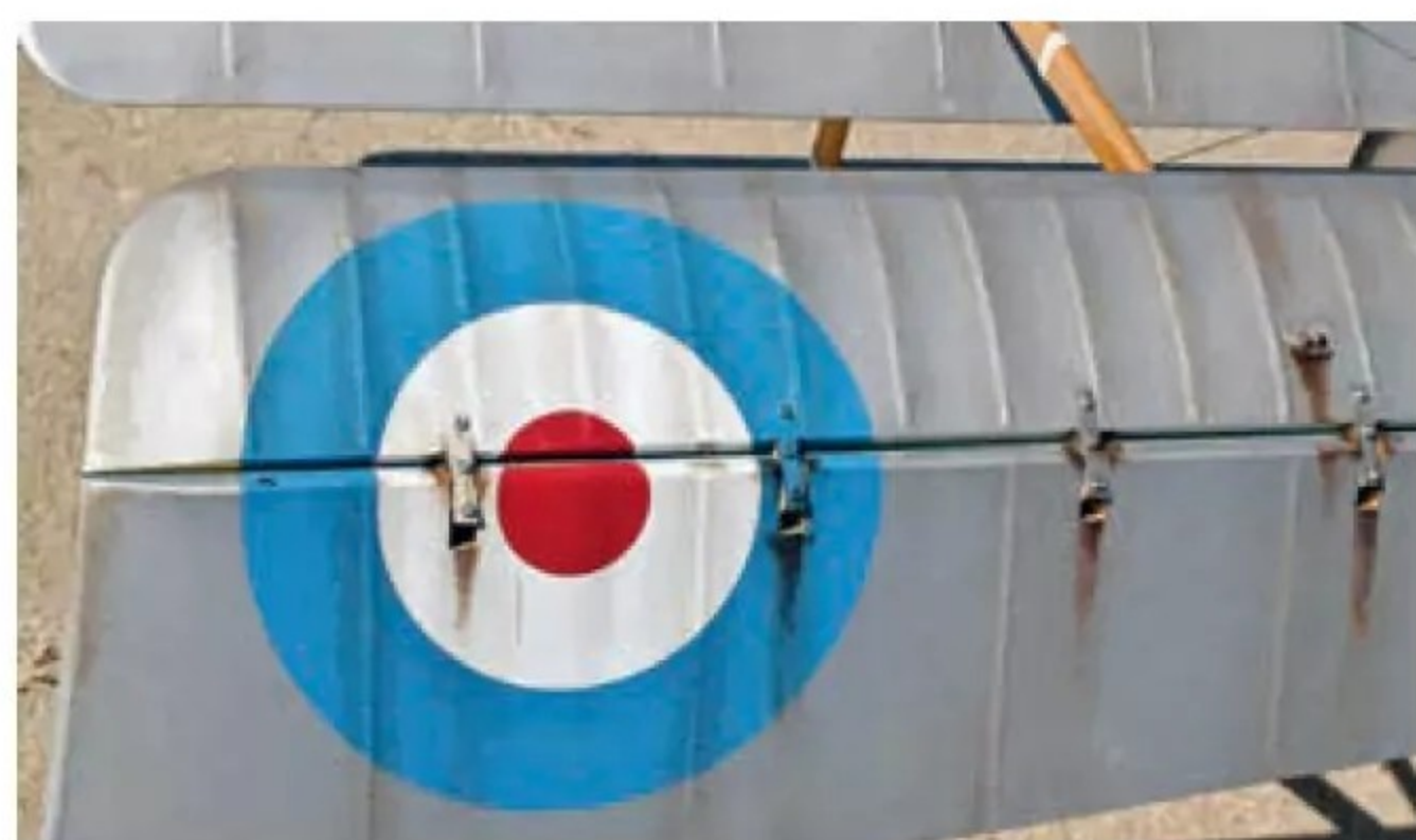
Upper port wing showing the aileron hinge details and rib tapes.
