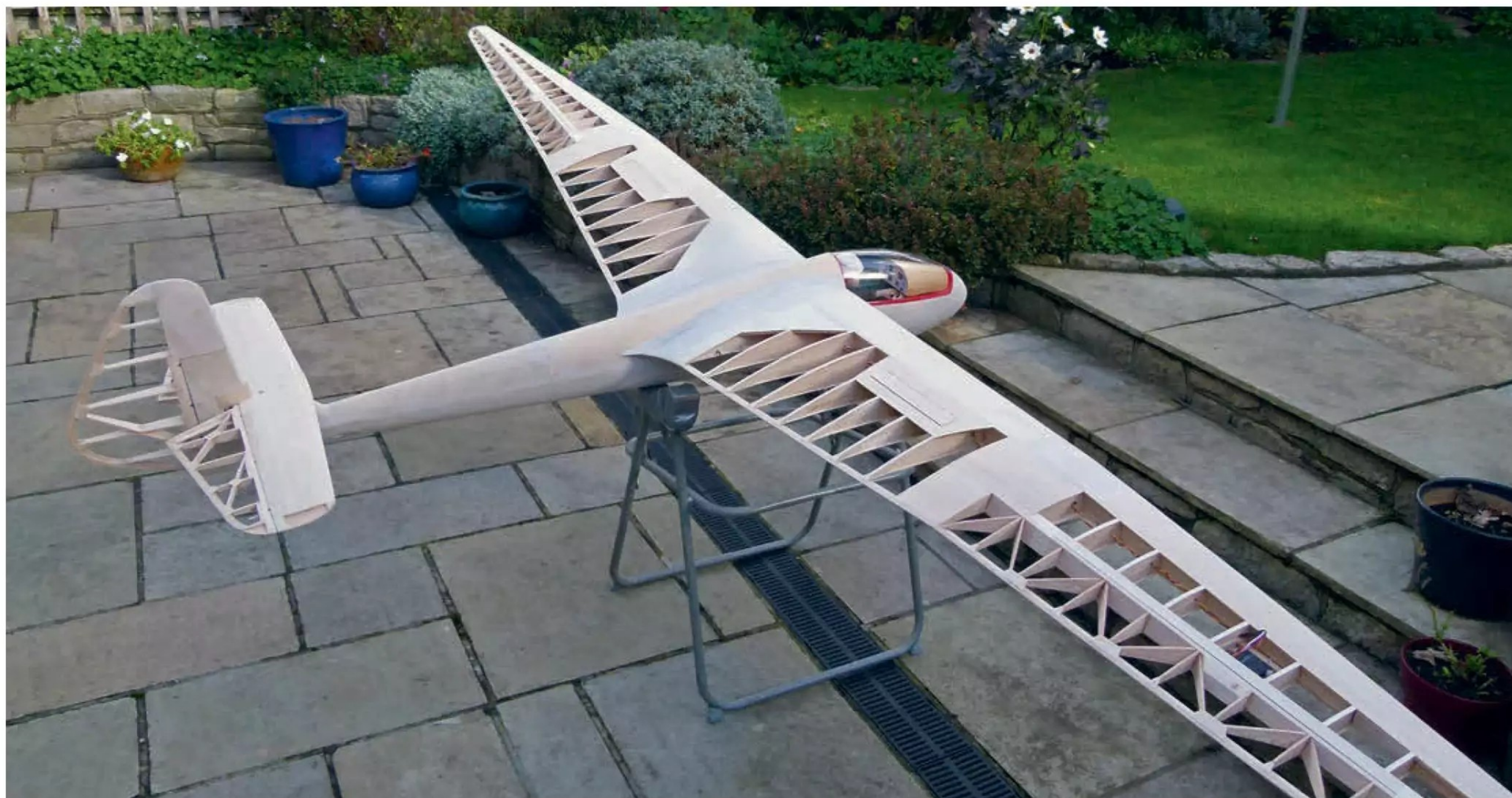
The 1:4.5 scale petrel airframe ready for covering.
