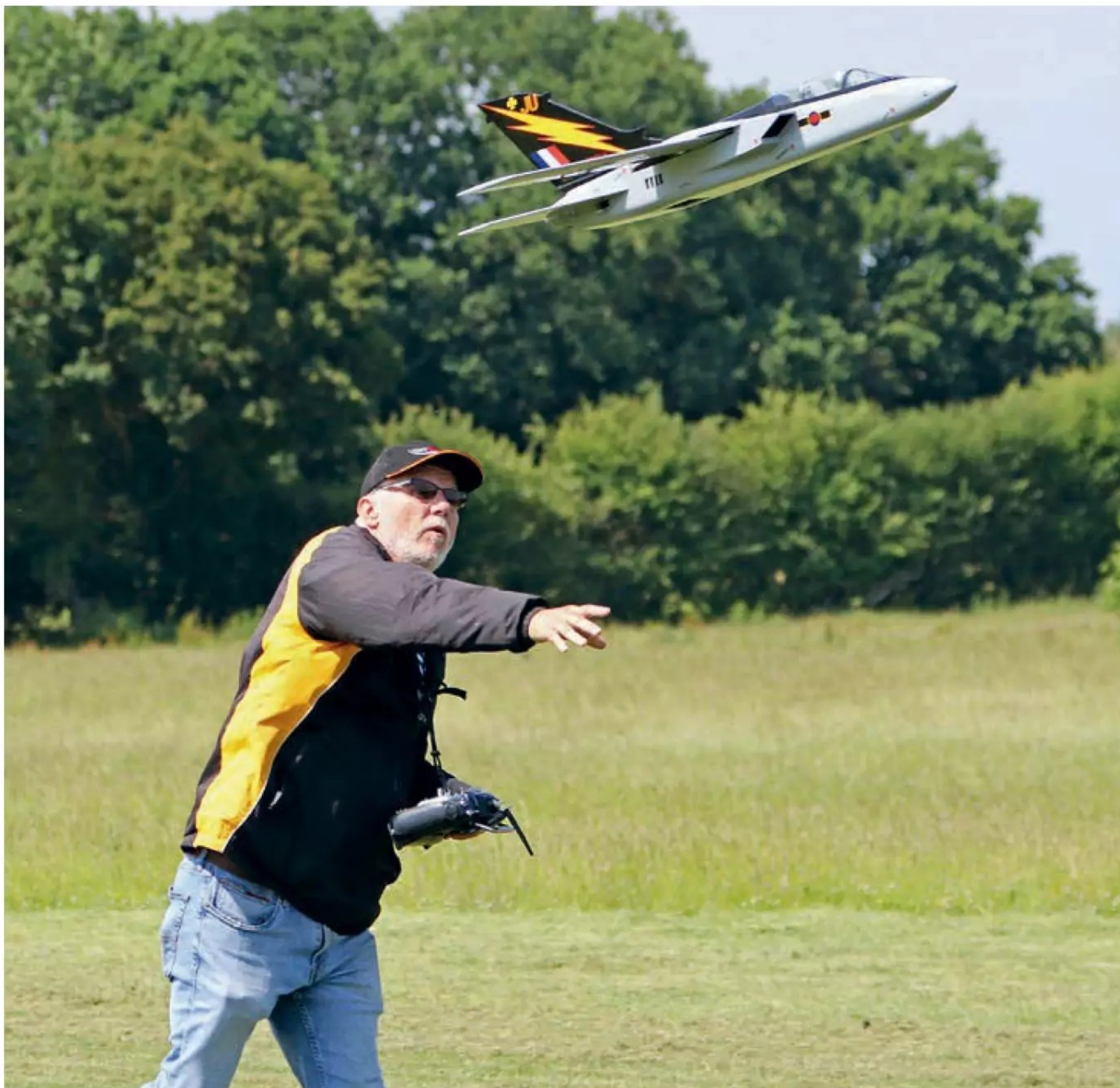
Hand launching the Tornado is easy using the javelin technique. The powerful throw and projection of the model upwards gives more time to get your fingers back on the Tx sticks.
