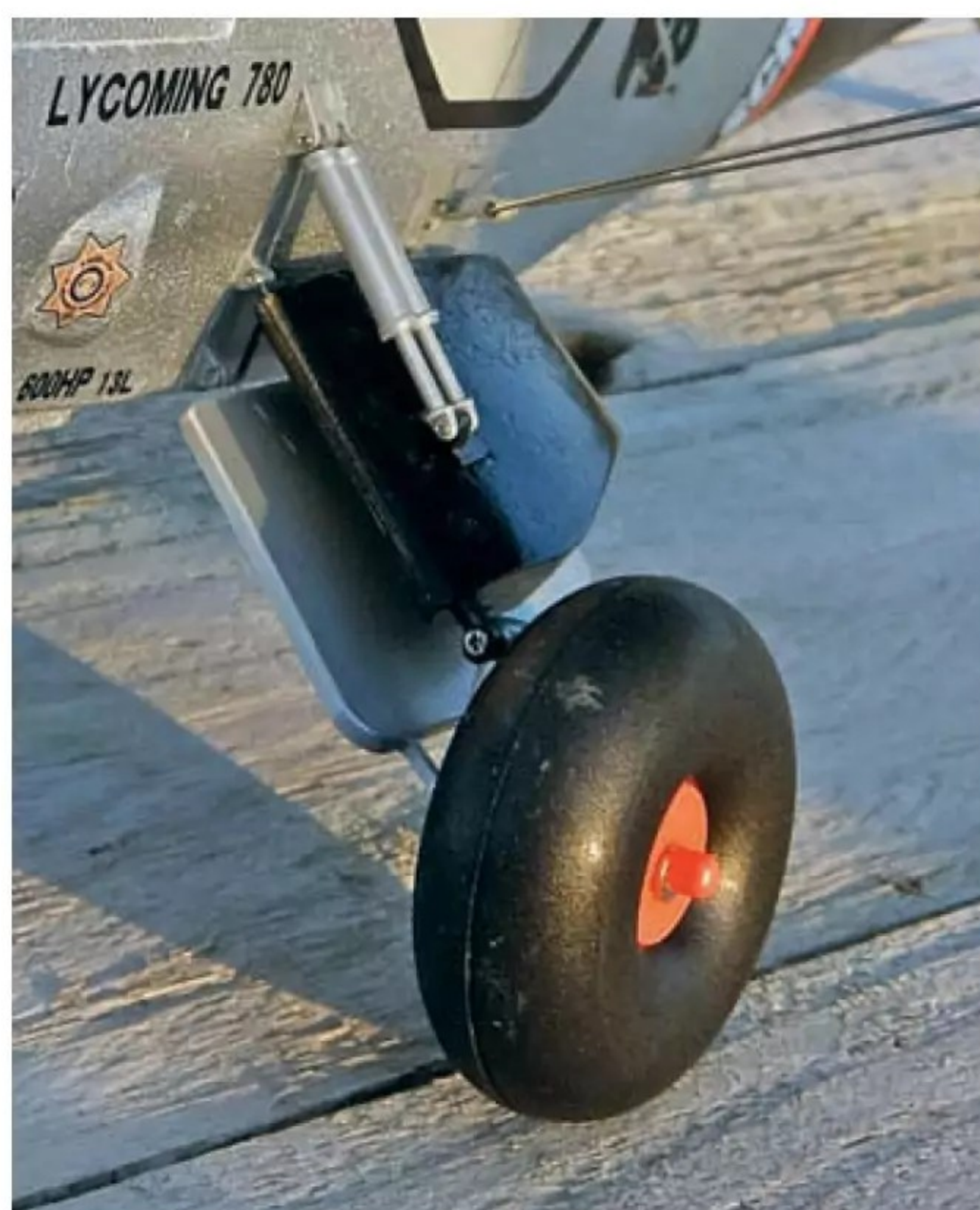
The long travel undercarriage of the full size Scrappy is neatly replicated but is not sprung.
