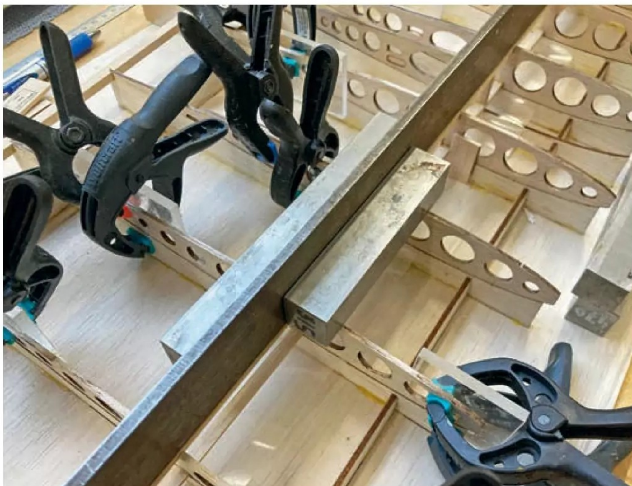
With the upper spar in place the ribs are kept in place against the plywood jig using small pieces of acrylic glass and lots of glue clamps. The lower spar is kept in place by a long metal ruler.
