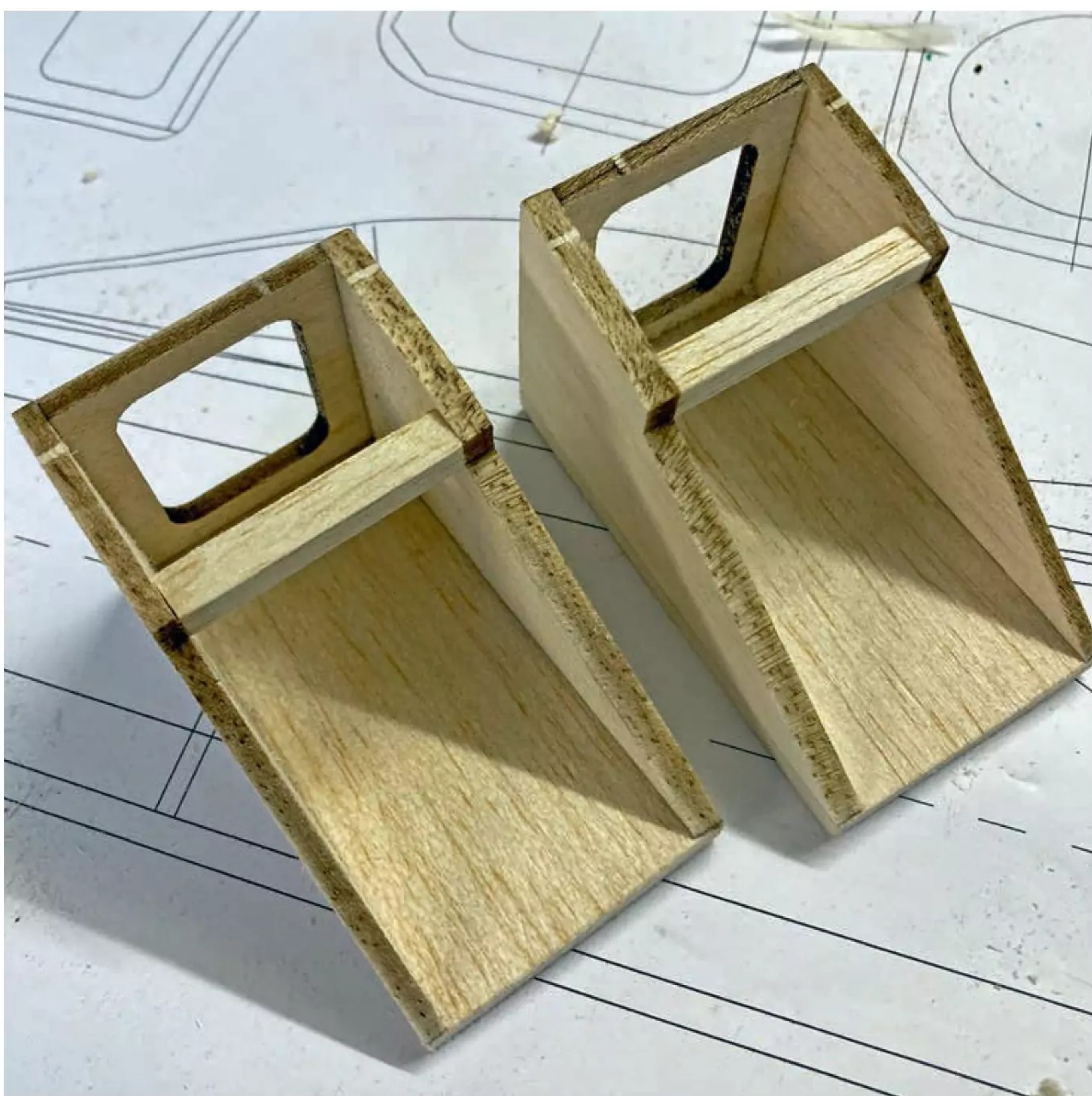
Dummy air intakes made up before gluing against F4 and the fuselage sides.
