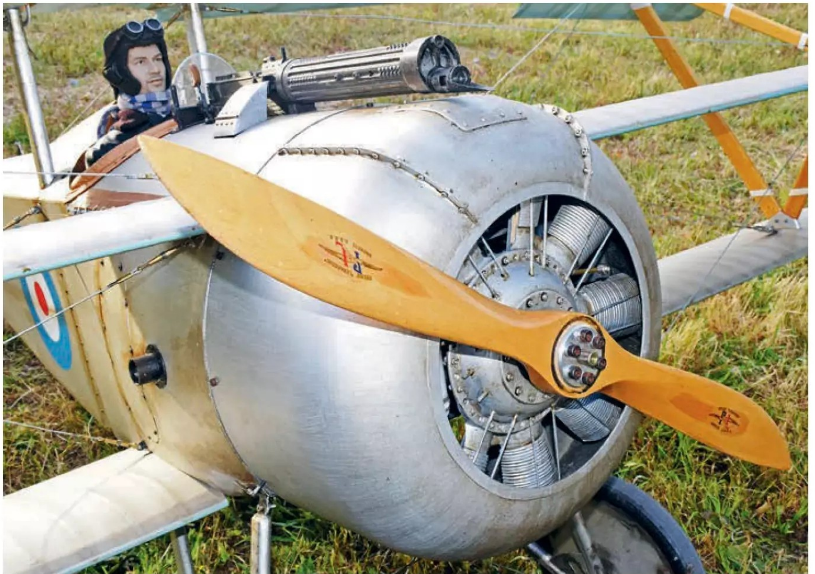
The original Ni 17 cowl was made from two aluminium pieces bolted together. Mário's was spun in one-piece, with dummy details added later. The finishing touch is the dummy engine from Mick Reeves Models.
