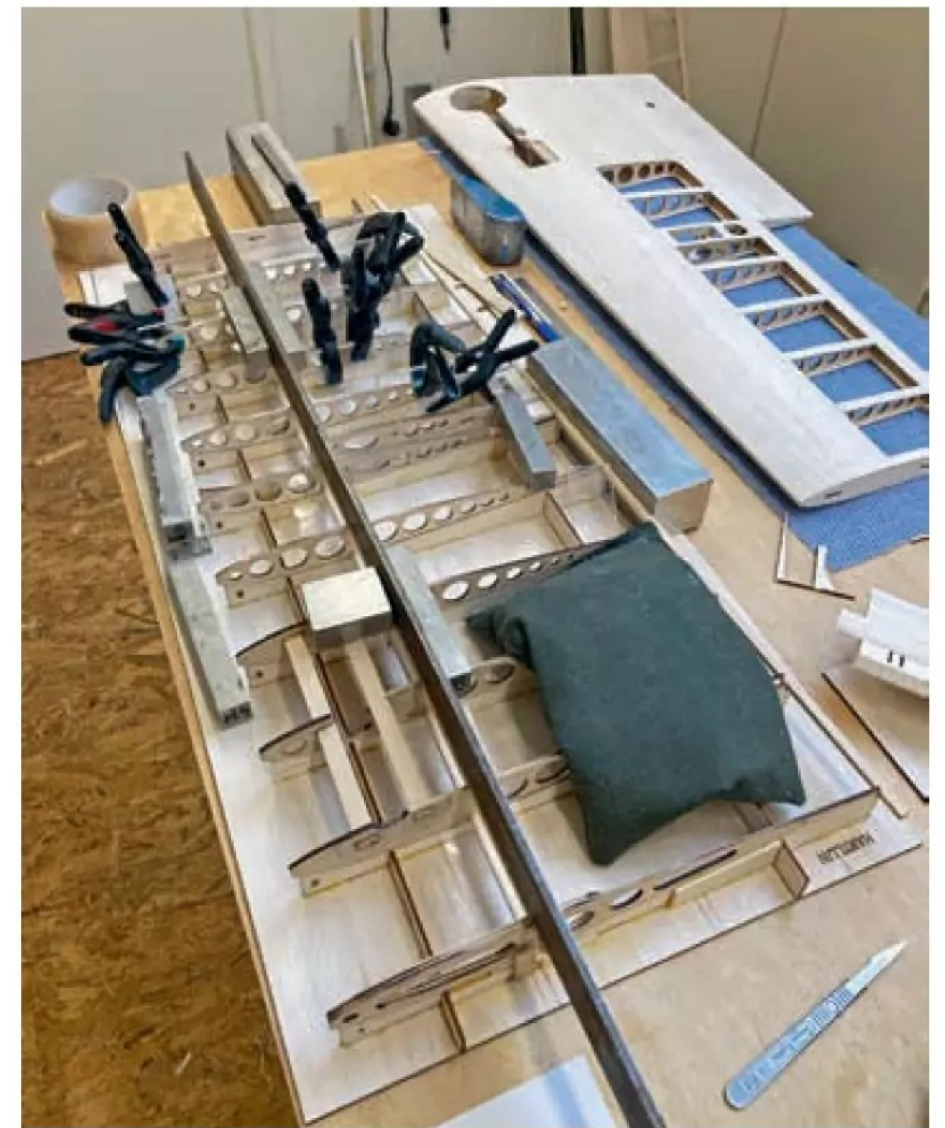
The wing is built inverted as the top of the wing is flat. The only dihedral comes from the tapering of the ribs.
