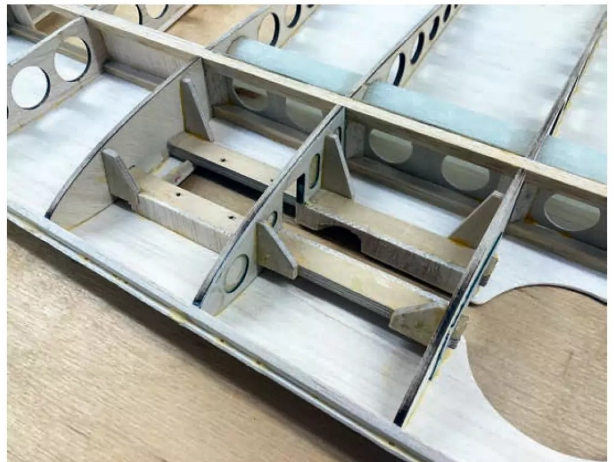
Close up view showing the epoxy wing tube sleeve at the rear and construction of the undercarriage bearers. Note the plywood webbing in this part of the wing for additional rigidity.
