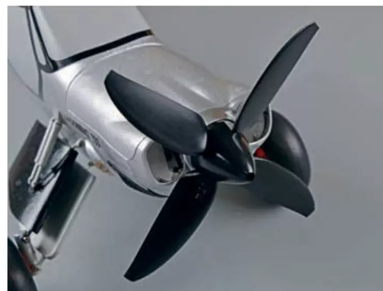
Four blade prop is well suited to the power system and is a good example of the time taken with the model's product development.
