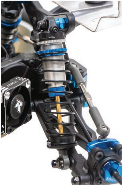
The silky-smooth 13mm big-bore shocks come standard for exceptional performance.
