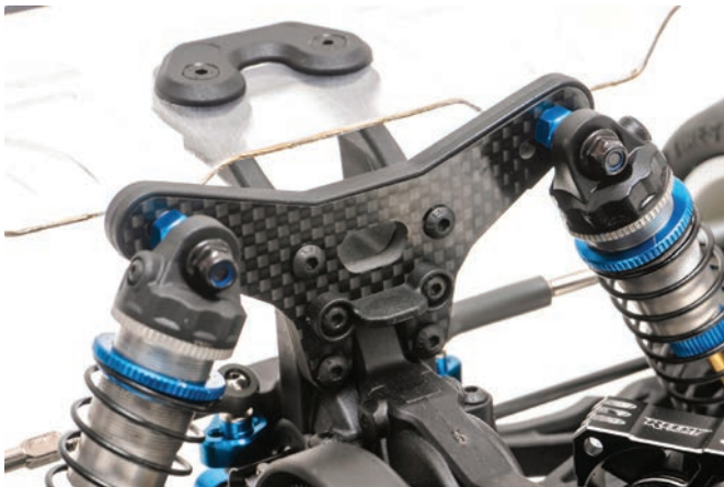
The new -2mm shock towers lower the overall CG of the B7.1D and add to its overall stability.
