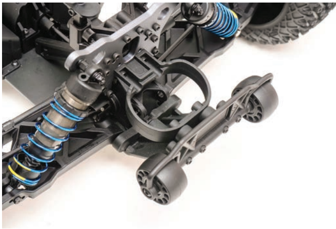
The rear bumper doubles as a wheel bar that keeps you from looping out during a gnarly wheelie.
