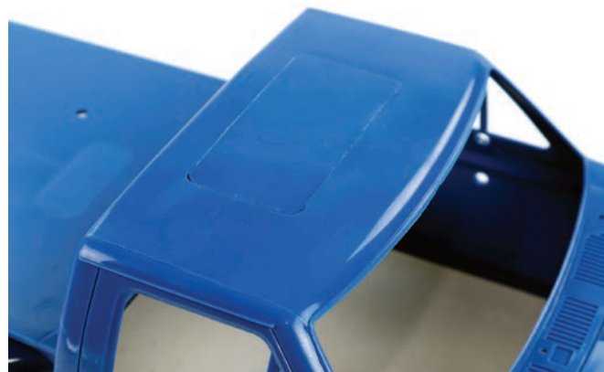
I like a clean roof on my Tamiya vehicles so I always glue the roof patch in place with CA glue, then I use the glue as a filler on the gap all around the patch.
