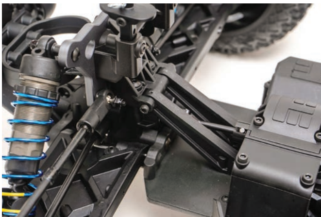
The dual chassis brace keeps unwanted flex to a minimum while adding stability to the rear end of the truck.
