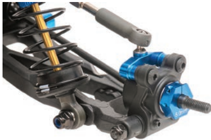
The rear hubs allow easy access to make camber link length adjustments, hub height, or different-width hex changes.
