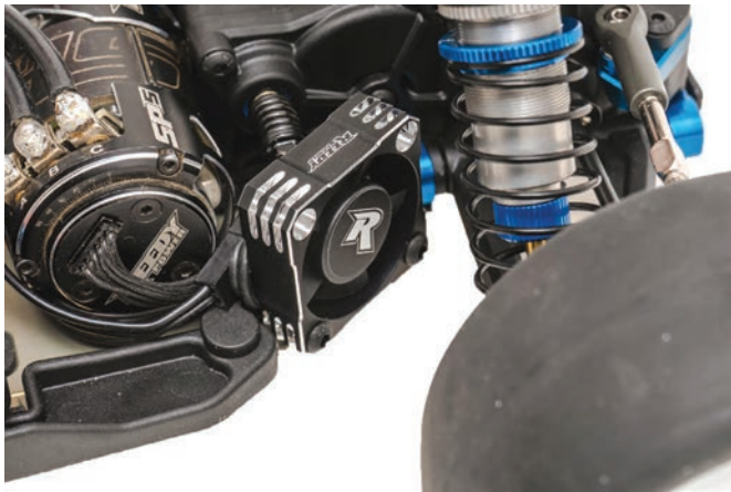
The integrated mount can fit a 30mm fan in the perfect position to effectively cool the motor.
