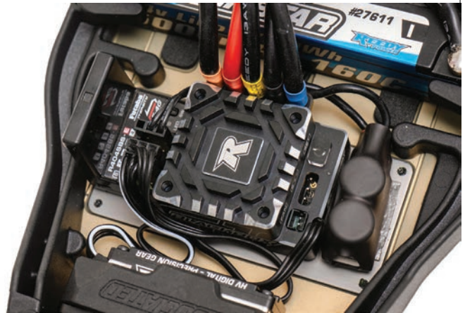
The included 11g aluminum chassis weight neatly fits the ESC and receiver and can be removed to allow easy maintenance.
