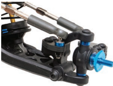
Up front, you can change the steering block height as well as the carbon fiber steering and camber plates for further suspension adjustments.
