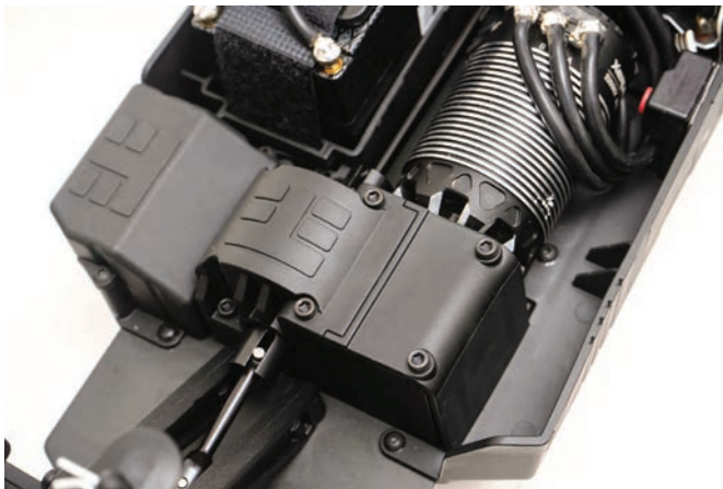
The receiver and spur/pinion gears are covered and well-shielded from dirt and debris during hard bash sessions.
