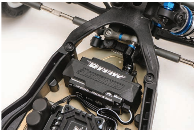
A straightforward but effective design, the dual bellcrank steering system can be height-adjusted—Ackermann adjustments being made by adding or removing blue aluminum shims.
