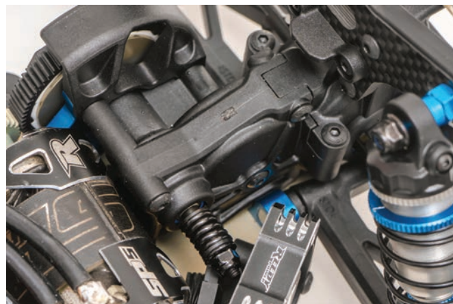
The compact three-gear transmission reduces rotating mass and gear mesh drag. The slipper clutch can be easily adjusted via the spring-loaded adjustment nut.
