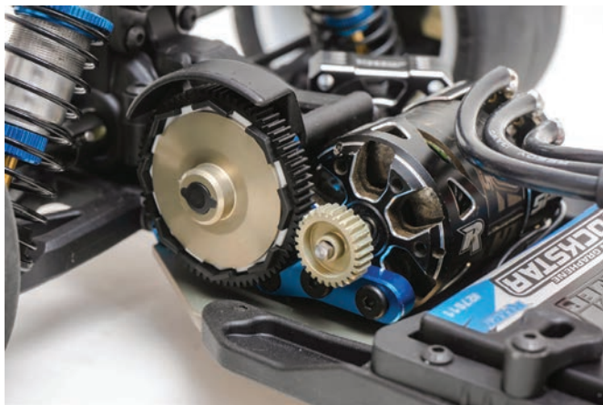
The motor mount side of the transmission is all business and allows easy access to gear mesh adjustments, motor swaps, and gear/pinion gear changes.
