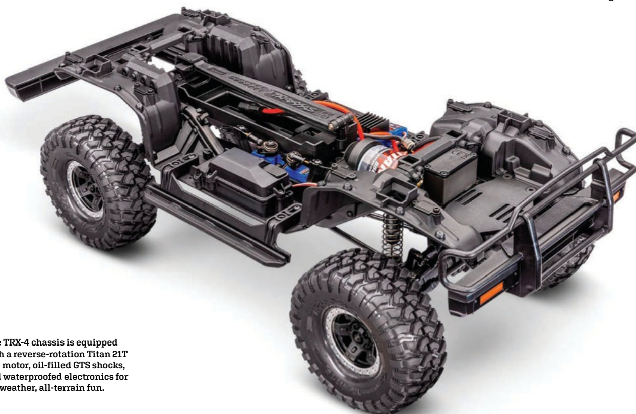
The remotely shifted two-speed transmission allows drivers to switch between higher speeds and low-range crawling.
