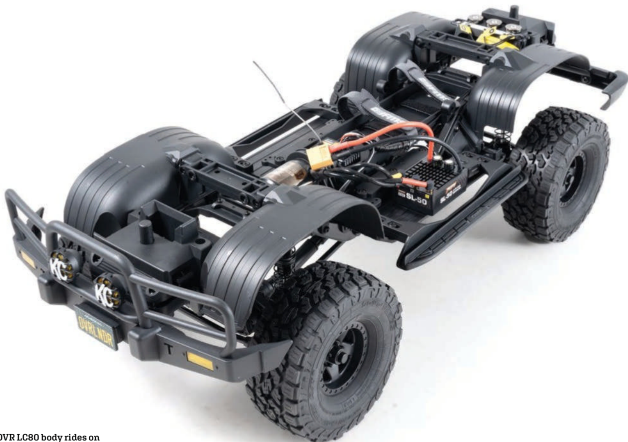
The OVR LC80 body rides on FMS's proven FCX10 chassis. Power is provided by a 1200kV motor and SL50A ESC.
