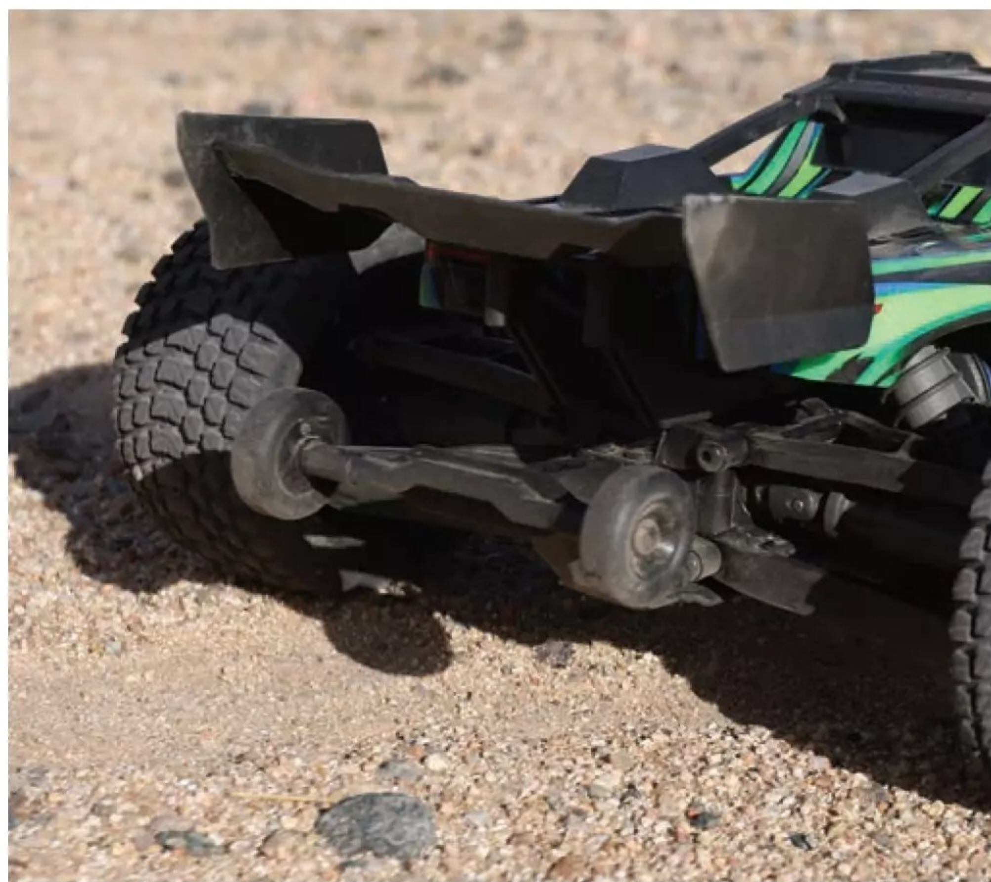
The reinforced wheelie bar shields the wing during extended wheelies—and doubles as a handy carry handle.
