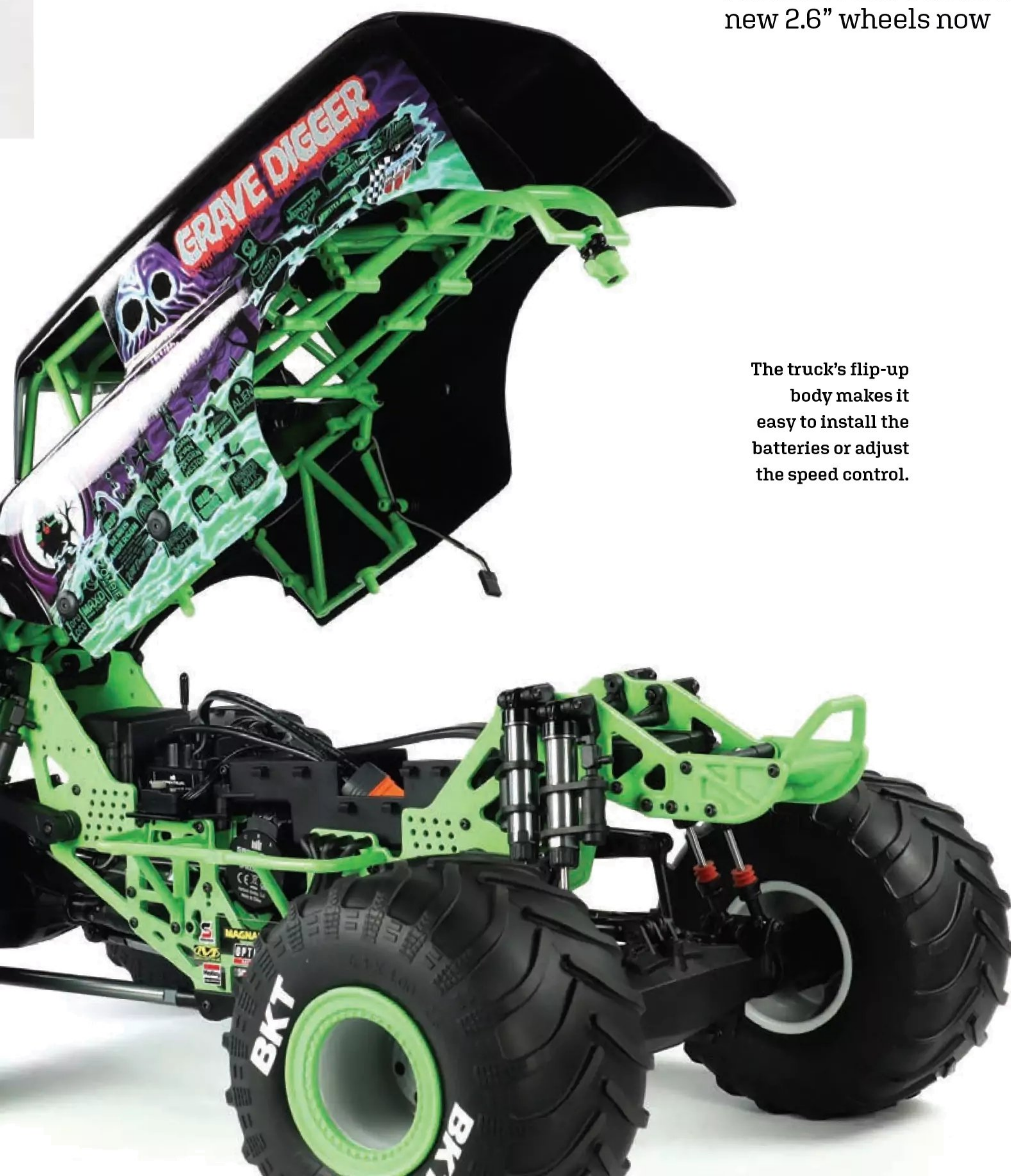
The new twist lock system on the back of the body is the key to ease of use when it comes to flipping the body up.
