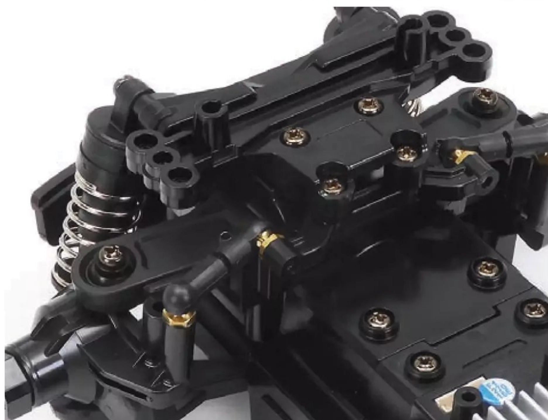
A sub-deck spacer is used to set the chassis wheelbase at 239mm, matching the Golf II GTI's proportions.
