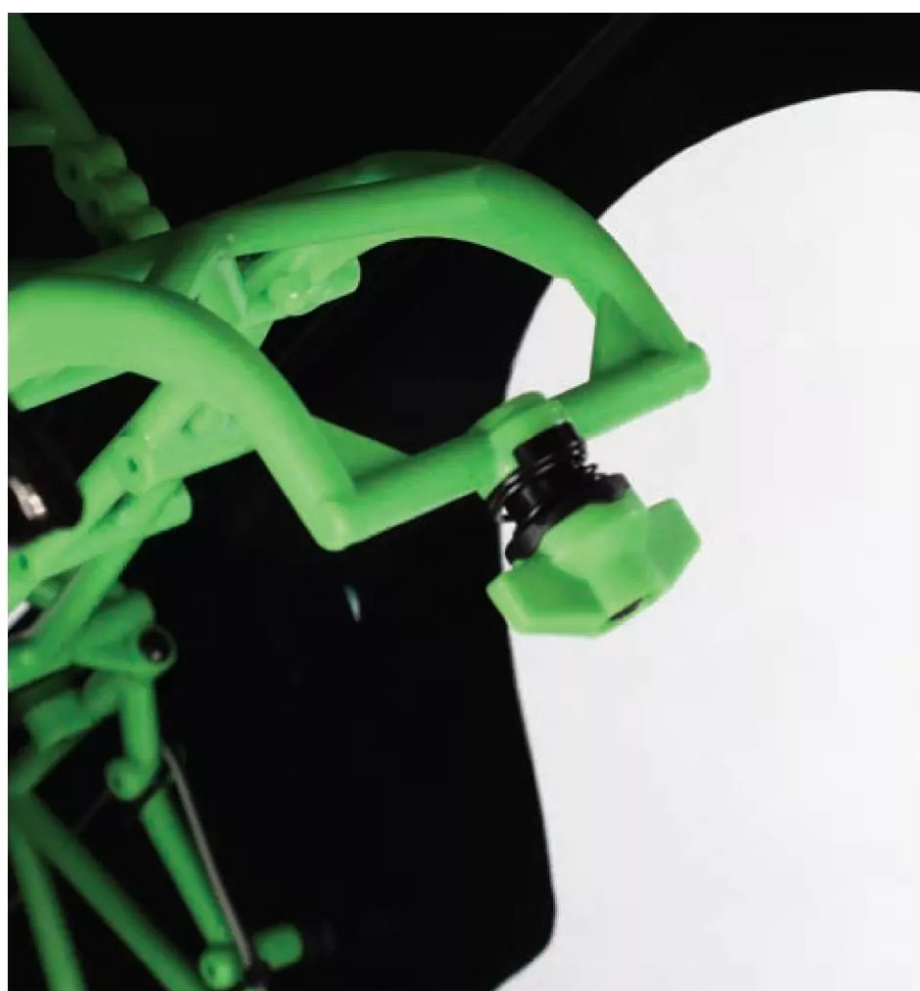
The new twist lock system on the back of the body is the key to ease of use when it comes to flipping the body up.
