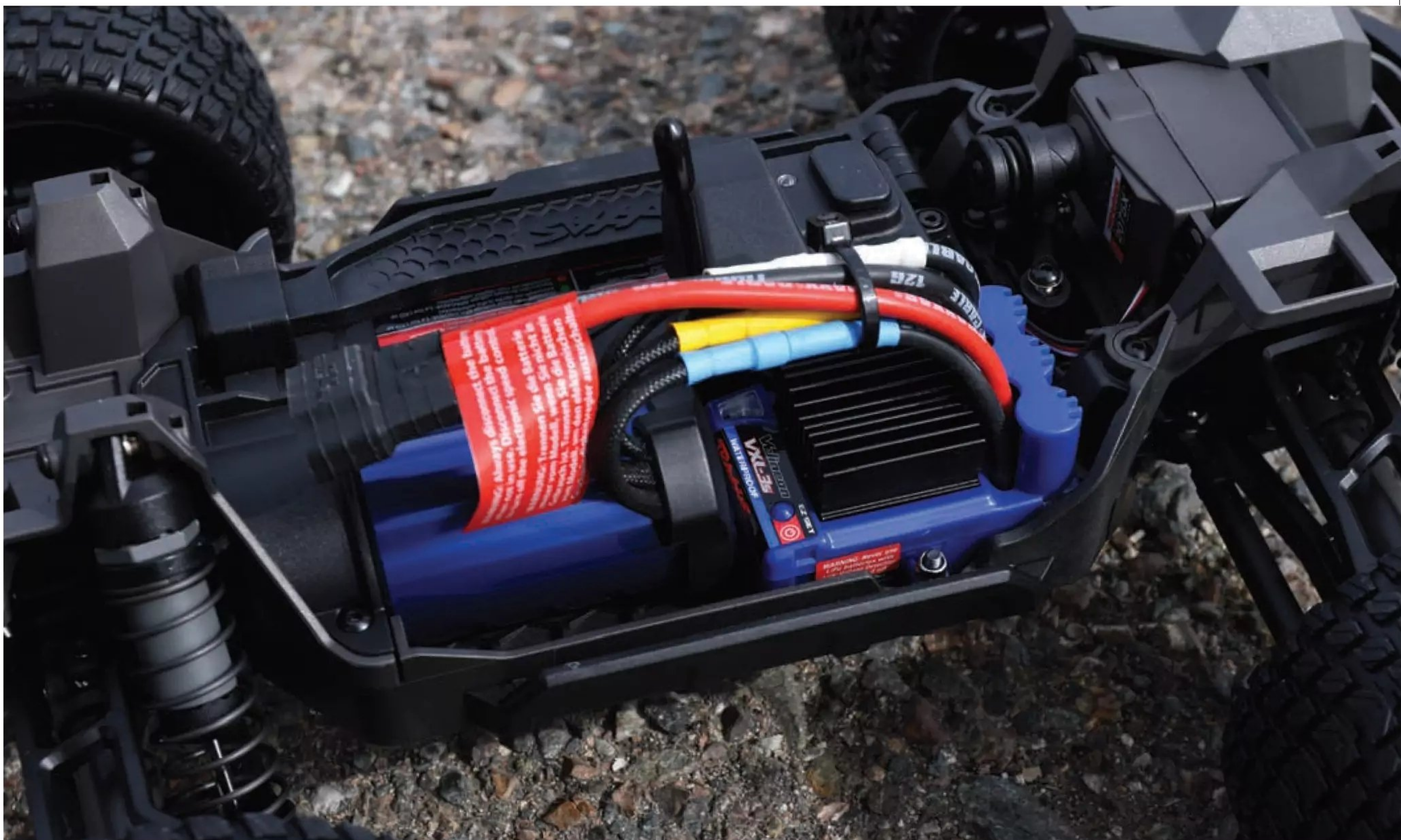
The Traxxas VXL-3 system delivers brushless power and efficient performance, perfectly matched to the Mini XRT's high-speed potential.
