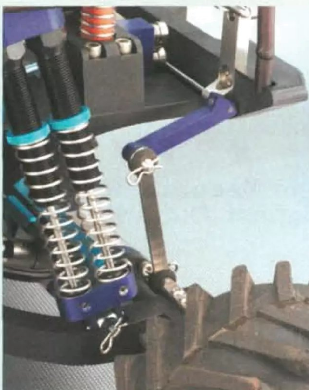
Even the swaybar looks good! It can quickly be disconnected by removing the lower carriage pin. The link can then be rotated and mounted on the frame and out of the way.
