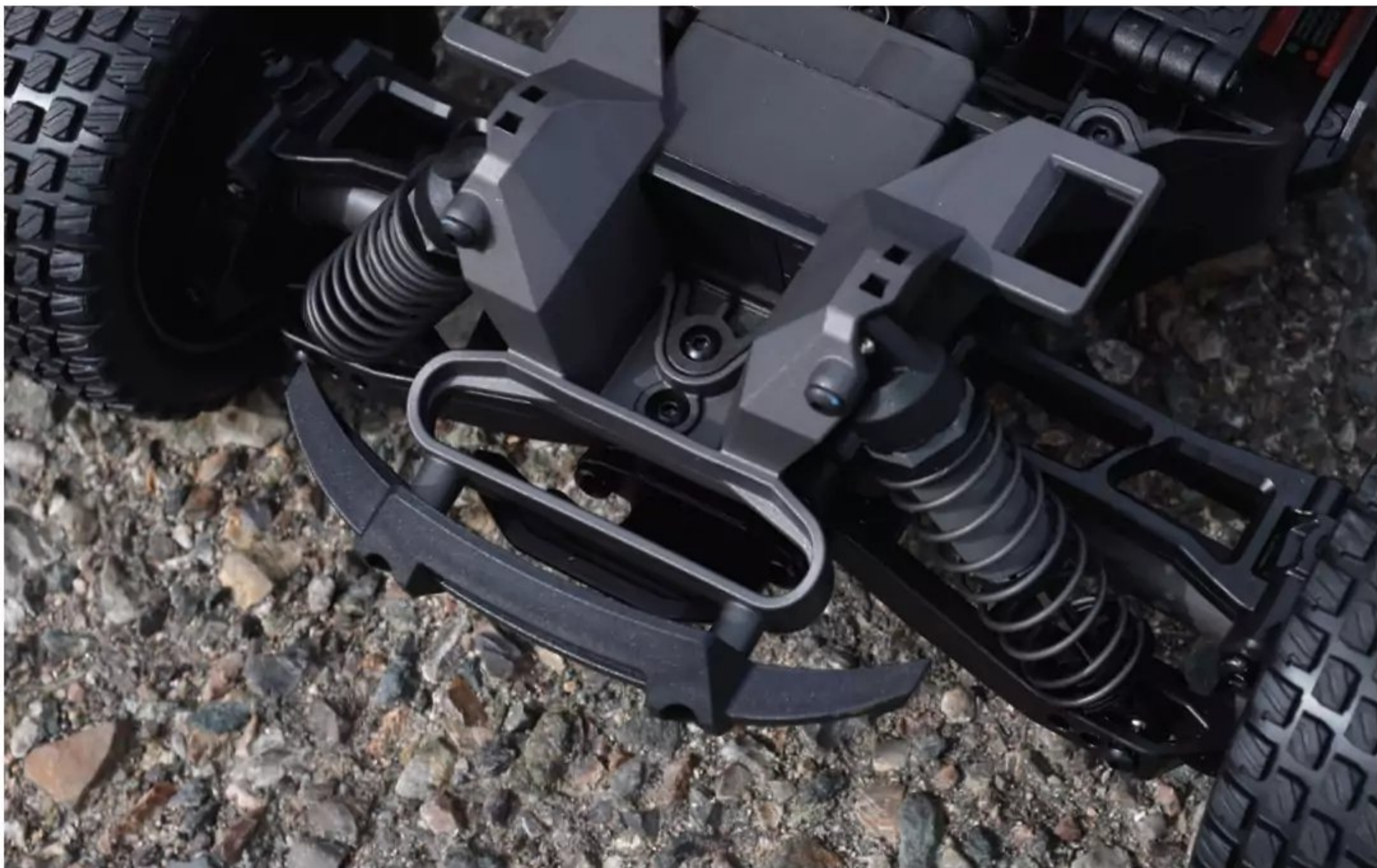
Oil-filled 1/10-scale Ultra Shocks front and rear provide the Mini XRT with impressive suspension travel and off-road control.
