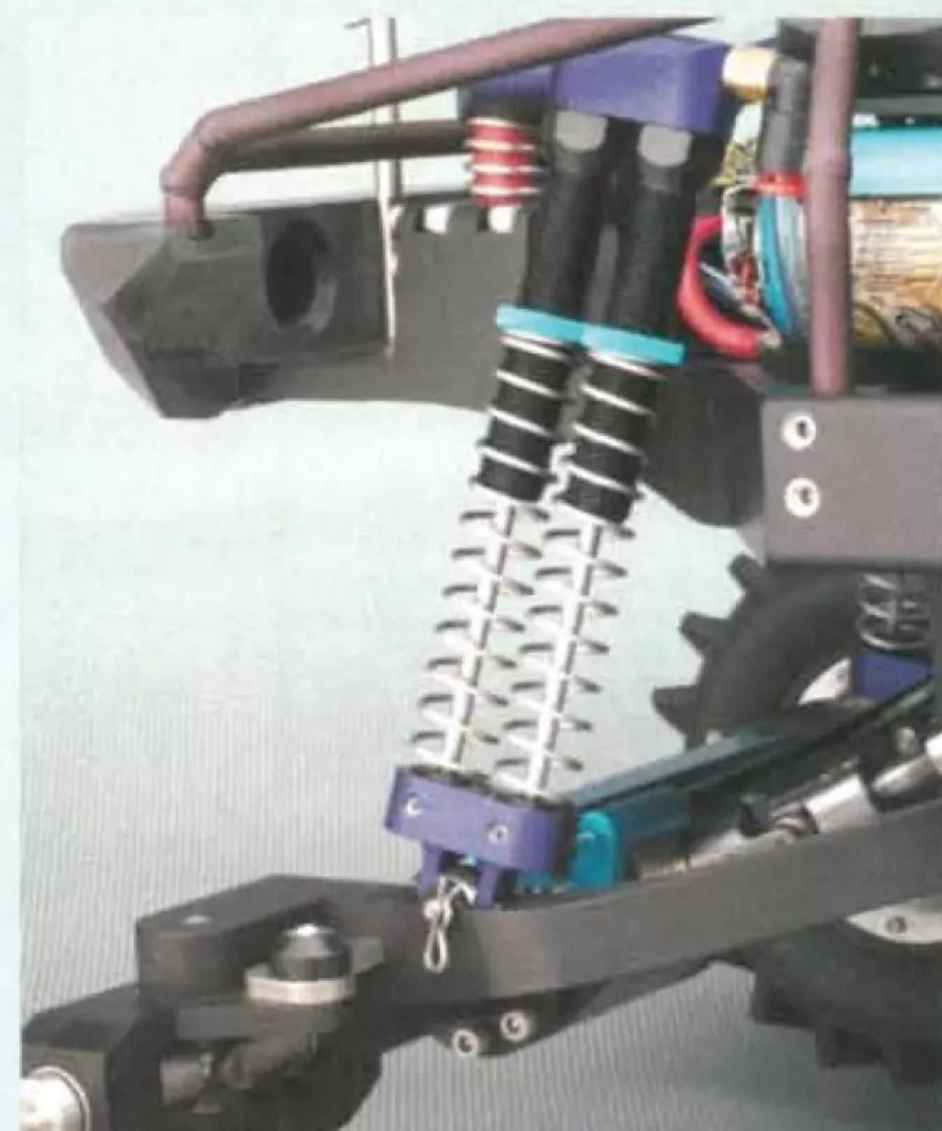
Two shocks at each wheel provide enough damping for this heavy truck; damping is adjusted by means of special, one-way valves.
