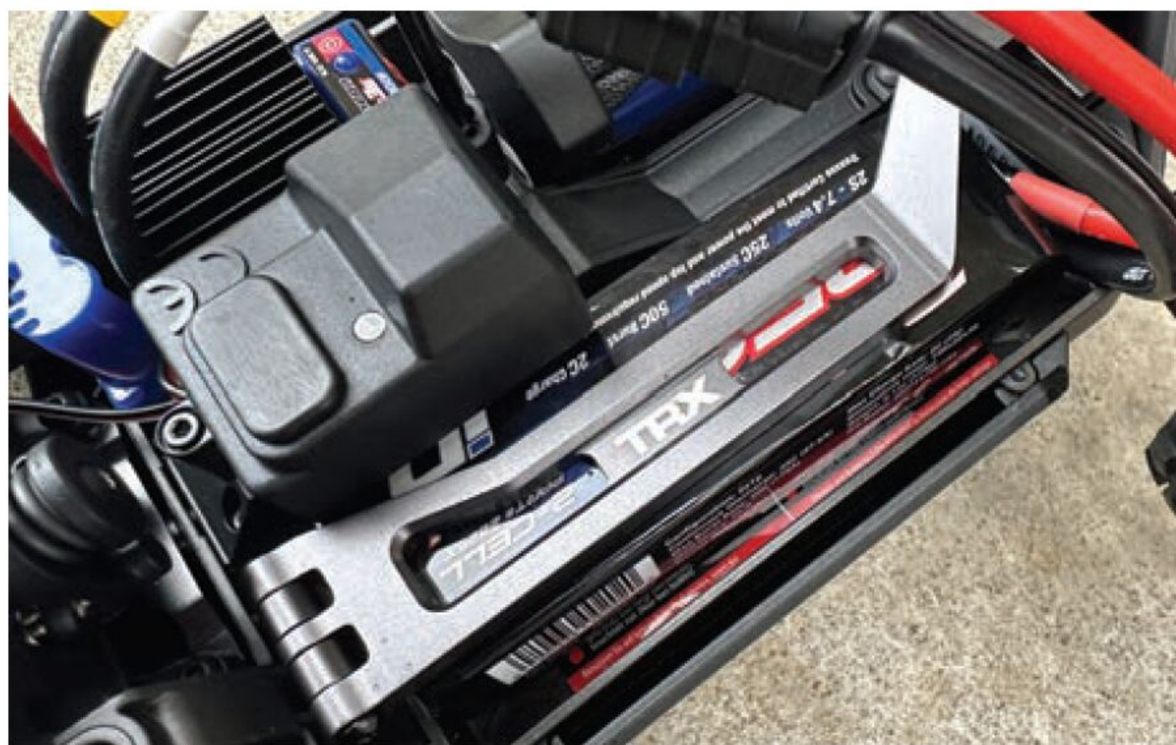
A billet aluminum battery hold-down adds a little bit of flair to the Mini Maxx's underpinnings.
