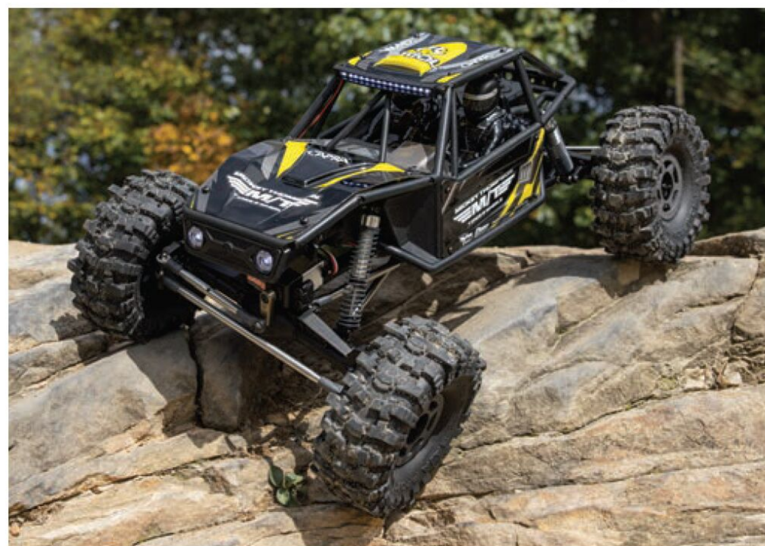
The redesigned, dig-ready transmission features 43% lower gearing for improved technical crawling capabilities.
