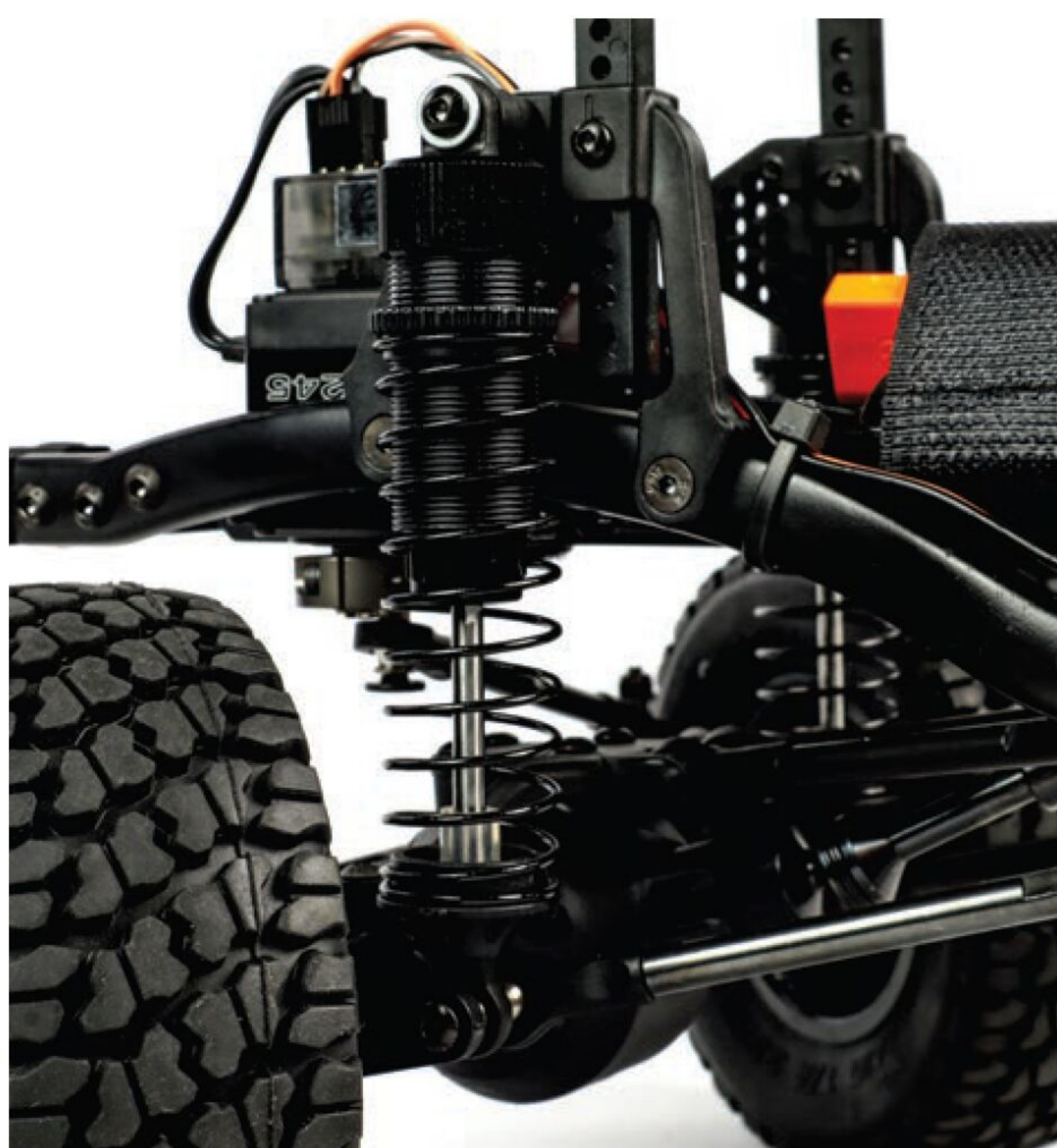
Large-diameter shocks on a trail truck is a little unusual, but they get the job done, and threaded bodies for ride height adjustment is a plus.
