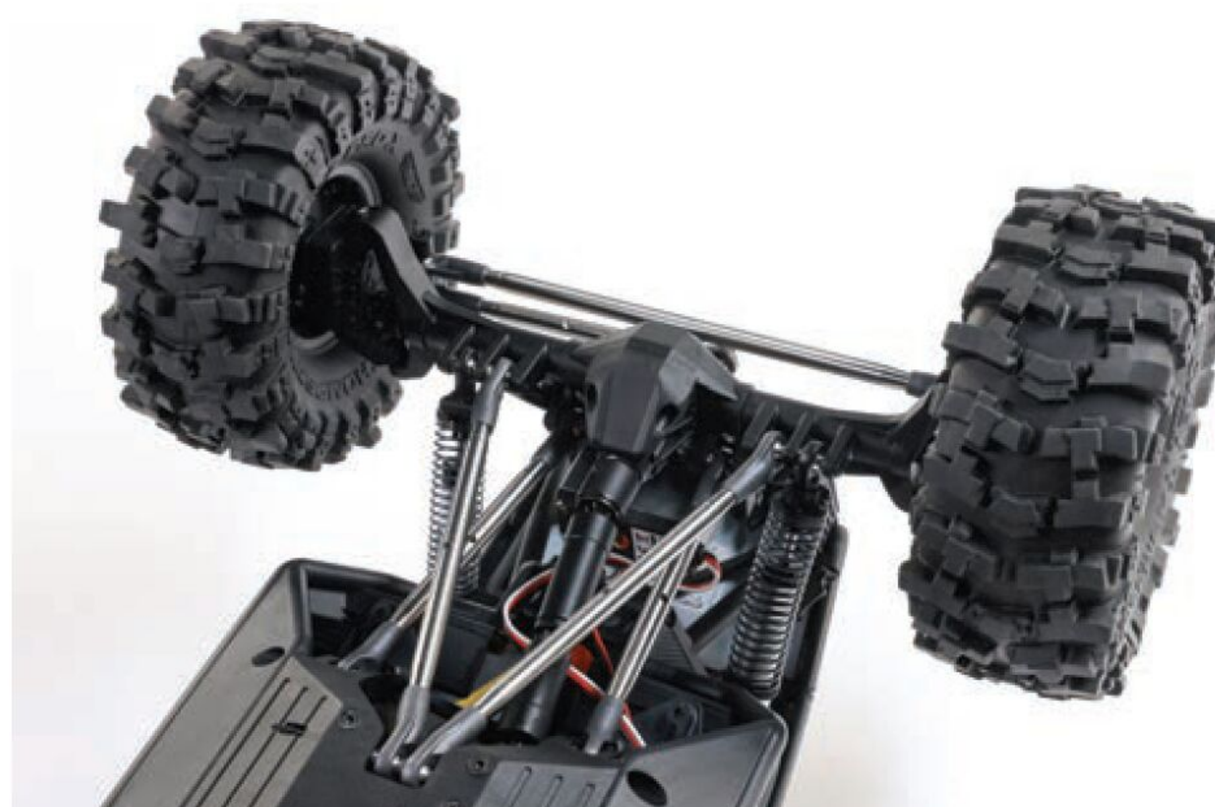
Steering performance has been addressed with the inclusion of a momentary switch-operated 4WS system.
