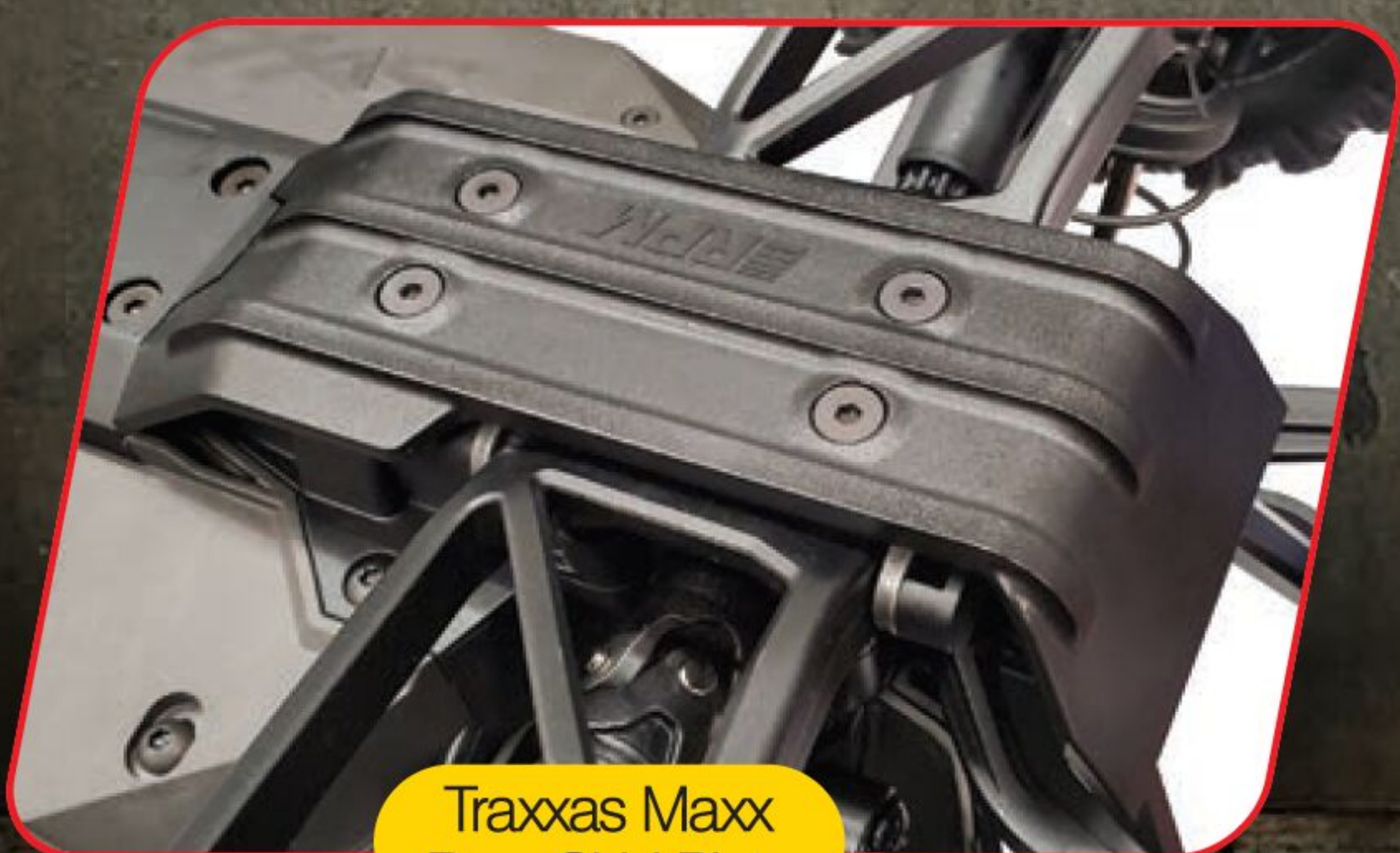
Rear Bumper Mount for the Traxxas XRT
