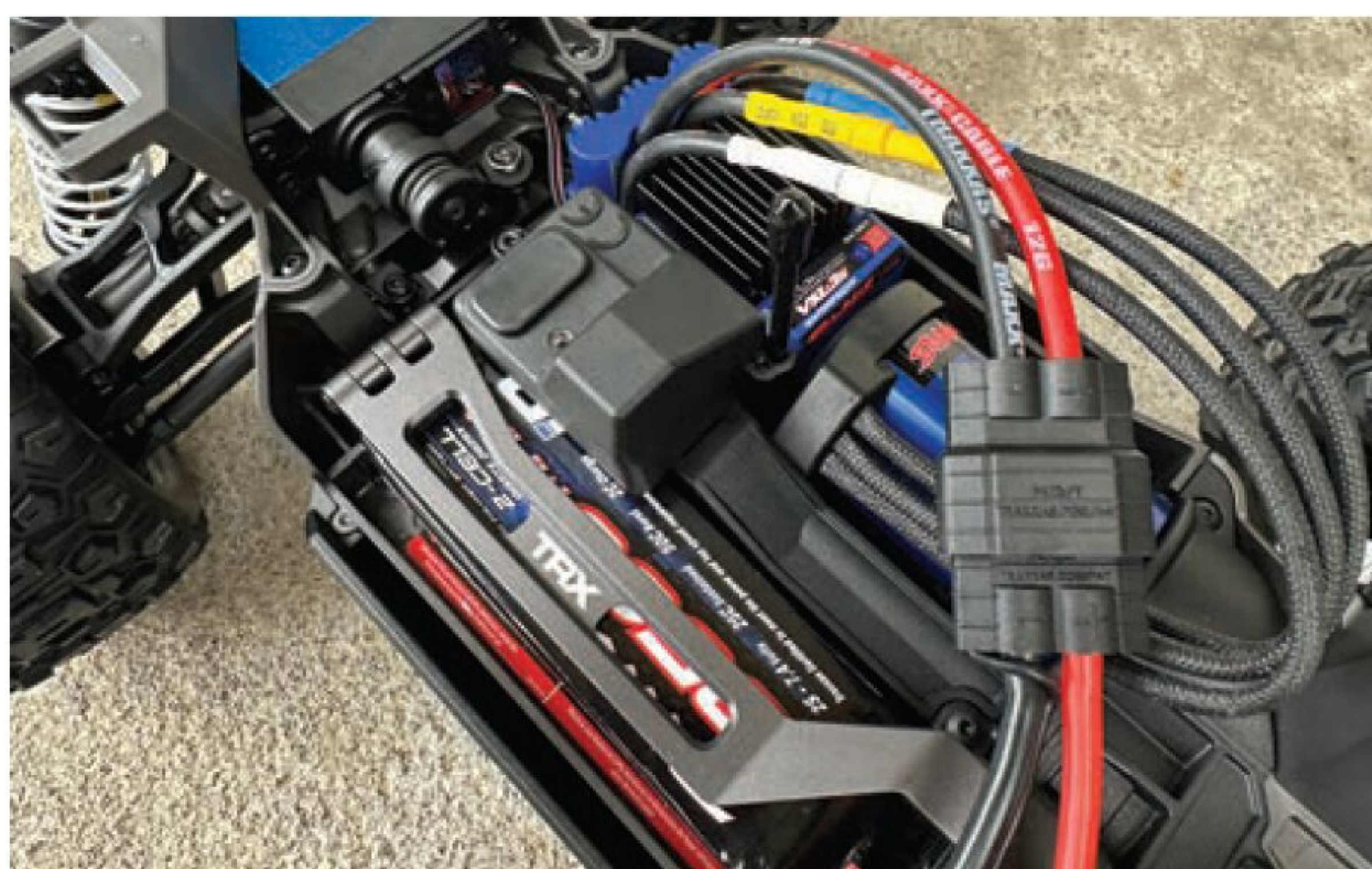
Upgrading to the Velineon VXL-3s Brushless Power System allowed us to run a 3S LiPo for even more power and speed.
