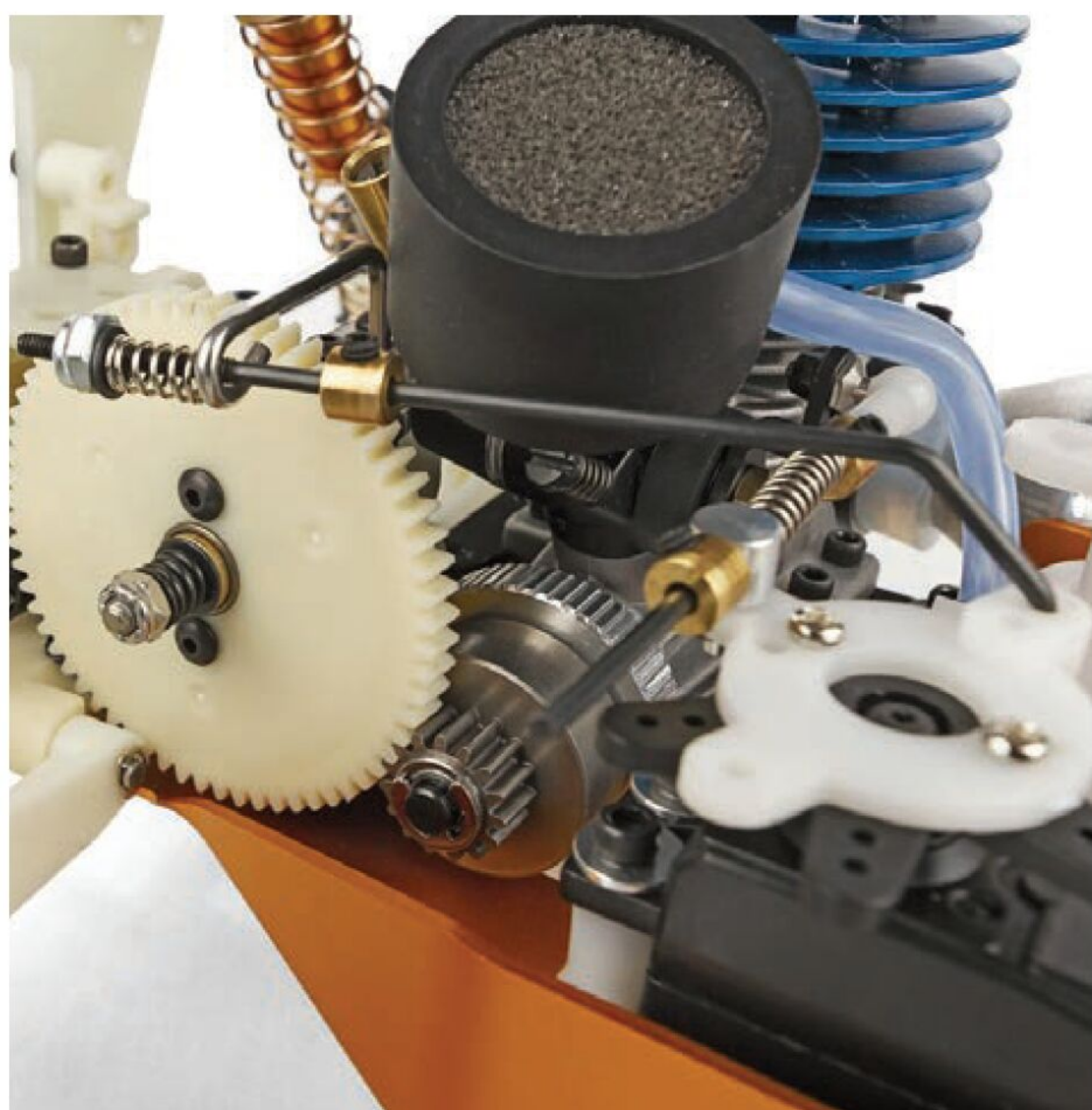
With a 2.6:1 gear reduction, Team Associated's Stealth ATC gearbox is perfectly optimized for the type of gas-powered truck racing that the RC10GT is known to dominate.
