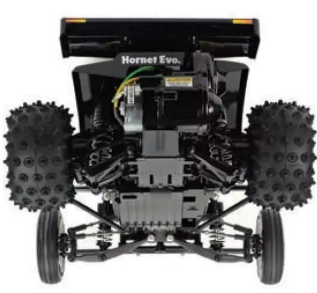
Like the front suspension, the rear also employs CVA oil dampers and upper turnbuckle arms. Dog bone type drive shafts are used.
