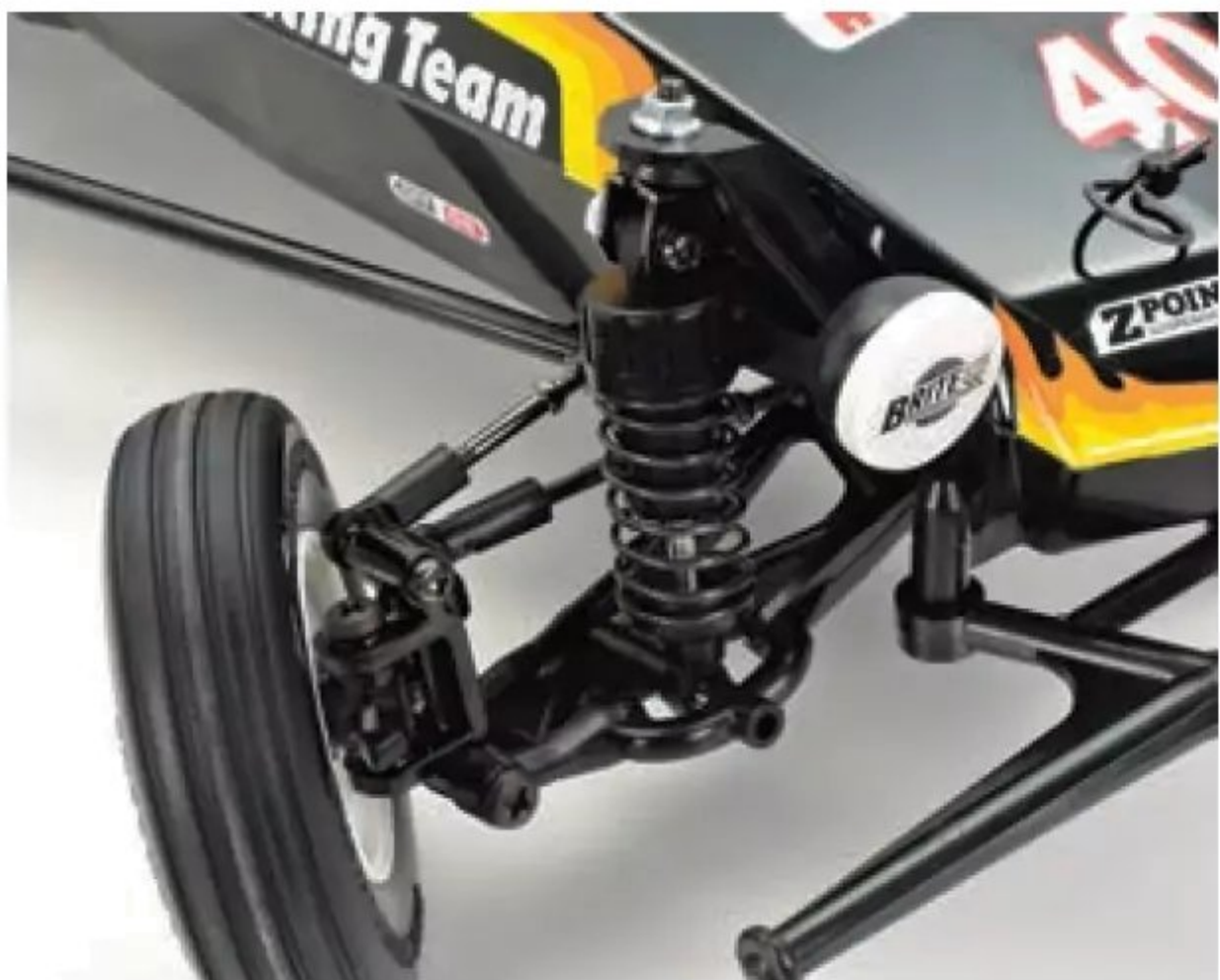
The front double wishbone suspension has turnbuckle upper arms for camber adjustment, and CVA oil dampers that give a great ride.
