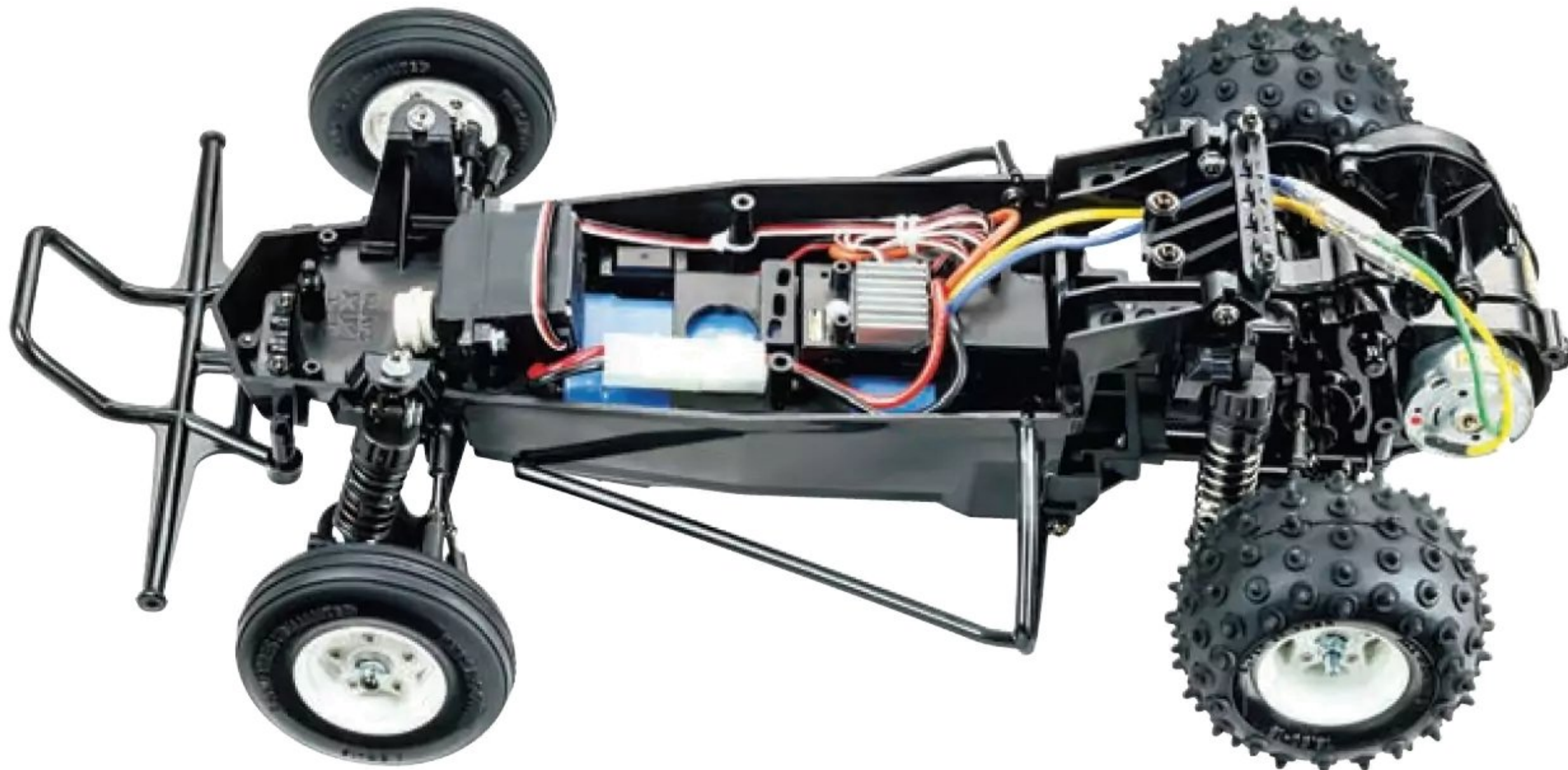
R/C equipment and battery pack are stowed in the sturdy bathtub frame.
