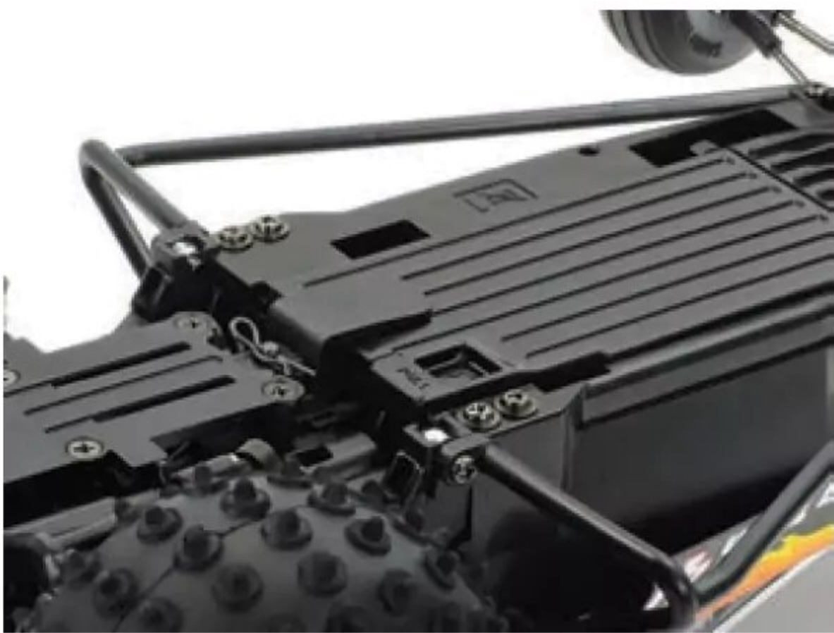
The slim ABS plastic bathtub frame has the battery mounted low, and accessible from the stopper-fixed battery hatch.
