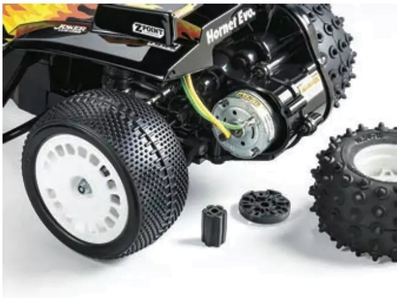
Two types of wheel hub are in the box, letting you attach various types of Hop-Up Option wheels and tires.
