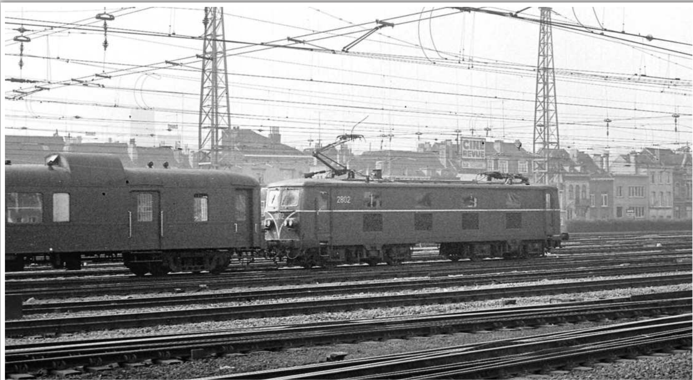
Also introduced in 1949, the three class 28 Bo-Bos (formerly class 120) ended their lives shunting rolling stock. Near the end of its life, No 2802 was seen from a distance at Brussels Midi hauling an empty train out of the station to the sidings. Its original box pantographs have been replaced by a modern single-arm variety. The type lasted until 1996. The class number 28 has since been reused for a batch of Bombardier Traxx locomotives. COLIN BOOCCOCK
