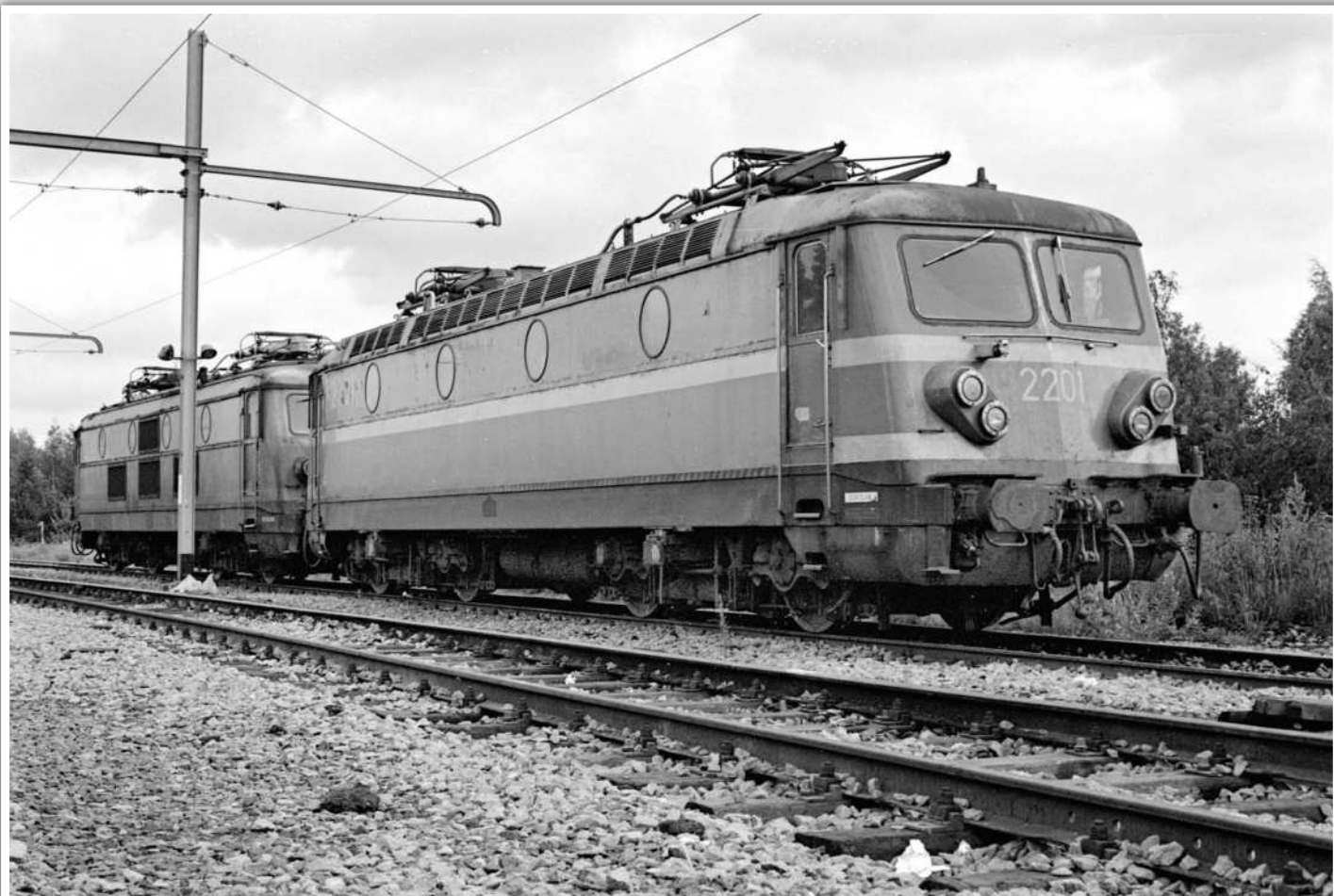
No. 2201 was the first of a class of fifty locomotives introduced in 1953 at which time it was numbered 122.001. These formed the basis of the standard SNCB fleet that expanded in the next dozen years to 155 locomotives. Other classes were variations on this theme of a basic mixed traffic Bo-Bo. It is pictured outside the former railway museum at Leuven in summer 1996 at about the time it was set aside for preservation. The museum later moved to the more public location of Schaerbeek, near the first station north of Brussels Nord. COLIN BOOCCOCK
