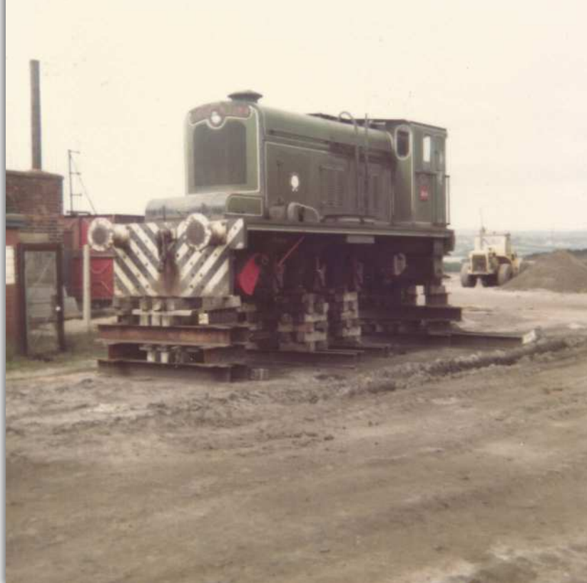
Hudswell Clarke DL4, minus its wheels is resting on sleepers at the colliery in April 1982.
