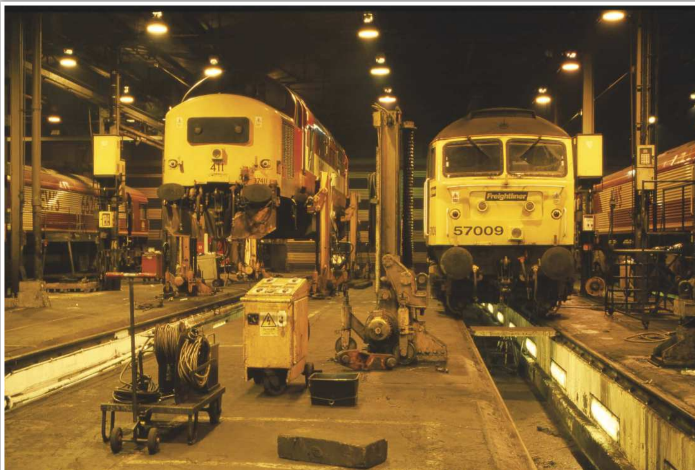
Friday 26th April 2002. Seen inside Crewe Diesel depot 37411 'The Scottish Railway Preservation Society' is undergoing a bogie overhaul and 57009 'Freightliner Venturer' is nearing the end of its stay for fitting of TPWS and long range fuel tanks.
