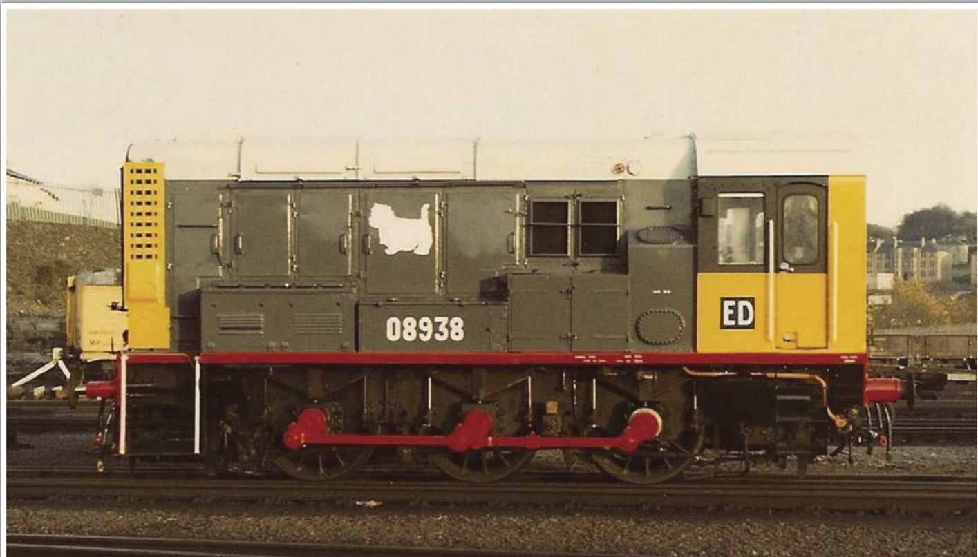
30th November 1985: Freshly painted 08938 at Eastfield; note its very thin tyres which prevented its use in most yards leading to a works visit and full overhaul and a second repaint very shortly afterwards. JOHN BAKER
