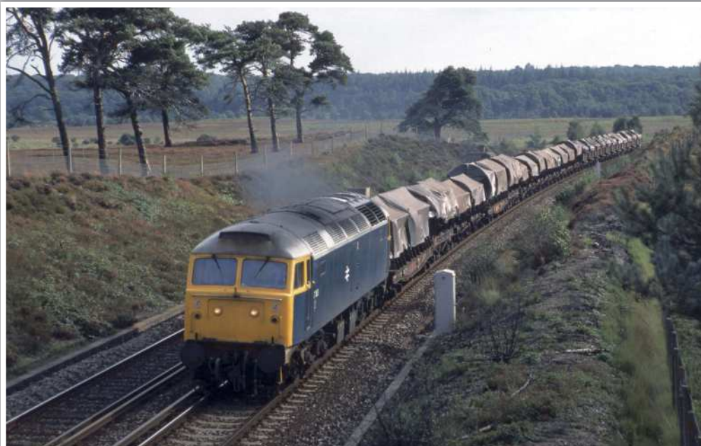
14th September 1984. 47363 is at Beaulieu Road with the 6V99 15:15 Hamworthy to Severn Tunnel Junction steel coil train. The first and fifth wagons are bogie JGV and the second and sixth wagons are bogie BNX, the rest of the train is made up of four wheeled SFV wagons with some shock hood wagons at the rear.
