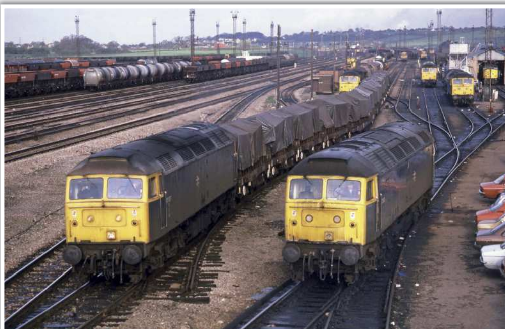
7th May 1986. It is early morning at Severn Tunnel Junction and 47007 is departing with 6045, the 07:00 Llanwern to Hamworthy empty steel wagons. The wagons are a mix of bogie BNX and JGV bogie steel coil wagons (ex-Warflats which have had cradles fitted to hold the steel coils). As can be seen this train doesn't include any SFV wagons. 47348 is the light engine on the right.
