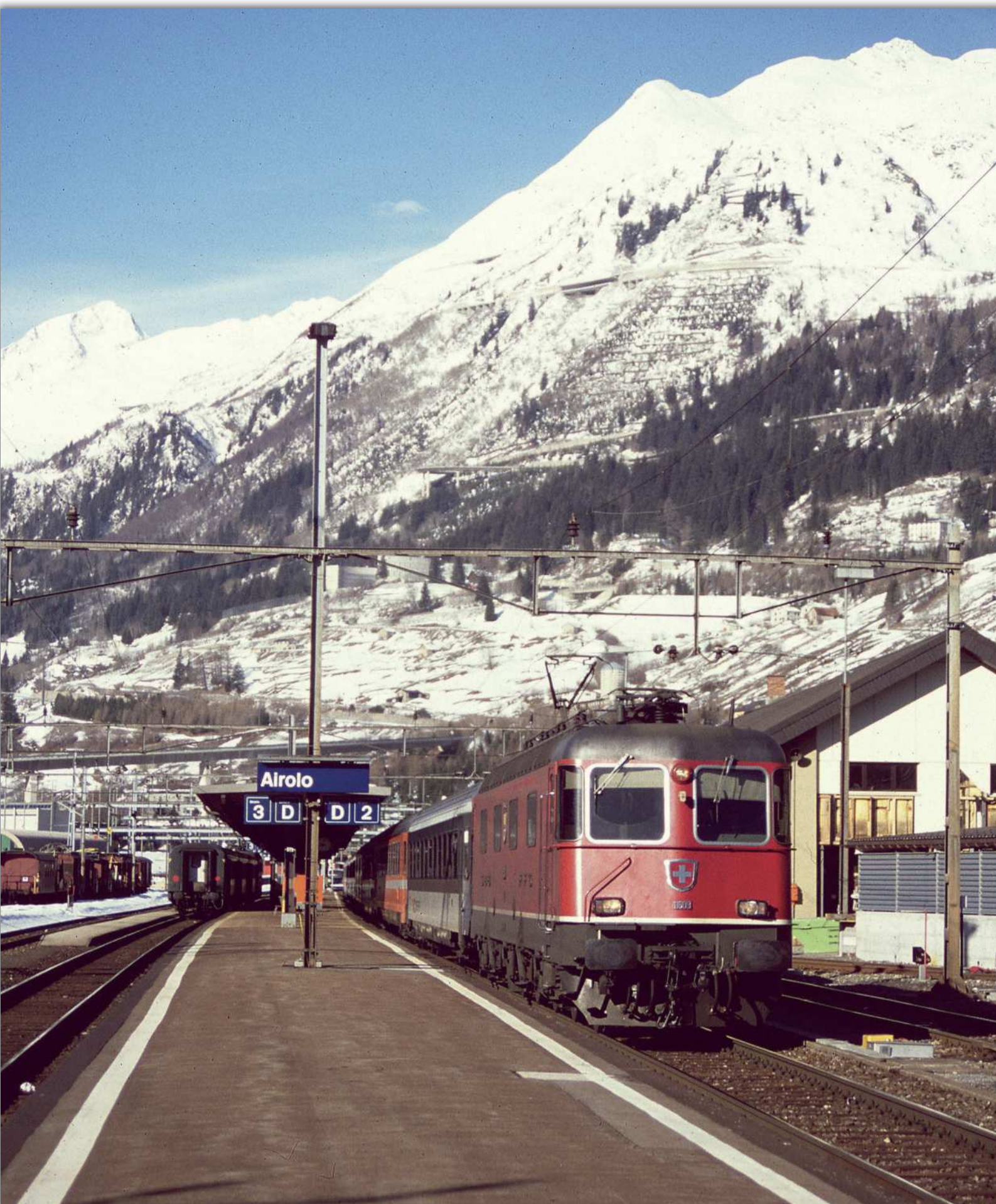
Re6/6 locomotives also work passenger services. No. 11609 'Uzwil' calls at Airolo with the 07.20 from Basel SBB to Milano Centrale on 28th February 1997. The locomotive will be exchanged for an Italian one at Chiasso due to the voltage difference in the overhead line. SBB trains work under 15kV ac, and FS trains under 3kV dc. COLIN BOOCOCK
