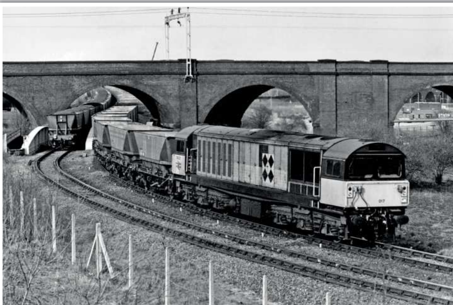
Friday 9th March 1990: The opening of the Oxley Chord in August 1983 eliminated time consuming run-rounds and reversals at Cannock Road Junction for loaded and empty Ironbridge MGR turns. 58017 negotiates the 'chord' at 10:10 with empties and has just passed a loaded train (the former alignment from Cannock Road Junction came in from the left). The viaduct carries the Stour Valley section of the Stafford to Wolverhampton and Birmingham main line from Bushbury Junction. Just visible in the distance through the righthand archway is Oxley Viaduct. The archway to the left of the loaded MGR once gave access to Wolverhampton's Stafford Road steam shed (closed September 1963). ANDY WILLIAMS.
