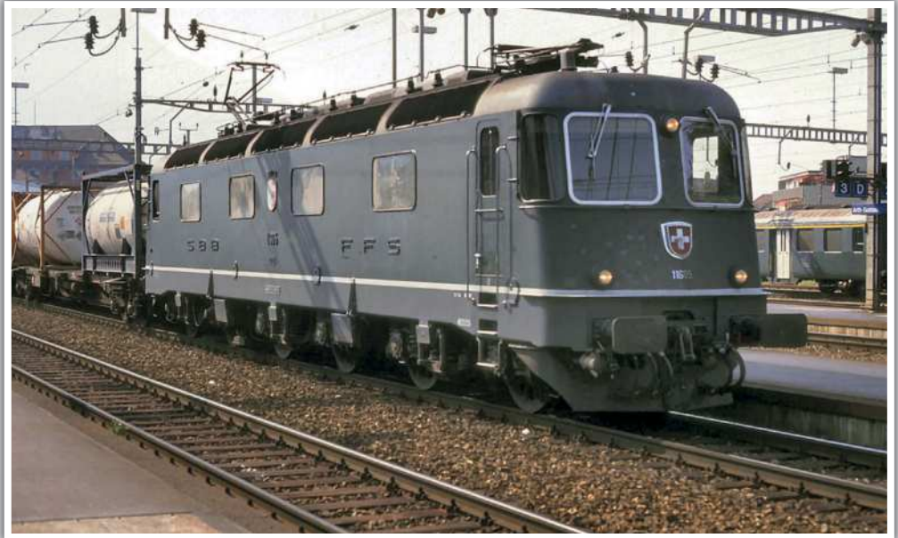
The big brutes of the Gotthard line are the Re6/6 Bo-Bo-Bos. Weighing 120 tonnes and outputting 10,000bhp, they have ruled that route for almost four decades now. No. 11605 'Uster' was seen at Arth Goldau with a southbound freight on 17th August 1988. DAVID FORD
