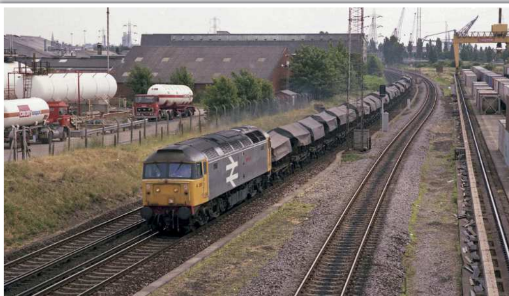
3rd July 1986. Railfreight Grey liveried 47280 'Pedigree' is passing the Southampton Maritime Freightliner Terminal with 6045 the 07:00 Llanwern to Hamworthy steel coil wagons. The train is made up of four wheeled SFV Strip Coil A wagons which will be loaded with imported steel at Hamworthy.
