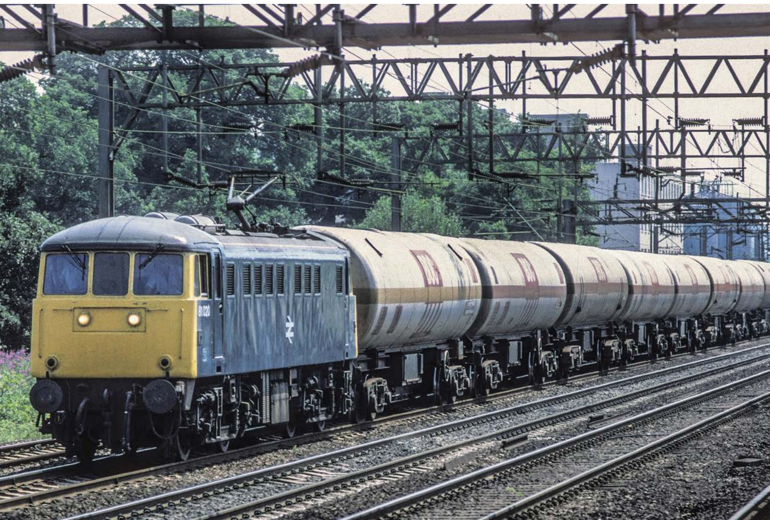
FRIDAY 6TH JULY 1984: After the Woodhead line closed in summer 1981, the only regular electric hauled BOC trains were those from Ditton to and from North Wembley and Polmadie. 81020 heads northwards along the WCML at South Kenton with ten discharged TEA bogie BOC tanks shortly after departure from the North London terminal. By the early 1990s, the North Wembley train had effectively been replaced by an electric hauled service to Ipswich, but even this was being diesel hauled throughout by the time the traffic ended in the mid-1990s. BRUCE GALLOWAY
