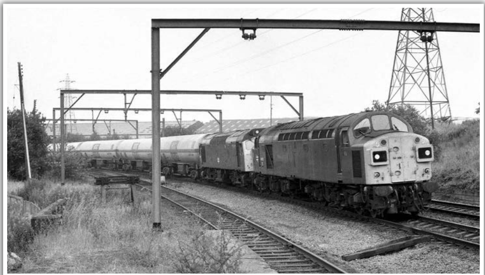
SATURDAY 16TH JULY 1983: Taken from the abandoned platform of Broughton Lane station (closed April 1956), 40131 and 25313 head towards Woodburn Junction as they depart from the South Yorkshire BOC terminal with the return empties to Ditton. Note the de-wired Woodhead electrification gantries at this location, which once allowed cross Pennine freights to be Class 76-hauled to and from the vast Tinsley Marshalling Yard complex, which was very much still active at this time. ANDREW WALKER
