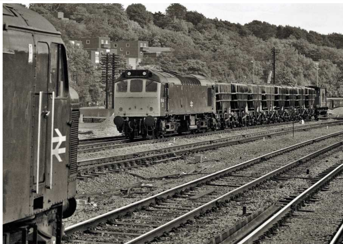
October 5th 1978: 'Peak' 45148 prepares to depart Luton with an express for London while 25183 has charge of a short raft of 'Pres-flo' cement wagons and a brake van for Dunstable. The cement terminal at Dunstable was regularly supplied from Northfleet. However, the cement wagons seen in this view would imply that this was a service from elsewhere and was most likely running as an additional special.
