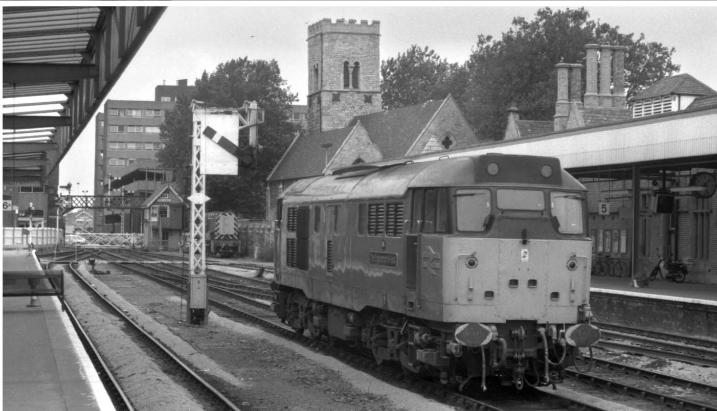
At 13.27 on Friday 31st August 1990, having allowed 31568 'The Engineman's Fund' to advance slowly towards High Street level crossing, Lincoln, the signalman there is about to close the gates and when he's done that, 'pull off' his down starter (no.9) to signal the locomotive away westwards. The original necessity to have the semaphore that the locomotive is about to pass cantilevered out from the lattice metal post, was so that the arm was clear of the 1848 canopy over platform 6 (to the left) and the adjacent track. Once the canopy had been removed in 1956 and replaced by the one seen here, sighting the signal was no longer a problem but oddly, when the lattice post and bracket was taken down (a few years after this photograph was taken), it was replaced by a tubular steel post that was also fitted with a short bracket on which the semaphore was mounted. In the background is Class 08 shunter D3187 put on static display there in April 1989. The precarious positioning of the bench seen on the left was to prevent passengers walking to the west end of platform 6 that was out of use on the day this photograph was taken.
