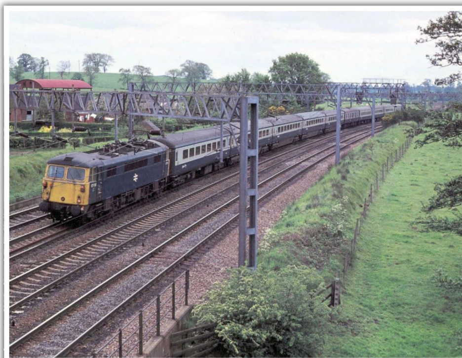
(RIGHT) A typical northbound West Coast Main Line express heads through Norton Bridge a few miles north of Stafford behind 87018 in May 1976. The '87s' were delivered new without four character headcode panels, which made identifying trains much more difficult. During the night hours the Class 87s were used almost exclusively on Freightliner trains as they were only fitted with air brakes. JOHN FORD
