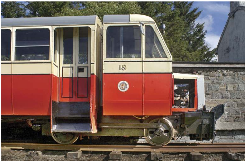
This side view of the power bogie of preserved Walkers CDR railcar No 18, standing at Fintown on the Finn Valley Railway heritage line on 8th May 2011, shows the way the carriage body rests on the rear section of the bogie. It also shows the side coupling rods that transfer the drive from the front axle to the rear one. The rest of the assemblage is a bit like a road bus!
