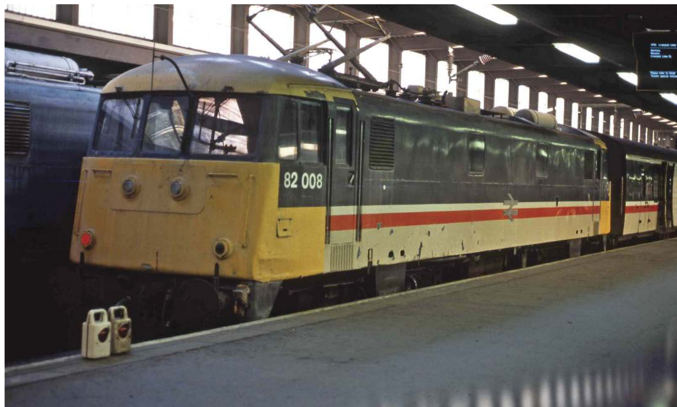
82008 was the first locomotive to be fitted with a prototype National Radio Network (NRN) handset, with the aerial being clearly visible above the cab in this view at Euston on April 21st 1987. The author was involved with the production of a training film about the NRN. JOHN DEDMAN
