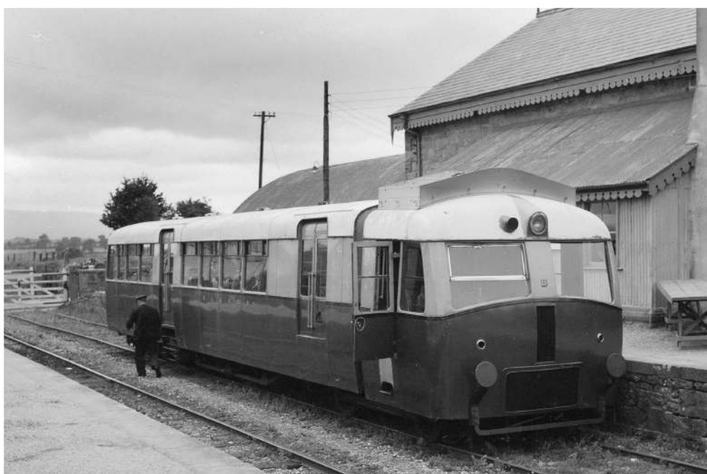
Probably the most advanced of the Gardner-Walker railcars is former Sligo, Leitrim & Northern Counties Railway railcar B, seen waiting at Belcoo in July 1957 for passport and customs formalities to be completed during a border crossing. This car had a second driving position in the rear of the passenger saloon, so did not need turning at journeys' ends. From its introduction in 1947 it shuttled twice daily between Enniskillen and Sligo until the railway closed at the end of September 1957. Since sold to CIÉ and used until 1971, it is now kept as an historical relic and was moved to the Downpatrick Steam Railway in 2005. That group see its restoration as a daunting project in view of serious corrosion, so it is likely to be a long time before we can see this running again.
