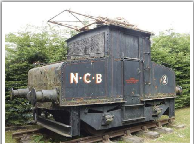
The first electric locomotives for the Harton railway system were delivered between 1908 and 1913 from Siemens, Germany. They were of at least two types, some being small four-wheeled locomotives like No. 2. This locomotive is now on display at Beamish Museum. The similar No. 10 is at the Tanfield Railway. R.L. KITTERMAN
