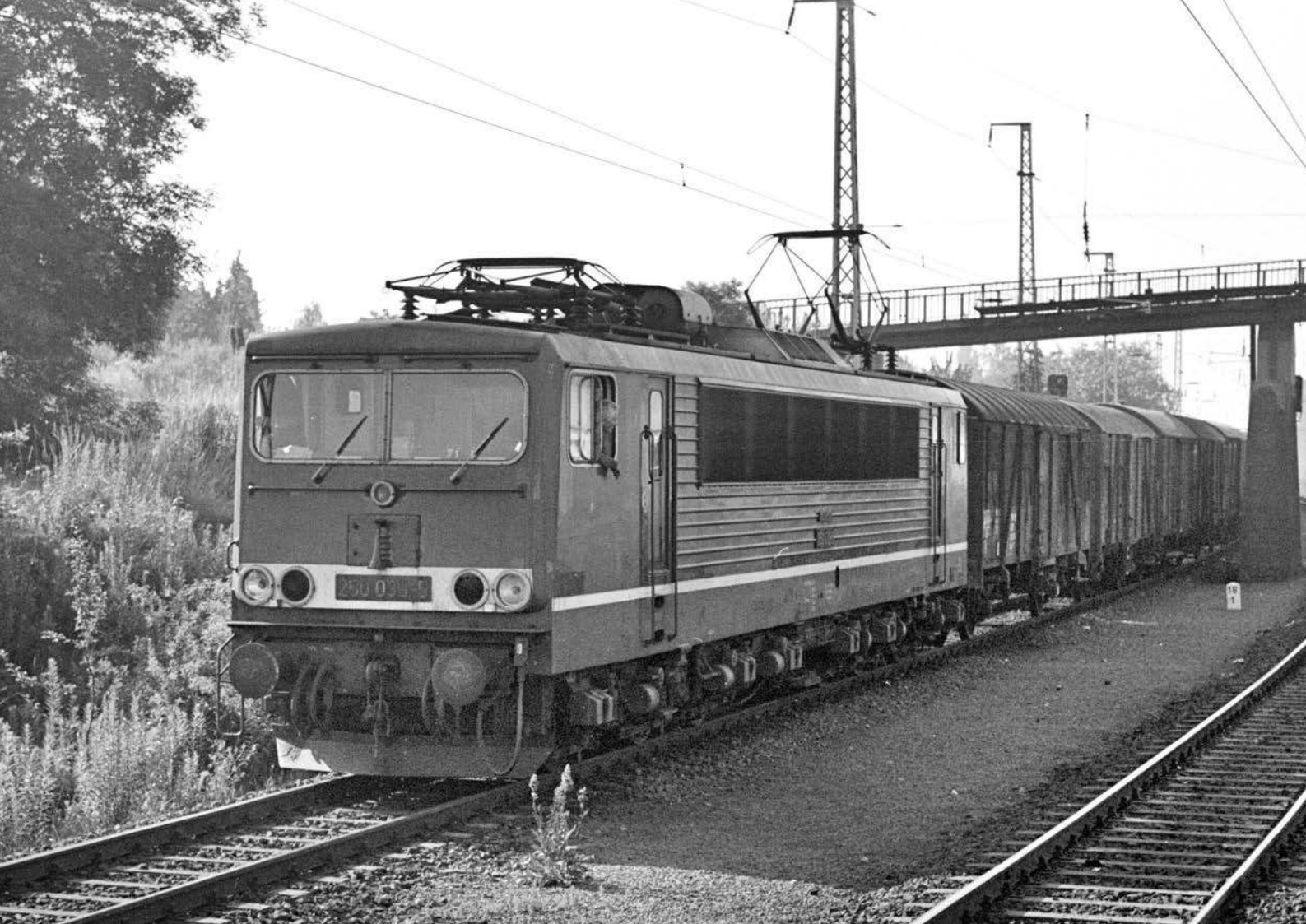
The East German standard freight Co-Co was the Class 250. Photographed from a train on an adjacent track, Co-Co No. 250 039 was approaching Dresden on the 5th July 1989 with a freight, doing what it was designed to do. This class had a maximum speed of 78mph which also enabled them to haul express trains on DR tracks as well as freight. The class became 155 at reunification as they could not adopt the 150 series of numbers because of the clash with the DB class. COLIN BOOCOCK
