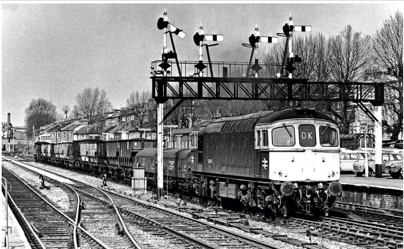
Tuesday 24th February 1976: Nicely framed by the signal gantry, 33057 passes Kensington Olympia with 8010, the 12:59 Acton to Plumstead coal turn, which was due through Kensington Olympia at 13:20 and booked to reach Plumsted around 14:15. Note the two RTV brake tenders positioned behind the loco, quite a common feature of traditional block coal trains traversing the WLL during the 1970s, which could also see their inclusion on such workings to Chelsea Basin Goods and Wimbledon. BRIAN MORRISON.
