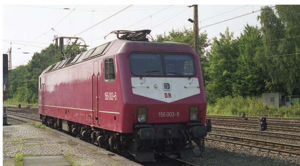
The Class 252 was an updated 250 with three-phase traction motors. Four prototypes appeared in 1991 and after reunification became DB Class 156. On 3rd August 1994, No. 156003 has just arrived at Reichenbach with a Dresden to Karlsruhe Inter City train and is being replaced by a diesel locomotive. The 156s are now in private ownership with Mitteldeutsche Eisenbahn Gesellschaft (MEG) which operates them on freight trains on the DB network. STEPHEN RABONE
