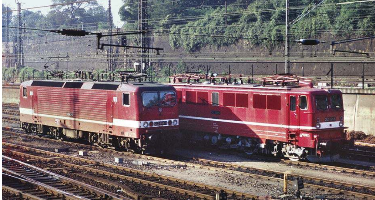
Two Deutsche Reichsbahn Bo-Bo electrics are seen stabled outside Dresden Hbf in 1992. On the right is 242 001, the first member of the earliest post-war DR freight electric locomotive of Class E42 that later became 242 under DR and were reclassified as 142 by Deutsche Bahn. The locomotive was built in 1963 and is now preserved. The 142s could also be seen on passenger work since speeds were generally not high in the East Germany. On the left is the newer standard mixed-traffic Bo-Bo 243 846, of a type that, after the reunification of Germany, spread across almost all of the country, running then as Class 143. Both are in the standard DR red livery. COLIN BOOCCOCK
