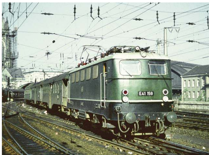
The lightweight Bo-Bo for general passenger train working was the Class E41. Here is E41 159 leaving Köln Hof with a regional passenger service on 29th August 1961. These push-pull fitted locomotives weighed just 66 tonnes compared with the bigger Bo-Bos which were in the 82 to 86 tonnes range.
