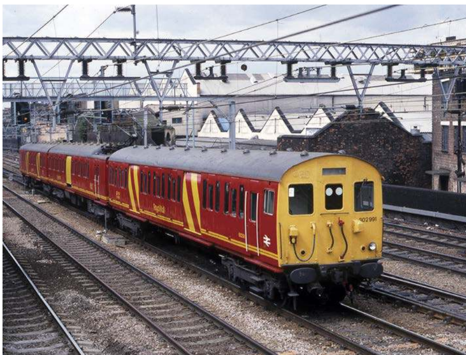
Looking resplendent in its Royal Mail livery, Class 302 No. 302991 is descending Bethnal Green bank heading for London Liverpool Street station on August 12th 1989. Note the large roller shutters that have been cut in the bodysides and allowed the rapid loading of mail.
