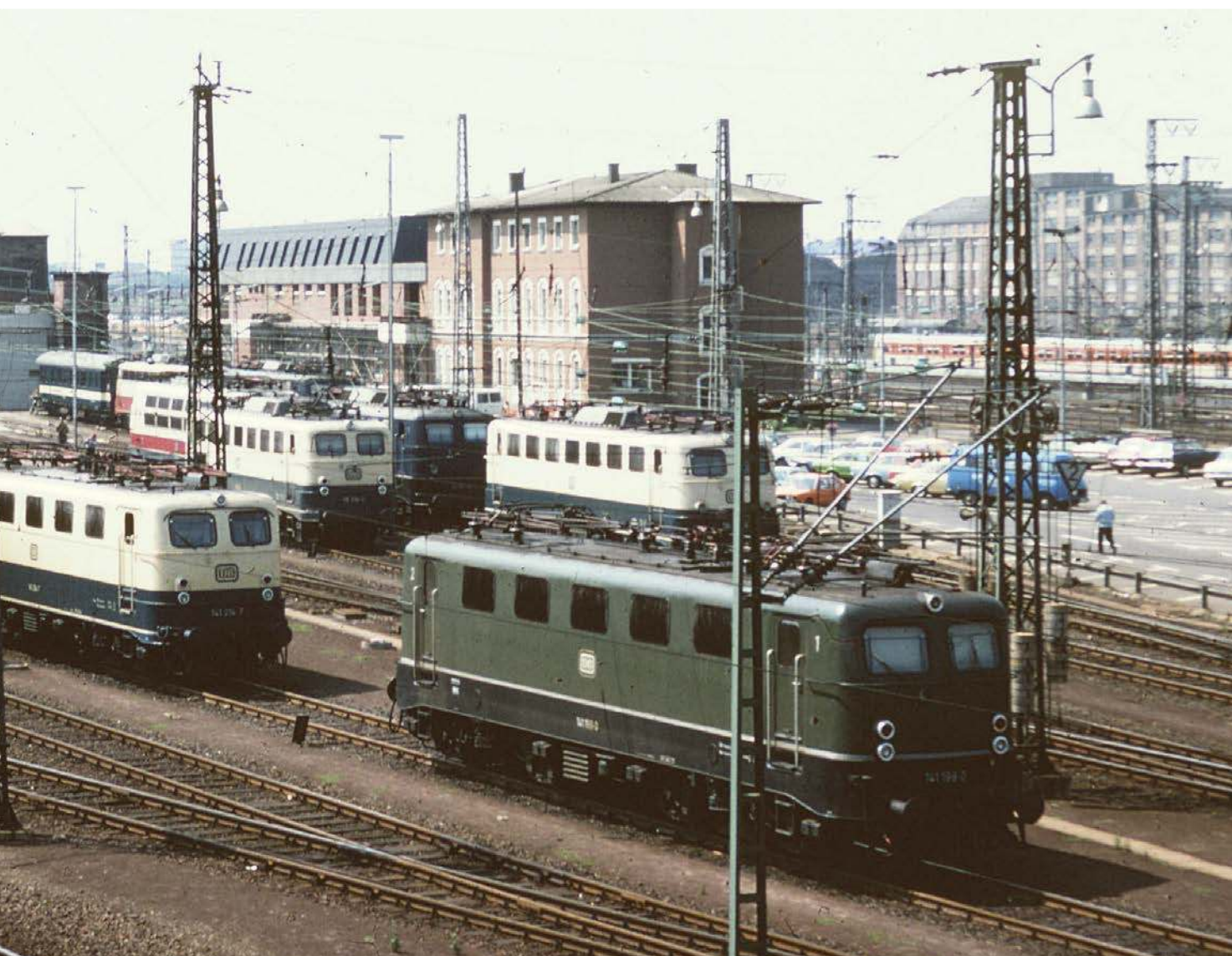
The lightweight Bo-Bo for general passenger train working was the Class E41. Here is E41 159 leaving Köln Hof with a regional passenger service on 29th August 1961. These push-pull fitted locomotives weighed just 66 tonnes compared with the bigger Bo-Bos which were in the 82 to 86 tonnes range.
