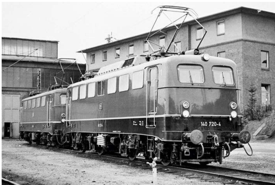
The new standard mixed traffic Bo-Bo type introduced in the 1950s was the E40 class, illustrated here by brand new 140 720 just delivered to Hamburg Eidelstedt depot in August 1968. This later variety had thyristor traction control. The white radiator pipes centrally placed under the body cool the transformer and rectifier.
