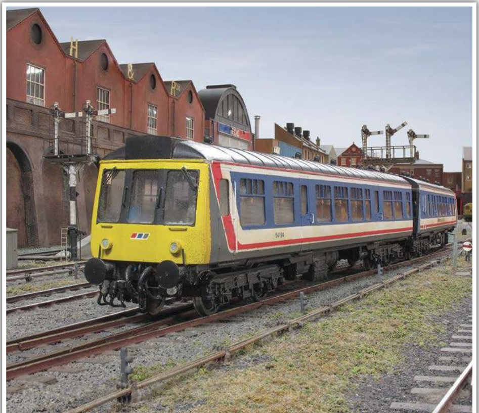
A Class 108 DMU in the darker NSE blue departs for Stratford. This is a Lima '117' model which was reduced to a skeleton and etched brass sides, then available from Craftsman Models, were added.
