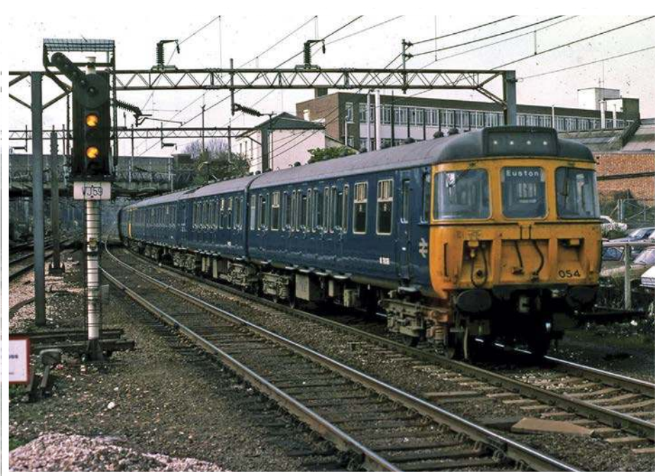
Electric multiple units were used on many outer suburban and long distance semi-fast services such as this Birmingham to Euston via Northampton working. Class 310, unit No. 054 is seen at Watford Junction on 15th April 1977. JOHN DEDMAN
