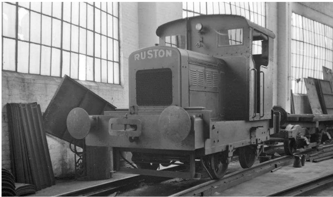
The replacement of 'Lively Polly' was this Ruston standard 0-4-0 diesel mechanical of the manufacturer's type 48DS, seen in 1955 inside the carriage shed at Seaforth Sands. It had a 48bhp Ruston 4YC diesel engine, mechanical four-speed gearbox and chain drive to the wheels. Two locomotives of this type also worked for British Railways: DS1169 at Broad Clyst civil-engineering depot near Exeter, and ED10 at Beeston creosote works. COLIN BOOCOCK
