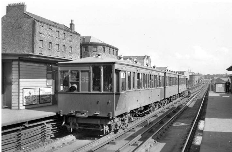
Sixty-two years old and going strong, one of the original electric units leaves James Street station heading south on the Liverpool Overhead Railway on 13th August 1954. The timber carriage bodies are panelled with teak slats, as is the interior together with its wooden seats for third class passengers. Access doors were outward-swinging slam doors, three doors on a third class carriage side, and two doors per side on the first class centre cars.
