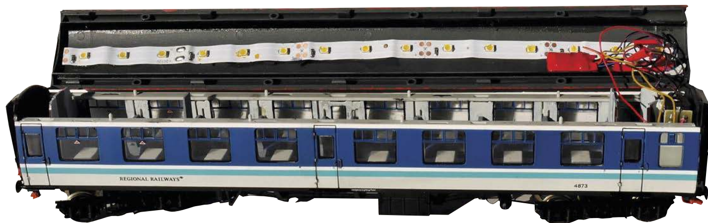
A Mark 1 coach showing the LED lighting strip in the roof and the circuitry used to control the lighting and flashing tail lamp.
