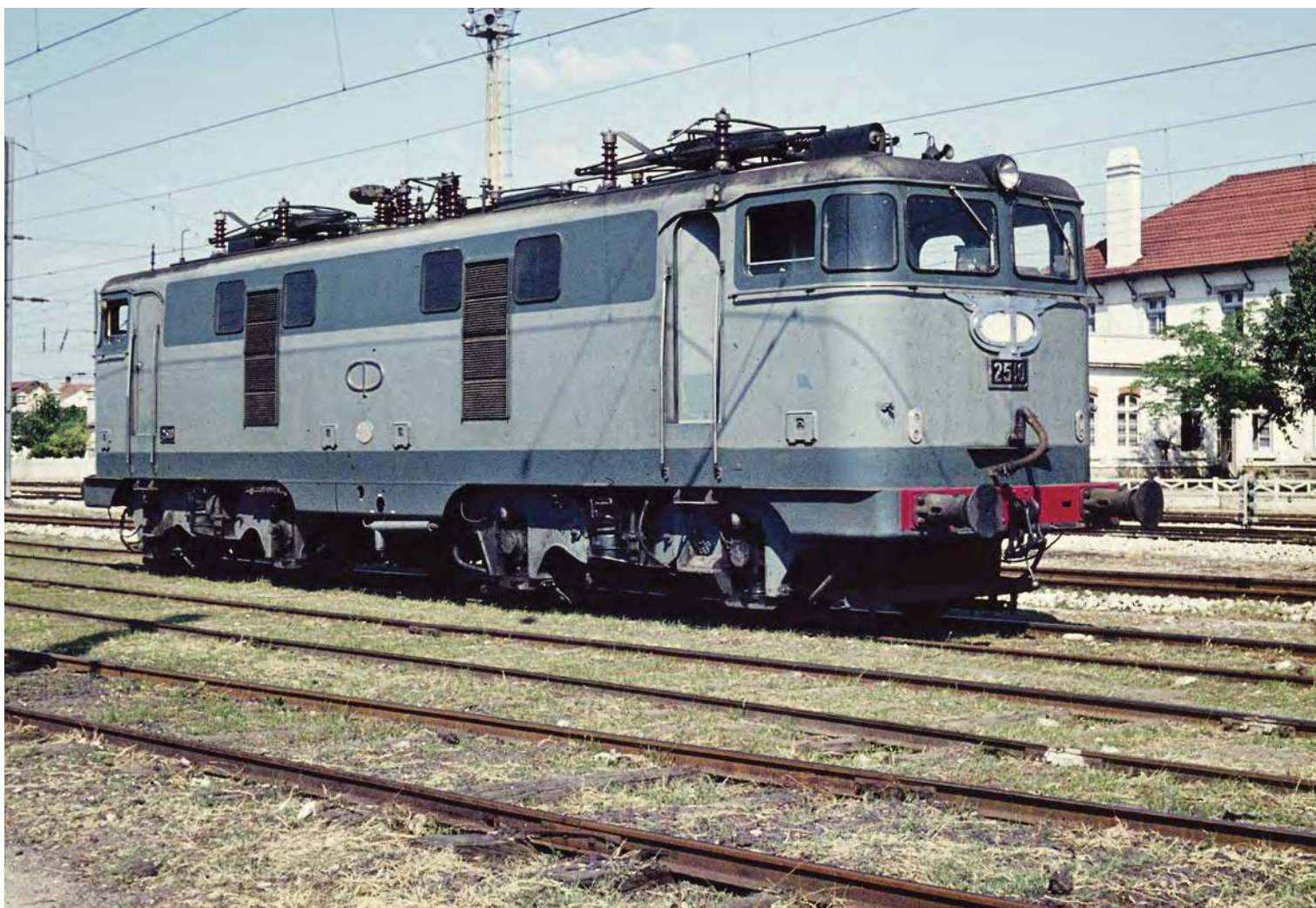
The first 25kV electric locomotives in Portugal were the fifteen Bo-Bos supplied from 1956 by Henschel with Alsthom equipment. This one was pictured at Entroncamento.
