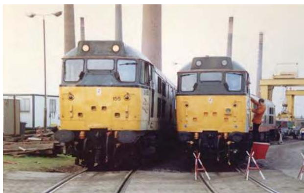
(ABOVE) Trains 6A11 and 6A13 stand on the gantry roads being reloaded with their emptied spoil containers. Note the protection in the form of barriers and a red flag fitted to 6A13, these being employed to prevent any unauthorised movement. The shunter Tony Caines, climbing down from the locomotive is in overall charge of all movements. GRAHAM BAKER
