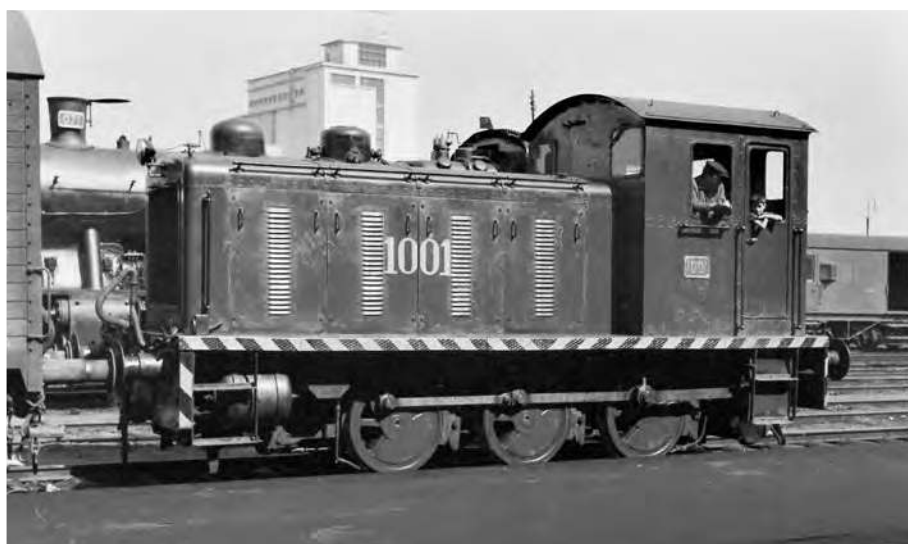
An early Drewry 204bhp diesel mechanical 0-6-0 shunter, No 1001 was shunting at Campanha depot, Porto. CP had six of these. (The domes above the engine compartment actually belong to the Swiss-built 2-6-4T behind.)
