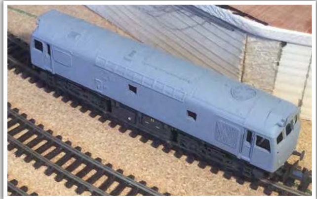
The rest of the original windows were then glued back in place and the body reassembled. Finally the loco and chassis were weathered using Lifecolor acrylics.
