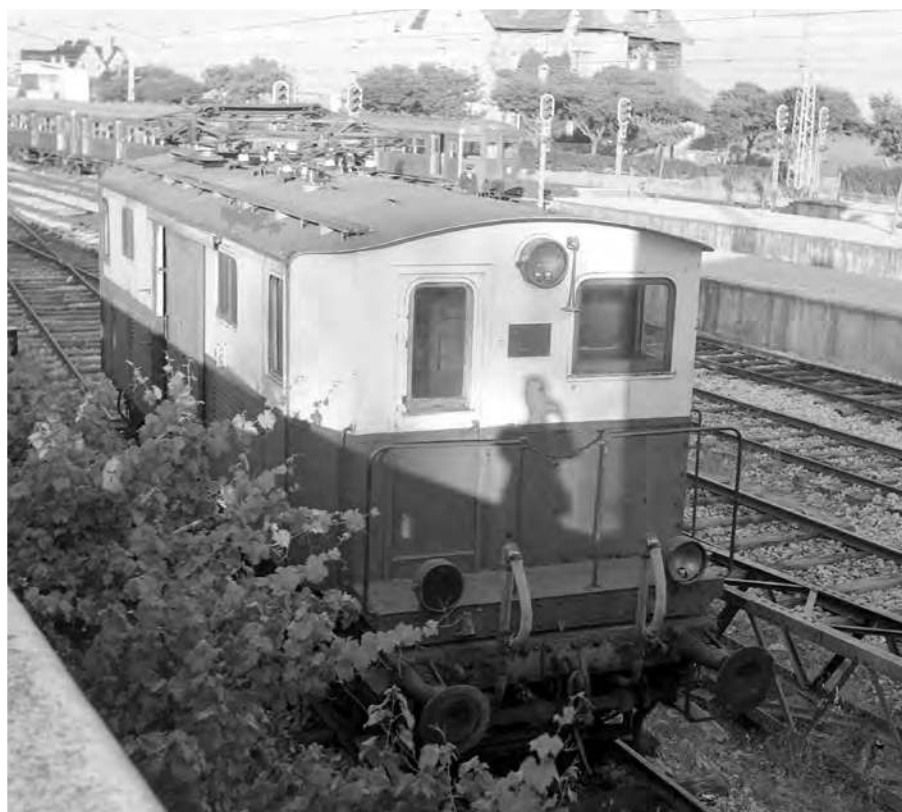
The unique Bo-Bo locomotive-cum-baggage car L303 was stored in a siding at Cascais in 1962 prior to works attention and re-equipping with GEC (UK) traction equipment. No L302 of this type is now preserved in the museum at Entroncamento.
