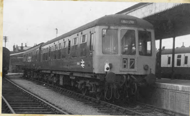
A two car DMU stands in the platform after arrival at King's Lynn from either Hunstanton (closed 1969) or the Wisbech line (closed 1968). The Class 114 Derby driving trailer appears to be No. E56023 and has bars across the door windows. The power car is a Cravens vehicle.
