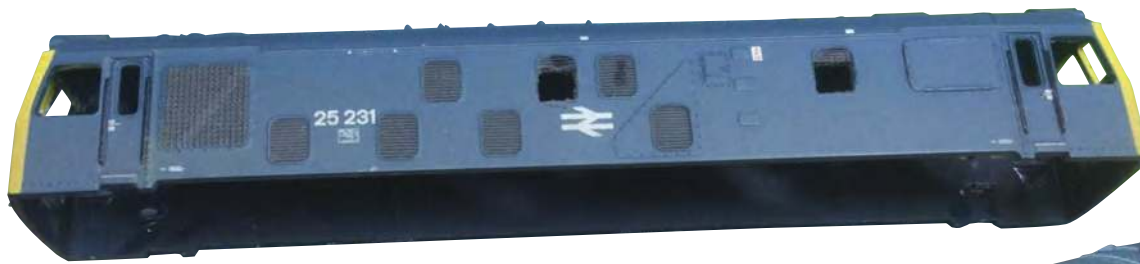
The engine room windows were also cut out using photographs and drawings to find the exact position.
