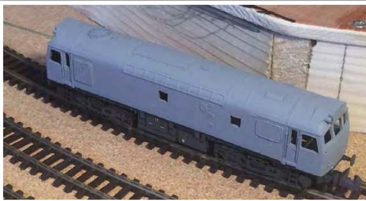
After a wash and brush up to remove any dust, the loco was given a coat of Halfords' grey primer. The photographs show both sides of the locomotive. The cab ends were then painted white followed by a coat of warning yellow. Body sides were painted next in Rail Blue followed by a gloss varnish coat from a spray can.
