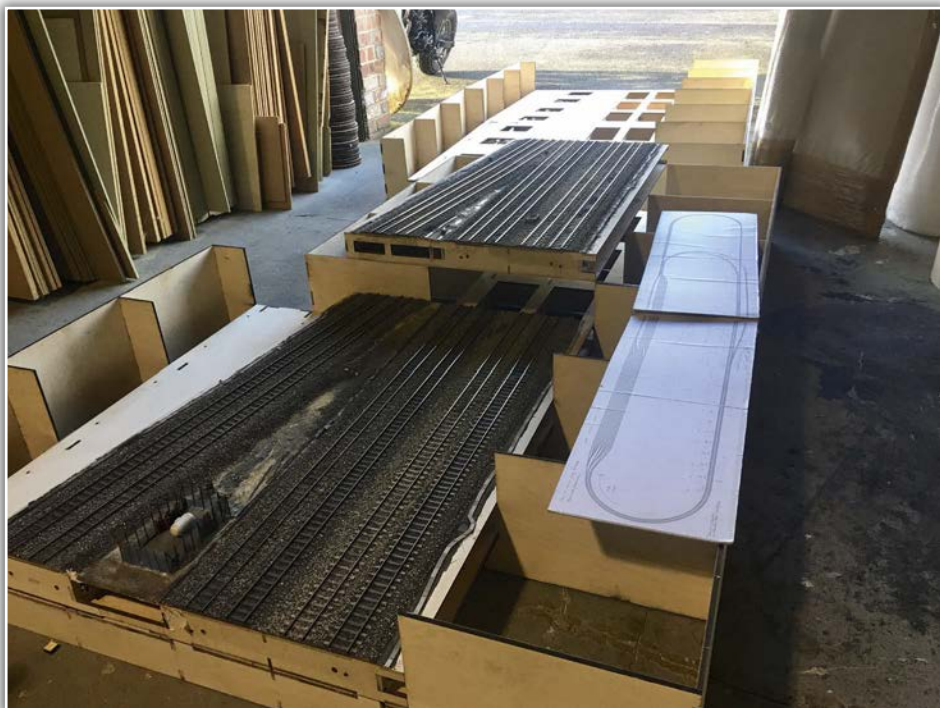
Three frames awaiting collection from White Rose Modelworks (who manufacture them) into which the track cassettes are fitted. These cassettes can be angled very slightly to represent the different gradients present at the real location. The frame furthest away is the most recent and shows how the frames widen to almost 6ft.
