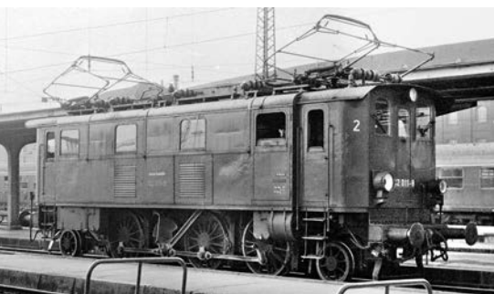
Introduced in 1924, 29 of these E32 1-C-1 jackshaft-driven electric locomotives were built for light passenger services. No. 132 011 was still in use at München Hauptbahnhof in summer 1970, on empty stock workings and shunting.
