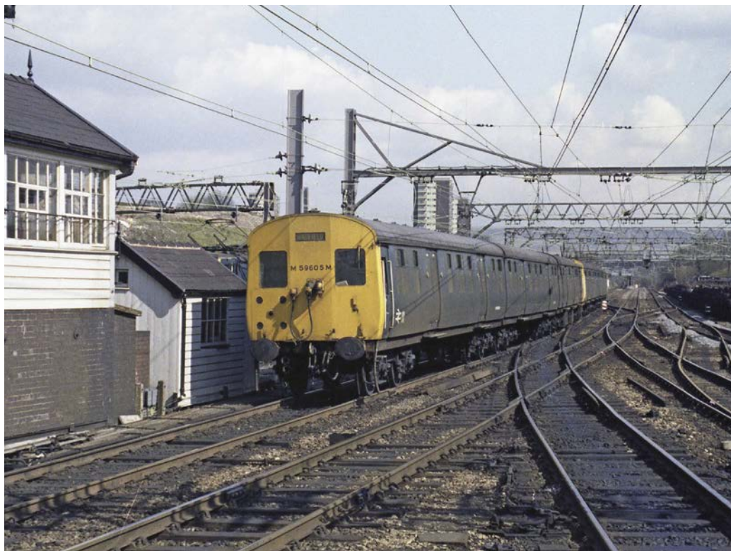
Generally the Glossop line services ran as three car trains but in the rush hours they were sometimes operated as a double set. With driving trailer No. M59605M at the rear, a pair of blue liveried Class 506 units leave Godley Junction with a service for Glossop and Hadfield in March 1983. RAILPHOTOPRINTS.CO.UK - COLLECTION
