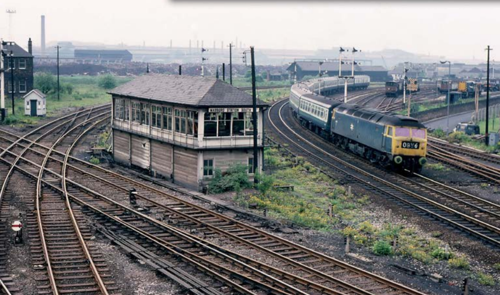
47107 rounds the curve from the Sheffield direction with a Cross Country train to Newcastle. The locomotive was seen later in the day so possibly it only worked this train as far as York. The size of Masborough signal box with its four bays is an indication of how many levers the box had. It opened in 1903 and closed in 1979 as a result of the Sheffield area resignalling scheme. Over to the right are Masborough yards which at this time provided work for at least two Class 08s. In the distance are scrap yards and steel mills that stretch as far as the eye can see.
