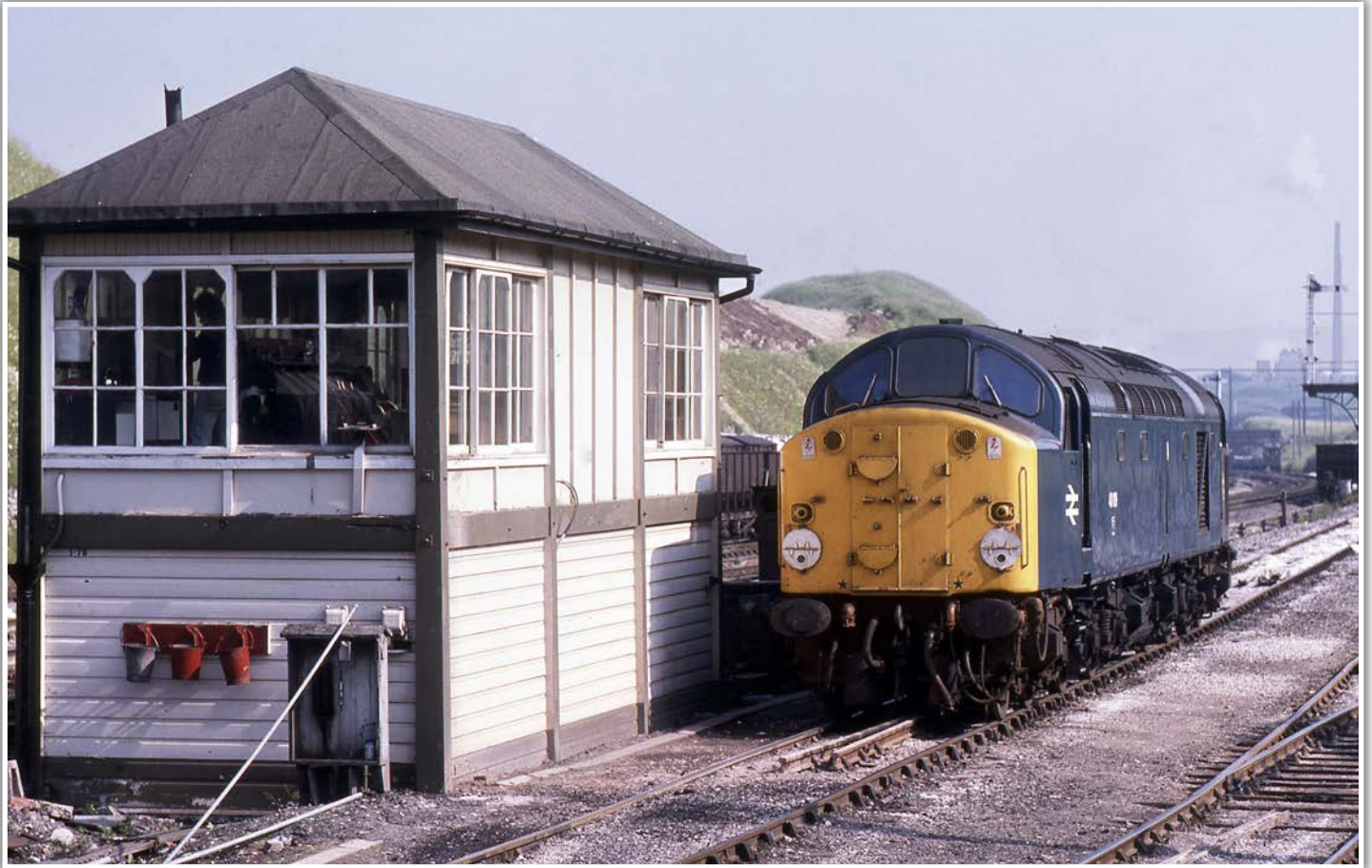
No. 40109 stands alongside Peak Forest South signal box on 3rd July 1979. A signal box had opened here before 1877, but was replaced in 1891 and again, with the one in view here, in 1925. The box was reframed in July 1974 and still stands today working absolute block to Great Rocks Junction in the south and to Chinley power signal box in the north. GAVIN MORRISON
