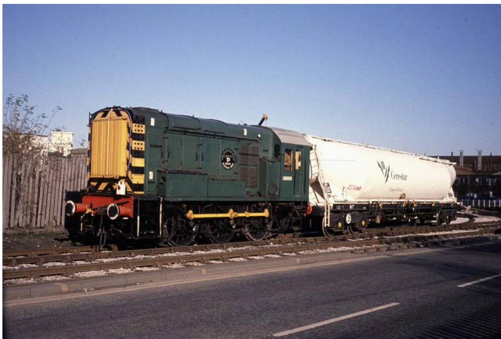
ABOVE: The Trafford Park Estate Co. purchased a couple of Class 08 locomotives to work their traffic between the industrial estate and Trafford Park Sidings. In November 1989 No. 08669 heads through 'The Park' with a starch wagon which was eventually destined for the Wiggins Teape paper mill at Corpach.
