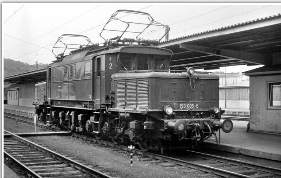
DB's Co-Co freight locomotive 193 005, one of the first batch of the E93 series introduced in 1933, was seen at Ulm Hauptbahnhof in the summer of 1970. DB painted both the E93 and E94 classes in green with black bogies.
