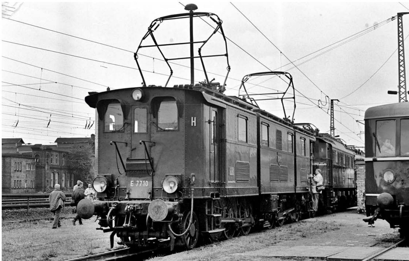
ABOVE: The exhibition at Halle depot in May 1995 included some preserved and really rare old-timers such as this 1B-B1 machine, No. E 77 10. Of 2,520bhp, these locomotives were introduced in 1924 and had Swiss electric motors driving a jackshaft in each bogie, using connecting and coupling rods to drive the wheels. The body was in three sections, allowing it to slightly articulate to ease forces on curves. There was an equivalent heavy freight design of 1926 laid out as a C-C, which lasted in service on DB until the 1970s, one of which, No. 191 099, is preserved.
