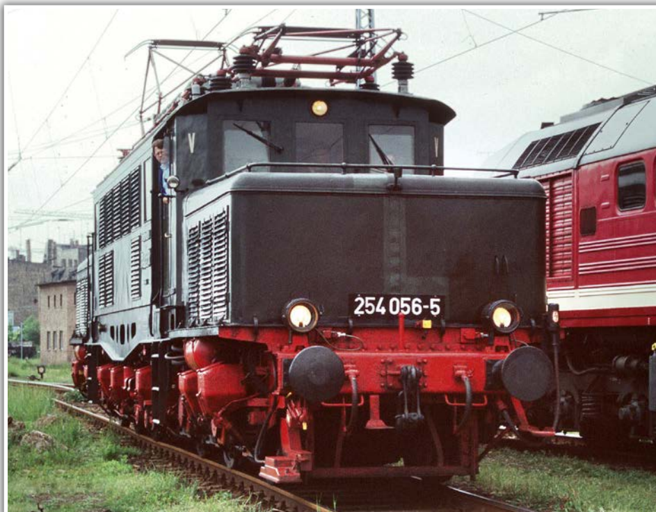
The DR renumbered the E94s in the 254 series and painted them green with red bogies. No. 254 056 was on display at Halle in May 1995, and shows the deeper side frames adopted for the majority of this type. The 'V' on the cabside denotes the vorder or leading cab. The one at the other end was marked 'H' for hinter or rear cab. Across the border, DB had numbered the cabs '1' and '2' respectively.
