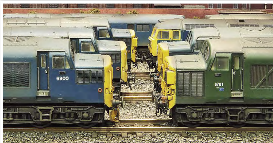
6900 was unusual as at this time it was not only painted in Rail Blue but also fitted with snowploughs and radiator frost grills as seen here facing another EE Type 3, green liveried 6701. ANDY YORK
