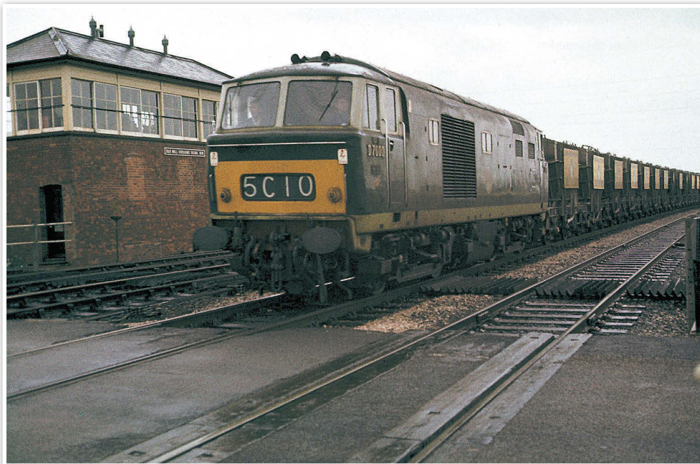
D7000 is seen at Taunton Silk Mill Crossing with a westbound train of Blue Circle presflo cement wagons in August 1966. By this time the horns have been relocated to the cab roof. JOHN FORD
