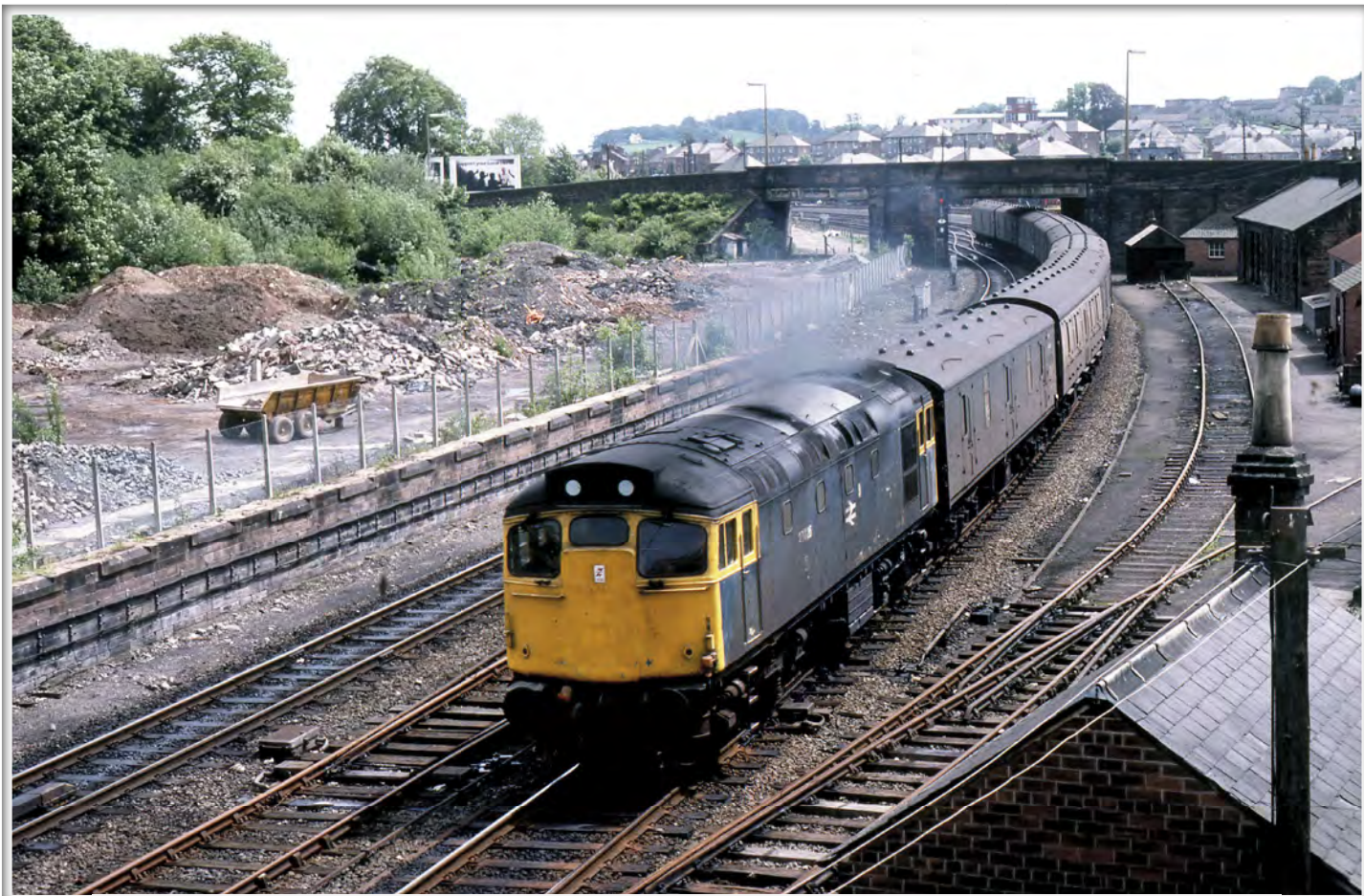
Seen from St. Mary's Street bridge Class 27/0 No. 27026 is approaching Dumfries and runs under Annan Road bridge on a northbound van train. This is probably the Euston to Stranraer service which passed through Dumfries in the early afternoon. The demolition site on the left is consigning the remnants of the former Dumfries locomotive shed to history. The date is 9th June 1983.
