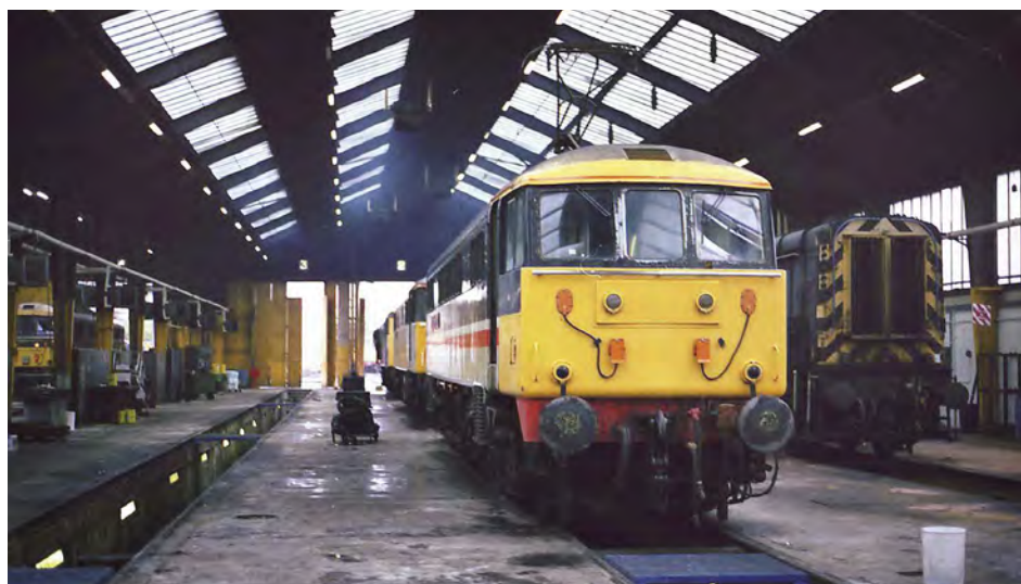
Three electric locomotives and a Class 08 diesel shunter await duty inside the running shed at Willesden traction depot at about the time the Total Quality project was under way. The nearest locomotive is a Class 86 with its pantograph raised in readiness for service. GAVIN WRIGLEY
