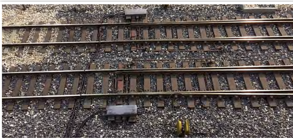
Pointwork details: the Westinghouse point motors were scratchbuilt from original Westinghouse (now Siemens) drawing as they were unavailable off the shelf whilst the track circuit detectors were also scratchbuilt and the cables are correctly attached to the rails. SIMON GEORGE
