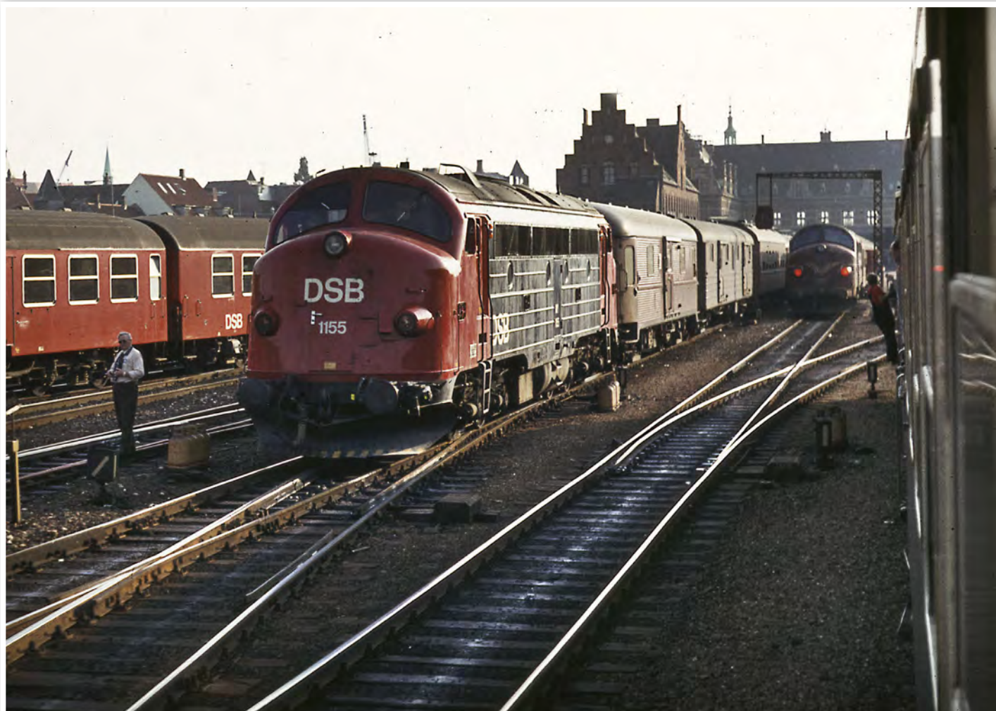
More powerful were the 16-cylindered Class MY A1A-A1A locomotives, also of the NOHAB 'streamlined' design. No. 1155 was photographed in 1980 shunting stock onto the ferry at Helsingør ready for the short crossing to Helsingborg in Sweden. By the time of the author's visit in 1988 these locomotives had been relegated to freight workings.
