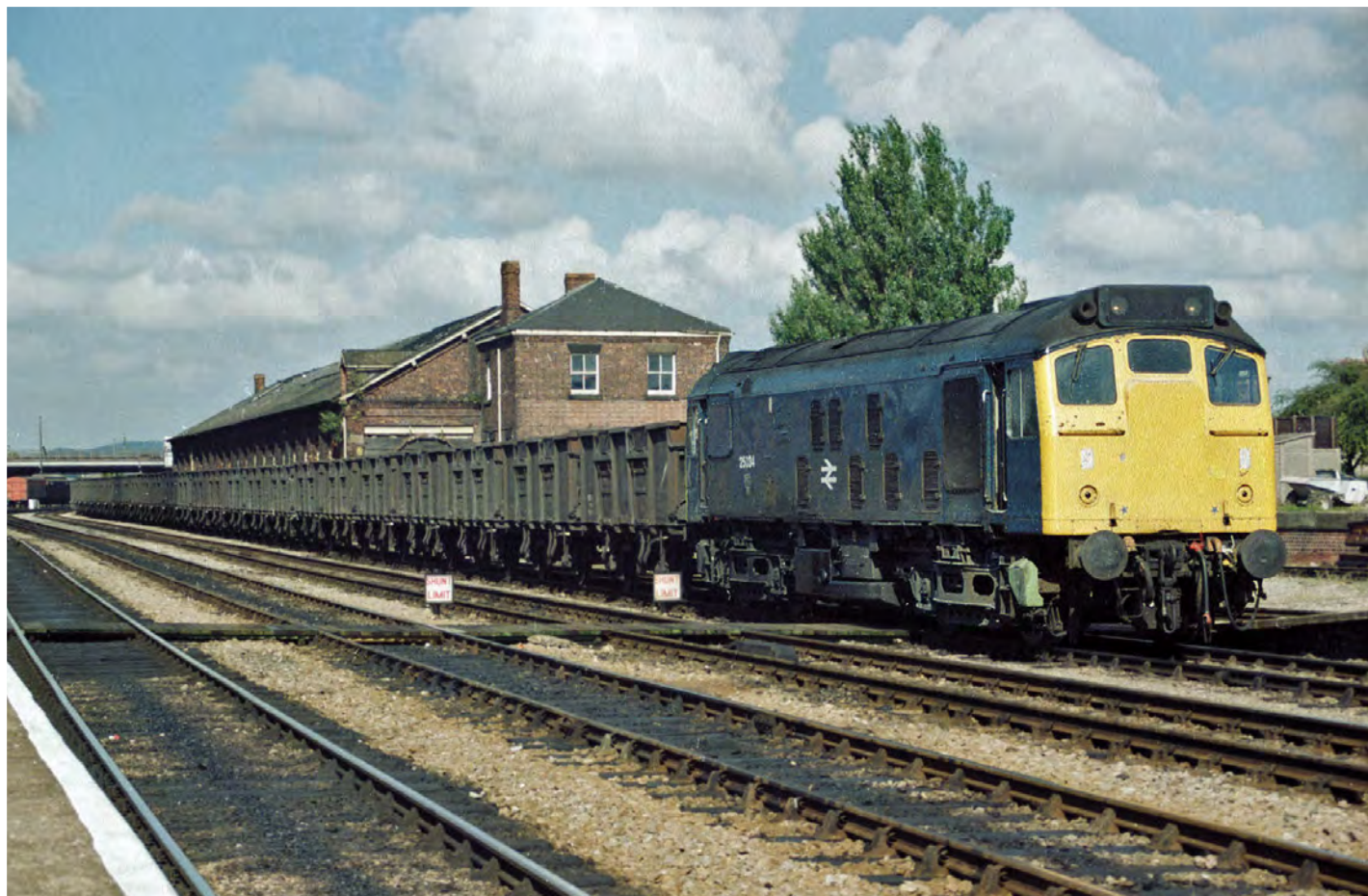
Thursday 18th September 1986: Coking coal from the North Staffordshire area was dispatched to the South Wales steel industry via the N&W using vacuum-braked wagons. Class 25 No. 25034 is seen at Hereford with what appears to be a lengthy raft of MDV type 21-tonners.
