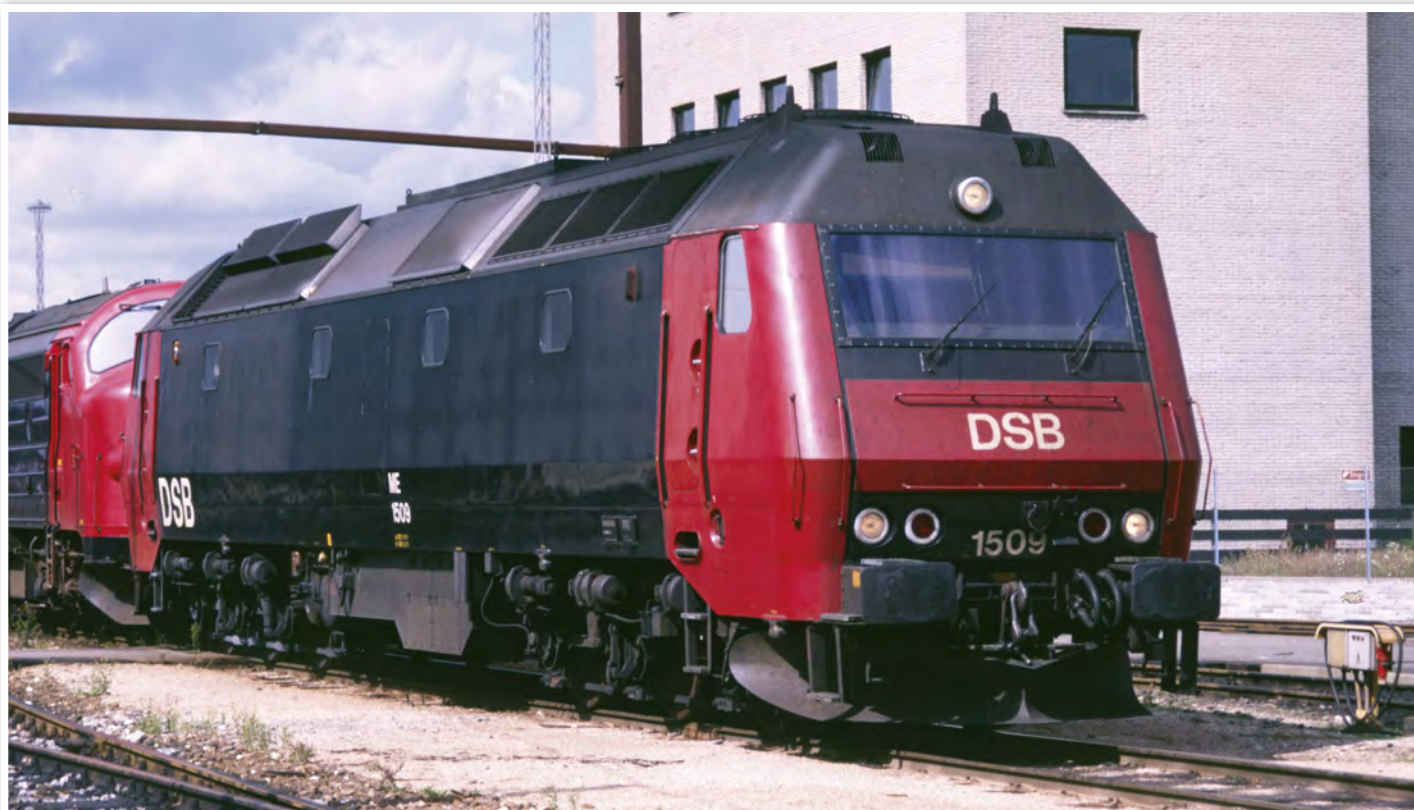
More modern, and fitted with three-phase ac traction equipment, are the Class ME Co Cos, many of which are still in use in Denmark in 2017. On 18th August 1988, handsome No. 1509 was stabled at the depot at Copenhagen East.
