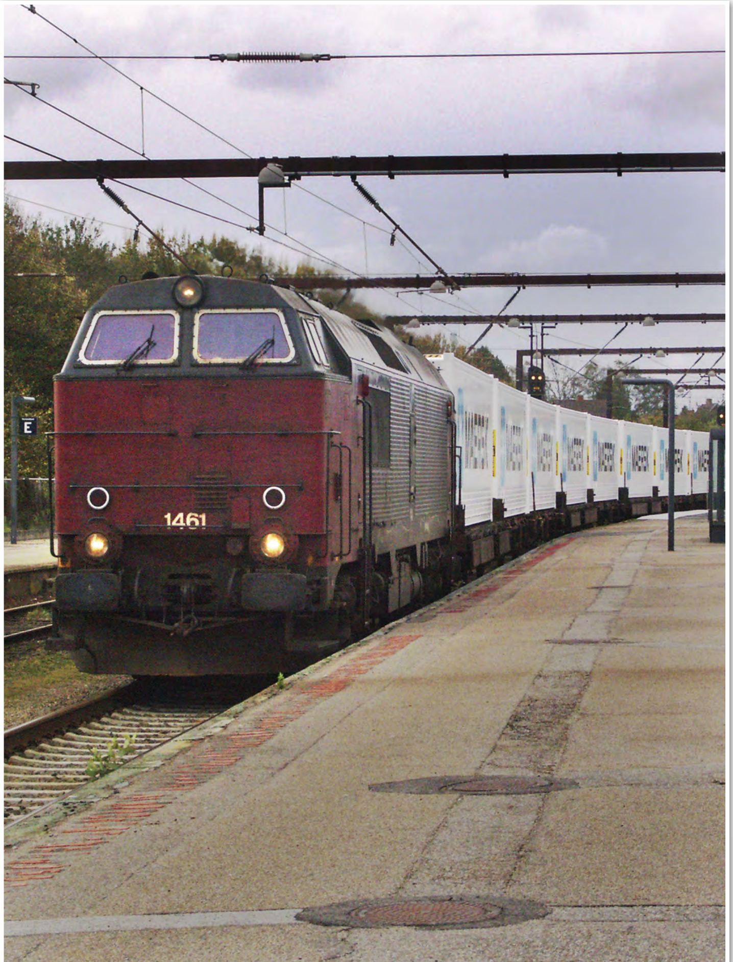
More brutish in appearance, with their higher bodysides and inset cab side windows, were the later batches of MZs such as No. 1461, seen at Fredericia in Jutland on 1st November 2006 heading north with a train of Maersk containers.
