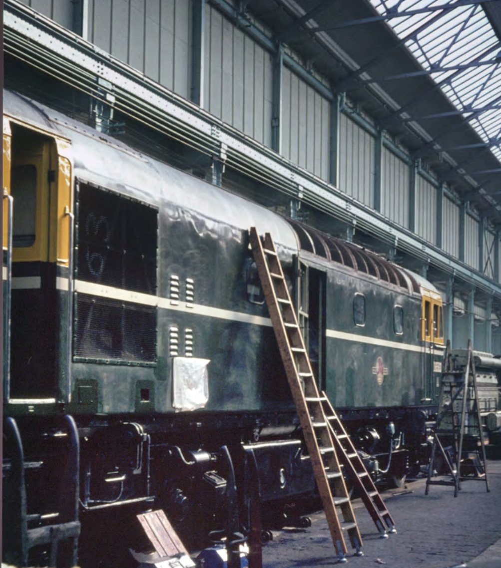
A feature of the system introduced at Eastleigh was the use of progress charts that would be displayed on the locomotive under overhaul, in this case D6553. These charts ensured everyone knew what needed to be done and when. A manager could glance at the chart and see how the overhaul was progressing against the plan.
