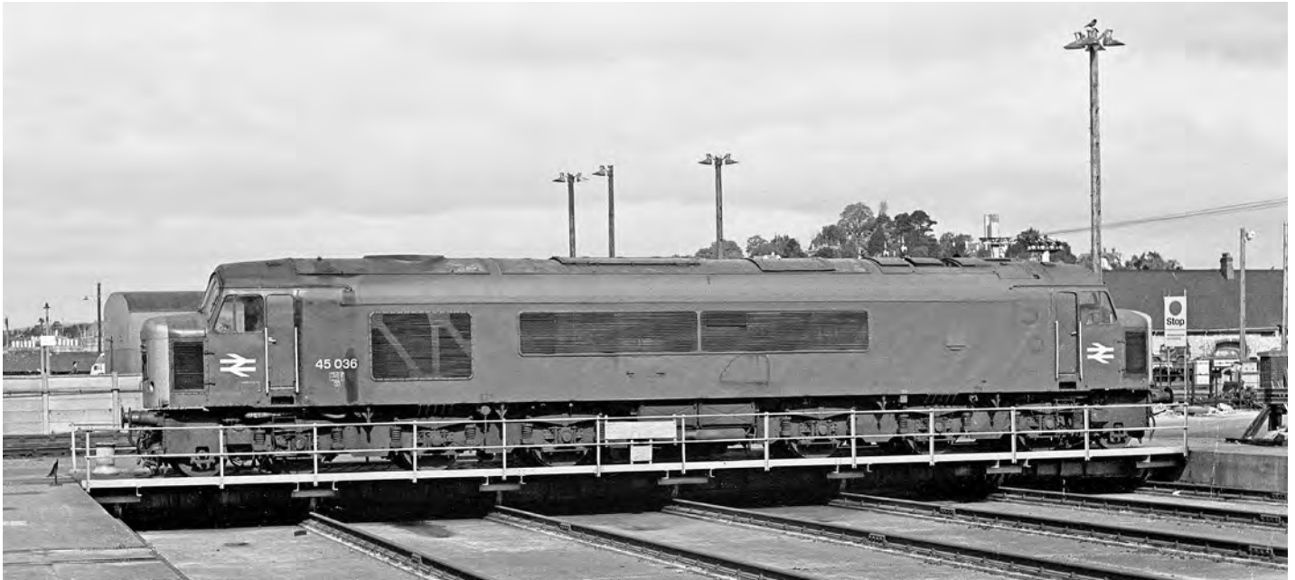
On 10th June 1978, 45036 is standing on the new traverser that was built at the east end of the depot. In 1962 the factory was rebuilt so that the old longitudinal traverser was removed and a new one was added at the end of the building to give access to four roads with servicing pits and cab level platforms. Railphotoprints.co.uk - John Chalcraft
