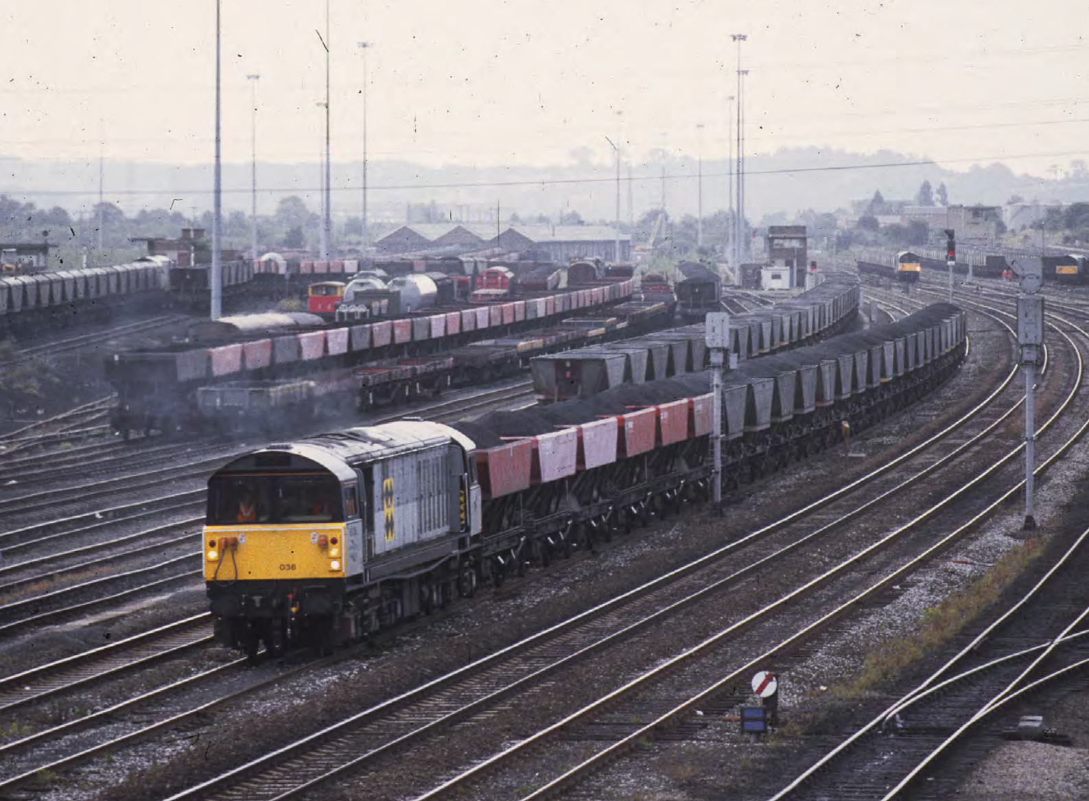
ABOVE: The pilot introduction of maintenance based on RCM was on the then relatively new Class 58 Co-Co diesel electrics which at that time were experiencing several unreliability issues. No 58036 arrives at Toton yard with a coal train on 17th September 1991.
