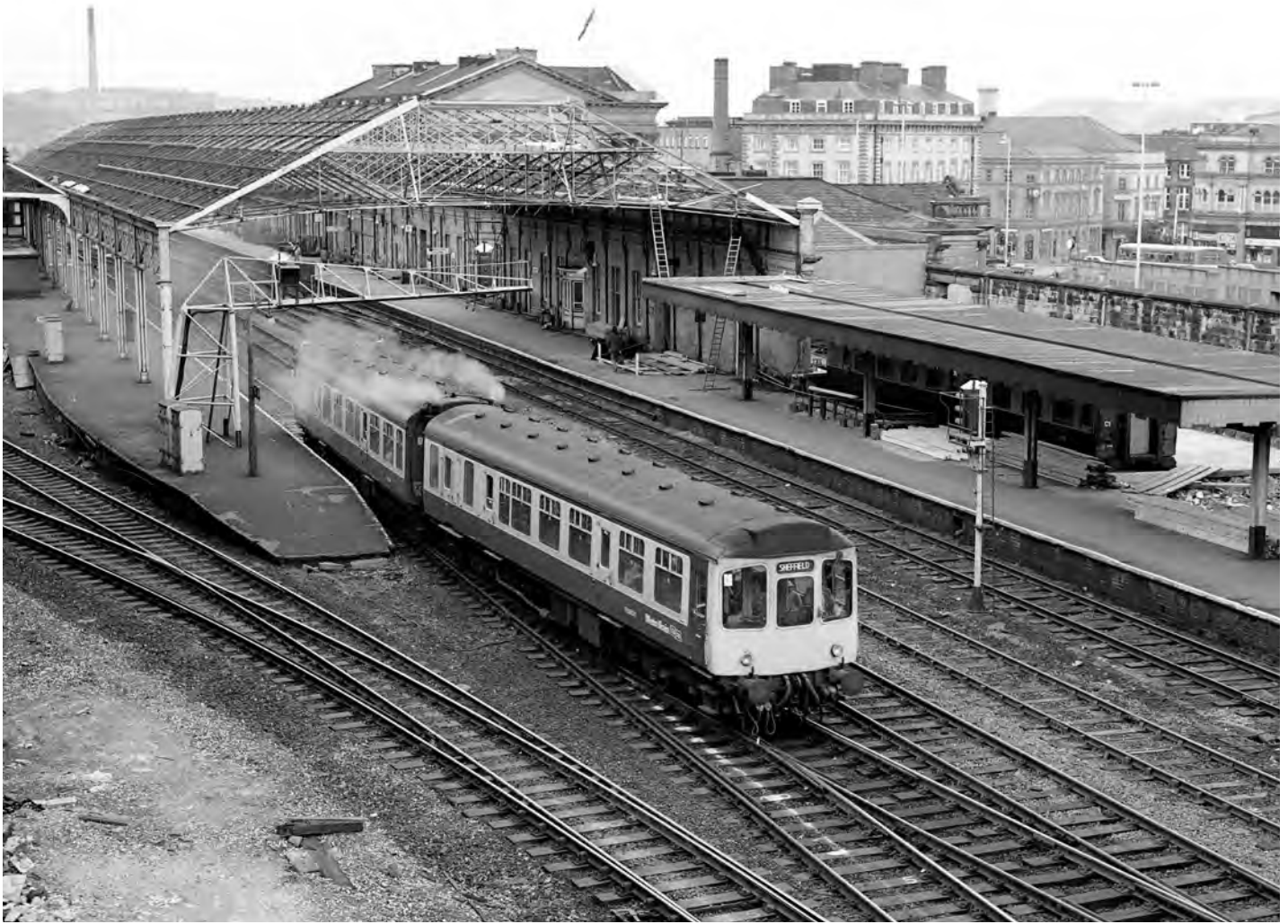
ABOVE: A Class 110 'Calder Valley' unit is seen leaving Huddersfield on the 16:18 departure to Sheffield. The leading vehicle No. E51824 was a Driving Motor Brake Composite (DMBC) and was paired with No. E51846 a Driving Motor Composite Lavatory (DMCL). In 1982 these former three-car units were reduced to two cars with the removal of the centre Trailer Second Lavatory (TSL) vehicle. This was done to reduce maintenance costs and to allow the higher performance needed for accelerated services on the Calder Valley line. Their power to weight ratio of 11.2 hp per ton gave these sets the best performance of any of the first generation DMUs, but at the expense of a significantly reduced capacity. At the same time the first class sections were declassified, although the original seats remained in place. Note that the unit carries the 'Metro Train' branding of the West Yorkshire Passenger Transport Executive.
