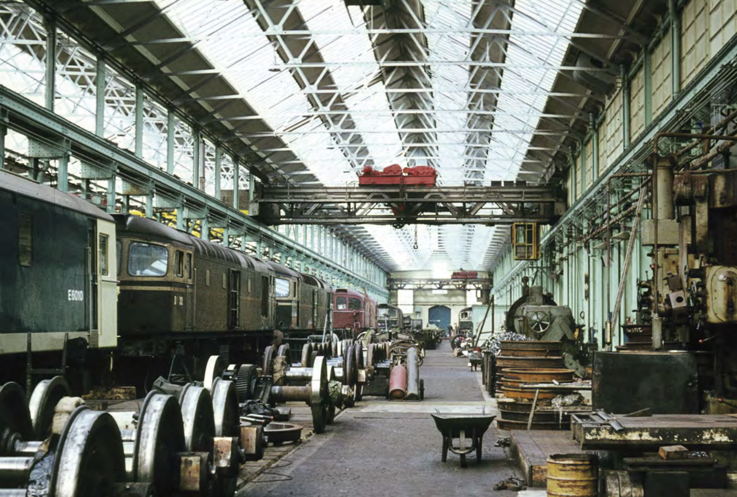
In this view of the Eastleigh Works erecting shop in 1966, four BRCW Type 3s are under overhaul or repair. At that time, the overhaul of these useful locomotives occupied about three weeks in this shop. Network analysis enabled this time to be reduced to six or seven days.
