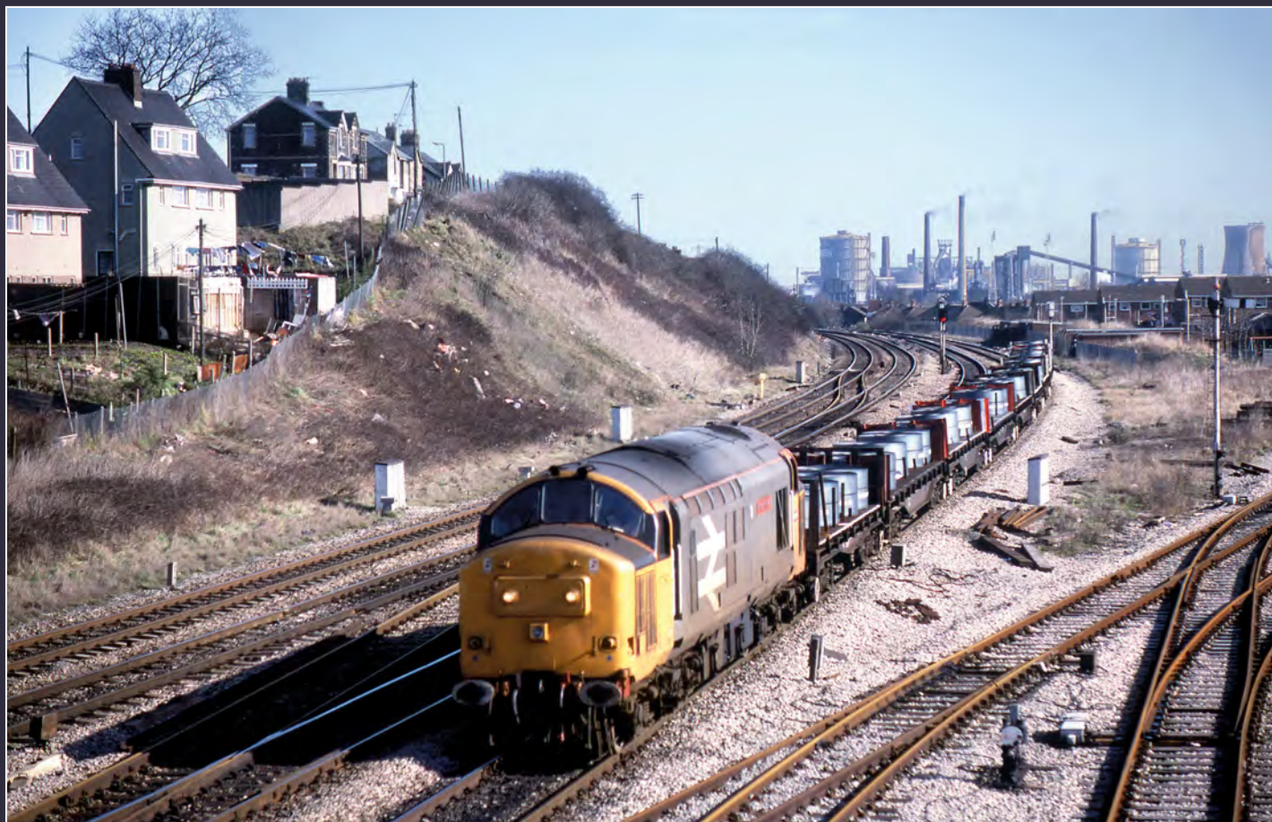
37901 Mirrlees Pioneer is seen passing Usk Junction at Newport on westbound steel coil train on 2nd March 1987. Built in 1963 and originally numbered D6850, the locomotive became 37150 in 1974. It was refurbished and re-engined in 1986 with a Mirrlees six cylinder 1800 hp power unit and Brush electronic equipment as part of BR's tests for the proposed Class 38.
