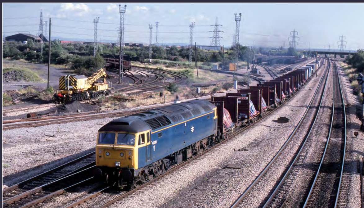
37901 Mirrlees Pioneer is seen passing Usk Junction at Newport on westbound steel coil train on 2nd March 1987. Built in 1963 and originally numbered D6850, the locomotive became 37150 in 1974. It was refurbished and re-engined in 1986 with a Mirrlees six cylinder 1800 hp power unit and Brush electronic equipment as part of BR's tests for the proposed Class 38.
