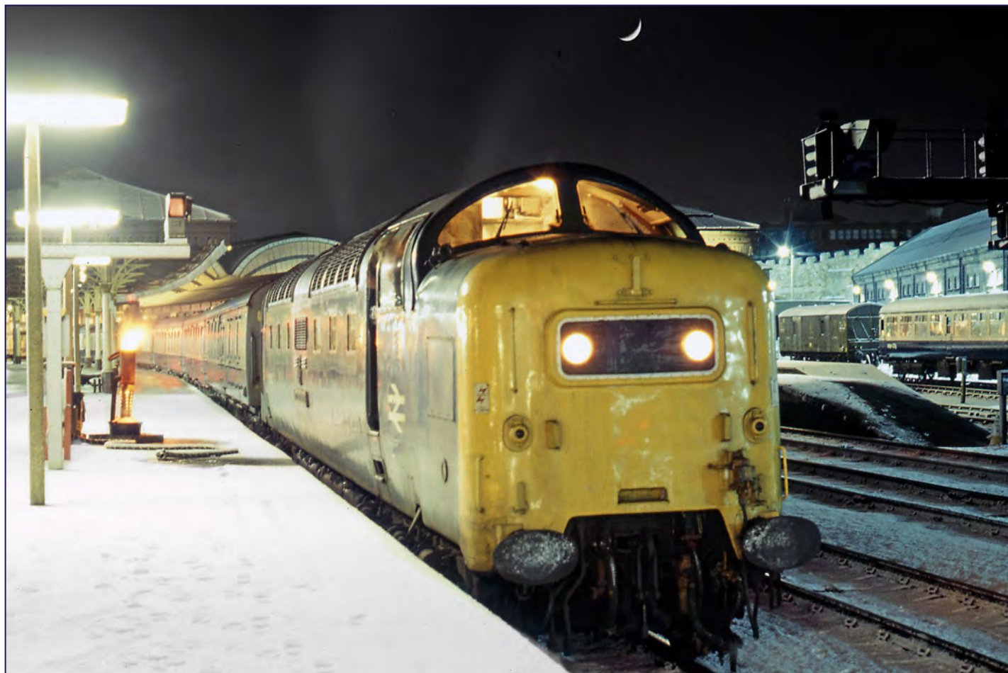
With the moon overhead, 55 008 The Green Howards pauses at York with the 1E40, the Saturdays only 19:15 Aberdeen to London King's Cross. To the left of the locomotive note the oil burning stove to keep the standpipes, used for refilling the steam heat boilers, from freezing up.
