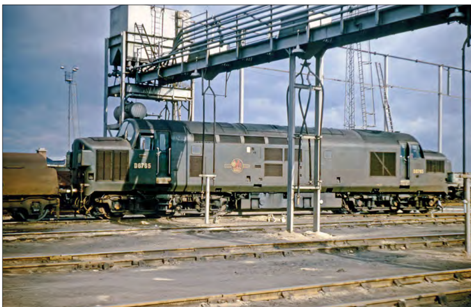
English Electric Type 3 D6765 is seen under the sand filling equipment at Thornaby depot in September 1965. Note the brake tender coupled to the locomotive. www.railphotoprints.co.uk - Robin Whittle
