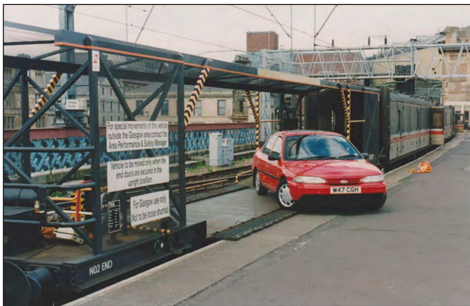
One of the 'scuds' is seen at Glasgow Central. Motorrail vehicle YXA No.96453 was a former 25T bogie WELTROL 900926 that had been rebuilt for use to enable loading of cars into the GUVs from the platform. David Warby
