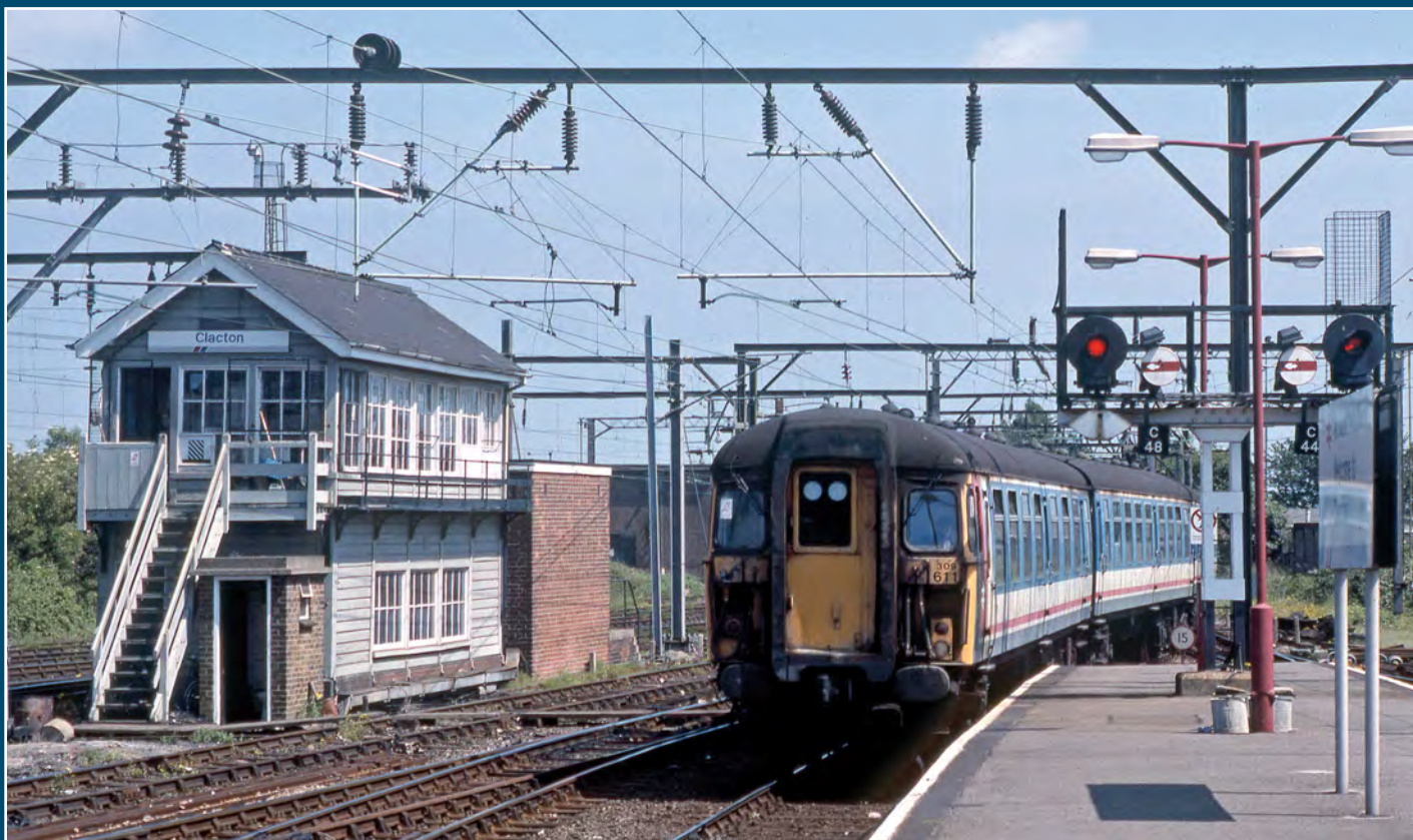
A rather grubby looking 309611 is arriving at Clacton on Sea with a train from Liverpool Street on June 16th 1990. Note the former Great Eastern railway signal box and the searchlight colour light signals.
