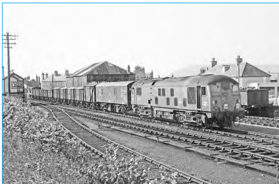
ABOVE: In 1969 Sulzer Type 2 No. 5084 passes Towyn (now Tywyn) with a Cambrian Coast freight service. The train has the typical mixture of wagons: a couple of vans, some empty coal wagons and a rake of explosives vans from Penrhyndeudraeth. Railphotoprints.co.uk - John Day collection
