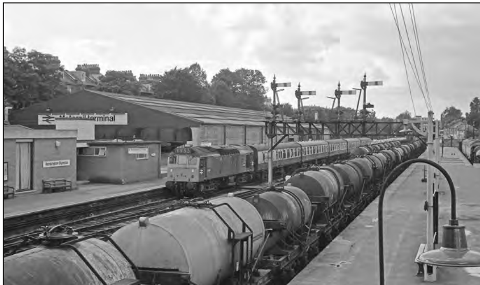
D7667 is at Kensington Olympia on Sunday 18th August 1968 with what is believed to be IV33 the 10:45 Holyhead to Kensington Olympia service. In the background is the purpose built Motorail car loading terminal building. The carflats at the rear of the train will shortly be uncoupled and propelled into the terminal for unloading. Rail-Online
