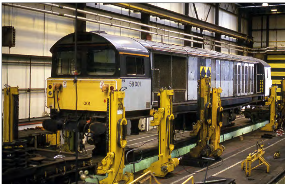
BELOW: 58001 is on the lifting jacks at Toton depot for a bogie change on September 6th 1992. Dave Higson
