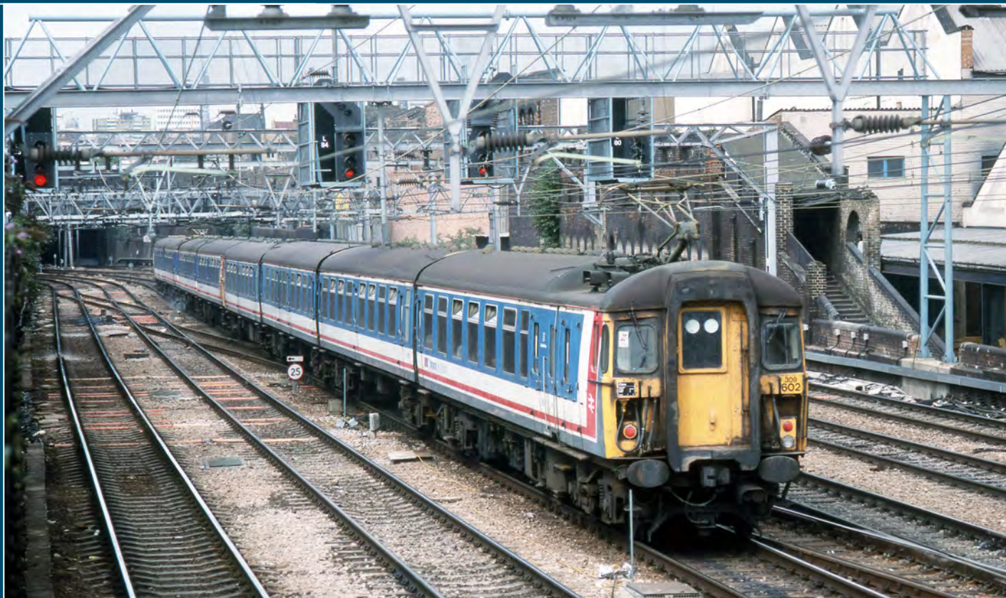
The Class 309 'Clacton' units were the the first 100 mph EMUs. They were at first painted in BR maroon and had stylish wrap-round cab windows. After refurbishment these were replaced with smaller windows as seen in the photograph. Unit 309602 is seen heading away from the photographer as it climbs Bethnal Green Bank en route to Clacton on August 12th 1989.
