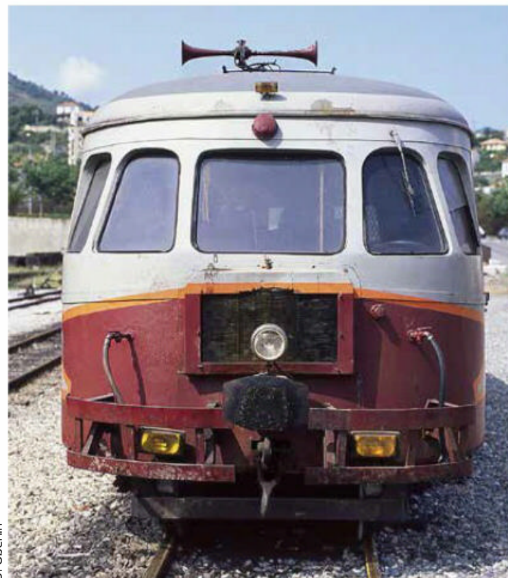
N° 513 seen from the carrying bogie end with its additional radiator.
