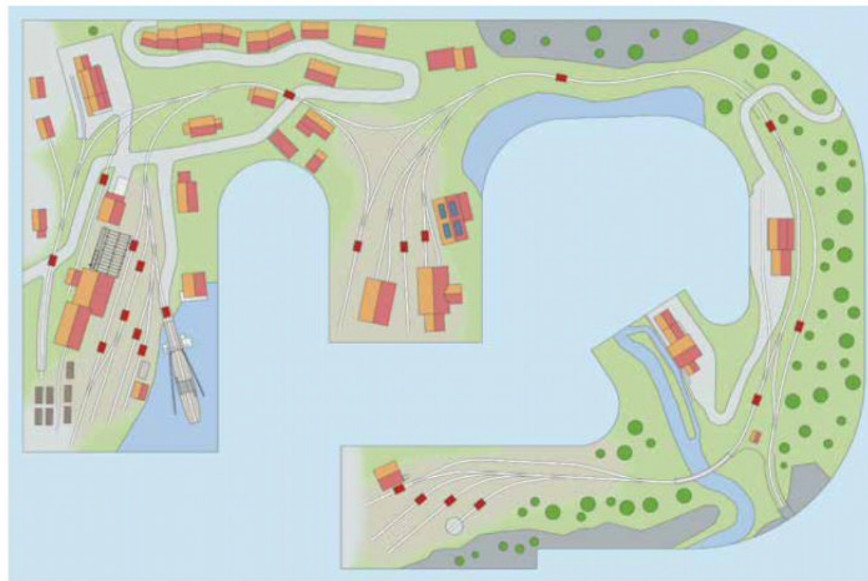
6 Location map of the uncouplers on the Carpatès layout.
