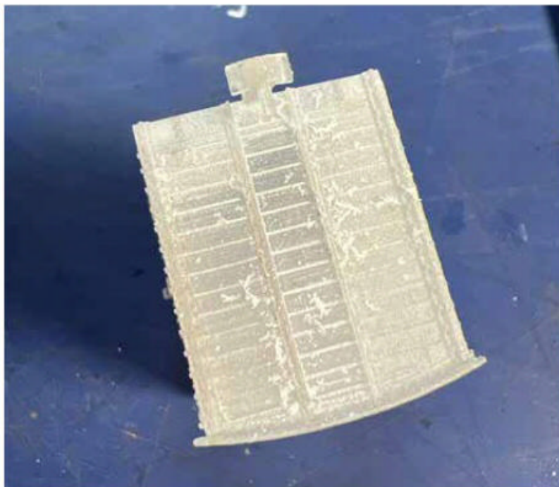
7 The wax leftovers, not eliminated by the alcohol bath, are clearly visible. But they are invisible to the naked eye.
