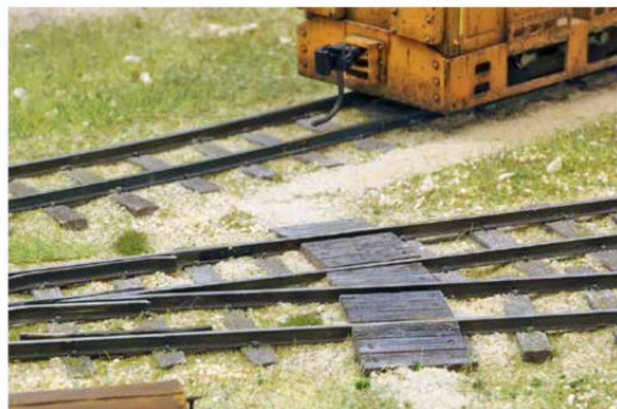
15 The barrow crossing conceals the uncoupler.
