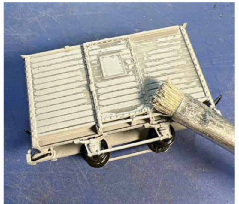
8 Here is the catastrophic result of faulty cleaning! A simple dry brushing is enough to remove the paint, which holds only onto the wax, not to the plastic.
