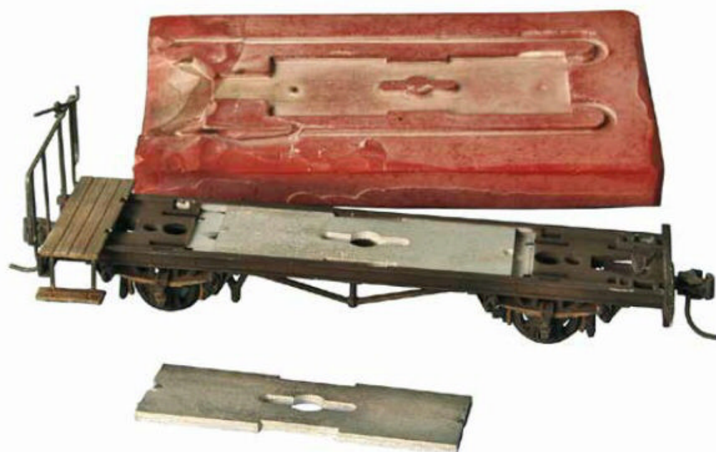
3 A Magic Train wagon with its Kadee On3 couplers and its new non-magnetic ballast.
