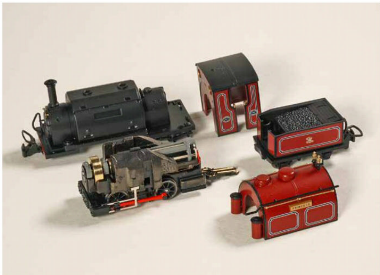
The model is easy to dismantle, note the conductive towbar between the loco and tender. The large loop couplings can be replaced by more discreet ones.
