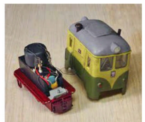
The body conceals the large condenser used to compensate for gaps in the electrical supply.
