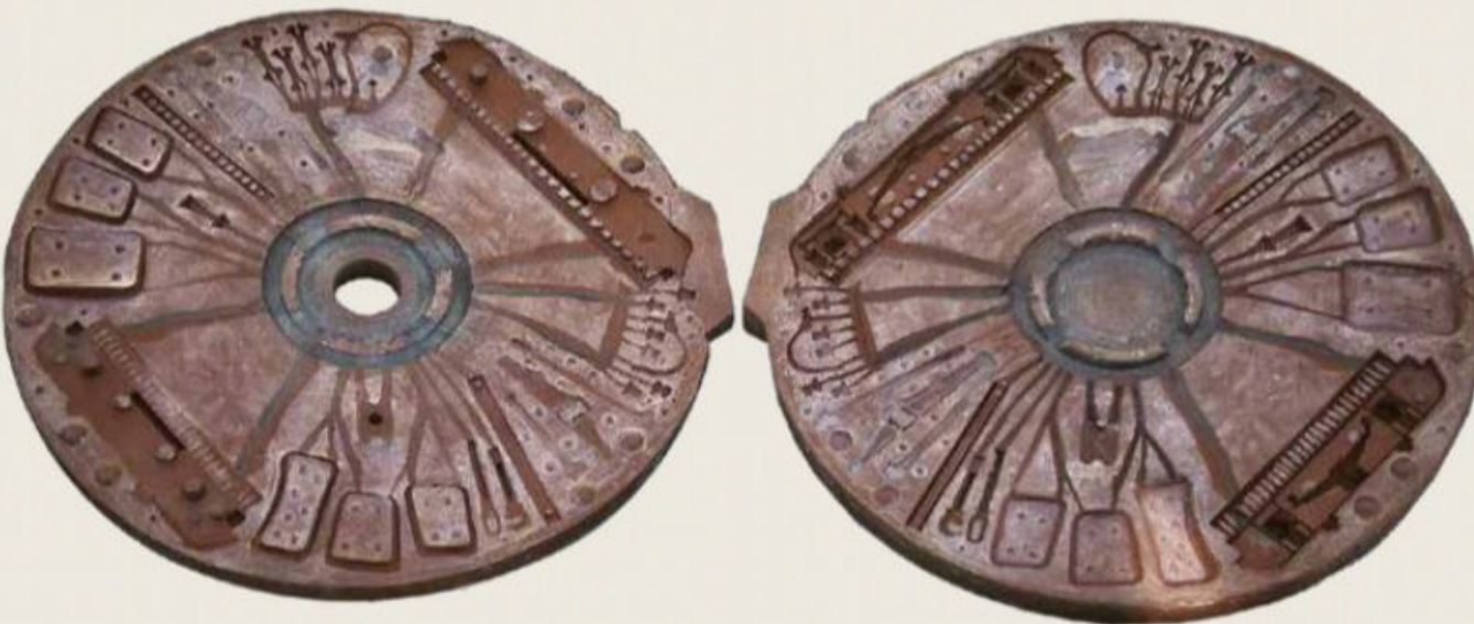
11 A high temperature silicone mould will be used casting the various detailing parts as well as the bogie frames.
