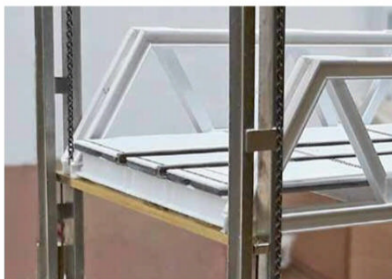
13 The brass cross-beam at each end is an essential part: it sits on the piano wire legs, ensures the guiding by sliding inside the uprights, and holds the hangers of the counterweight chains.
