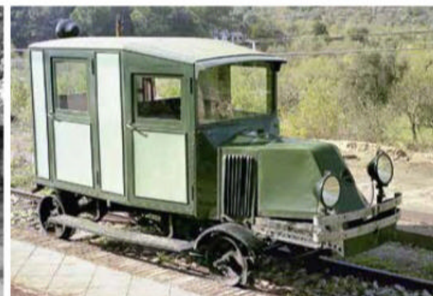
A Renault car converted into a rail motor trolley, built in 1924, modified in 1937, seen at Soller, 25th October 1974.
