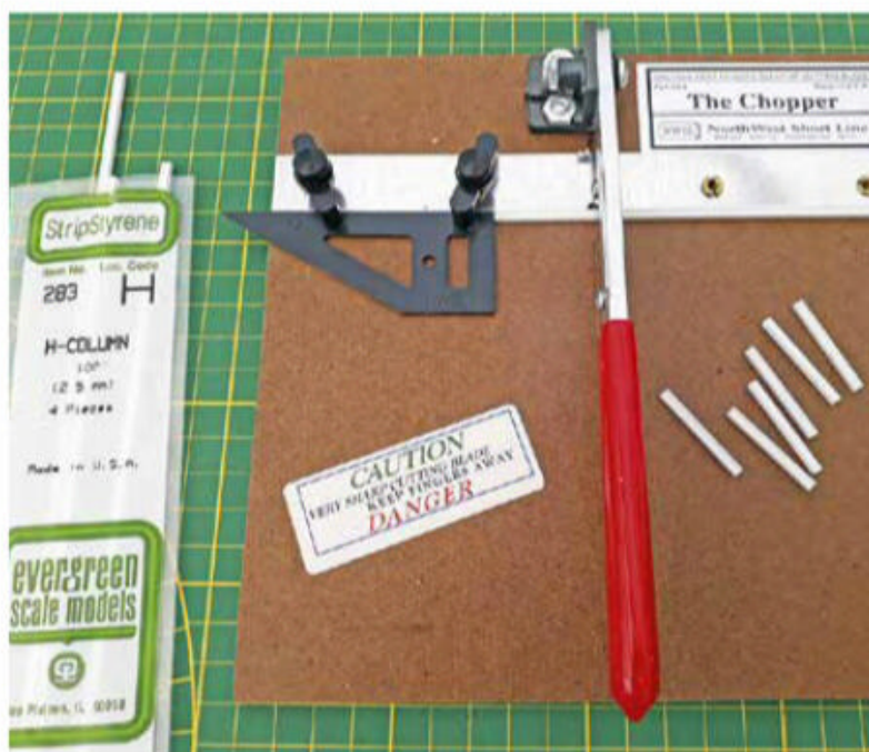
4 The H girders are cut to the right length using a Chopper tool.
