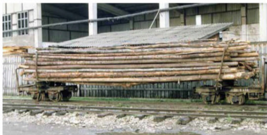
At Moldovita , on 17 August 1992 , close up on a load. The logs are loaded to the very upper limit of the stanchions. There is no connecting rod between the disconnects.
