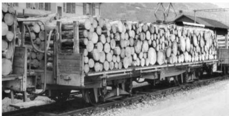
Squared logs loaded onto a bogie flat wagon at Châtel-Saint-Denis in March 1960 . Note the logs that act as bolsters on the wagon.
