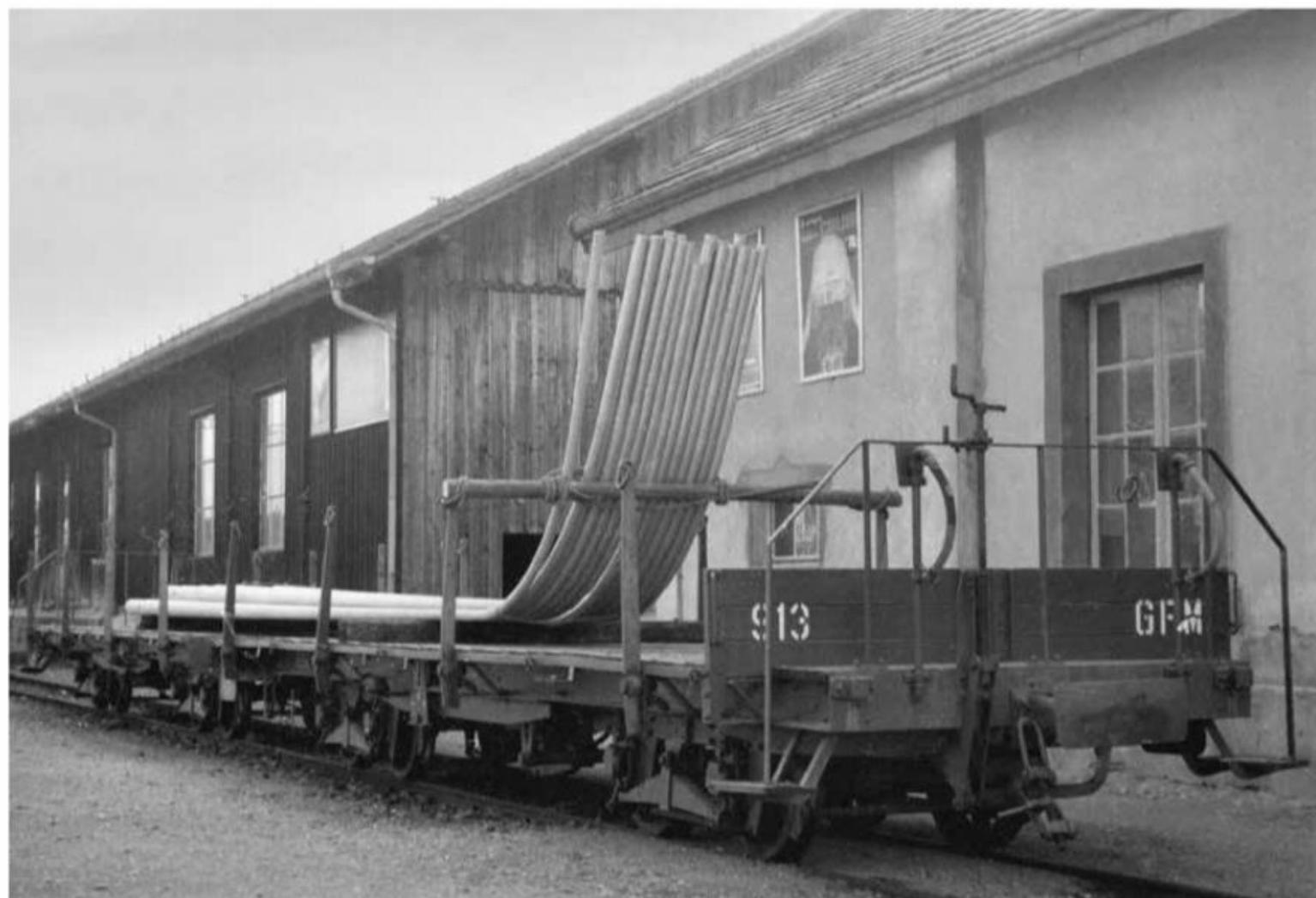
March 1960 at Châtel-Saint-Denis , a flat wagon carrying a metal structure. The ends are held in place by a rope tied around a simple log, itself lashed to the stanchions.
