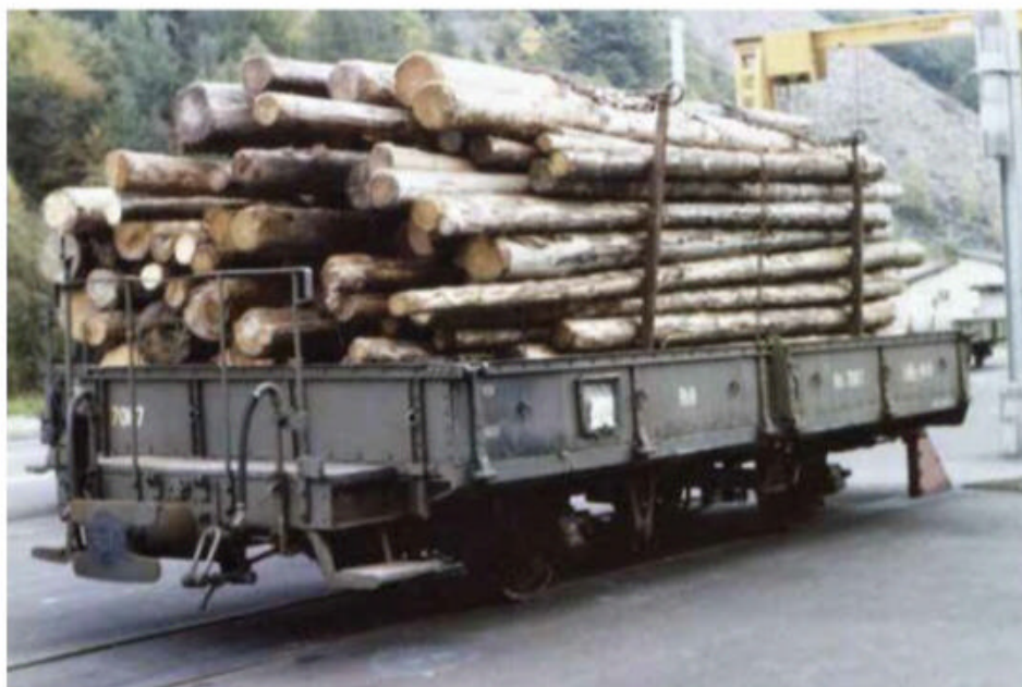
At Samedan on the Rhaetian Railways , this small flat wagon is loaded with logs. Note the chains of various sizes that hold the load in place.
