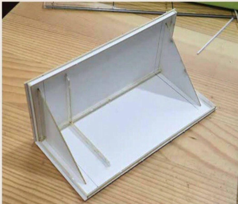
The roof is assembled on two formers that fit inside the gables.
