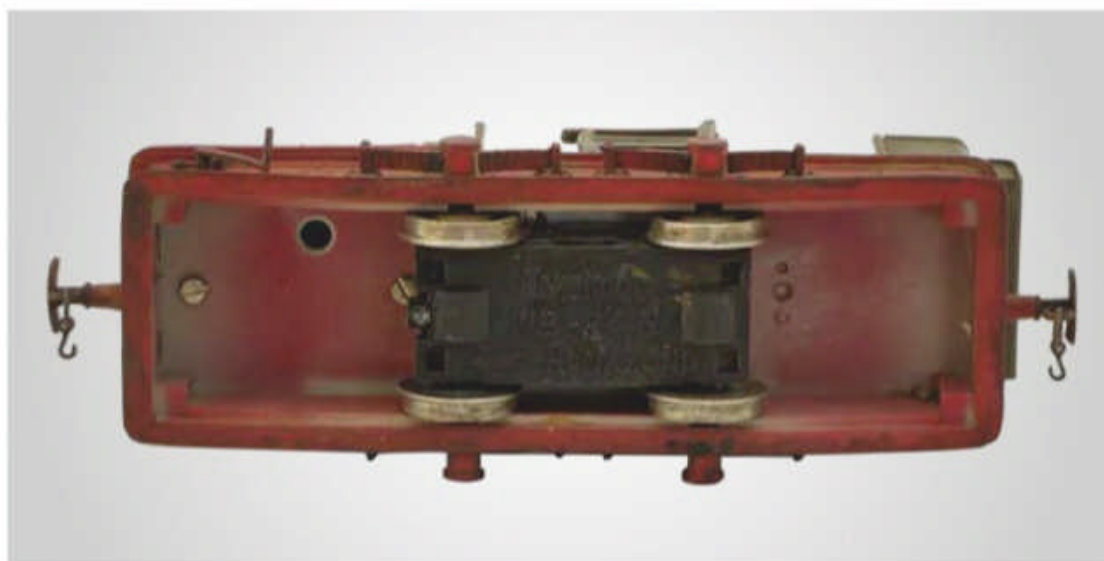
3 The Tenshodo bogie under the chassis, fixed with double-sided tape.
