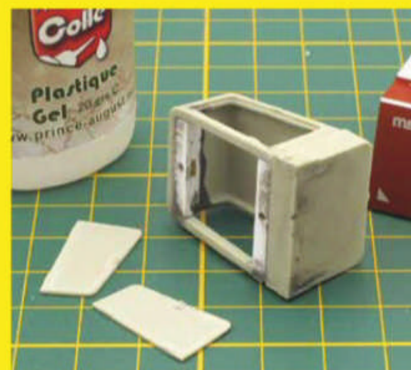
The nut brackets are glued in place with two-part epoxy adhesive.
