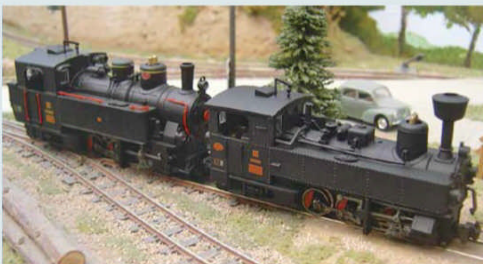
U n°2 (from the set ref. L177700) in front of the impressive Zillertalbahn Uh n°5 (ref. L141491): in addition to the blackened motion and loop couplings, the third generation brass flywheel can just be seen inside the cab of the U.
