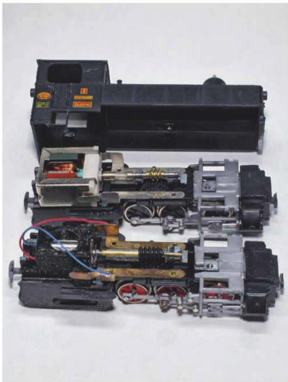
The chassis of my Liliput 0-6-2 T engines. In the foreground, the modified model. Behind, the chassis with the original motor. It is quite obvious that both motors take up exactly the same volume.
