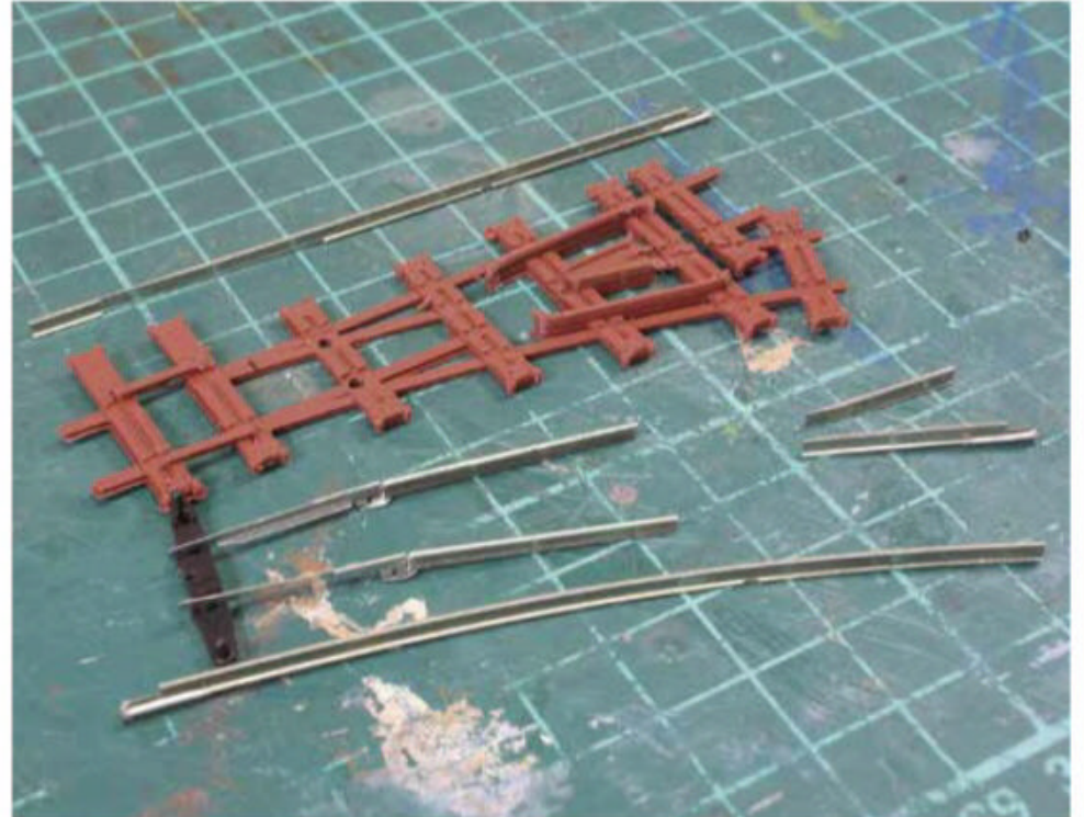
The Peco turnout was completely and carefully dismantled, so as not to warp the parts. The frog connecting wires were simply eliminated. The tie-bar was re-used.
