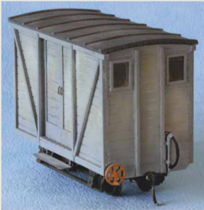
A fully-fitted wagon end, with its brake wheel and brake hose.
