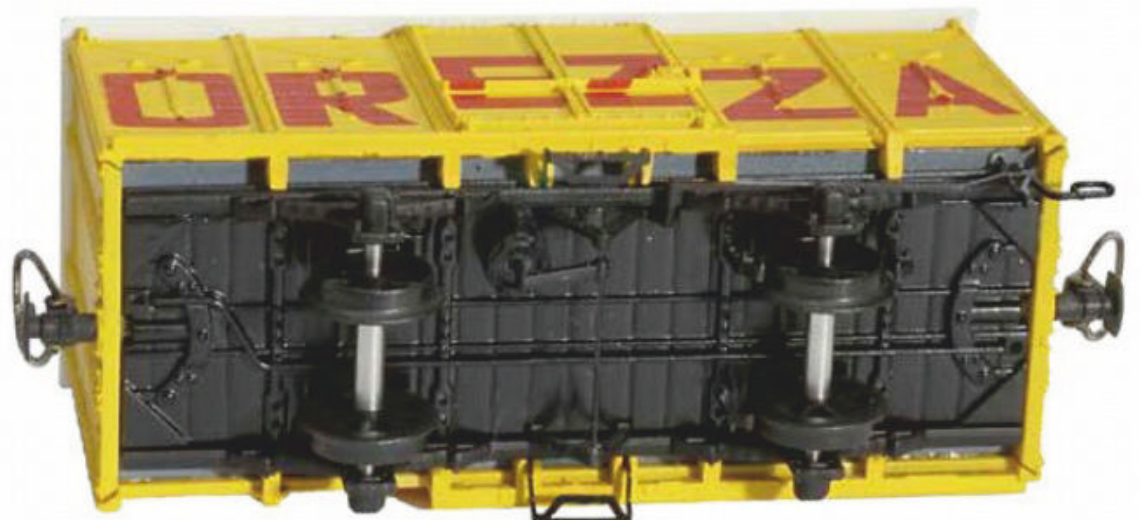
With the wagon upside down, let's take a look at the cast metal chassis. Besides the cast couplings, the brake cylinder and the steps are add-on parts. Note the apertures to accommodate the wheels, and the various holes for fitting the brake shoes. This OREZZA box van is fitted with 9mm gauge axles.
