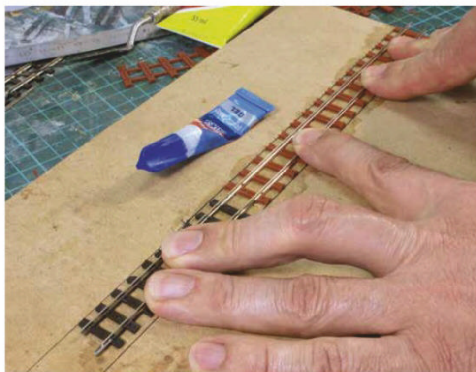
Once the sleepers are in place, I glue the rails with cyano adhesive. The groove is dimensioned to provide a tight fit for the rail. The unmolested Peco length is just there for laying the track. It helps to position the two rails lengthways.
