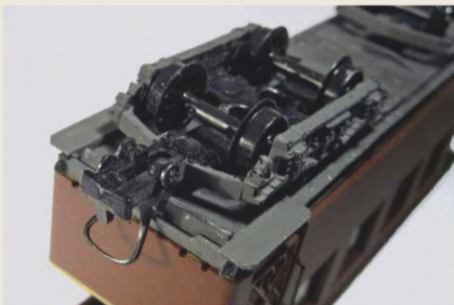
12 The steps must not impair the rotation of the bogies.
