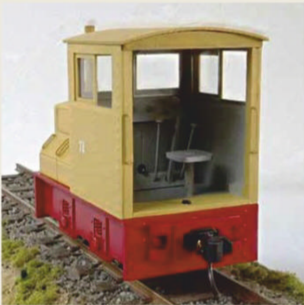
14 And the assembly is then give a coat of primer before being painted.
