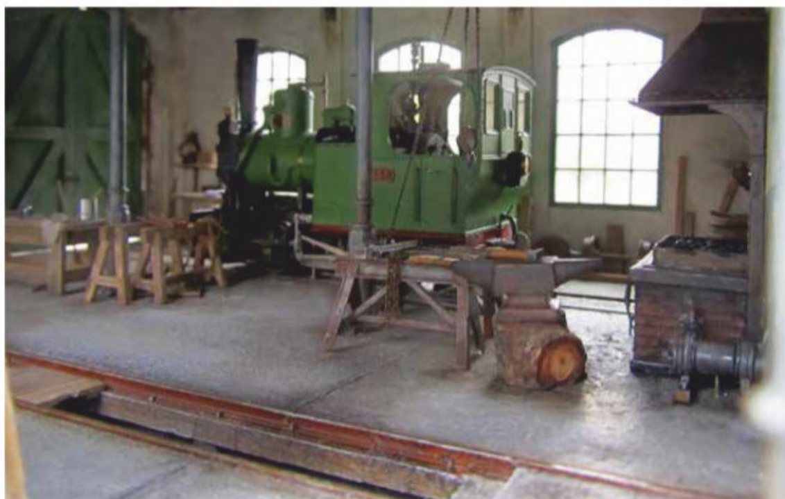
14 The Stainz rests between duties. Note, in the foreground, the inspection pit whose rails are laid on girders.
