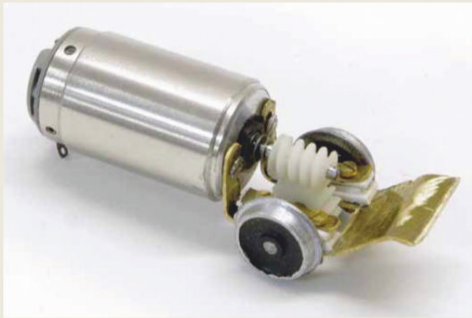
9 The 0.5 module worm wheel and gear combination is from a Jouef locomotive!
