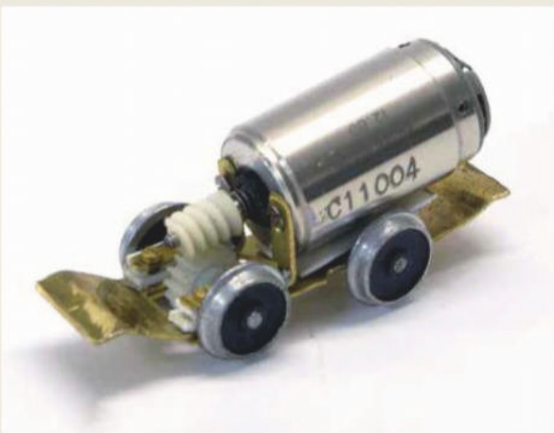
10 One of the tabs that hold the motor has an oblong hole drilled in it to adjust the pressure of the worm wheel on the gear.
