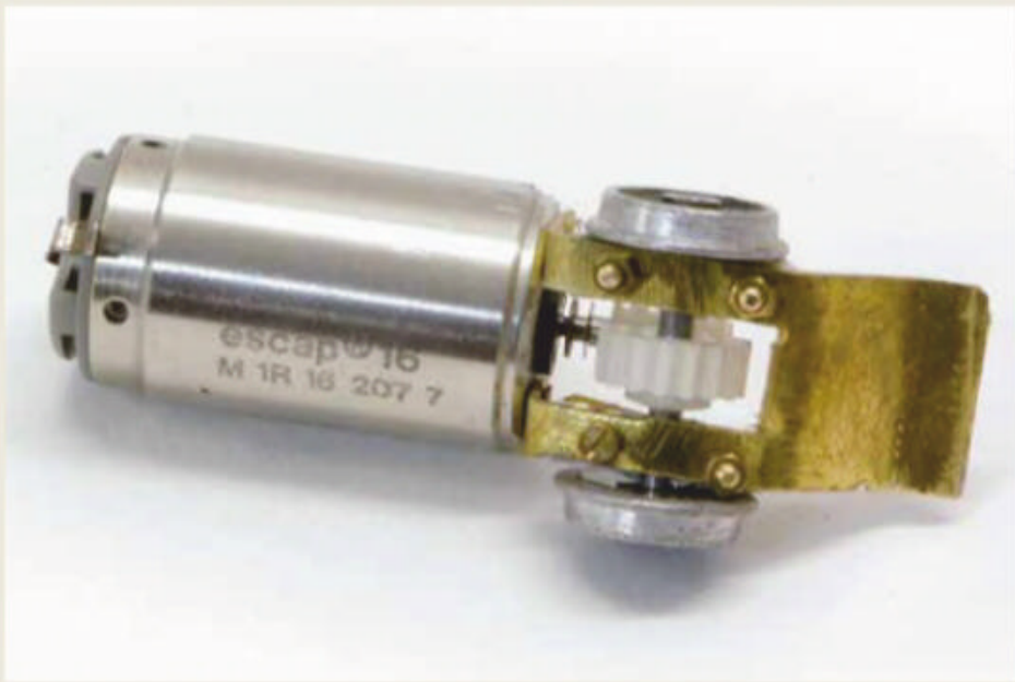
8 The driving axle part of the cradle, cut out of 0.5mm thick brass sheet.
