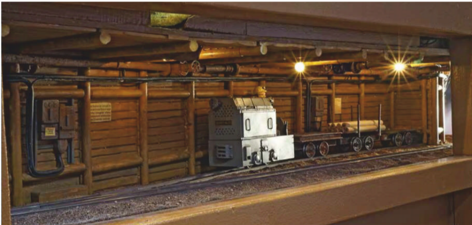
A gallery with a siding. Admire the wooden props, the electric wiring and the pipes for the mine water.
