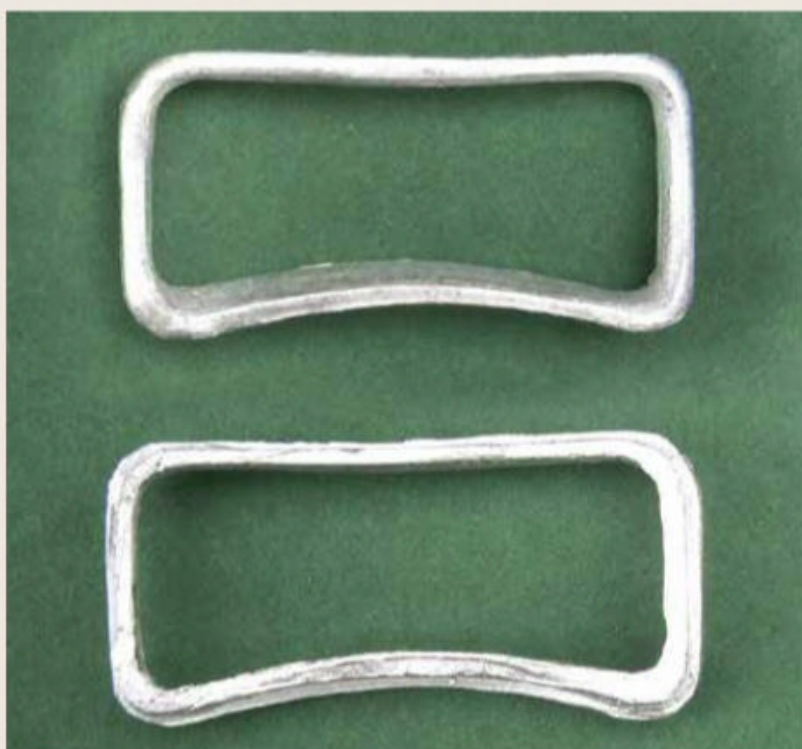
12 Two white metal frames, for the railcar windscreen on the radiator side.
