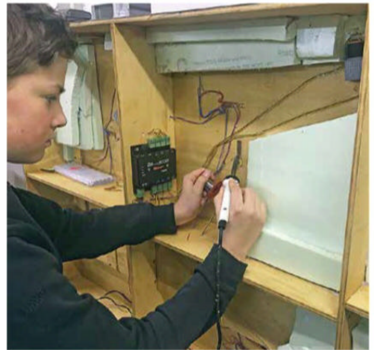
A more delicate phase, soldering the electrical connections. The Z21 block is wired up to the turnout motor connectors visible at right.
