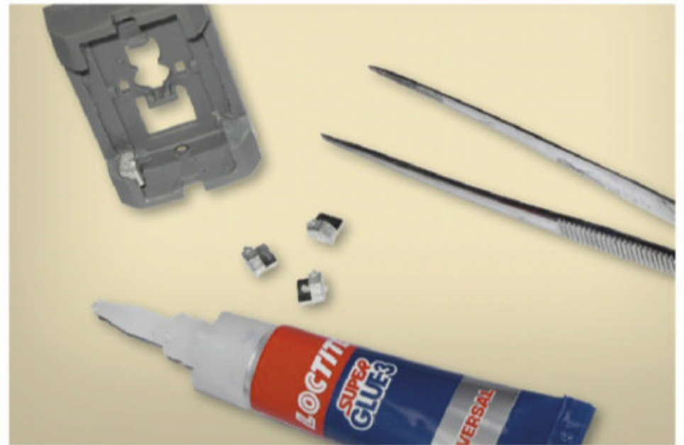
The white metal sandboxes are fixed onto the running board using instant adhesive.
