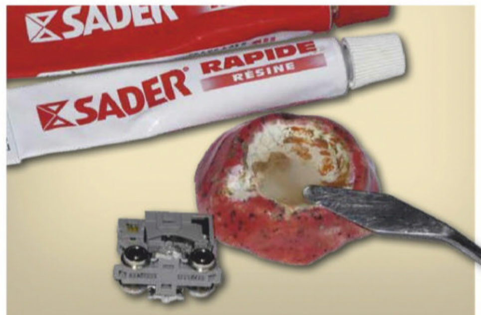
The brake blocks are fixed using two-part epoxy.
