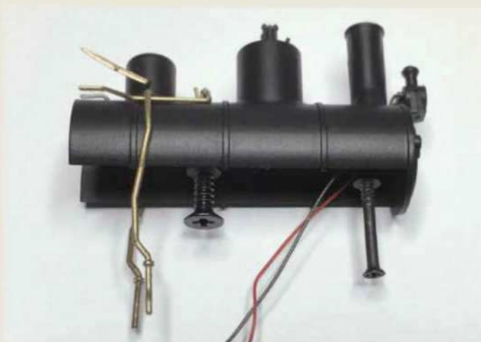
7 The boiler without its ballast.
