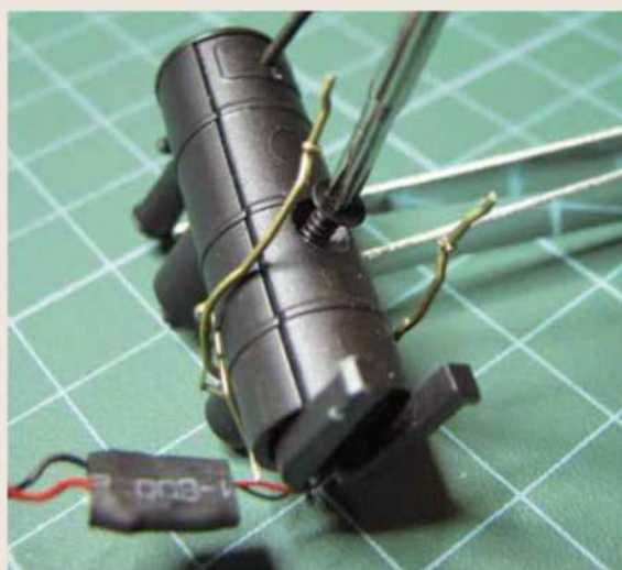
6 Removing the ballast from the boiler.
