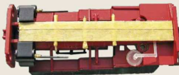
17 Masking the mechanical parts before painting.
