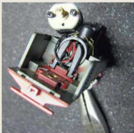
3 The circuit board housing, accessible after the motor has been removed.
