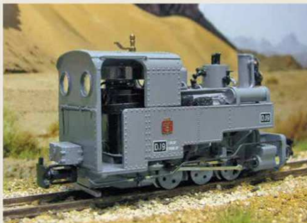
19 The buffers are painted black, the toolbox and the fire tools are fitted at the rear, the decals (Spike 3D), the Narrow Planet plates and the briquettes on the water tanks are all in place.
