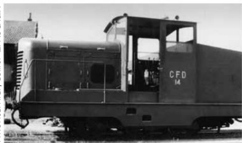
Tractor N° 14 built on the chassis of 2-6-0 T locomotive N° 207 seen at Toulon-sur-Arroux, in 1953 , and subsequently transferred to Egreville, on the Seine-et-Marne CFD network.
