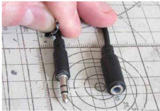
The jack connector. Male part to the left, female part to the right.
