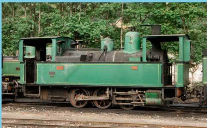
Pinguely 0-6-0 T locomotive N° 31 restored by the SGVA with its two cabs, seen at Tournon, 26 May 1996 .
