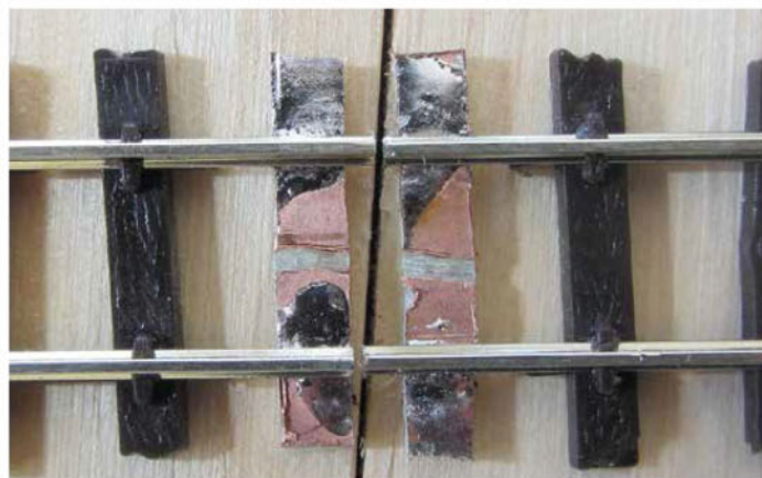
The tips of the rails are soldered to copper-clad epoxy.
