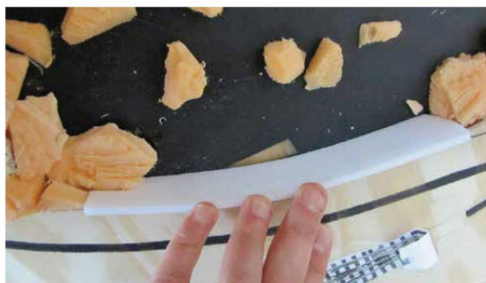
The wall is cut out of foam board and fitted in place.
