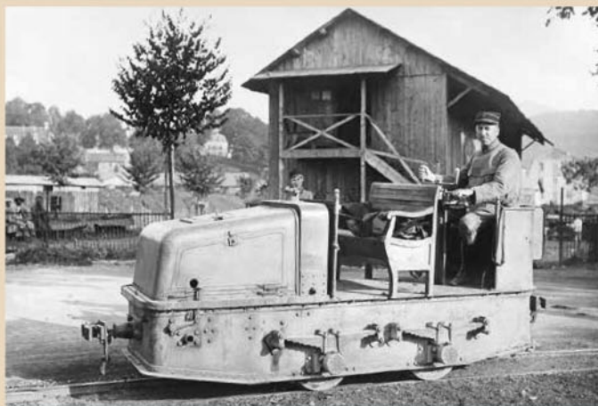
Wesserling, 8 August 1916, a petrol-driven motor-trolley on 60cm gauge track, used by the Engineer Corps.
