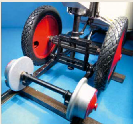
10 The rear bogie in place on the motor-trolley.
