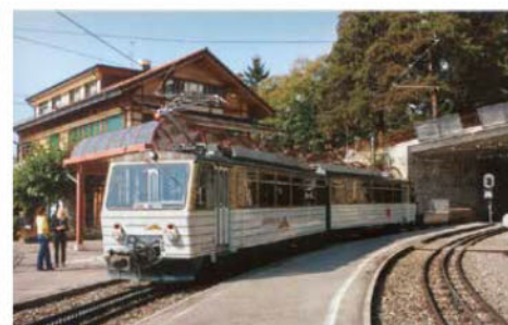
Articulated motor unit Bhe4/8 305, built in 2009/2010 by the company using spare bogies for the Bhe4/8 301 to 304 series, seen at Glion. 30 September 2015.
