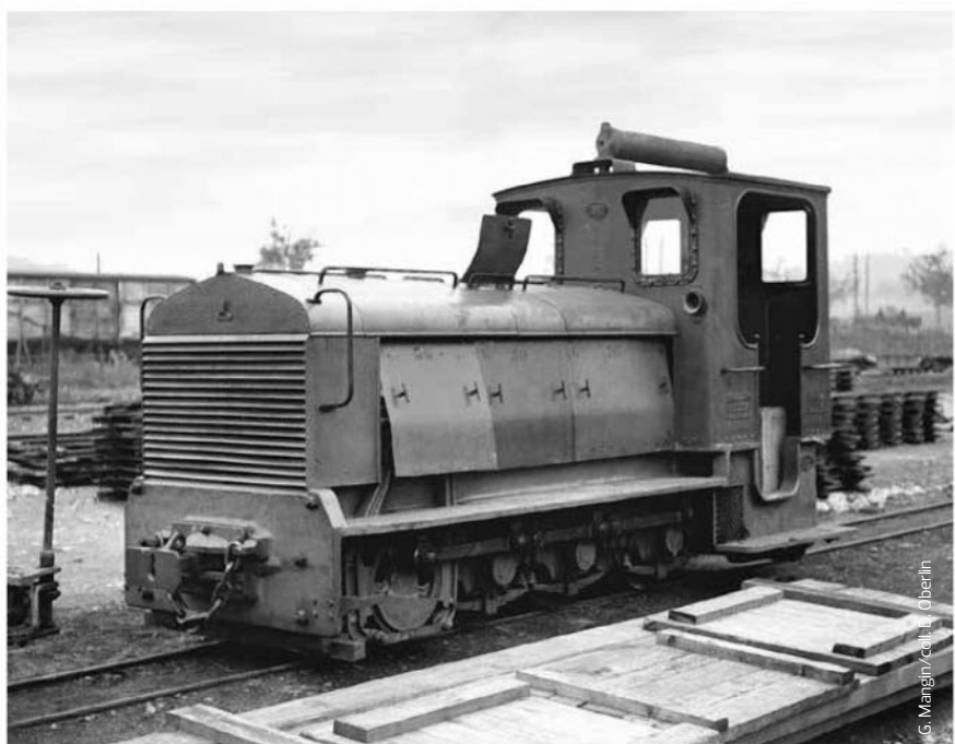
A Schneider mechanical transmission locotractor seen in a depot, behind the front line.
