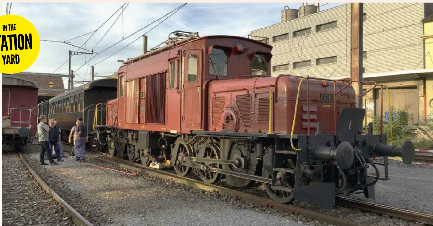
The small Seethalbahn crocodile has recently joined the shed. This locomotive was built in 1923 by assembling back-to-back two shunting engines, Ee 3/4 16301 and 16302! Extraordinary machines are not only found on narrow gauge!
