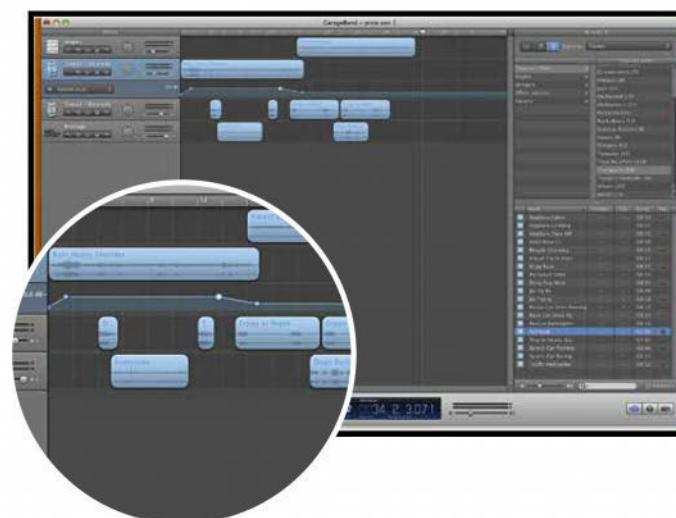
Example of soundtrack: four tracks, but three maximum played simultaneously. The atmospheres, tracks 1 and 2 are muted, even though the storm on track 2 is a bit louder. The narrative sounds are at their nominal level. This small track lasts one minute and weighs 1MB.
