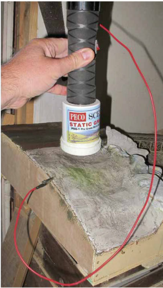
On a coat of diluted glue, I apply a first layer of 2mm long fibre.
