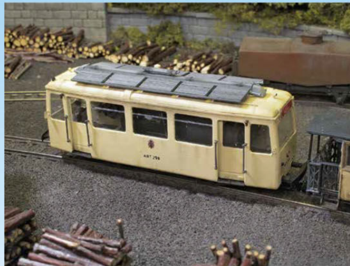
ART unit N°298, with its curvaceous shape and roof-mounted radiators. The driving bogie with its Lenz decoder fitted on top is visible inside.
