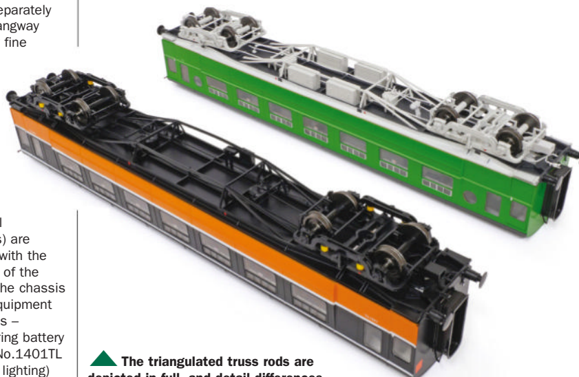
▲ The Irish Commonwealth bogies feature full-relief spring detail.
