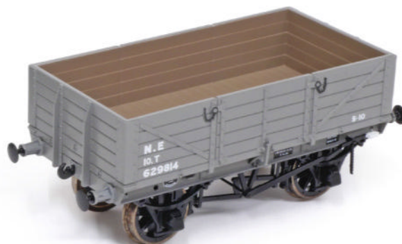
▲ Diagram 17 wagons in post-1902 GER and post-1936 LNER grey liveries.
