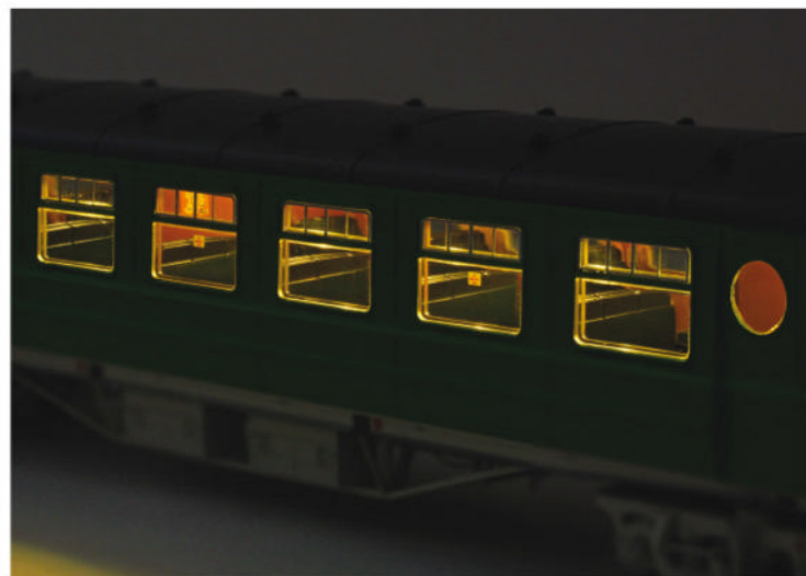
▲ Interior lighting is provided by an LED bar collecting current from the bogies.
