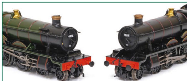
▲ The main visual difference between the Hall and Modified Hall is the front running plate arrangement.
