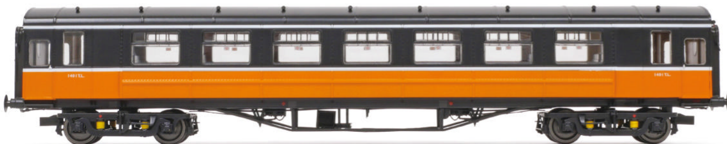
▲ The Irish Commonwealth bogies feature full-relief spring detail.
