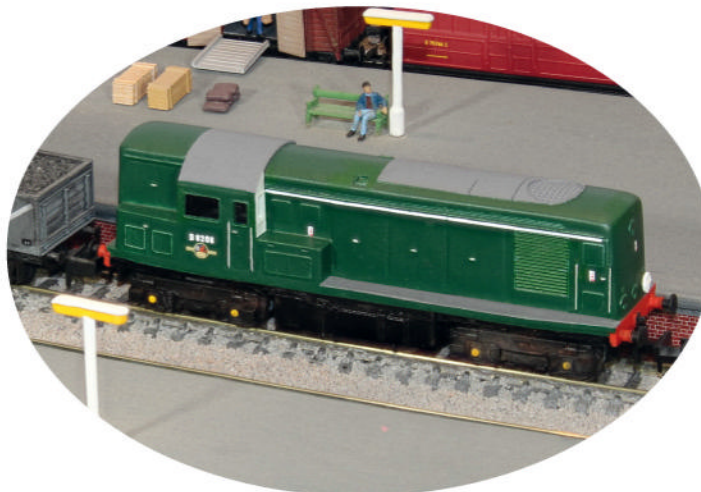
▲ The model in action on the author's Ferryhill layout, hauling a coal train; the Japanese chassis can manage up to 30 of these BR 16-ton mineral wagons on second radius curves.
