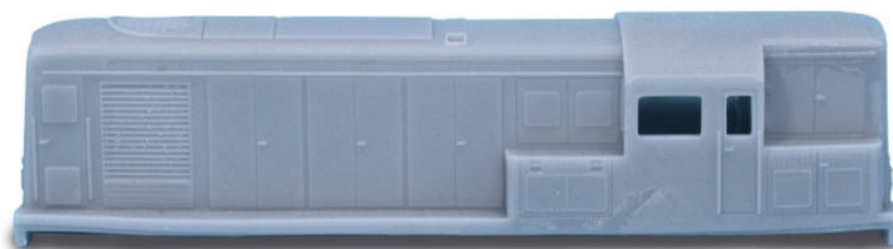
▲ The resin 3D-print of the Class 15 body as supplied, complete with handrails and the cab window apertures already open.
