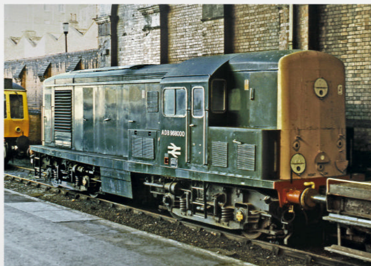
▲ The last Class 15 to be built, D8243, was converted to a coaching stock pre-heating unit with the number ADB968000. It is pictured at London Marylebone in 1985, when it was employed to heat the stock for steam charters. Photo: Gordon Edgar/Rail Photoprints
