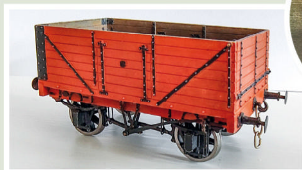
▲ The society's kit for a 1923 RCH seven-plank open wagon comprises plastic body parts and etched chassis components.
