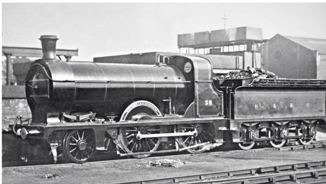
▲ An archive view, recorded at Springhead on 19 September 1904, of Hull & Barnsley Kirtley H1 Class 2-4-0 No.38, the example modelled in this article.
