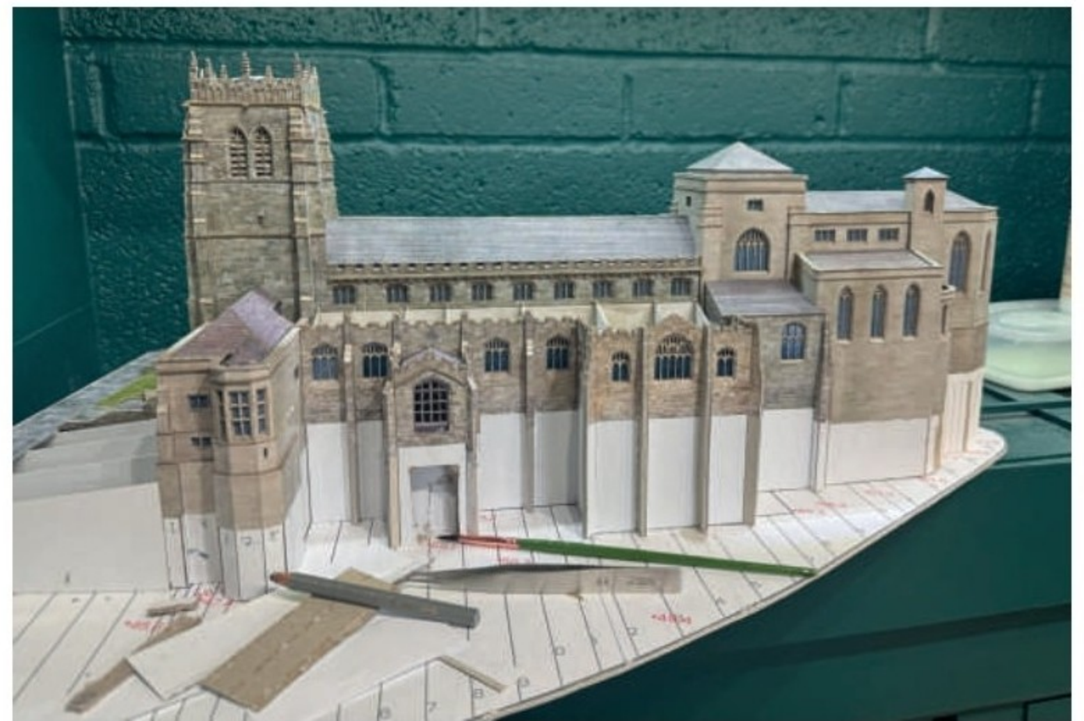
The part-complete model assembled on its foundations, with full-height walls and buttresses used to confirm alignment across the sloping site.
