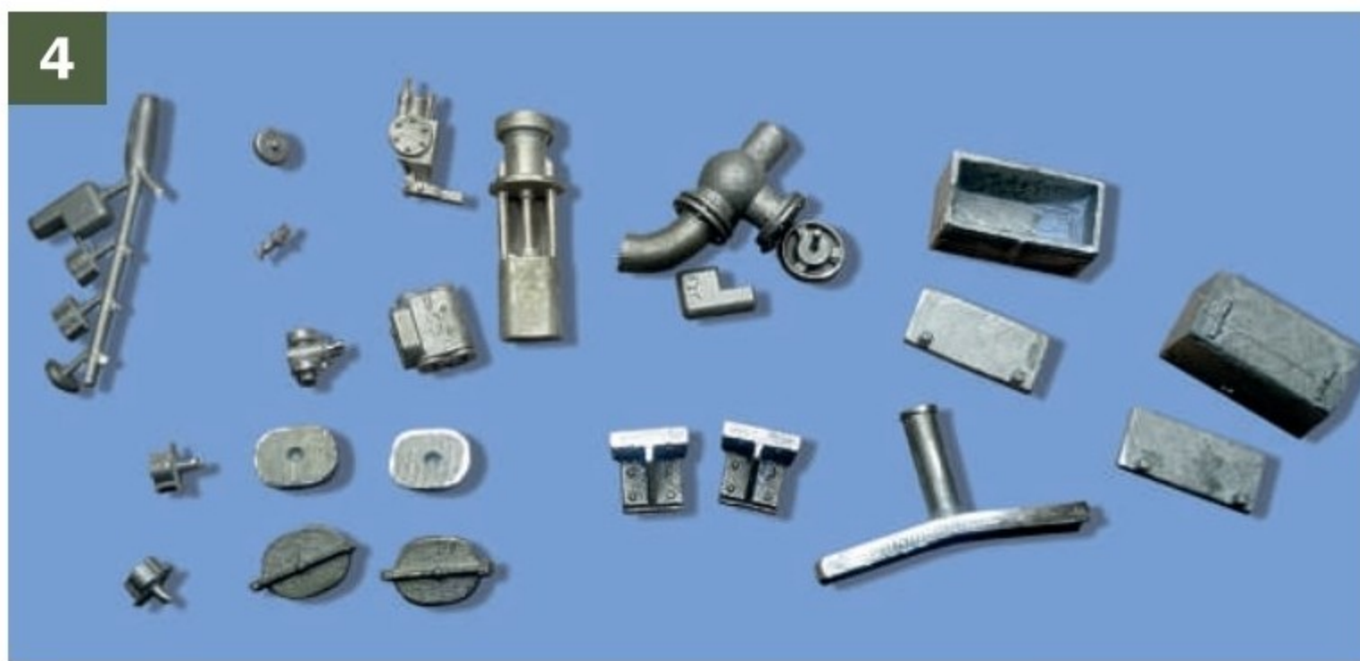
4 The kit includes lost wax castings for fittings that are unique to the '9700', including the Weir pump. The castings come on a number of sprues, and have to be detached and cleaned up. I use a fine piercing saw to cut through the sprues near the casting, so there is less filing required. Here, I have cleaned up those I need – the sprue on the left carries spares.
