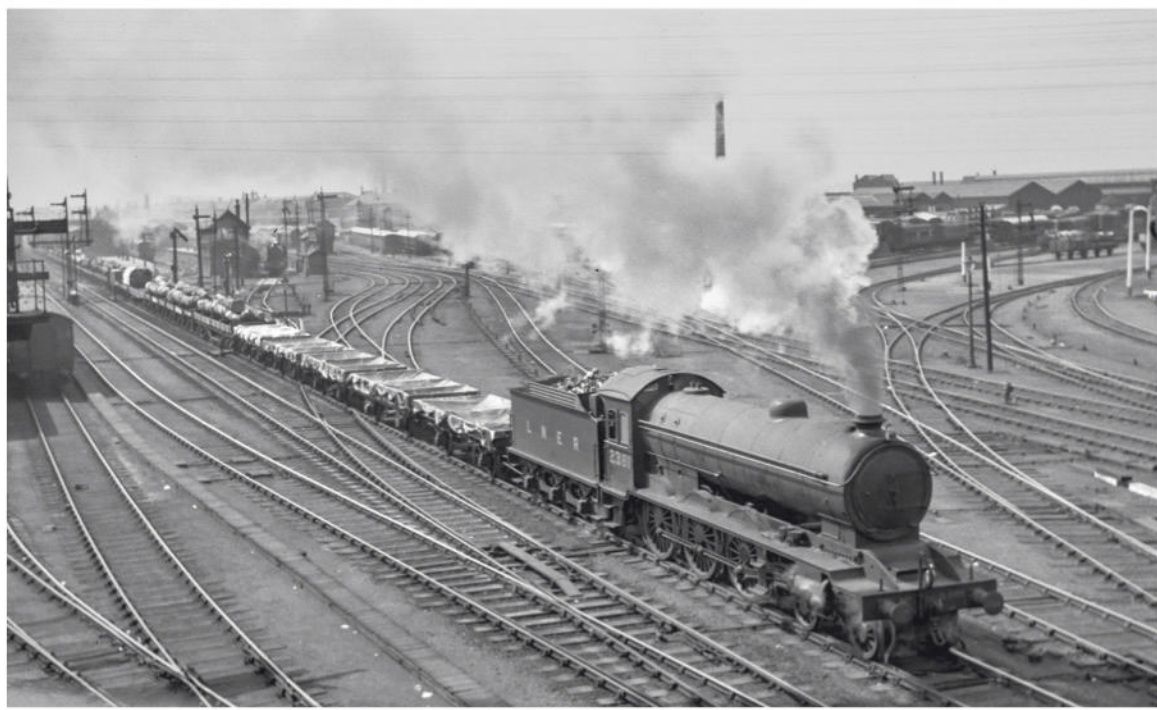
▲ Former North Eastern Railway Class B16 4-6-0 No.2381 passing Doncaster with a goods train on 5 July 1936. The layout will permit the operation of such prototypically long trains. Photo: George Barlow/The Transport Treasury
