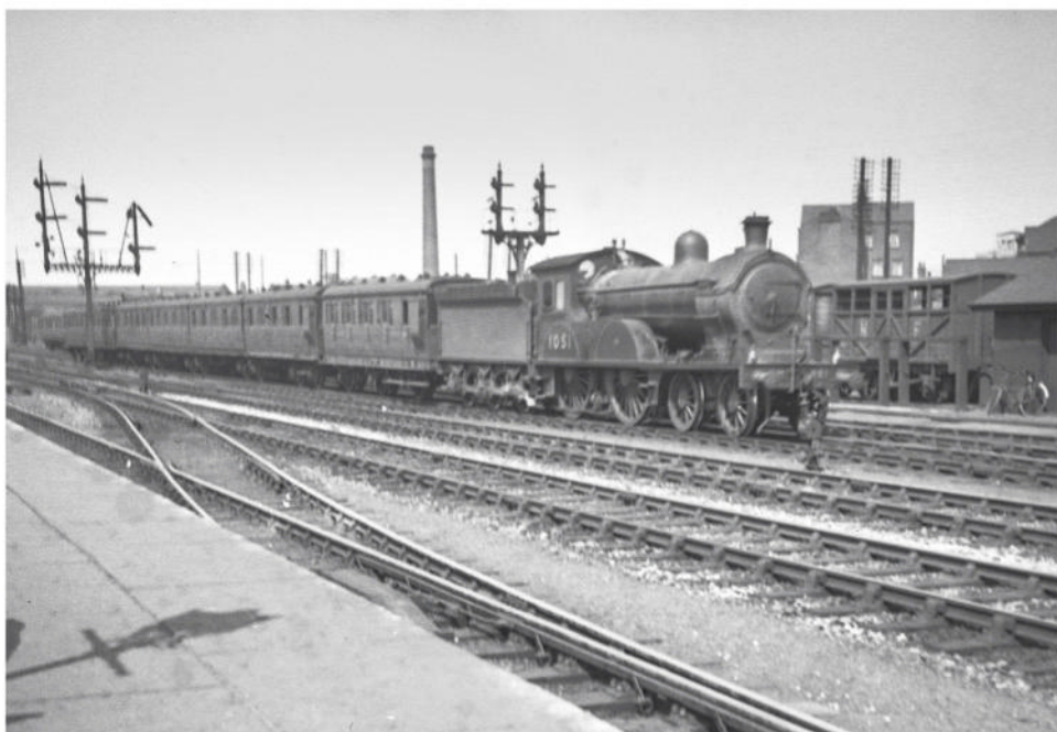
▲ Ex-North Eastern Railway Class D20 4-4-0 No.1051 arriving at Doncaster in 1934. Photo: George Barlow/The Transport Treasury
