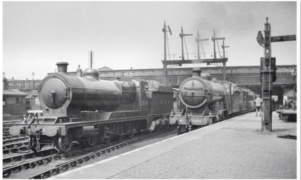
▲ An undated view of Doncaster, with Great Central Railway Robinson 04 2-8-0 No.5354 passing Great Northern Railway Ivatt C1 4-4-2 No.3286. Photo: Mike Morant collection
