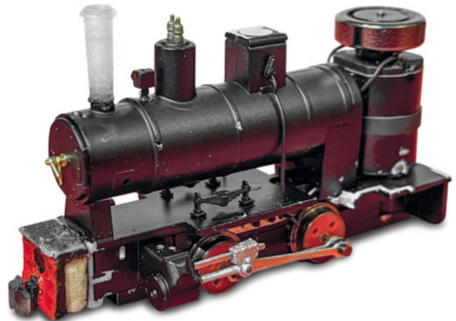
▲ The front bufferbeam was cut and filed back in preparation for the 3D-printed frame extension to be reused from the Mk.I version of the model. This was secured in place with a lump of filler, which was cut back to be flush with the profile of the frames. Little could be done about the exact shape of the cylinders, so I simply pretended not to notice any difference between them and the real things. The new chimney and smokebox dart were also added.
