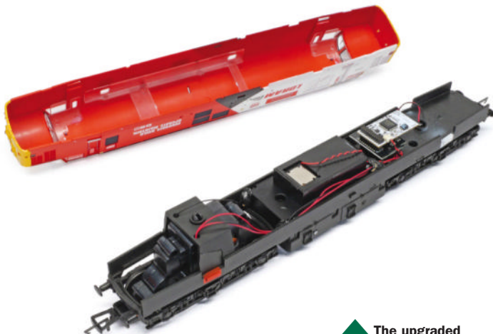
▲ The upgraded chassis includes a 21-pin DCC interface.
