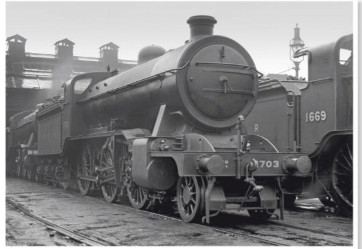
▲ GNR H3 Class 2-6-0 No.1703 at King's Cross shed circa 1922, alongside classmate No.1669. Photo: W J Reynolds/Rail-Online
