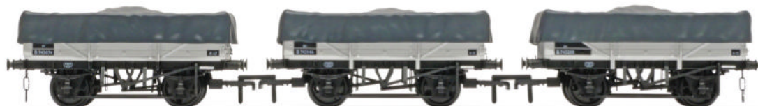
▲ The 'pent' hoods in place on the bauxite wagons.
