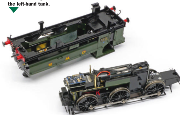
▲ This view shows the resonance chamber and metal weight in the left-hand tank.
