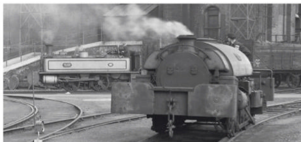
Becton gasworks Nos.12 and 21 (nearest), which conformed to the site's 6" loading gauge. Photo: The Transport Treasury
