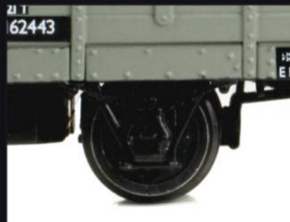
METAL SPOKED OR 3-HOLE DISC WHEELSETS ACCORDING TO PROTOTYPE
