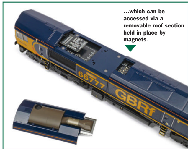
▲ Atop the cast metal chassis block is the Plux22 DCC decoder interface...
