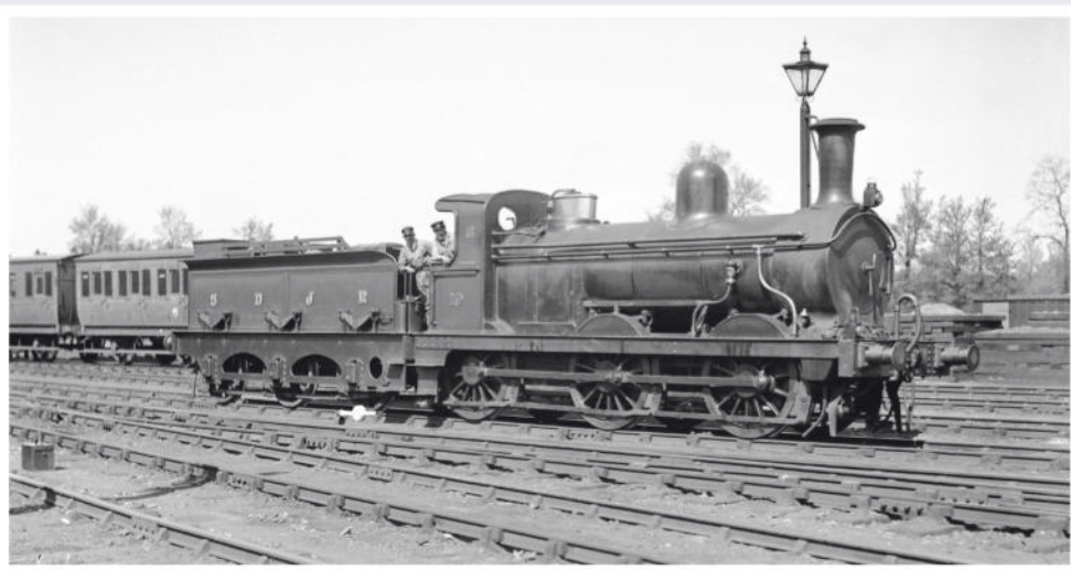
▲ SDJR No.19 was an 0-6-0 tender engine built by John Fowler & Co. of Leeds in 1874 and is depicted in all its finery at Templecombe in 1925. All of this class of six engines had working lives of 54 years, being withdrawn in 1928. Photo: Mike Morant collection
