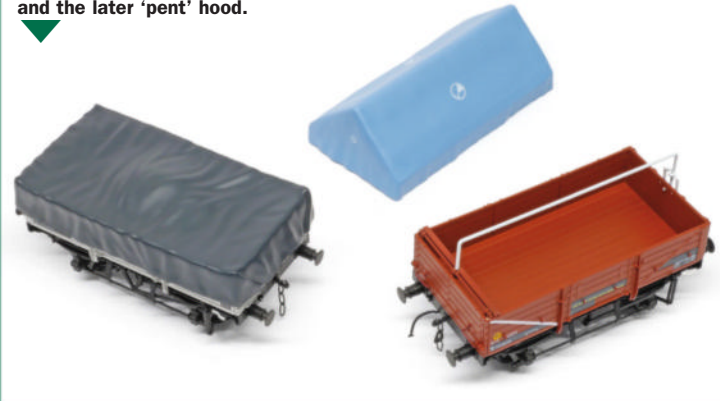
The original tarpaulin sheet (left) and the later 'pent' hood.
