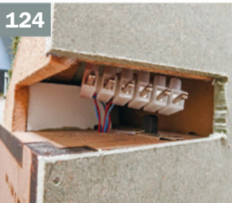
124 Here the inner end of the station board is seen from the rear with the backscene fitted. The cut-outs allow the plug-style terminal blocks (see part two – RM December 2025) to be connected without scrabbling around under the layout. (This arrangement was necessary owing to the intended counter-top display of the model.)
