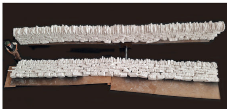
▲ Lengths of dry-stone walling were modelled by fixing individual stones to backing boards. The stones started out as a tray of cast hydrocal lightweight plaster, which was then scribed, cut, and fettled to suit.
