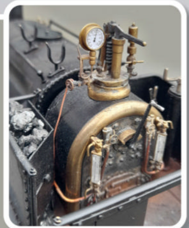
▲ Holy War showing the convincing steam effect (left) and the highly detailed firebox backhead (above).
