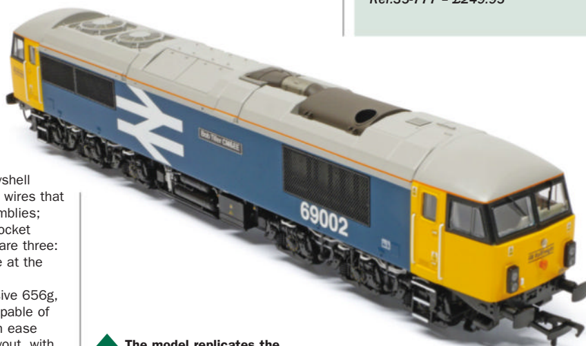
▲ The model replicates the distinctive new roof profile of the rebuilt Class 69s.
