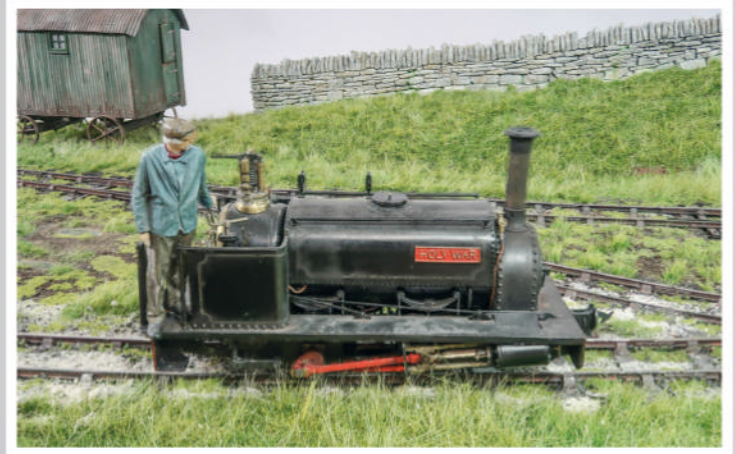
▲ The locomotive that started it all – the Slater's Quarry Hunslet 0-4-0ST, finished as Holy War . The kit comprises etchings, resin parts, castings and turned components.
