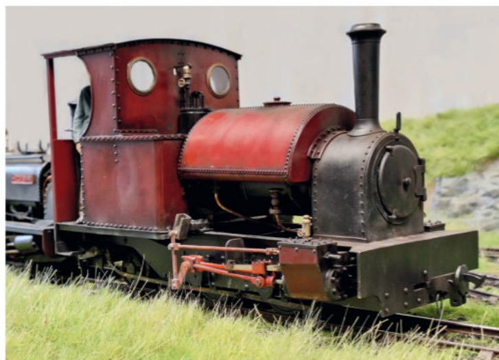
▲ The Kerr Stuart 0-4-2ST, scratch-built using 3D-printed parts and a milled chassis.
