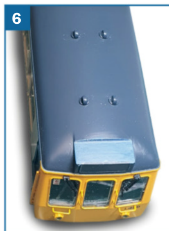
▲ To convert the Class 117 into a 118, the top of the headcode box is cut flat...
