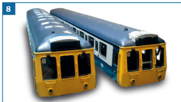
▲ Scrap brass was used to replicate the author's chosen Class 118, which had the headcode boxes plated over on the Driving Motor Second.
