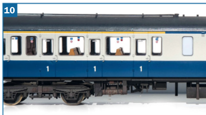
▲ An optional job would be to paint out the yellow First Class stripe and remove the '1s' from the doors, to represent a declassified TCL.
