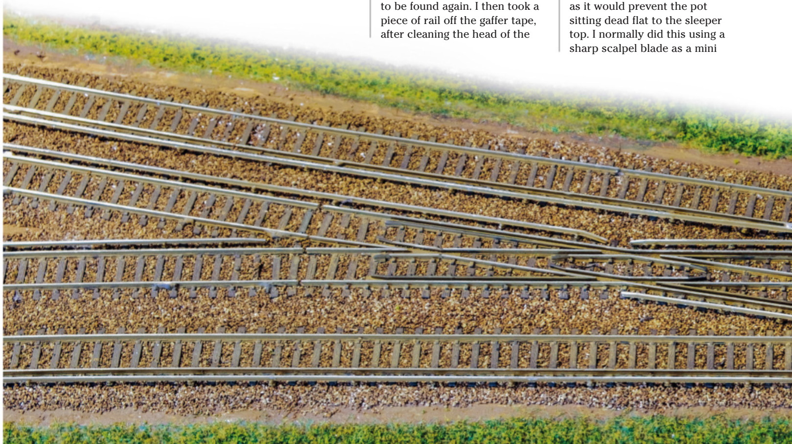
▲ A completed test section of conductor rail, with the 'pots' positioned at every fifth sleeper. The conductor rail is formed using code 40 flat-bottom rail. Photo: author
