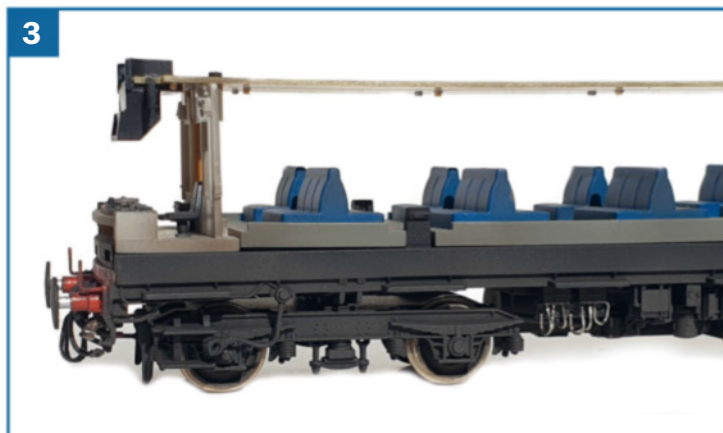
▲ The chassis of the Bachmann Class 117, with some extra details added. It is advisable to disconnect the speedometer cable – visible by the left-hand wheel – to avoid damaging it while working on the model.
