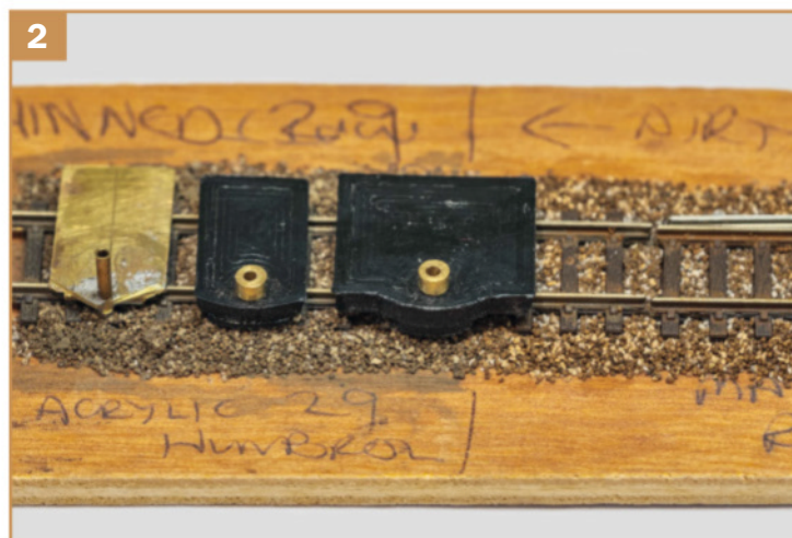
▲ A series of tests led to three iterations of a jig for drilling the sleepers being developed. The brass one on the left was the first, fabricated by the author. 3D-printed nylon ones were then produced by another member of the N Gauge Forum, these enabling the drilling to be undertaken with a far greater degree of accuracy.
