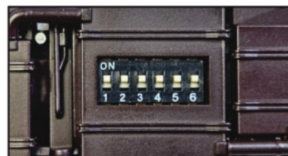
CHASSIS MOUNTED SWITCHES FOR LIGHTING CONTROL
