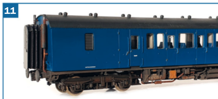
▲ 0.5mm brass wire was used to modify the handrails on the Guard's compartment of the Class 116, making them two parts rather than one.
