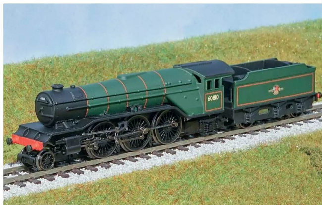
▲ The 3D-printed body of the Gresley V2, fitted to a modified Hornby Gresley A1 Pacific chassis, and finished as No.60810 in BR lined green with late crest.
