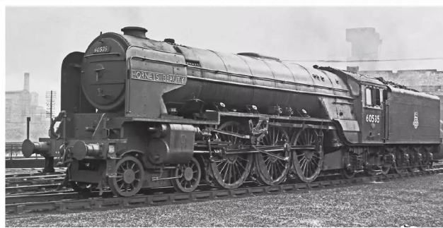
▲ No.60535 Hornets Beauty outside its home shed of Haymarket in Edinburgh on 12 July 1953. The A2s were very similar to the Peppercorn A1s, except for smaller 6' 2" driving wheels. Photo: Rail Photoprints
