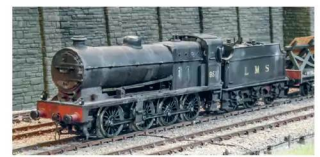
▲ ...which is finished as LMS No. 9517. The model is a Cotswold kit with a milled brass chassis, Mashima motor and High Level 108:1 gearbox. Both photos: Steve Flint
