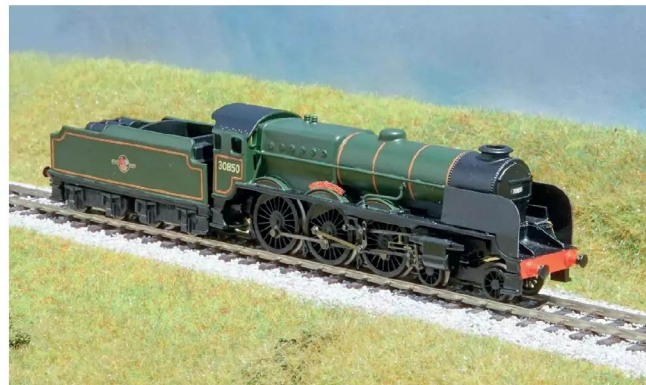
▲ Lord Nelson was modelled in TT:120 using a 3D-printed body from Lincoln Locos, with the tender and its bogies included, and the latter fitted with Jackson wheels.
