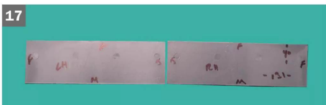
17 The roof sections were made up (each measuring 131mm x 40mm). More notes are evident on the parts, this time 'J' for joint and 'F' denoting a shallow feathered edge at the ends and foot, whilst 'M' is for a mitre (of c.45°) at the top edge.
