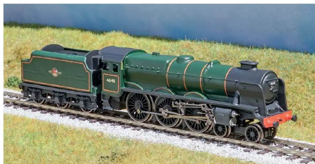
▲ The rebuilt Royal Scot involved fitting Hornby 'Duchess' cylinders and valve gear onto the A1 chassis. Finished as No.46145, it and the A2 will receive nameplates by Silver Tay Models.
